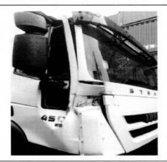
Stacking Machine involved in the Incident and Damage Prime Mover XD8263A
