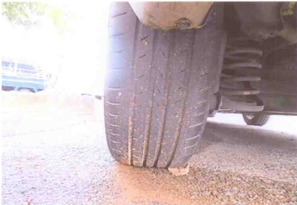
Photo 12 shows the condition of the rear left tyre of the Motor Car, which was observed to be in serviceable condition with remaining tread depth of approximately 6mm. The tyre, which was wrapped around alloy wheel rim, was also observed to be sufficiently inflated for vehicular operation.
