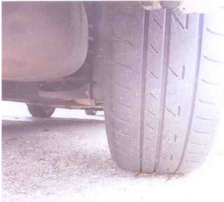
Photo 13 shows the condition of the rear right tyre of the Motor Car, which was observed to be in serviceable condition with remaining tread depth of approximately 6mm. There was also no tear, cut or burst mark(s) on the outer and the inner sidewalls as well as across the tread of the 4 tyres.
