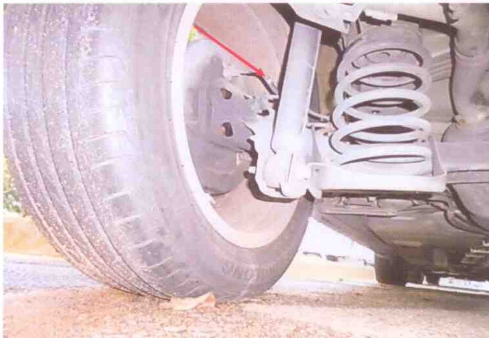
Photo 18 shows the brake hose (arrowed) at the rear left wheel of the Motor Car. We did not observe any leakage of brake fluid at the time of our inspection of the Motor Car. Our visual inspection of the various mechanical components of the Motor Car's braking system revealed all to be intact and without visible damage, indicating that the braking system was likely to be in serviceable condition at the material time of accident.
