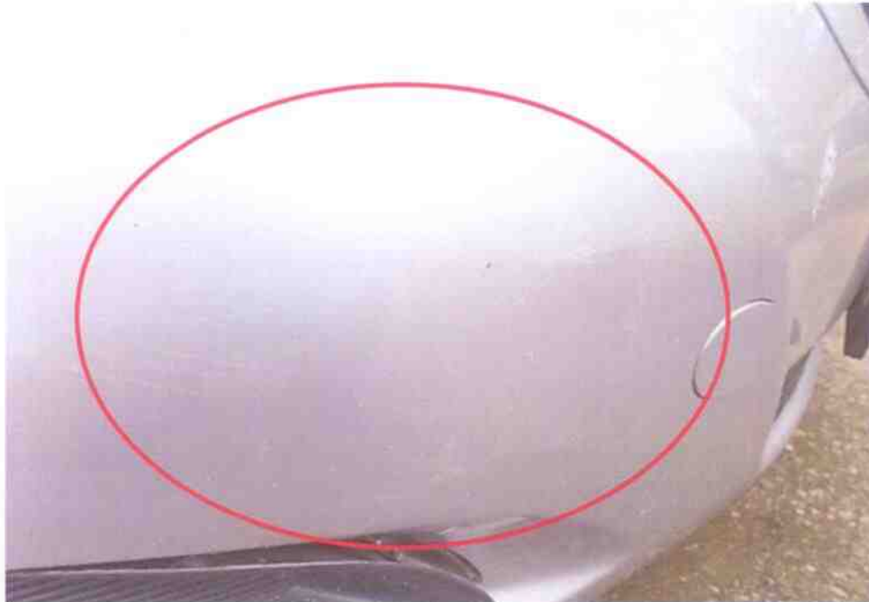
Photo 7 shows a close up view of the front bumper of the Motor Car at the time of our inspection. It was observed to be with deformation marks.
