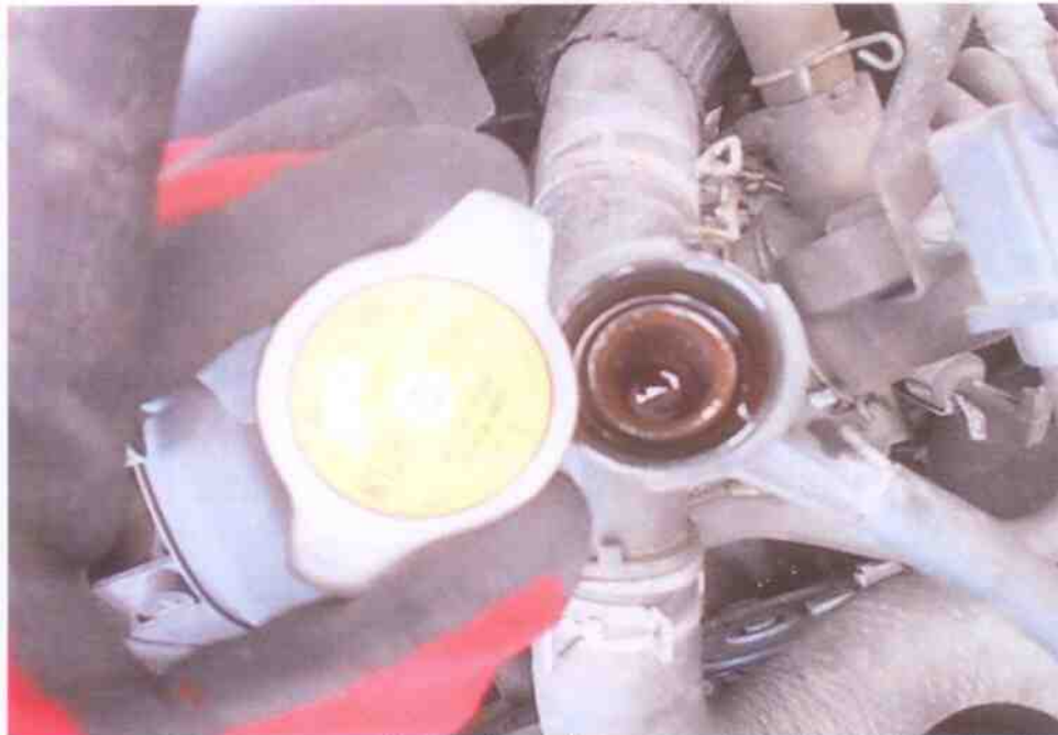
Photo 16 shows the coolant fluid in the radiator tank of the Motor Car at the time of our inspection. The coolant fluid was observed to be of sufficient level and without any visible contamination.
