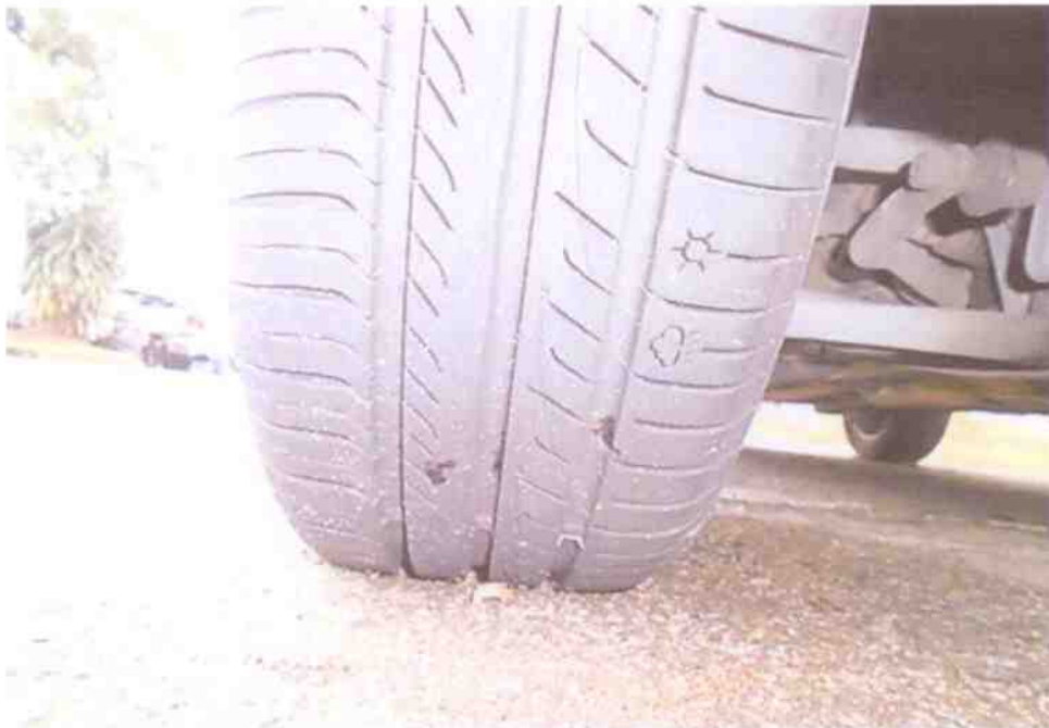
Photo 11 shows the condition of the front right tyre of the Motor Car, which was observed to be in serviceable condition with remaining tread depth of approximately 7mm. The tyre, which was wrapped around alloy wheel rim, was also observed to be sufficiently inflated for vehicular operation.
