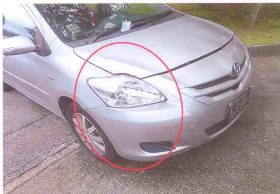
Photo 4 shows a semi close up view of the front left of the Motor Car at the time of our inspection. The Motor Car had sustained relatively minor impact at the front left of the Motor Car.
