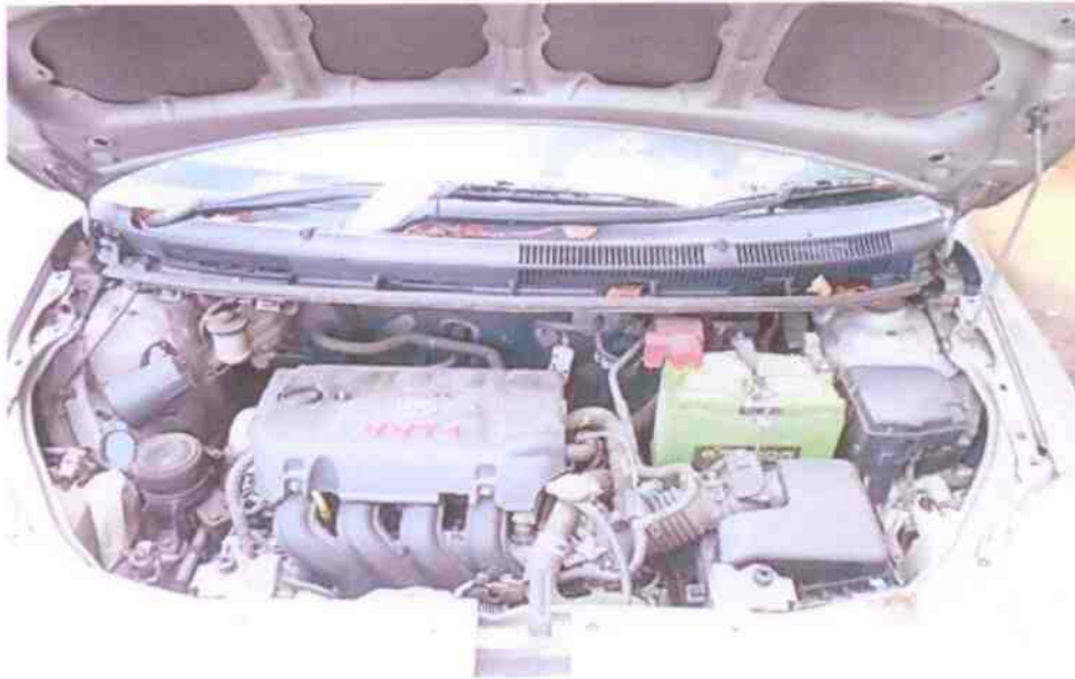
Photo 14 shows a general view of the Motor Car's engine compartment. The various parts and components inside the engine compartment were unaffected by the accident. There was also no sign(s) or indication(s) of fluid leakage and/or fluid stain within the engine compartment.
