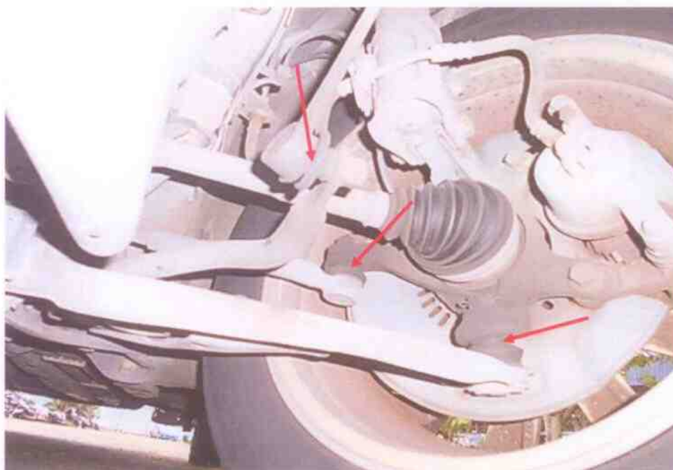
Photo 20 shows the various undercarriage components at the front left wheel of the Motor Car, in particular the steering tie rod (arrowed). The various steering components were all found to be intact, suggesting that the steering system of the Motor Car was likely to be in serviceable condition.
