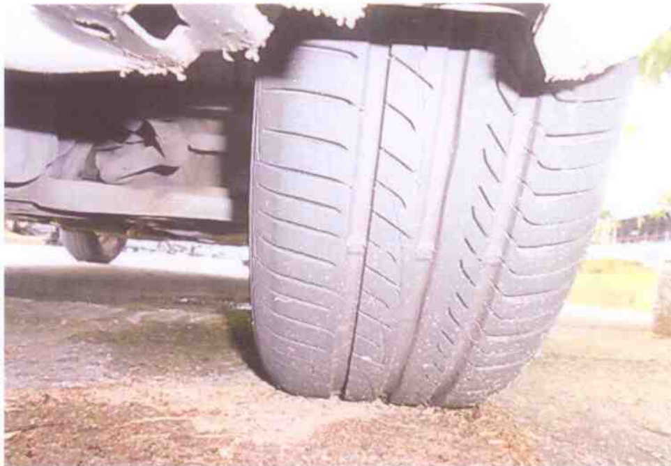
Photo 10 shows the condition of the front left tyre of the Motor Car, which was observed to be in serviceable condition with remaining tread depth of approximately 7mm. The tyre, which was wrapped around alloy wheel rim, was also observed to be sufficiently inflated for vehicular operation. There was no tear, cut or burst mark(s) on the outer and the inner sidewalls as well as across the tread of the 4 tyres.
