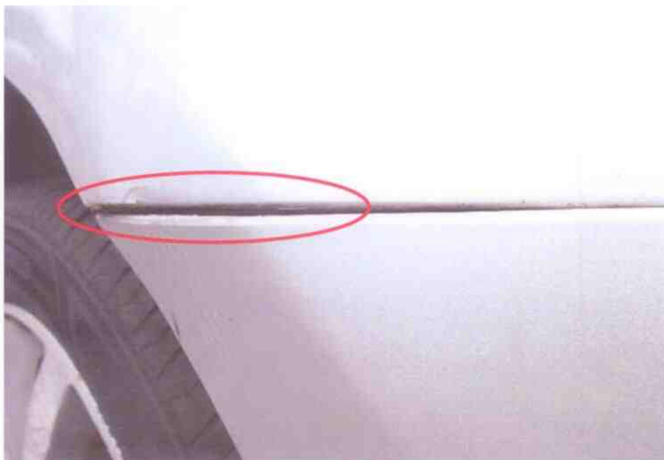
Photo 8 shows a close up view of the front bumper of the Motor Car at the time of our inspection. It was observed to be misaligned.
