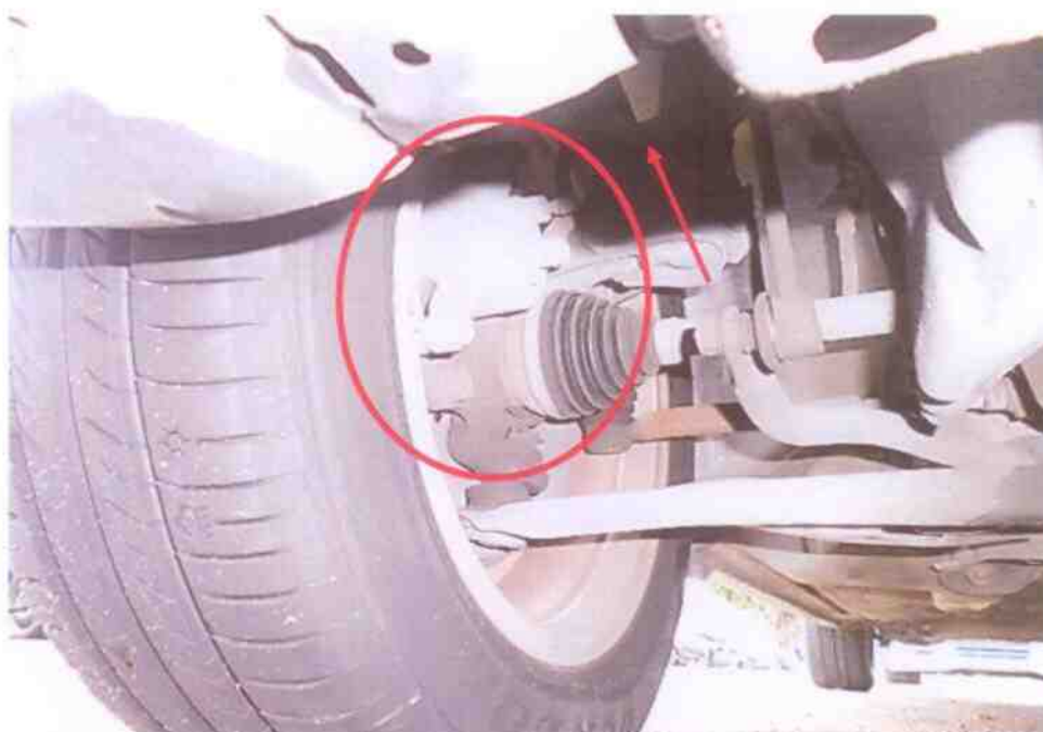
Photo 19 shows the brake hose (arrowed) at the front right wheel of the Motor Car. We did not observe any leakage of brake fluid at the time of our inspection of the Motor Car. Our visual inspection of the various mechanical components of the Motor Car's braking system, including its brake calliper (circled), revealed all to be intact and without visible damage, indicating that the braking system was likely to be in serviceable condition at the material time of accident.
