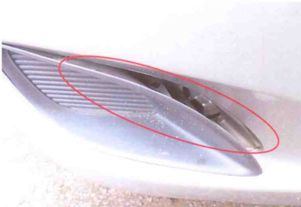
Photo 6 shows a close up view of the spot light garnish of the Motor Car at the time of our inspection. It was observed to be dislodged from its original installation.
