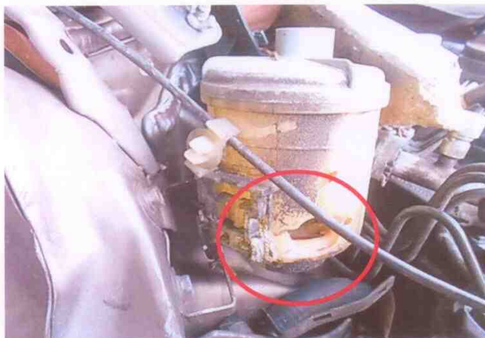
Photo 22 shows the close up view of the steering fluid reservoir that was broken likely due to the accident impact.
