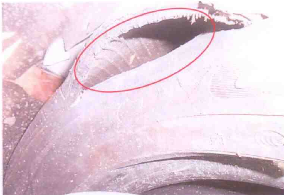
Photo 17 shows the condition of the front left tyre of the Motor Car, which was observed to be torn due to the accident's impact.
