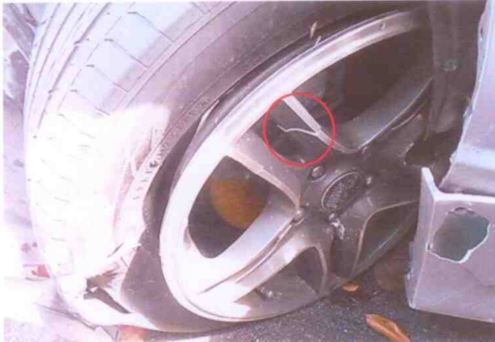
Photo 18 shows the condition of the front left wheel rim of the Motor Car, which was observed to be damaged due to the accident's impact.
