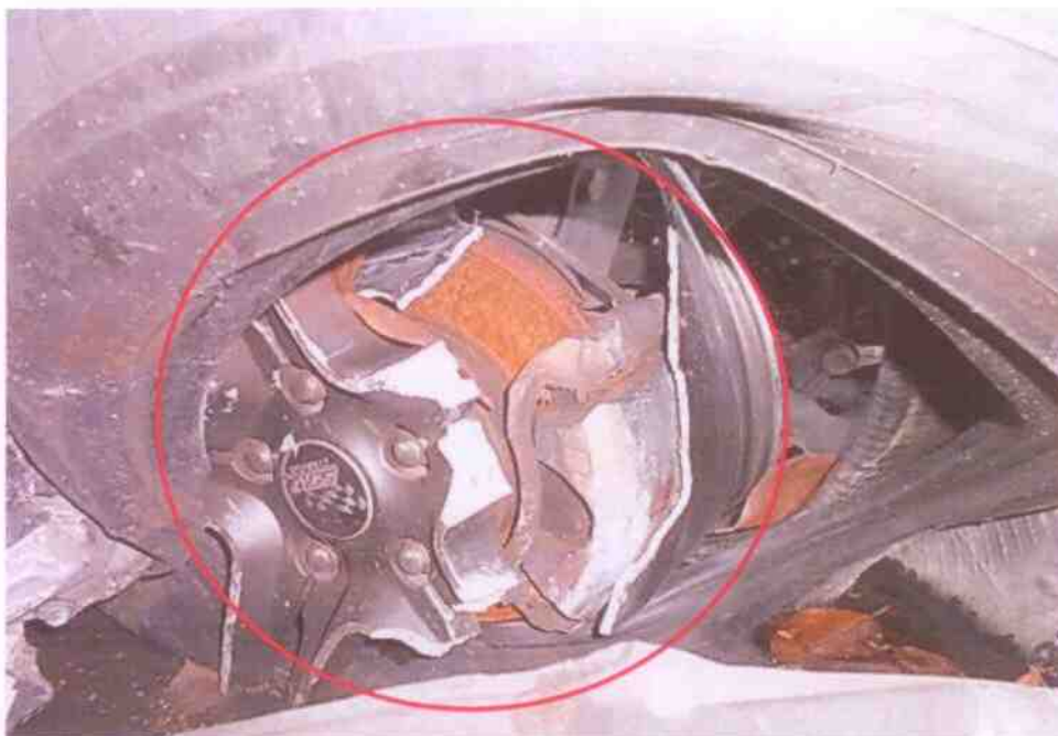
Photo 15 shows the condition of the front right wheel rim of the Motor Car, which was observed to be damaged due to the accident's impact.
