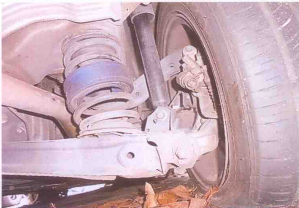
Photo 27 shows the braking & steering components at the rear right wheel of the Motor Car. We did not observe any leakage of brake fluid at the time of our inspection of the Motor Car.
