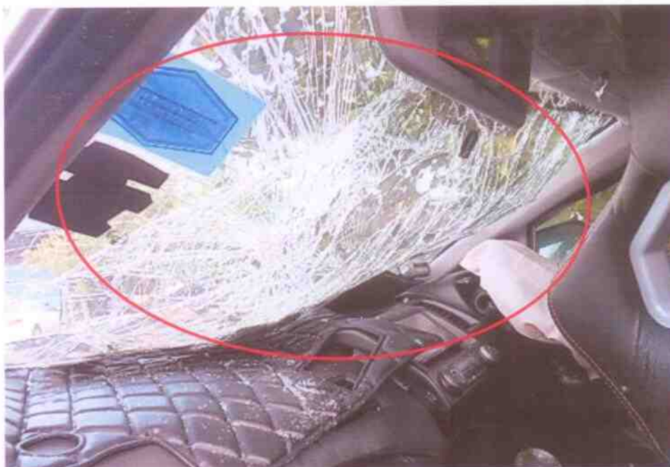
Photo 8 shows a closer view of the damage at the windscreen area of the Motor Car. The impact force was significant, causing the windscreen to sustain a shattering cracked.
