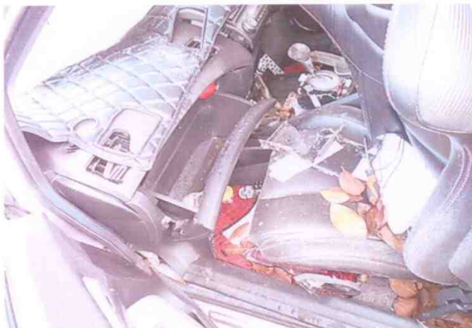
Photo 9 shows a closer view of the left front passenger seat of the Motor Car. The impact force was significant, causing the components such as driver & passenger's seat, glove compartment, gear knob assembly amongst others to be damaged likely due to the accident's impact collision.
