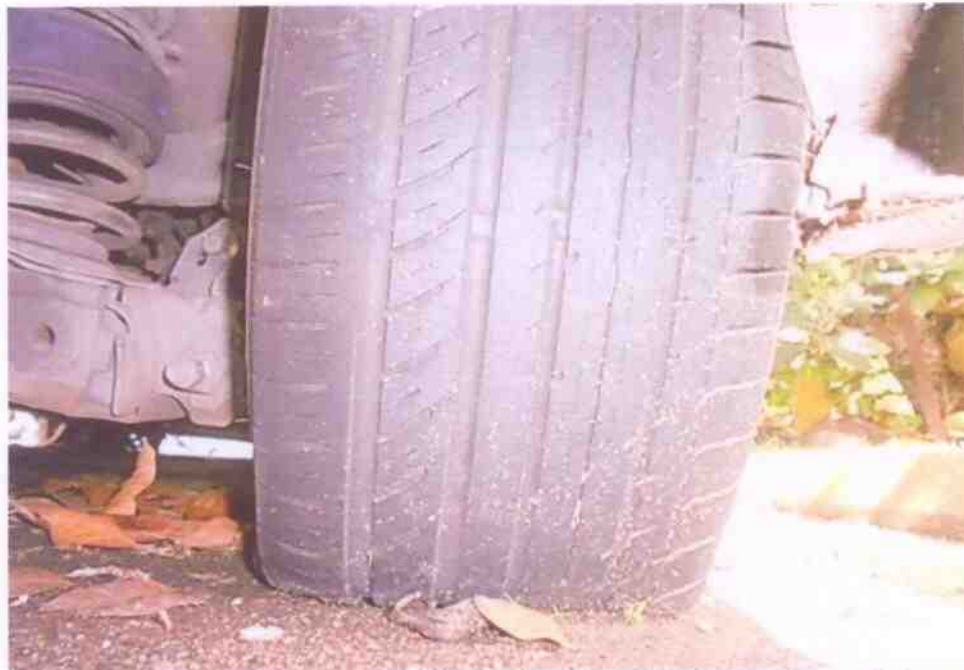
Photo 20 shows the condition of the rear right tyre of the Motor Car, which was observed to be deflated likely due to the accident's collision impact.
