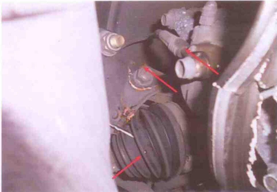
Photo 26 shows the damaged on the front left drive shaft of the Motor Car. We were not able to conduct any tests on the steering system of the Motor Car due to the damage to this components, as well as leakage of fluids.
