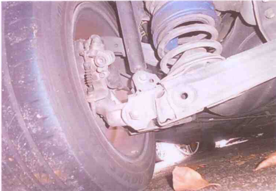
Photo 28 shows the braking & steering components at the left right wheel of the Motor Car. We did not observe any leakage of brake fluid at the time of our inspection of the Motor Car.
