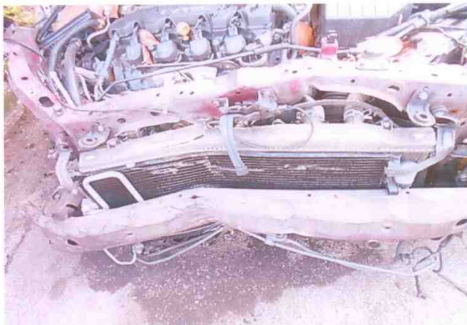
Photo 6 shows a closer view of the damage at the frontal portion of the Motor Car. The impact force was significant, causing the various parts and components inside the engine compartment to be pushed inwards, towards the rear of the Motor Car.
