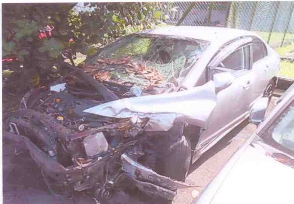
Photo 3 shows a general view of the front left portion of the Motor Car at the time of our inspection. The Motor Car was observed to have sustained with extensive impact damage at its frontal portion.
