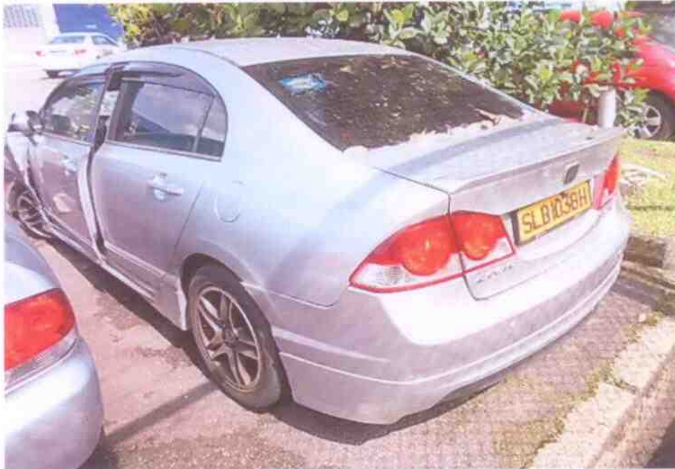
Photo 10 shows a general view of the rear left portion of the Motor Car. The rear portion was observed to be in good condition, no damages found at time of our inspection.
