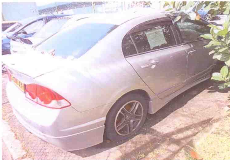
Photo 11 shows a general view of the rear right portion of the Motor Car. The rear portion was observed to be in good condition, no damages found on the Motor Car's body at time of our inspection. However, we found that the rear right tyre was deflated due to the accident.
