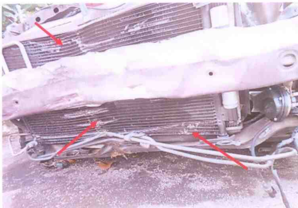
Photo 21 shows the close up view of the radiator's tank that was observed to be damaged likely due to the accident impact.
