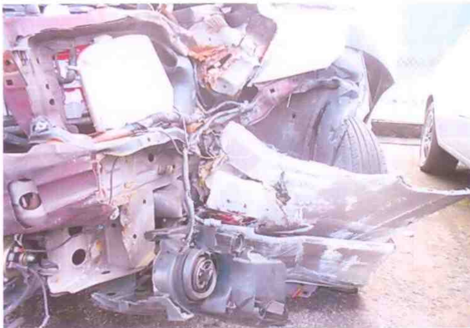
Photo 4 shows a closer view of the damage at the frontal portion of the Motor Car's engine. The impact force was significant, causing the various parts and components inside the engine compartment to be pushed inwards, towards the rear of the Motor Car.
