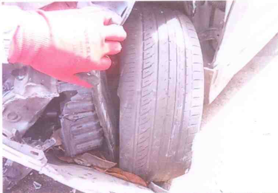
Photo 16 shows the condition of the front left tyre of the Motor Car. The tread patterns were obvious visually. The remaining tread depth of the front left tyre was approximately 3mm.
