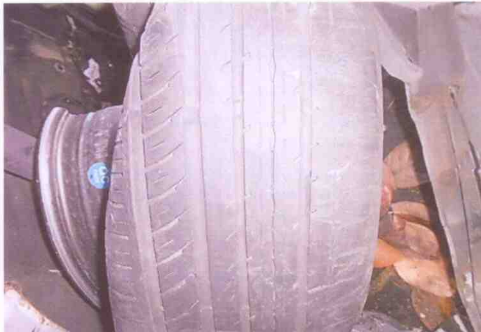
Photo 13 shows the condition of the front right tyre of the Motor Car. The tread patterns were obvious visually. The remaining tread depth of the front left tyre was approximately 3mm.
