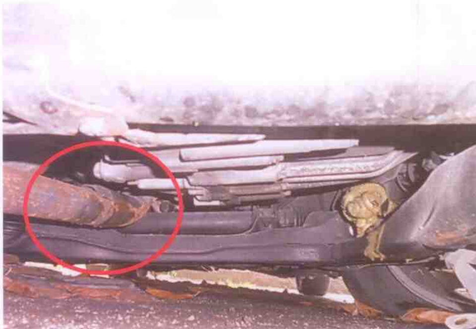
Photo 23 shows the close up view of the fluid leakage at the undercarriage area likely due to the accident impact.
