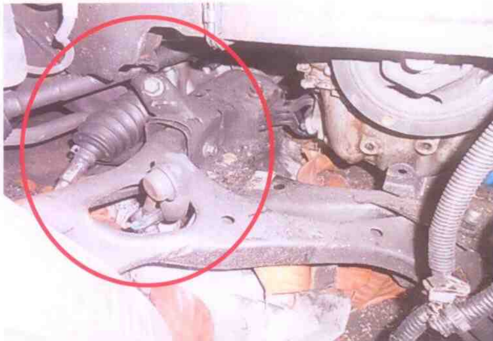
Photo 25 shows a close up view on the front right drive shaft of the Motor Car. We were not able to conduct any tests on the steering system of the Motor Car due to the damage to this components, as well as leakage of power steering fluid.
