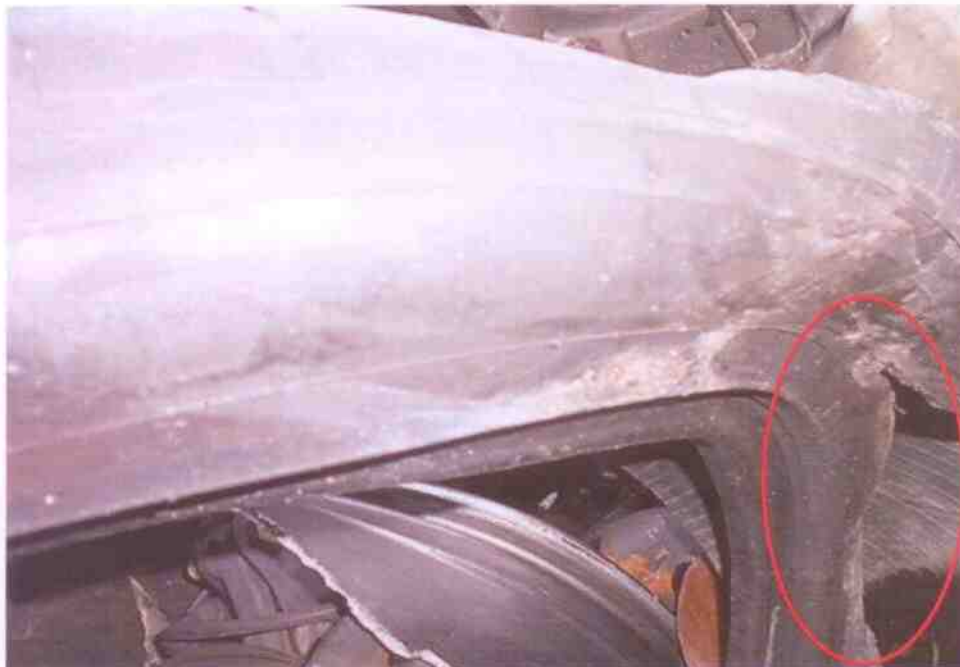
Photo 14 shows the condition of the front right tyre of the Motor Car, which was observed to be torn due to the accident's impact.
