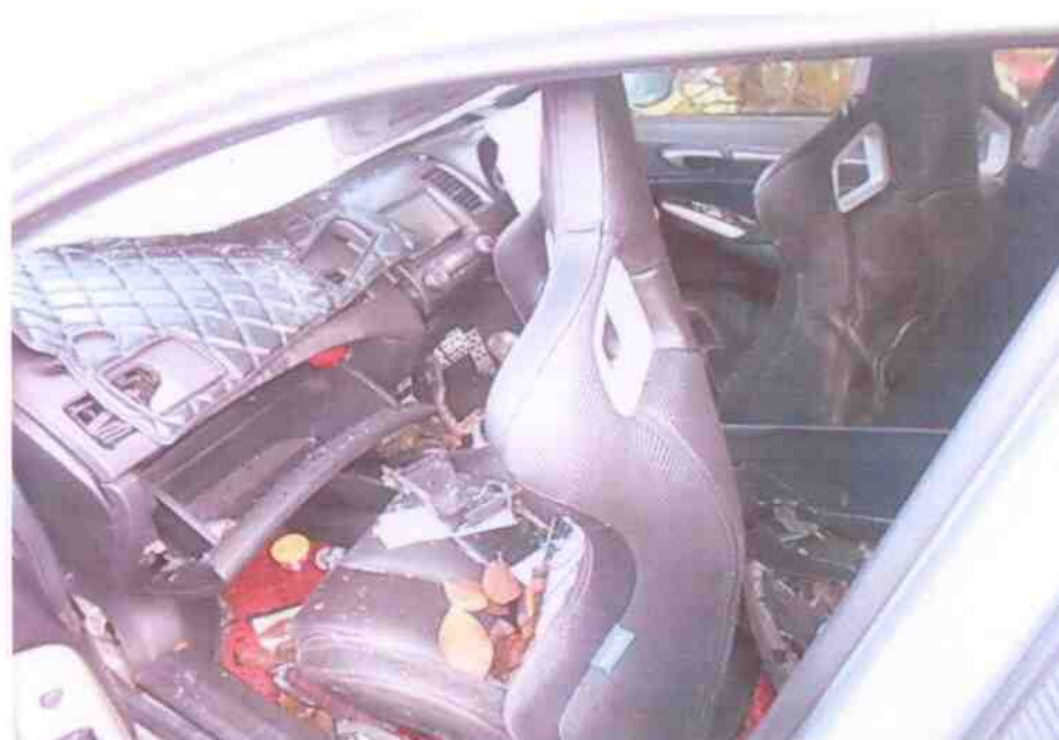
Photo 7 shows a closer view of the left front passenger seat of the Motor Car. The impact force was significant, causing the components such as driver & passenger's seat, glove compartment, gear knob assembly amongst others to be damaged likely due to the accident's impact collision.
