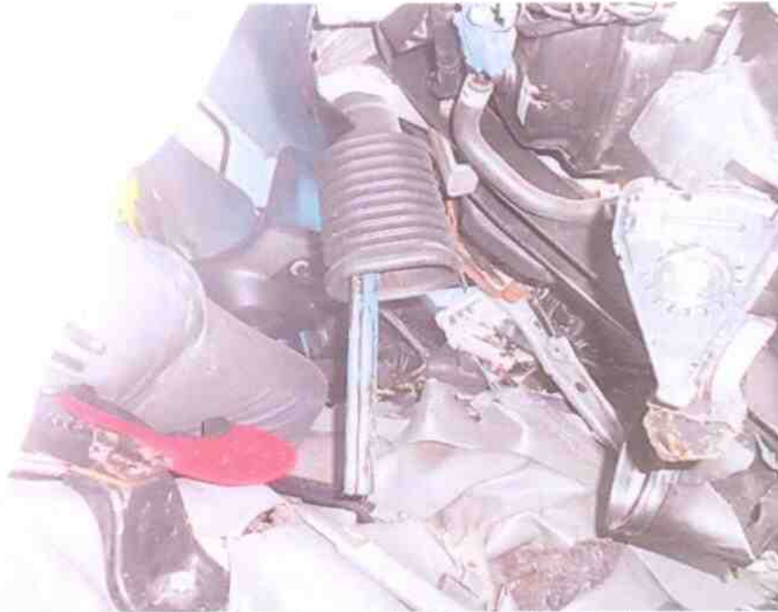
Photo 5 shows the interior of the front cabin. The dashboard, steering wheel, seats, floor panel and roof panel inside the front cabin were all observed to be pushed/buckled inwards, towards the rear of the Motor Lorry. This is consistent to the nature of this accident where the direction of impact onto the Motor Lorry was from the front to rear direction.
