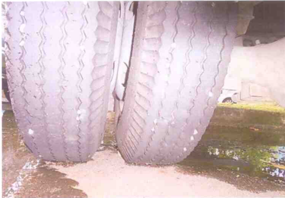
Photo 8 shows the condition of the rear right tyres of the Motor Lorry, which was observed to be in serviceable condition with remaining tread depth of approximately 5mm. There was no tear, cut or burst mark(s) on the outer and the inner sidewalls as well as across the tread of this 2 tyres. The tyres, which was wrapped around alloy wheel rim, was also observed to be sufficiently inflated for vehicular operation.
