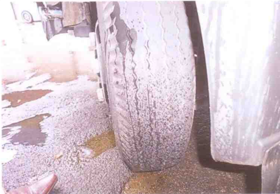
Photo 10 shows the condition of the front left tyre of the Motor Lorry, which was observed to be in serviceable condition with remaining tread depth of approximately 5mm. There was also no tear, cut or burst mark(s) on the outer and the inner sidewalls as well as across the tread of this tyre.
