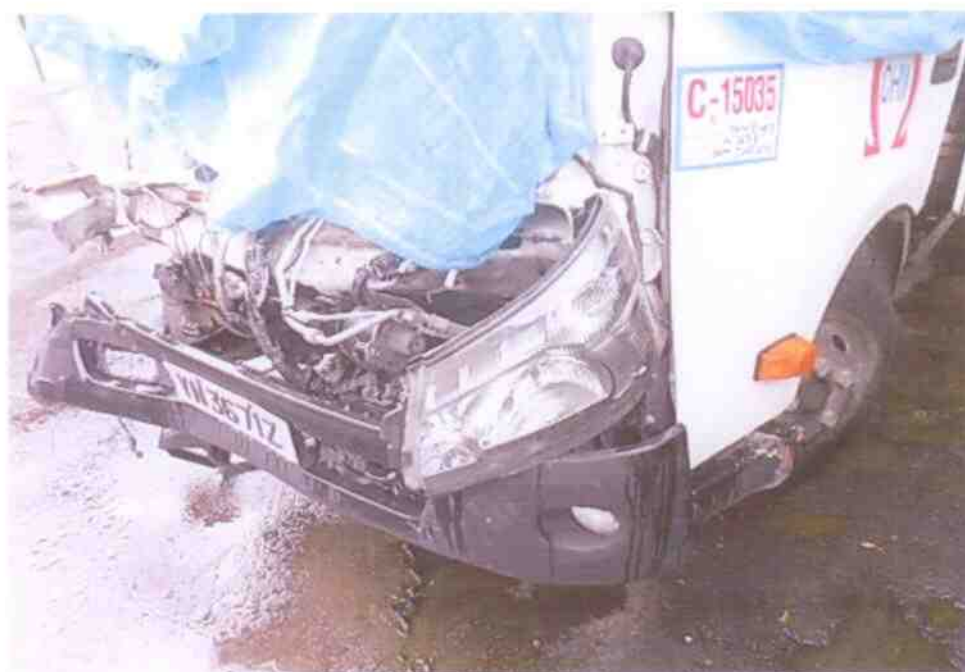
Photo 4 shows a general view of the front right portion of the Motor Lorry at the time of our inspection. The Motor Lorry was observed to have sustained extensive impact damage at its front left portion. The impact force was relatively significant, causing its entire front cabin to be buckled and crumpled.
