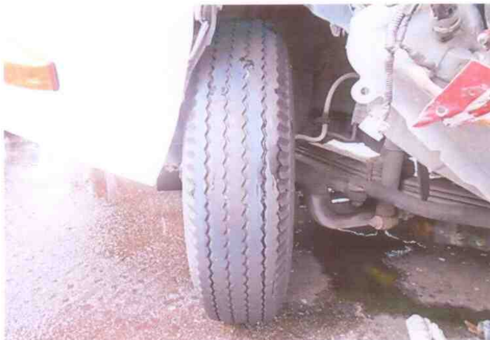
Photo 11 shows the condition of the front right tyre of the Motor Lorry. The front right tyre was observed to be in serviceable condition with remaining tread depth of approximately 5mm. There was also no tear, cut or burst mark(s) on the outer and the inner sidewalls as well as across the tread of this tyre.
