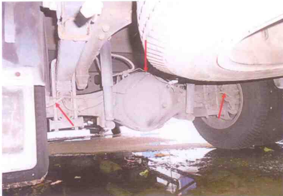
Photo 16 shows the brake hose (arrowed) at the rear right wheel of the Motor Lorry. At the time of our inspection, we did not find any sign(s) of brake fluid leakage along the brake hoses and brake pipes.
