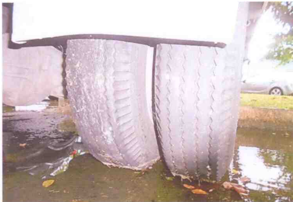
Photo 9 shows the condition of the rear left tyres of the Motor Lorry, which was observed to be in serviceable condition with remaining tread depth of approximately 5mm. There was no tear, cut or burst mark(s) on the outer and the inner sidewalls as well as across the tread of these 2 tyres, which were also observed to be sufficiently inflated for vehicular operation.
