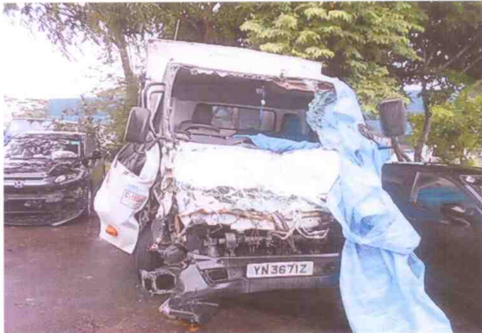
Photo 1 shows a general view of the frontal portion of the Motor Lorry at the time of our inspection. The Motor Lorry was observed to have sustained extensive impact damage at its frontal portion. The impact force was relatively significant, causing its entire front cabin to be buckled and crumpled.
