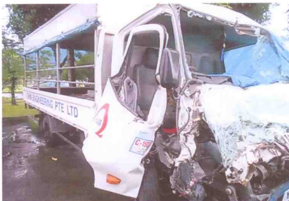
Photo 3 shows a general view of the front left portion of the Motor Lorry at the time of our inspection. The Motor Lorry was observed to have sustained extensive impact damage at its front left portion. The impact force was relatively significant, causing its entire front cabin to be buckled and crumpled.
