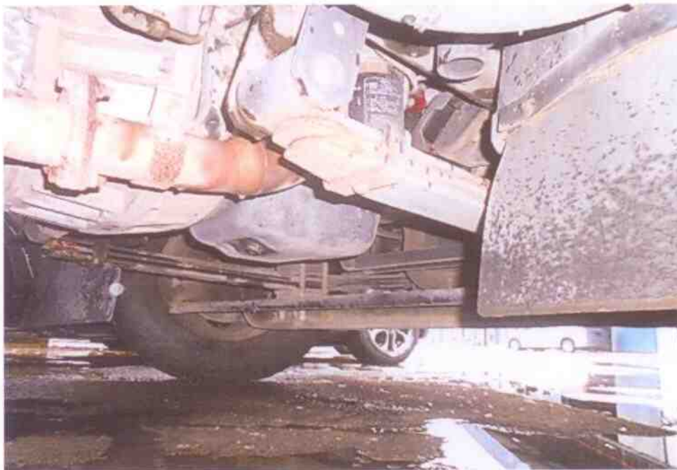
Photo 12 shows the underside of the Motor Lorry, at the area where the engine is located. We were not able to closely inspect the engine compartment of the Motor Lorry due to the extensive damage to its front cabin. Our visual checks from the underside had however appear to indicate that the engine assembly and transmission assembly were both intact and unaffected by the collision.
