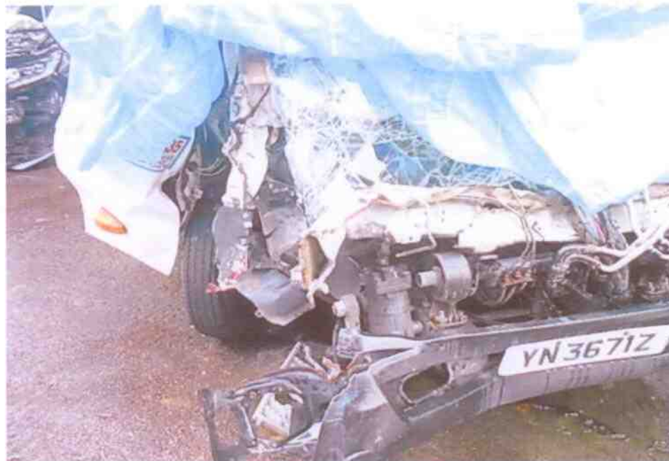
Photo 2 shows a closer view of the frontal portion of the Motor Lorry at the time of our inspection. A number of mechanical parts and components at the frontal portion were also severely damaged as a result of the accident.
