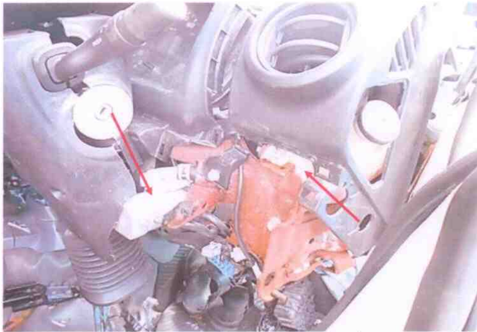
Photo 18 shows the damages on the brake fluid reservoir as a result of the accident.
