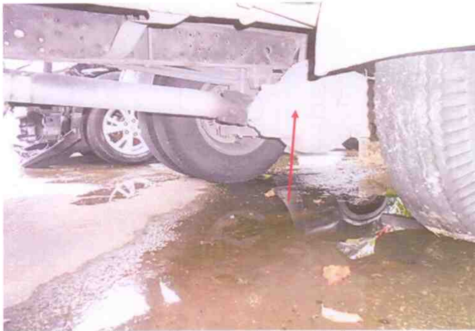
Photo 13 shows the transmission assembly (arrowed) of the Motor Lorry intact and unaffected by the collision.
