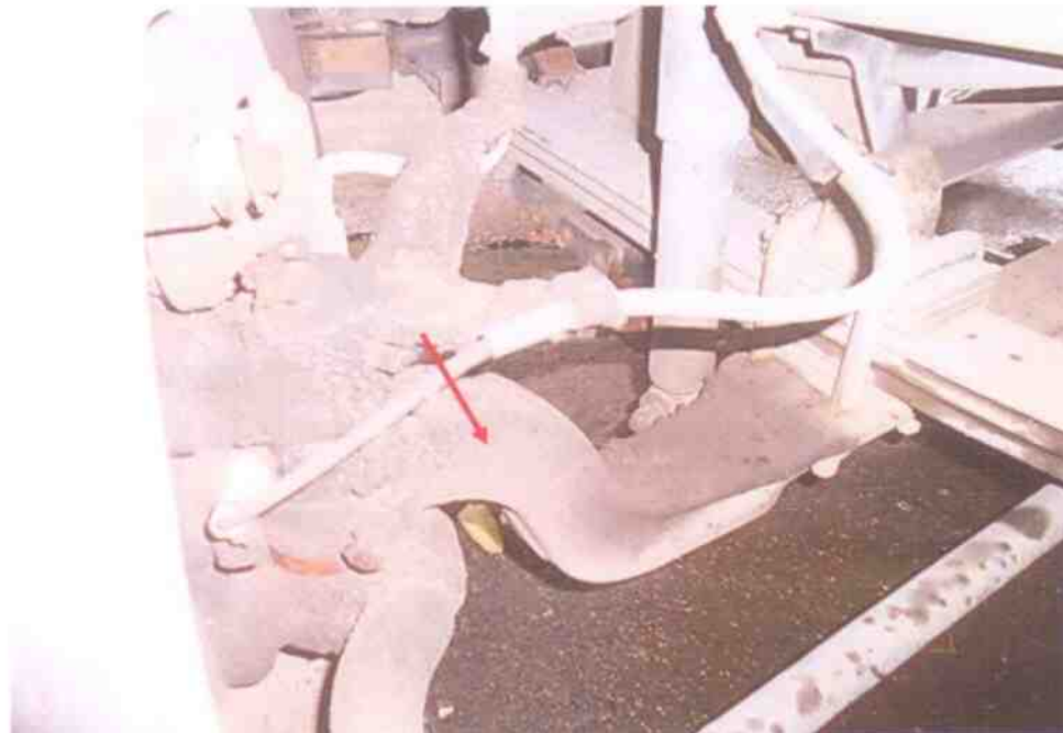
Photo 15 shows the undercarriage components at the front left wheel of the Motor Lorry. The various undercarriage components of the Motor Lorry were all observed to be intact and without any visible damage. This had included the steering rack (arrowed) of the Motor Lorry.
