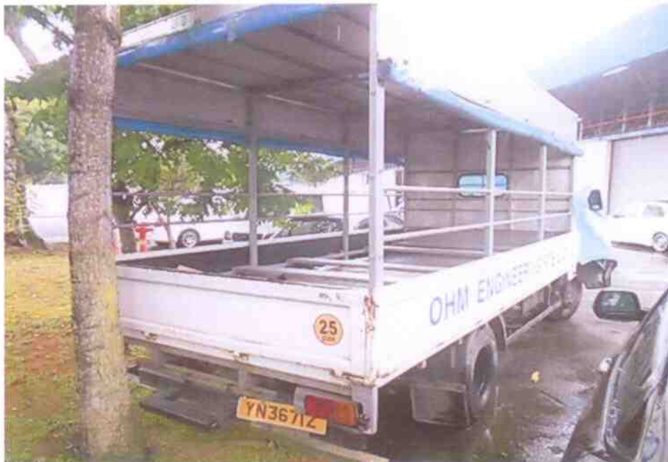
Photo 6 shows a general view of the rear right portion of the Motor Lorry at the time of our inspection. The rear portion was observed to be relatively unaffected by the accident.
