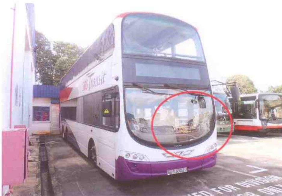
Photo 2 shows a general view of the front right body of the Motor Bus at the time of our inspection. The Motor Bus was observed to have sustained relatively minor damage at its front body. Its windshield was observed to be cracked.
