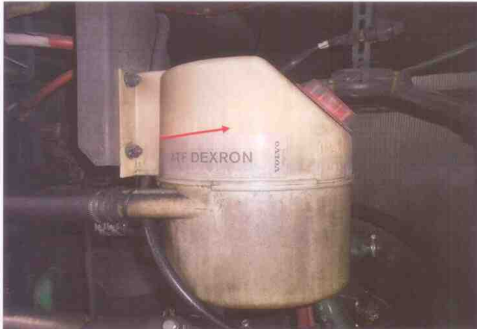
Photo 14 shows the Auto Transmission fluid of the Motor Bus. It was observed to be of sufficient level without any contamination at time of our inspection.
