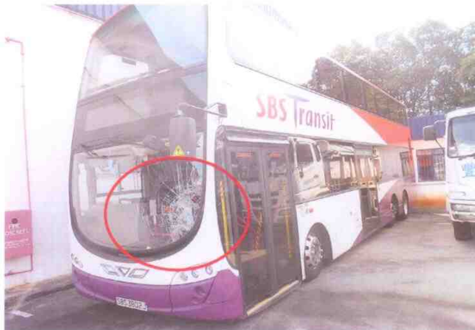
Photo 3 shows a general view of the front left body of the Motor Bus at the time of our inspection. The Motor Bus was observed to have sustained relatively minor damage at its front body. Its windshield was observed to be cracked.
