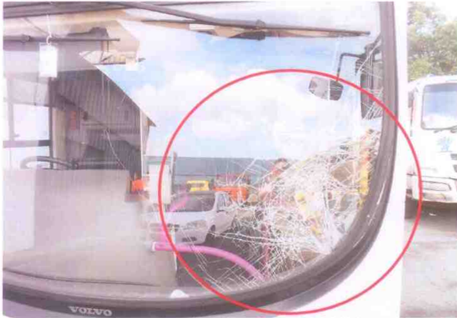
Photo 5 shows a close-up view of the Motor Bus's windshield. It was observed to be cracked likely due to the accident's impact.
