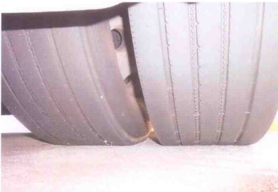
Photo 12 shows the condition of the rear left tyres (centre axle) of the Motor Bus, which were observed to be in serviceable condition with remaining tread depth of approximately 4mm. The tyres, which were wrapped around standard alloy wheel rims, were also observed to be sufficiently inflated for vehicular operation.
