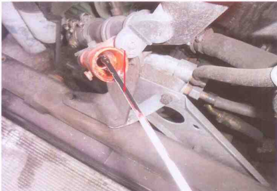
Photo 15 shows the engine fluid of the Motor Bus. It was observed to be of sufficient level without any contamination at time of our inspection.
