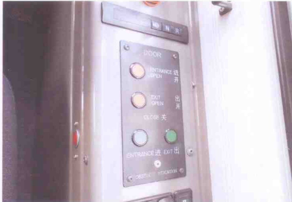
Photo 23 shows the indicators at the driver's seat. Other operational indicators were unable to be initialized due to the flat battery. Hence, no test was carried out to the Motor Bus additional devices.
