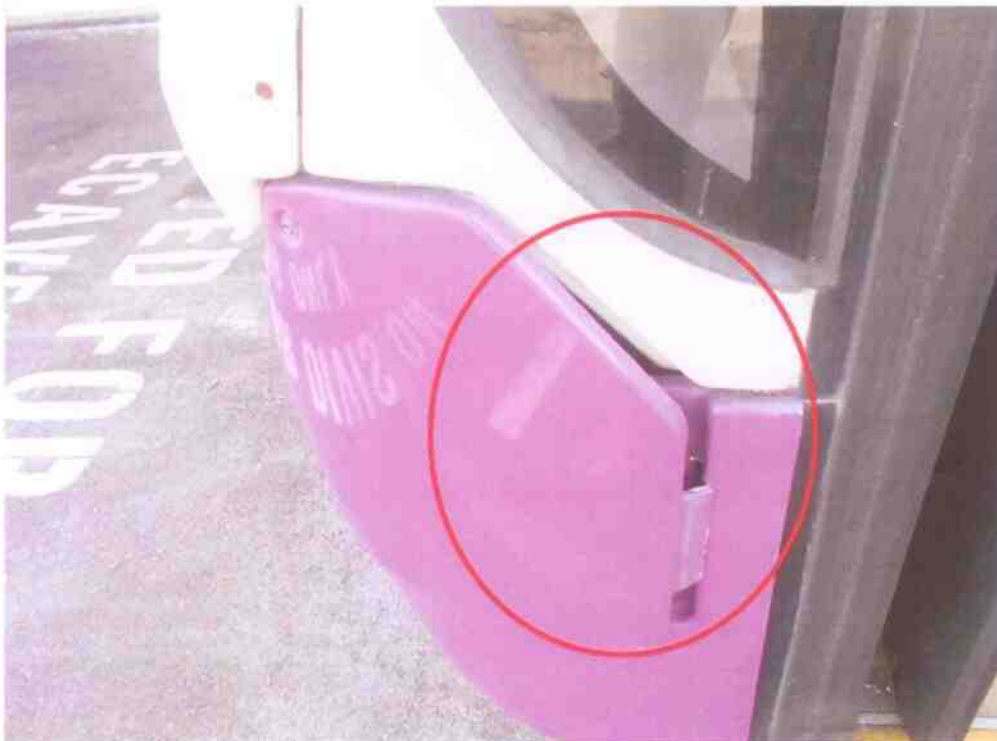
Photo 6 shows a close-up view of the Motor Bus's left hand lower bumper. It was observed to be misaligned likely due to the accident's impact.
