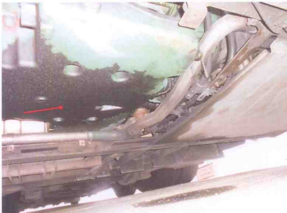
Photo 17 shows the engine underside of the Motor Bus. It was observed to be sighted with fluid leakage. However it was noted to be a pre-existed fluid leakage due to the dust stain that associated with it.
