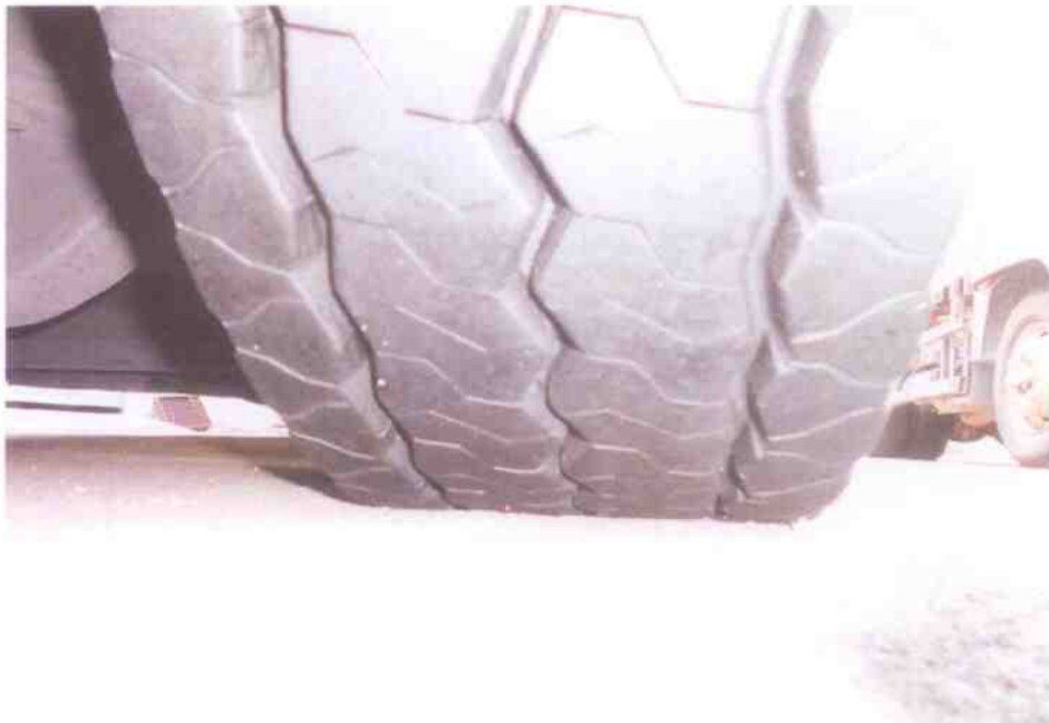
Photo 8 shows the condition of the front left tyre of the Motor Bus, which was observed to be in serviceable condition with remaining tread depth of approximately 18mm.
