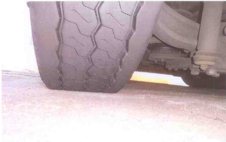
Photo 9 shows the condition of the rear right tyres (centre axle) of the Motor Bus, which were observed to be in serviceable condition with remaining tread depth of approximately 13mm.
