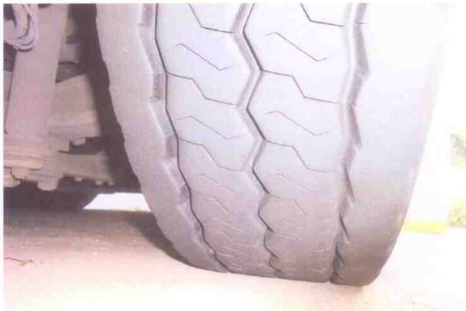
Photo 10 shows the condition of the rear left tyres (centre axle) of the Motor Bus, which were observed to be in serviceable condition with remaining tread depth of approximately 15mm. The tyres, which were wrapped around standard alloy wheel rims, were also observed to be sufficiently inflated for vehicular operation.
