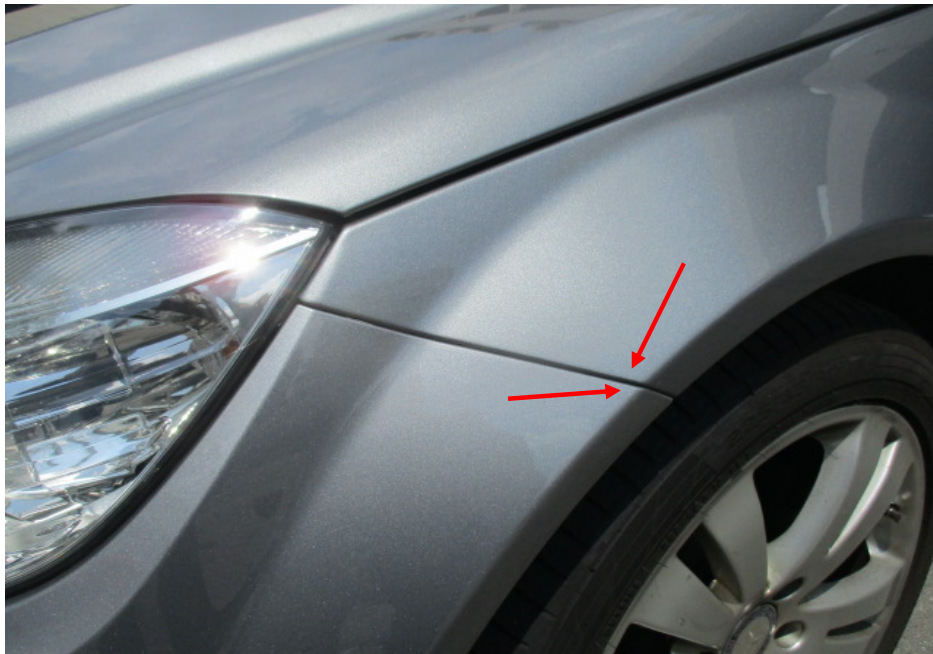
Photo 13 shows a close up view of the left corner edge of the front bumper of the Mercedes. We observed that there was no misalignment at the corner edges (red arrows).
