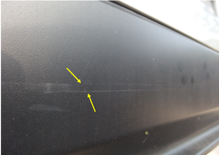
Photo 4 shows a close up view of the horizontal whitish marks observed on the left portion of the Toyota's lower rear bumper (arrowed).
