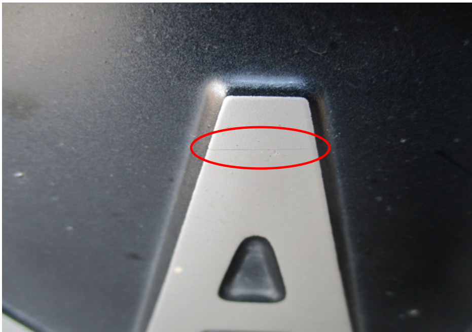
Photo 11 shows a close up view of the horizontal blackish marks on some of the alpha-numeric letterings of the Mercedes front number plate (circled).
