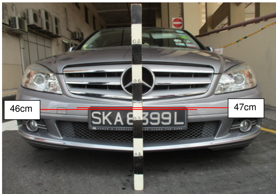
Photo 16 shows the height measurement being conducted on the front portion of the Mercedes. The body part at the height range of between 46cm to 47m above ground level was the top portion of the front number plate frame.
