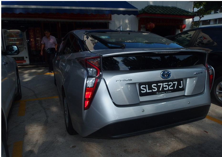
Photo 1 shows the general view of the rear of the Toyota at the time of the Pre-Repair Survey conducted by LKK Auto Consultants Pte. Ltd. which was taken about 2 weeks after the accident. The damage to the Toyota was observed to be confined to its rear portion, at the rear bumper.
