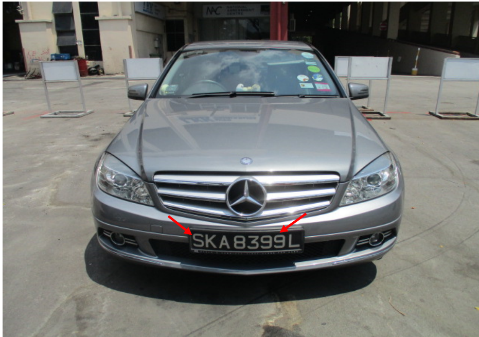
Photo 6 shows the general view of the front portion of the Mercedes at the time of our inspection. The only body part shape on the front of the Mercedes that could possibly correspond to the horizontal whitish marks found on the lower rear bumper of the Toyota was the top portion (arrowed) of its rectangular shaped front number plate frame.
