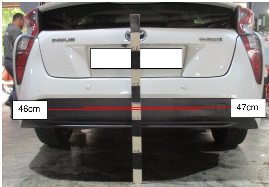
Photo 15 shows the height measurement being conducted on the rear portion of the Toyota (using a similar make and model). The height range above ground level of the lower rear bumper of the Toyota, at the area where the horizontal whitish marks were found was measured to be approximately between 46cm to 47cm.
