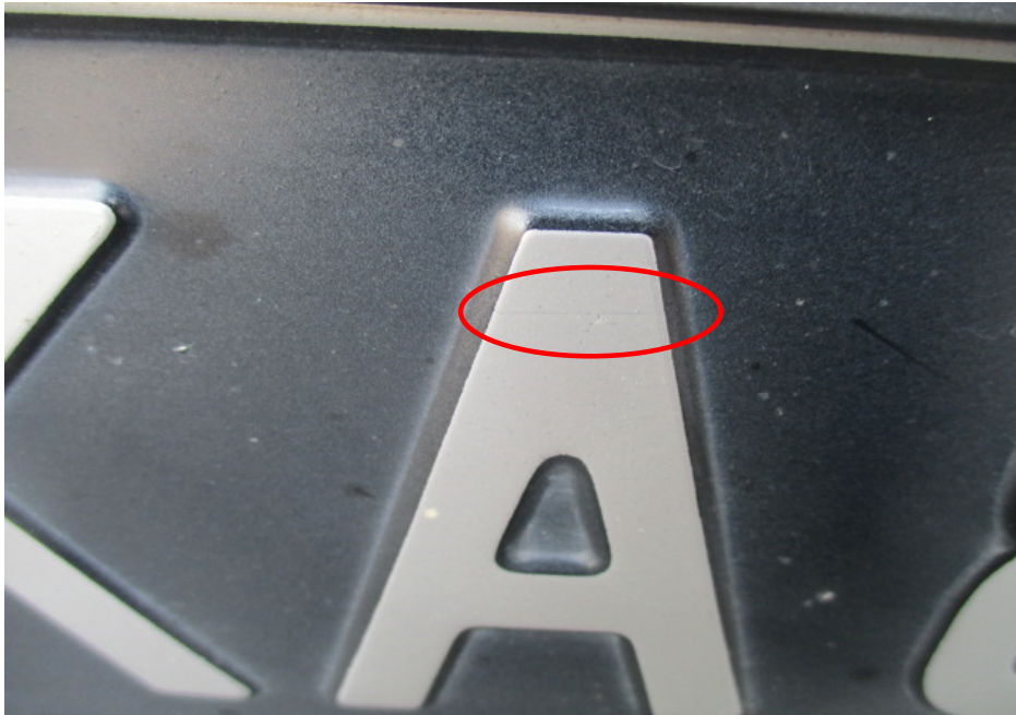
Photo 10 shows a closer view of the horizontal blackish marks on some of the alpha-numeric letterings of the Mercedes front number plate (circled).
