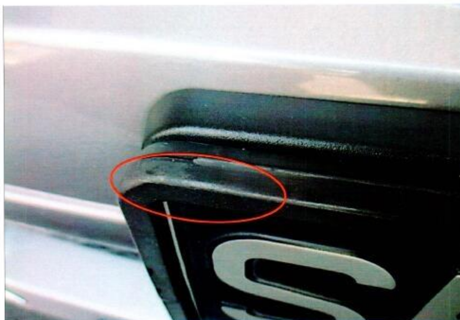
Photo 7 shows a close up view of the top right portion of the Mercedes's front number plate frame. The frame was observed to be slightly distorted (circled). However there was no obvious crack or break on the front number plate frame.
