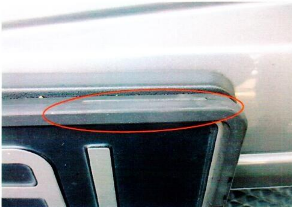
Photo 8 shows a close up view of the top left portion of the Mercedes's front number plate frame. The frame was observed to be slightly distorted (circled). However there was no obvious crack or break on the front number plate frame.
