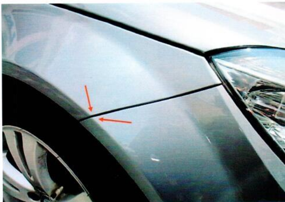
Photo 12 shows a close up view of the right corner edge of the front bumper of the Mercedes. We observed that there was no misalignment at the corner edges (red arrows).
