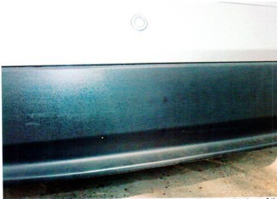
Photo 2 shows a closer view of the rear bumper of the Toyota at the time of the Pre- Repair Survey conducted by LKK Auto Consultants Pte. Ltd. which was taken about 2 weeks after the accident. Horizontal whitish marks were observed on the left portion of the lower rear bumper (arrowed).
