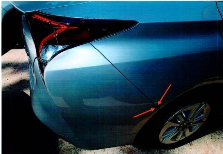
Photo 5 shows a close up view of the right corner edge of the rear bumper of the Toyota. We observed that there was no misalignment at the corner edges (red arrows).
