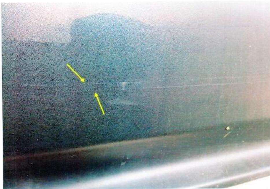
Photo 3 shows a close up view of the horizontal whitish marks observed on the left portion of the Toyota's lower rear bumper (arrowed).
