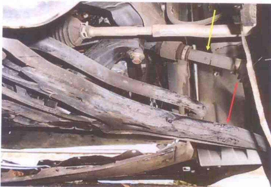
Photo 10 shows the undercarriage components at the front right wheel of the Motor Car. My checks on the underside of the Motor Car revealed damage to the various undercarriage components at the front right wheel and front left wheel of the Motor Car. Components like the front right lower arm (red arrow), front right drive shaft (yellow arrow) and front right steering tie rod were all found to be have been damaged.
