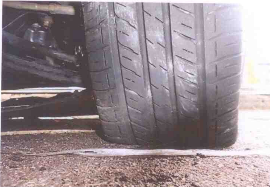
Photo 7 shows the condition of the front right tyre of the Motor Car, which was observed to be in serviceable condition with remaining tread depth of approximately 6mm. The tyre was observed to be deflated and loosely wrapped around the front right wheel rim as a result of the accident.
