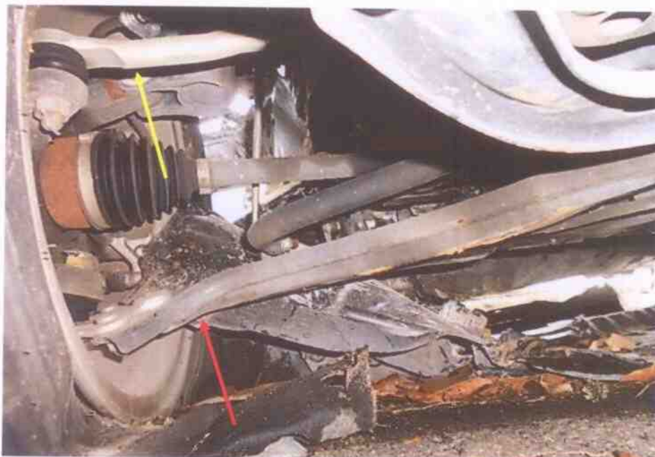
Photo 11 shows the undercarriage components at the front left wheel of the Motor Car. My checks on the underside of the Motor Car revealed damage to the various undercarriage components at the front right wheel and front left wheel of the Motor Car. Components like the front left lower arm (red arrow) and front left steering tie rod (yellow arrow) were damaged.
