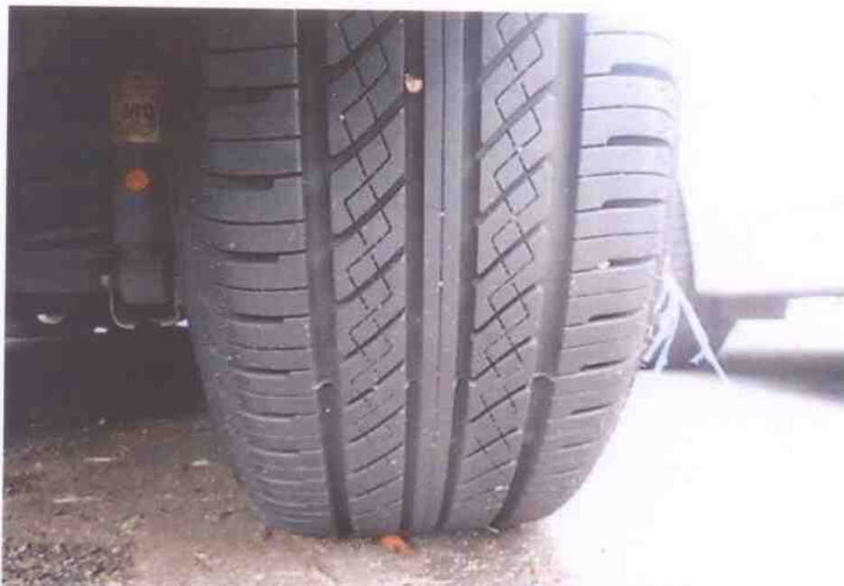
Photo 5 shows the condition of the rear right tyre of the Motor Car, which was observed to be in serviceable condition with remaining tread depth of approximately 7mm. There was no tear, cut or burst mark(s) on the outer and the inner sidewalls as well as across the tread of this tyre. The tyre, which was wrapped around alloy wheel rim, was also observed to be sufficiently inflated for vehicular operation.
