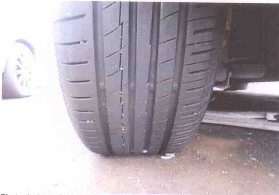
Photo 4 shows the condition of the rear left tyre of the Motor Car, which was observed to be in serviceable condition with remaining tread depth of approximately 7mm. There was no tear, cut or burst mark(s) on the outer and the inner sidewalls as well as across the tread of this tyre. The tyre, which was wrapped around alloy wheel rim, was also observed to be sufficiently inflated for vehicular operation.
