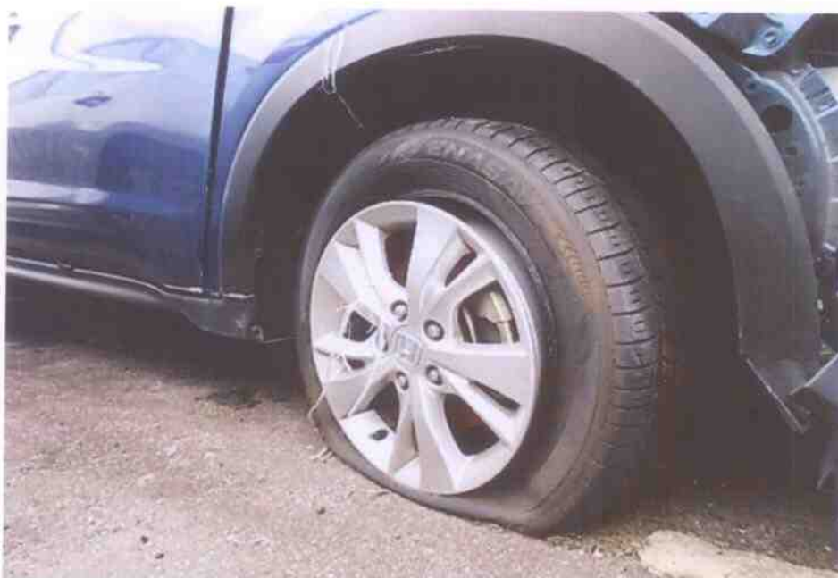
Photo 6 shows a general view of the front right wheel rim and tyre of the Motor Car. The front right tyre was observed to be deflated and loosely wrapped around the front right wheel rim as a result of the accident.
