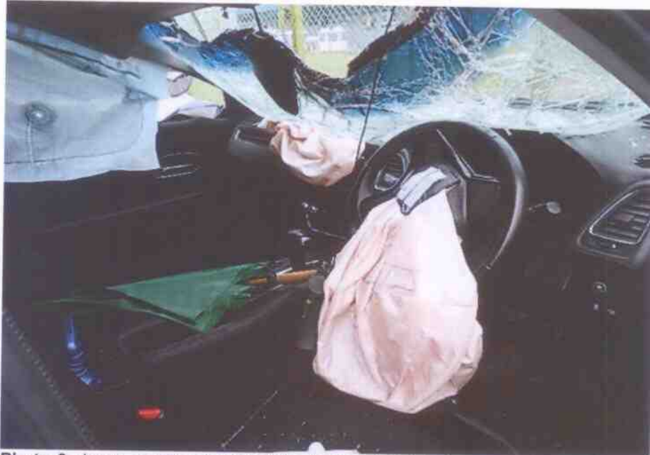
Photo 3 shows a general view of the Motor Car's interior compartment. Several parts and components inside the interior compartment were observed to have been damaged. This had included the front dashboard, trims and seats. The driver's air bag, front left passenger air bag and left curtain air bag were also deployed as a result of the accident.
