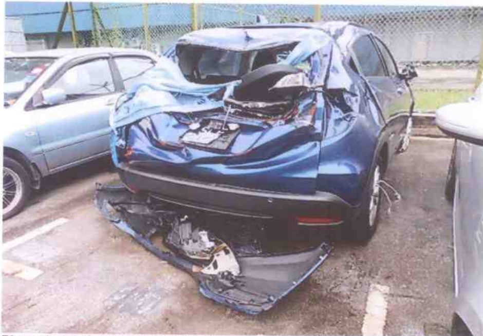
Photo 1 shows a general view of the rear portion of the Motor Car at the time of my inspection. Its rear tailgate, rear windscreen, rear right fender and roof panel were amongst the body parts that were severely damaged as a result of the accident.
