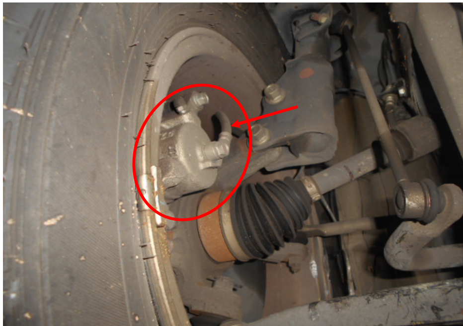
Photo 12 shows the brake hose (arrowed) at the front right wheel of the Motor Car. I did not observe any leakage of brake fluid at the 4 wheels of the Motor Car. My visual inspection of the various mechanical components of the Motor Car's braking system, including its brake caliper (circled), revealed all to be intact and without visible damage, indicating that the braking system was likely to be in serviceable condition at the material time of accident.
