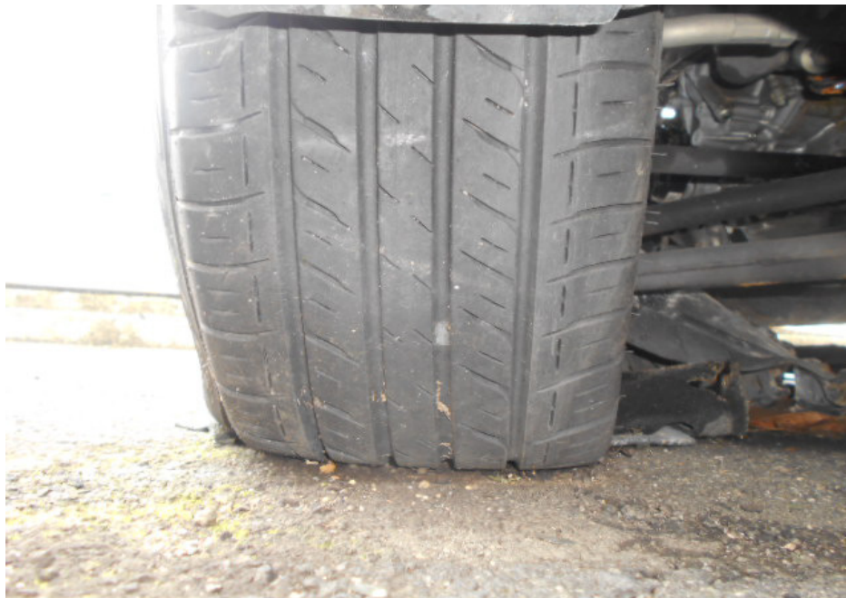
Photo 9 shows the condition of the front left tyre of the Motor Car, which was observed to be in serviceable condition with remaining tread depth of approximately 6mm. The tyre was observed to be deflated and cut as a result of the accident.
