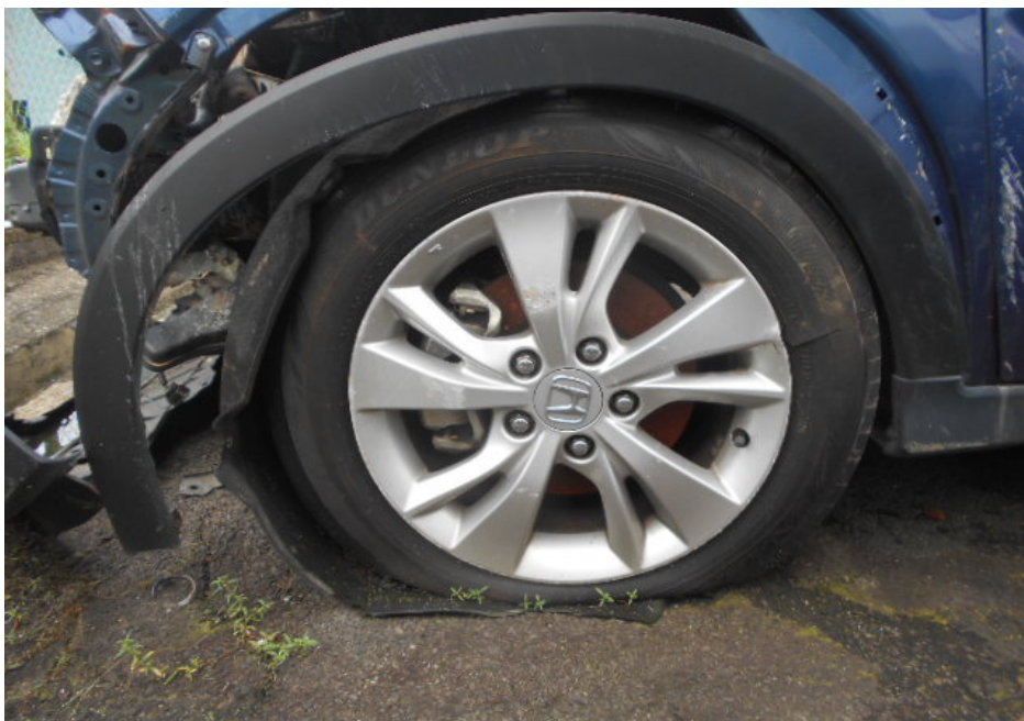
Photo 8 shows a general view of the front left wheel rim and tyre of the Motor Car. The front left tyre was observed to be deflated with a cut on its outer sidewall. The front left wheel rim was also observed to be dented as a result of the accident.
