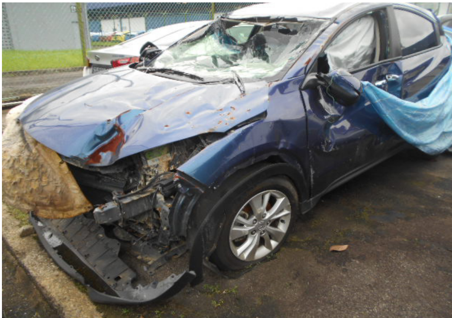
Photo 2 shows a general view of the front left portion of the Motor Car at the time of my inspection. The Motor Car was also observed to have sustained extensive impact damage at its frontal portion and left portion. Its front bumper, front bonnet, front left fender, front windscreen, left front door and roof panel were amongst the body parts that were observed to have been damaged as a result of the accident.
