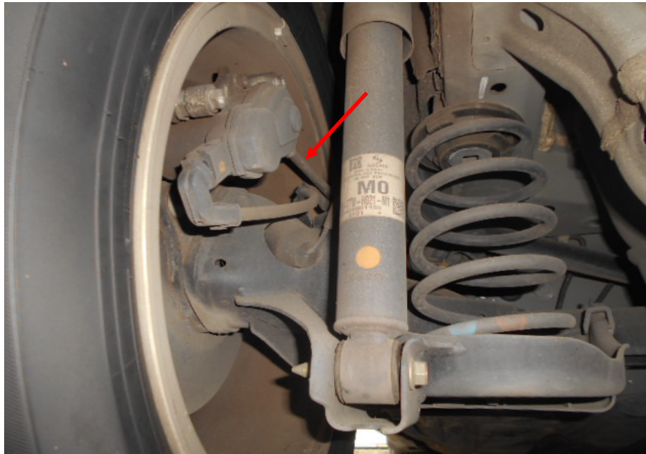
Photo 13 shows the various undercarriage components at the rear left wheel of the Motor Car, in particular the brake hose (arrowed). I did not observe any leakage of brake fluid at the 4 wheels of the Motor Car. My visual inspection of the various mechanical components of the Motor Car's braking system revealed all to be intact and without visible damage, indicating that the braking system was likely to be in serviceable condition at the material time of accident.
