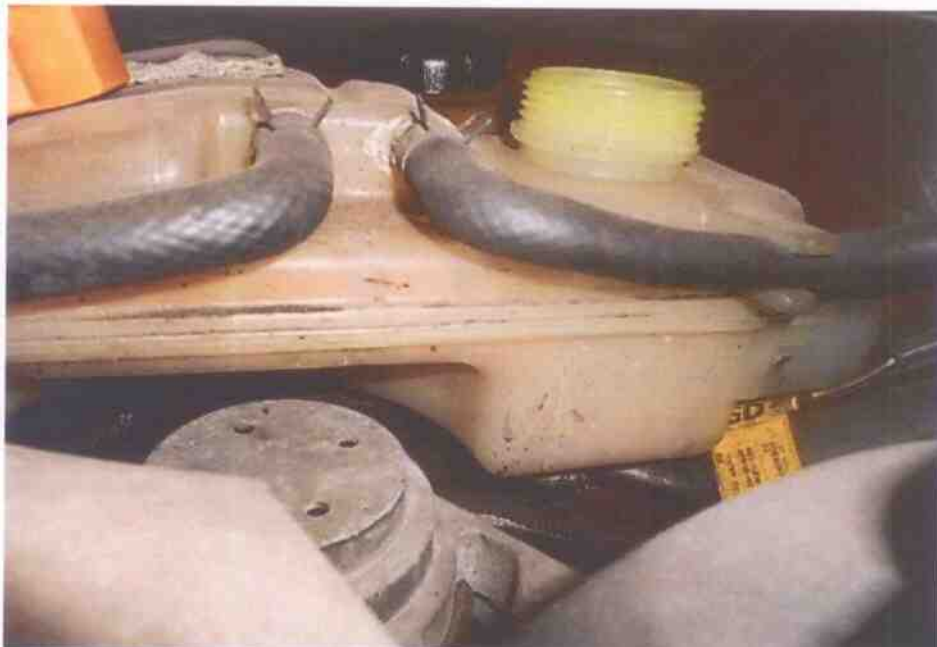
Photo 10 shows the engine coolant reservoir tank of the Motor Taxi at the time of my inspection. The engine coolant was observed to be of insufficient level for operating purposes. This was due to engine coolant leakage from a damaged radiator.
