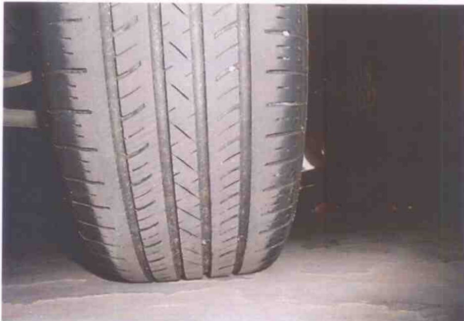
Photo 7 shows the condition of the rear right tyre of the Motor Taxi, which was observed to be in serviceable condition with remaining tread depth of approximately 6mm. There was no tear, cut or burst mark(s) on the outer and the inner sidewalls as well as across the tread of the tyre.
