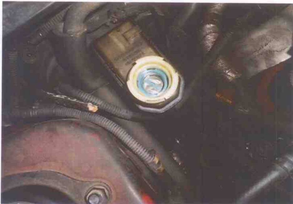
Photo 9 shows the brake fluid reservoir of the Motor Taxi at the time of my inspection. I had found the brake fluid to be of sufficient level for operating purposes, and without any visible contamination.
