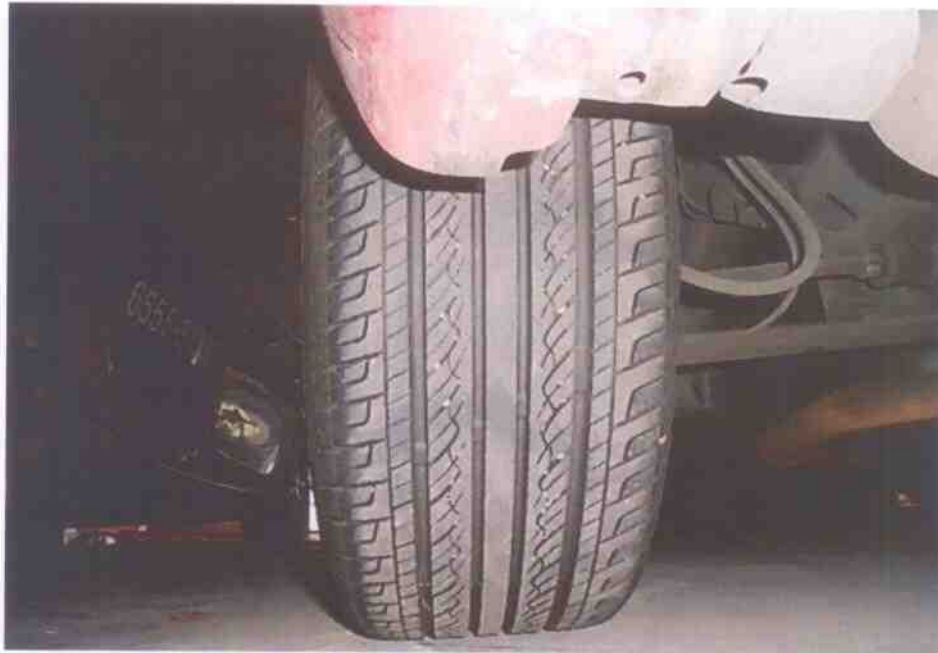
Photo 6 shows the condition of the rear left tyre of the Motor Taxi, which was observed to be in serviceable condition with remaining tread depth of approximately 6mm. The tyre, which was wrapped around standard wheel rim, was also observed to be sufficiently inflated for vehicular operation. The 4 tyres of the Motor Taxi were wrapped around standard wheel rims that were without any damage.
