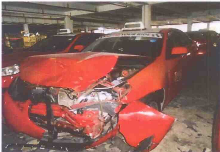
Photo 1 shows a general view of the front left body of the Motor Taxi at the time of my inspection. The Motor Taxi was observed to have sustained impact damage that was confined to its frontal body. Its front bumper, front bonnet, front left headlamp and front left fender were amongst the body parts that were damaged as a result of the accident. The mileage of the Motor Taxi was not recorded due to the extent of damage, which had affected the ignition system of the Motor Taxi.
