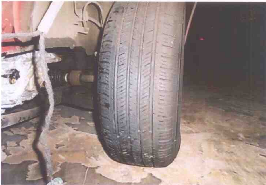
Photo 4 shows the condition of the front left tyre of the Motor Taxi, which was observed to be in serviceable condition with remaining tread depth of approximately 6mm. The tyre, which was wrapped around standard wheel rim, was also observed to be sufficiently inflated for vehicular operation. There was no tear, cut or burst mark(s) on the outer and the inner sidewalls as well as across the tread of the tyre.
