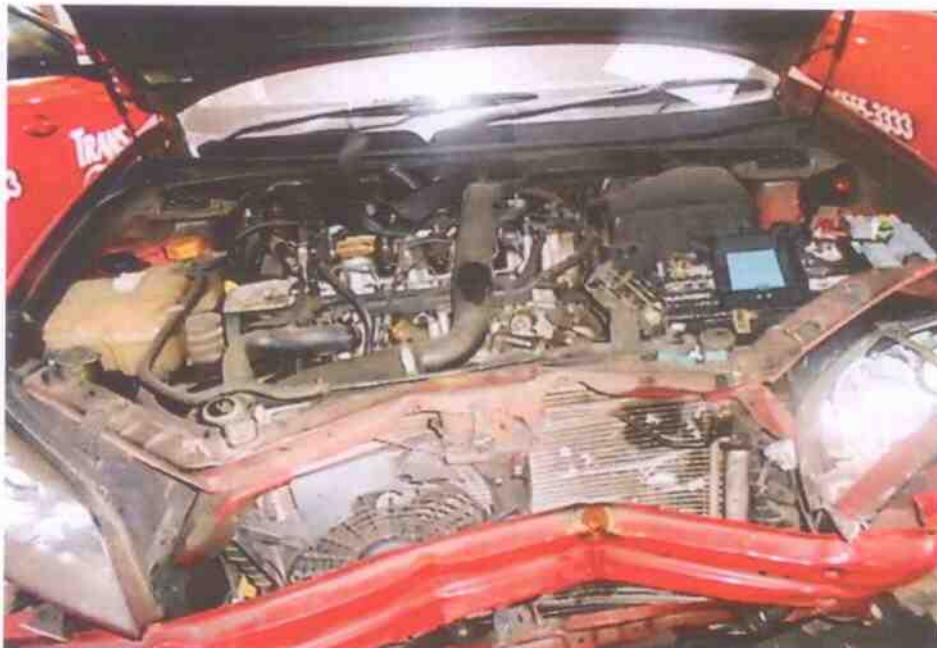
Photo 8 shows a general view of the Motor Taxi's engine compartment. Parts that were mainly towards the front of the engine compartment were pushed inwards as a result of the impact force onto the frontal body of the Motor Taxi. The front support panel, front bumper reinforcement, cooling fan, air condenser and radiator were all observed to have been damaged.
