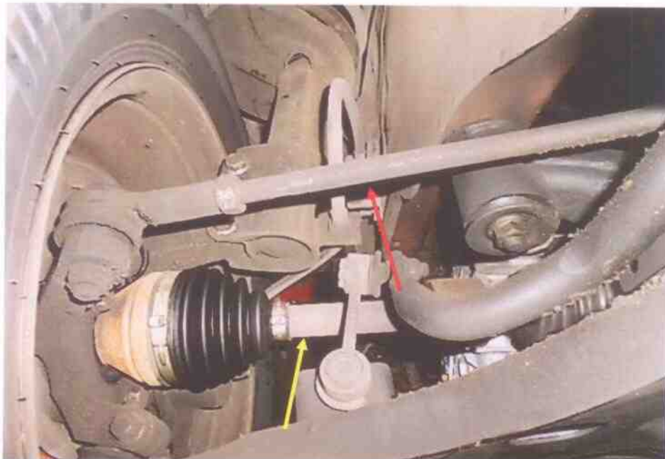
Photo 13 shows the various undercarriage components at the front left wheel of the Motor Taxi, in particular the steering tie rod (red arrow) and front left drive shaft (yellow arrow). The various steering components were all found to be intact, suggesting that the steering system of the Motor Taxi was likely to be in serviceable condition at the material time of accident.
