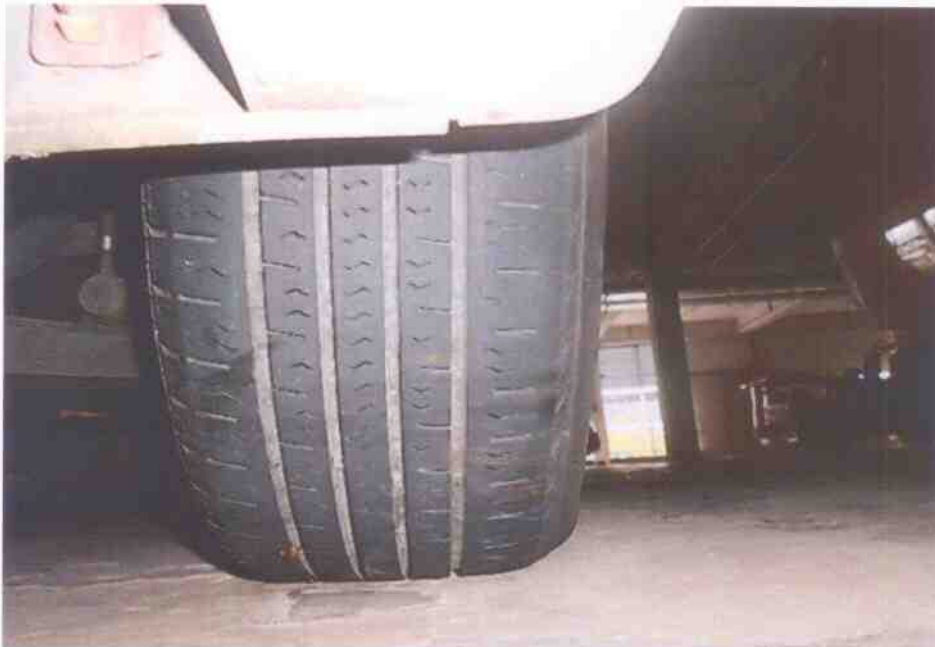
Photo 5 shows the condition of the front right tyre of the Motor Taxi, which was observed to be in serviceable condition with remaining tread depth of approximately 6mm. The tyre, which was wrapped around standard wheel rim, was also observed to be sufficiently inflated for vehicular operation.
