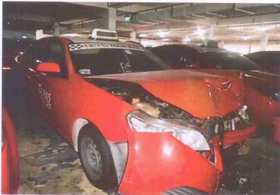
Photo 2 shows a general view of the front right body of the Motor Taxi at the time of my inspection. The Motor Taxi was observed to have sustained impact damage that was confined to its frontal body. Its front bumper, front bonnet and front right headlamp were amongst the body parts that were damaged as a result of the accident. The mileage of the Motor Taxi was not recorded due to the extent of damage, which had affected the ignition system of the Motor Taxi.
