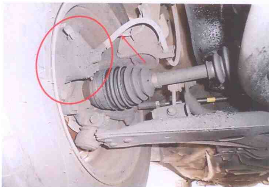
Photo 17 shows the brake hose/pipe (arrowed) at the front right wheel of the Motor Taxi. There was no brake fluid leak observed. Visual examination of the various components of the braking system like the brake caliper (circled), brake booster, brake pedal etc had revealed all to be intact and without visible damage.
