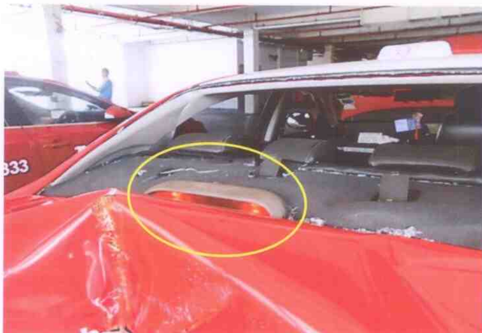
Photo 21 shows the brake light (circled) for the Motor Taxi's third brake lamp illuminated upon stepping on the brake pedal.
