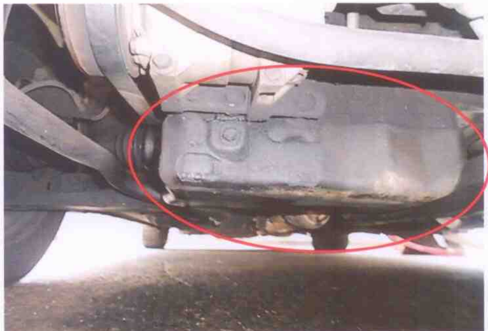
Photo 14 shows the underside of the Motor Taxi. Fluid stains were observed on the engine oil sump (circled) and some undercarriage components of the Motor Taxi. This was due to the leakage of engine fluid. I also note the presence of dirt and dust particles accumulated around the fluid stain areas, indicating that the fluid leak was pre-existing for a period of time and not a result of the accident.
