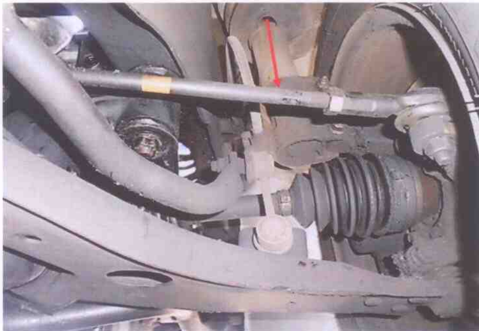
Photo 19 shows the various undercarriage components at the front right wheel of the Motor Taxi, in particular the steering tie rod (arrowed). The various steering components were all found to be intact, suggesting that the steering system of the Motor Taxi was likely to be in serviceable condition at the material time of accident.
