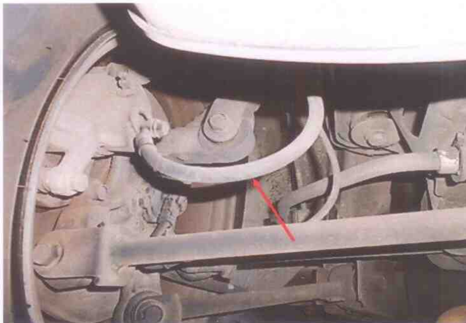
Photo 16 shows the brake hose/pipe (arrowed) at the rear left wheel of the Motor Taxi. There was no brake fluid leak observed. Static tests of the Motor Taxi's braking system had indicated that there was no internal leakage of pressure/vacuum. Hence the braking system was likely to be in serviceable condition at the material time of accident. The undercarriage components of the Motor Taxi were also all found to be intact and without any visible damage.
