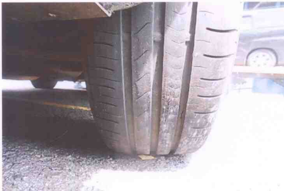
Photo 8 shows the condition of the rear right tyre of the Motor Taxi, which was observed to be in serviceable condition with remaining tread depth of approximately 7mm. The tyre, which was wrapped around standard wheel rim, was also observed to be sufficiently inflated for vehicular operation.
