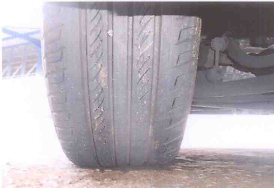
Photo 4 shows the condition of the front left tyre of the Motor Taxi, which was observed to be in serviceable condition with remaining tread depth of approximately 5mm. The tyre, which was wrapped around standard wheel rim, was also observed to be sufficiently inflated for vehicular operation. There was no tear, cut or burst mark(s) on the outer and the inner sidewalls as well as across the tread of the tyre.
