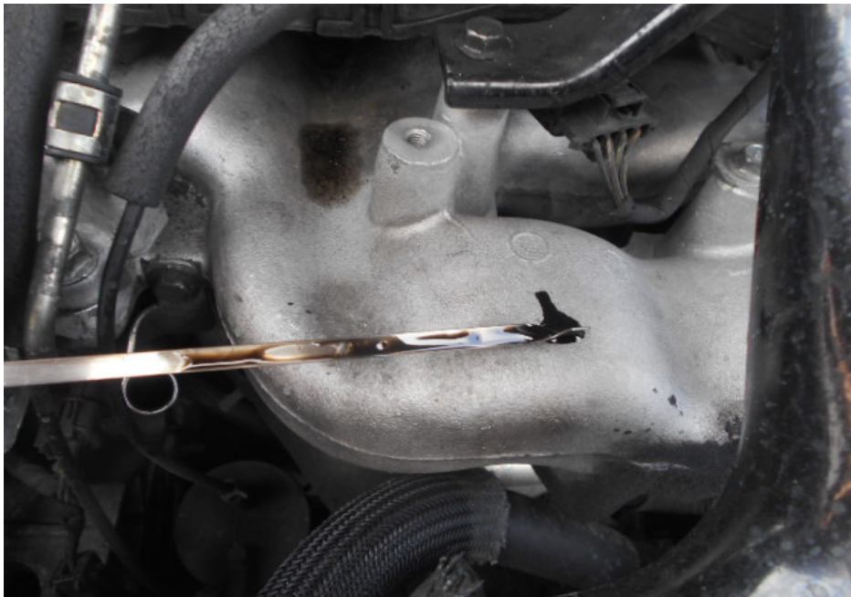
Photo 12 shows the engine oil dip stick of the Motor Taxi at the time of my inspection. The engine oil was observed to be of sufficient level and without any visible contamination.
