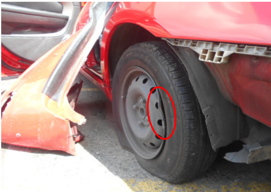
Photo 6 shows a general view of the rear left wheel rim and rear left tyre of the Motor Taxi. The rear left wheel rim was observed to be dented (circled) while the rear left tyre was observed to be deflated. Both were a result of the accident.
