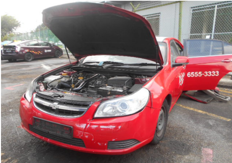
Photo 1 shows a general view of the front left body of the Motor Taxi at the time of my first inspection. The Motor Taxi was observed to have sustained damages at its frontal portion and rear portion. The front number plate, front bonnet, front grille, front bumper reinforcement and front support panel were amongst the body parts at the frontal portion that were damaged. The mileage of the Motor Taxi was recorded to be 739,101km.
