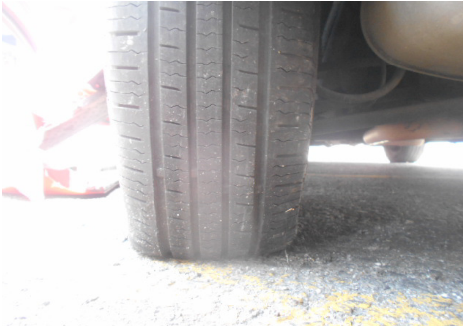
Photo 7 shows the condition of the rear left tyre of the Motor Taxi, which was observed to be in serviceable condition with remaining tread depth of approximately 6mm. The tyre was observed to be deflated as a result of the accident.
