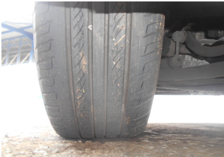
Photo 4 shows the condition of the front left tyre of the Motor Taxi, which was observed to be in serviceable condition with remaining tread depth of approximately 5mm. The tyre, which was wrapped around standard wheel rim, was also observed to be sufficiently inflated for vehicular operation. There was no tear, cut or burst mark(s) on the outer and the inner sidewalls as well as across the tread of the tyre.
