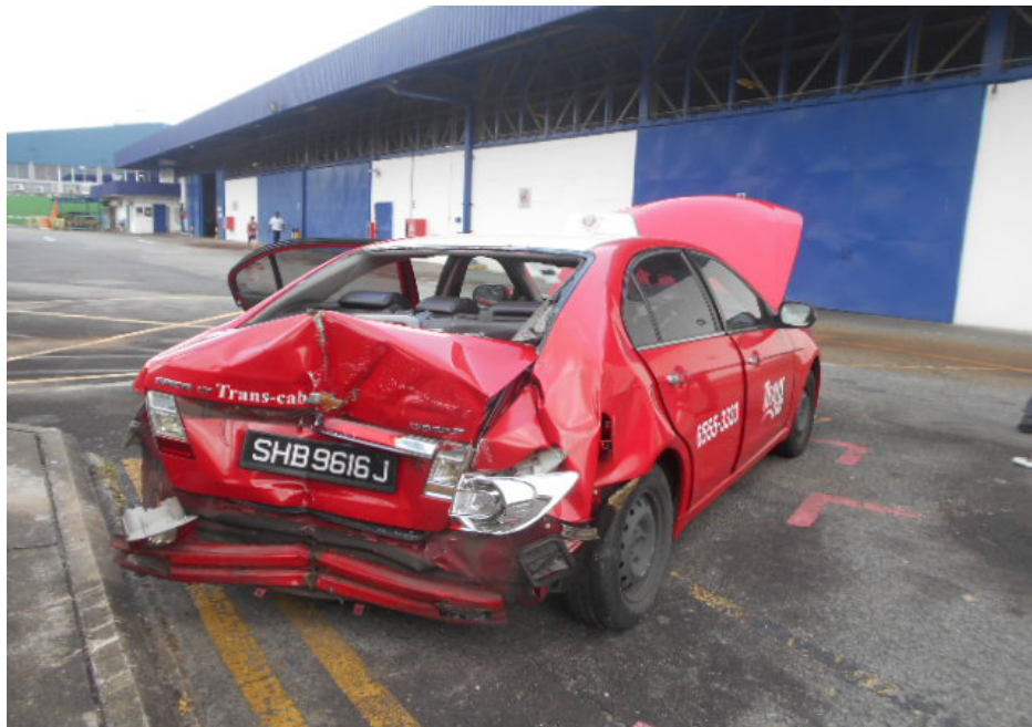
Photo 3 shows a general view of the Motor Taxi's rear right body at the time of my inspection. The rear bumper, rear bootlid, rear taillamps, rear right fender, rear bootlid lamps and rear windscreen were amongst the body parts at the rear portion of the Motor Taxi that were observed to have been damaged as a result of the accident.
