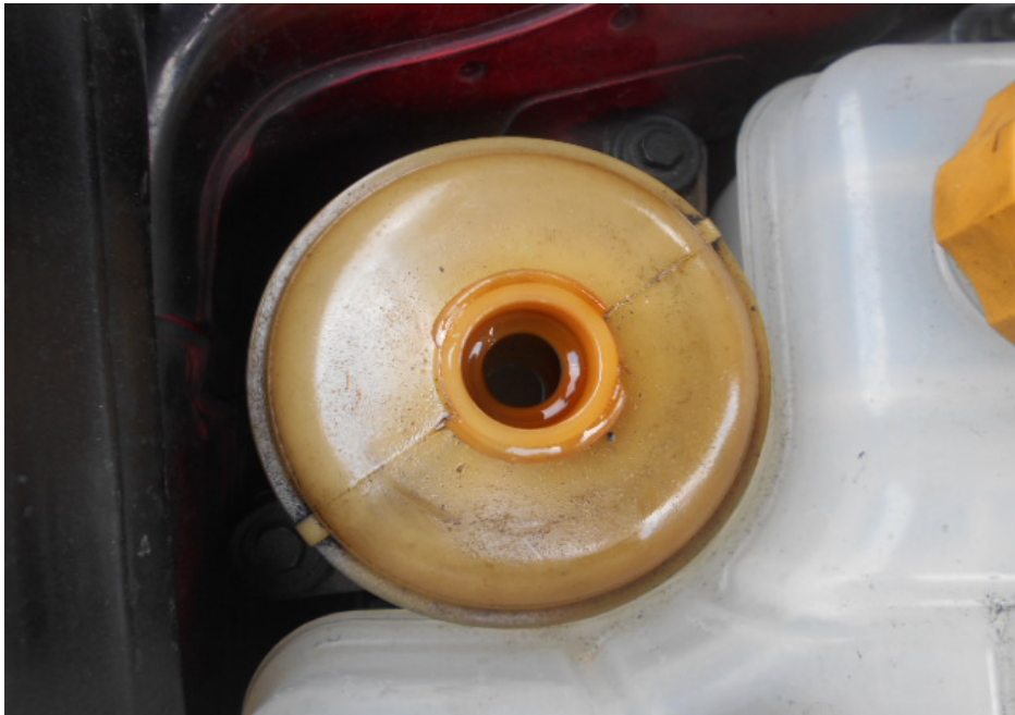
Photo 13 shows the power steering fluid reservoir tank of the Motor Taxi at the time of my inspection. The power steering fluid was observed to be of sufficient level and without any visible contamination.
