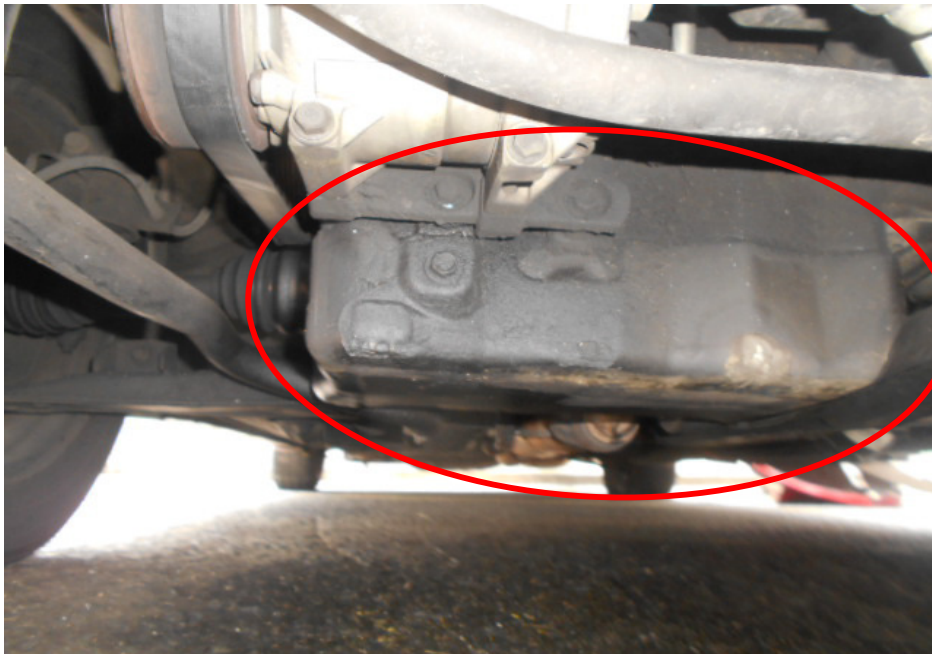
Photo 14 shows the underside of the Motor Taxi. Fluid stains were observed on the engine oil sump (circled) and some undercarriage components of the Motor Taxi. This was due to the leakage of engine fluid. I also note the presence of dirt and dust particles accumulated around the fluid stain areas, indicating that the fluid leak was pre-existing for a period of time and not a result of the accident.
