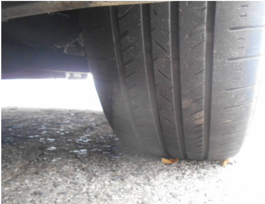
Photo 5 shows the condition of the front right tyre of the Motor Taxi, which was observed to be in serviceable condition with remaining tread depth of approximately 5mm. The tyre, which was wrapped around standard wheel rim, was also observed to be sufficiently inflated for vehicular operation. A slight dent was observed on the front right wheel rim as a result of the accident.
