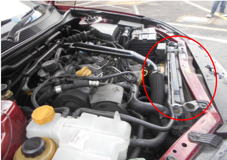
Photo 9 shows a general view of the Motor Taxi's engine compartment. The parts that were mainly towards the front of the engine compartment (circled) were pushed inwards as a result of the impact force onto the front body of the Motor Taxi. Parts like the front support panel, air condenser and radiator were affected.
