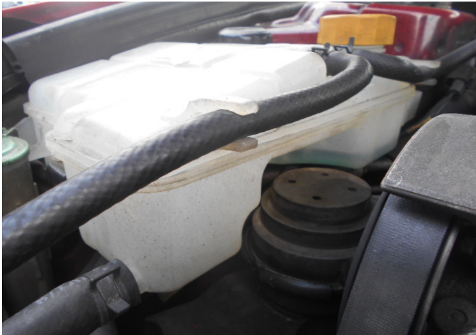
Photo 11 shows the engine coolant reservoir tank of the Motor Taxi at the time of my inspection. The engine coolant was observed to be of insufficient level. This was due to leakage of engine coolant from the Motor Taxi's damaged radiator.
