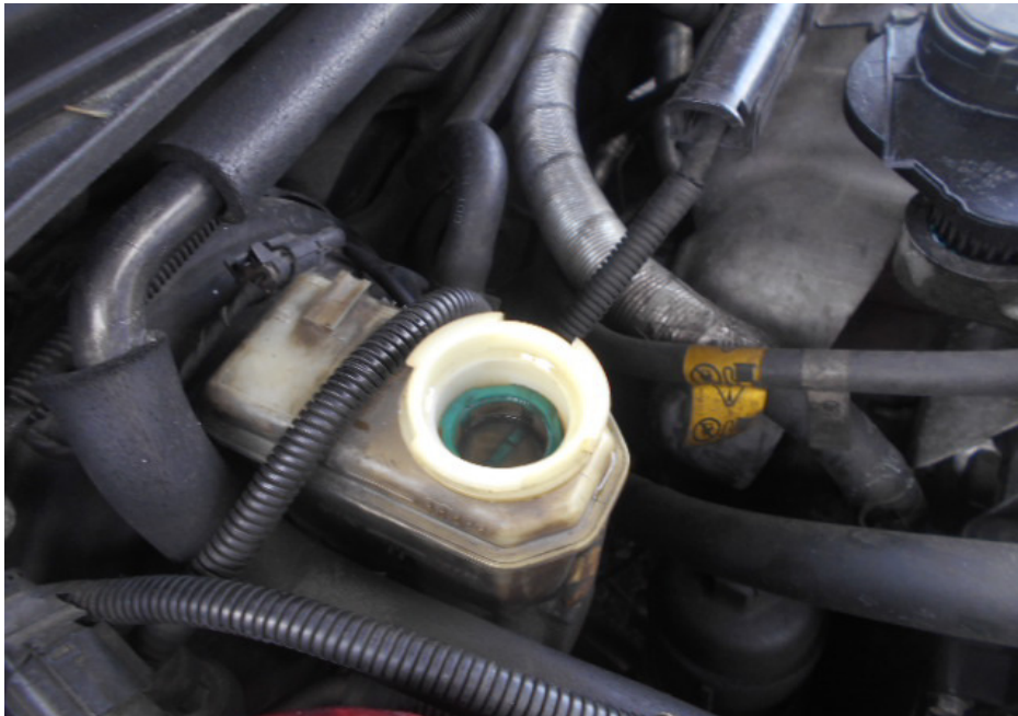
Photo 10 shows the brake fluid reservoir of the Motor Taxi at the time of my inspection. The brake fluid was observed to be of sufficient level and without any visible contamination.
