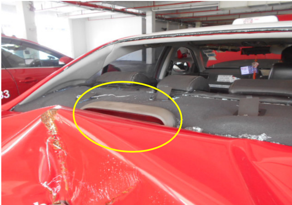
Photo 20 shows the third brake light (circled) of the Motor Taxi. The bulbs of the Motor Taxi's brake lights were observed to be in working condition at the time of my inspection. The brake lights at the rear left taillamp, rear right taillamp and the third brake light illuminated when the brake pedal of the Motor Taxi was depressed.
