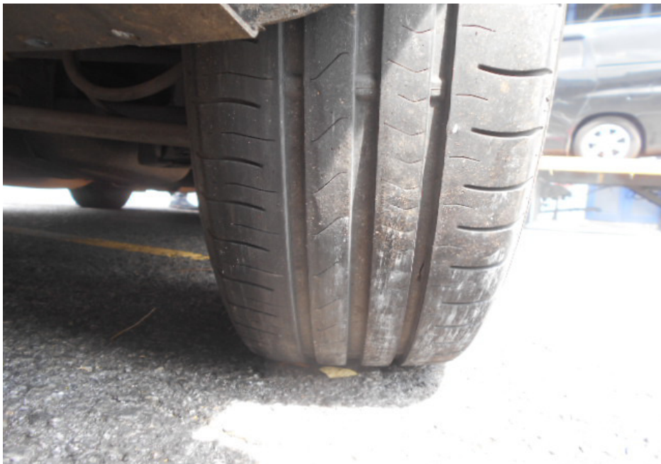
Photo 8 shows the condition of the rear right tyre of the Motor Taxi, which was observed to be in serviceable condition with remaining tread depth of approximately 7mm. The tyre, which was wrapped around standard wheel rim, was also observed to be sufficiently inflated for vehicular operation.
