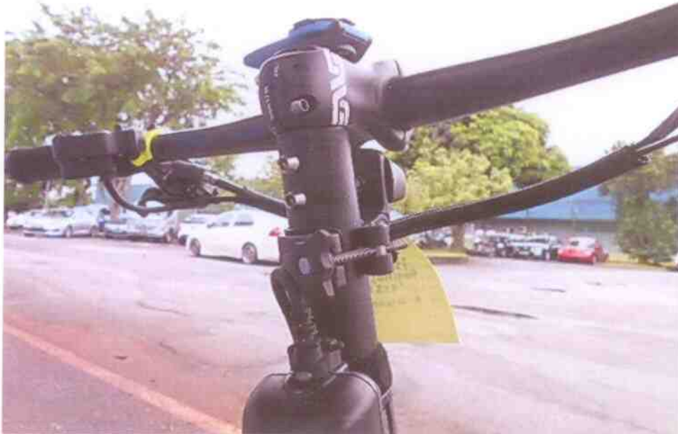
Photo 7 shows steering components of the Electric Scooter had revealed that its steering system was in serviceable condition & its front fork was found to be intact and undamaged. It was observed to be able to turn to full left & full right.
