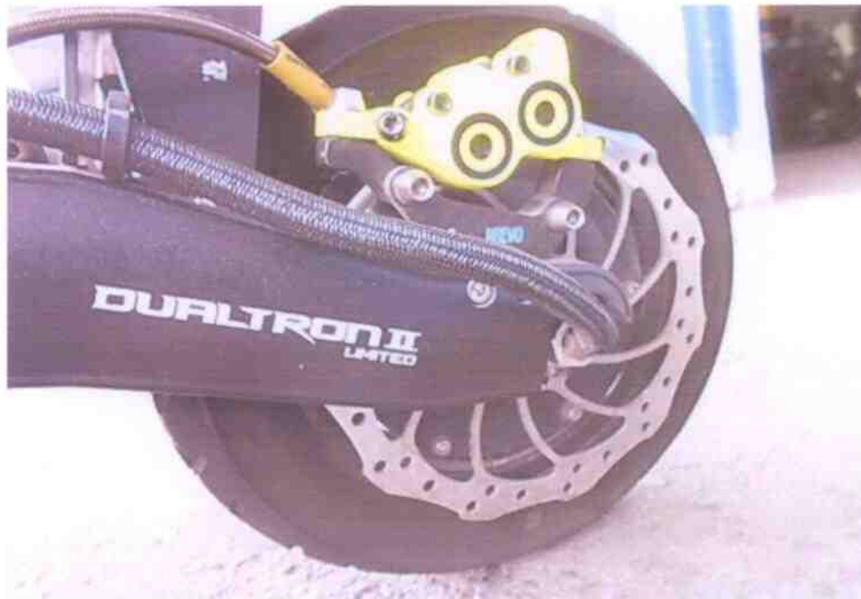
Photo 10 shows the rear brake callipers, revealed that it was in a serviceable condition.
