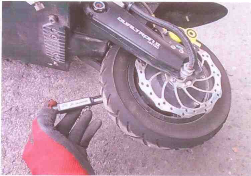
Photo 5 shows the rear tyre of the Electric Scooter at the time of our inspection. The tread pattern of the 2 tyres was clearly visible. We did not observe any tear, burst mark(s) and/or punctured hole(s) on the sidewalls.
