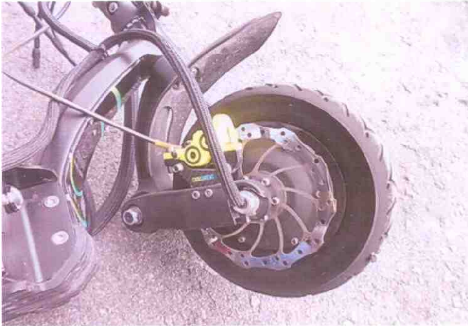
Photo 8 shows steering components of the Electric Scooter had revealed that its steering system was in serviceable condition & its front fork was found to be intact and undamaged. It was observed to be able to turn to full left & full right.
