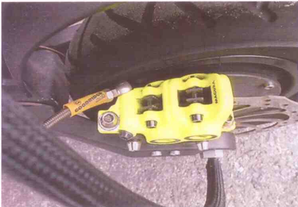
Photo 9 shows the front brake callipers, revealed that it was in a serviceable condition.
