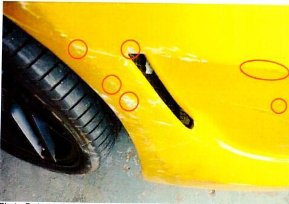
Photo 7 shows a close up view of the left rear portion of the Insured Vehicle during the accident reporting. We observed bluish paint transfer marks at the left rear portion of the Insured Vehicle (circled). This correlates with Mr Boo's statement that the Insured Vehicle was hit on its left rear portion by the Taxi.
