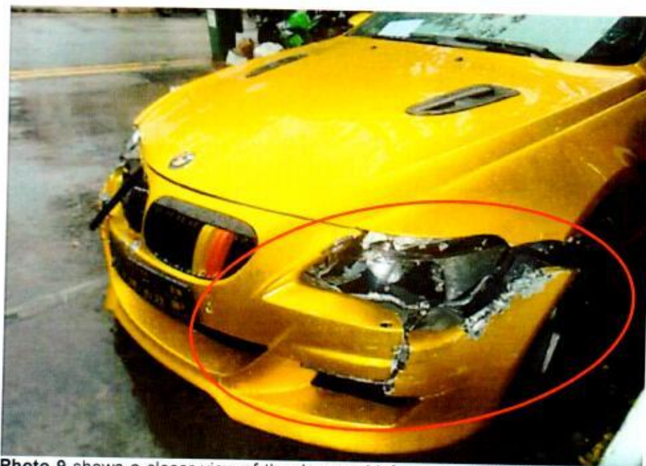
Photo 9 shows a closer view of the damaged left portion of the front bumper of the Insured Vehicle during the accident reporting (circled). The extensive damages sustained seem to corroborate with Mr Boo's statement that he had hit the right front portion of the Honda at the material time of accident.
