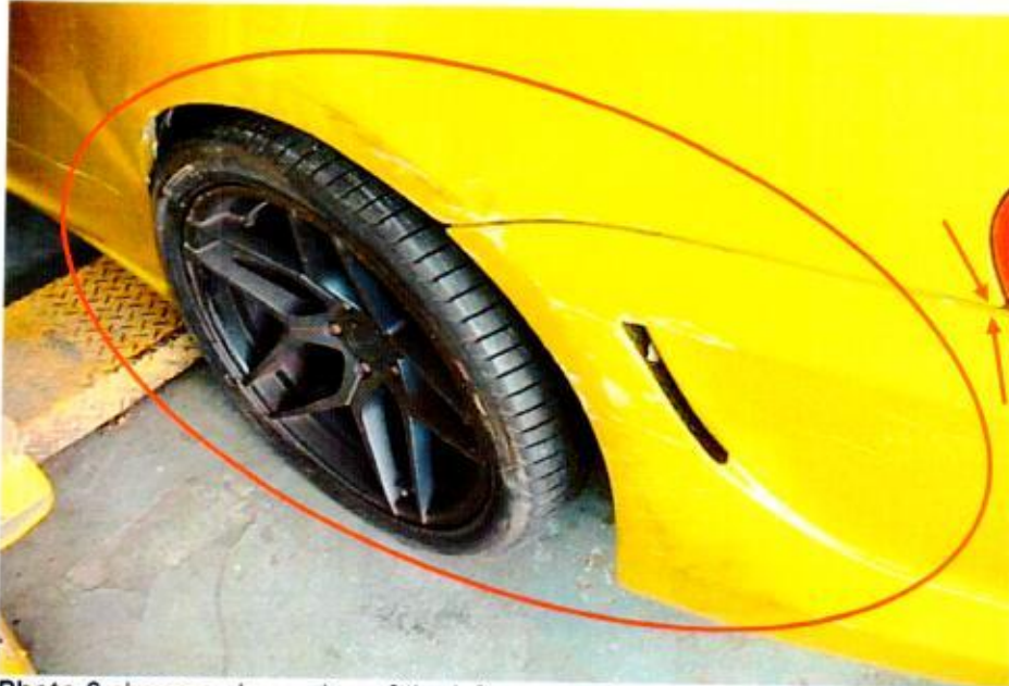
Photo 6 shows a closer view of the left rear portion of the Insured Vehicle during the accident reporting. The left rear wheel fender and rear bumper had sustained a dent and paint graze marks. The left rear wheel had also sustained similar marks of grazing nature and was punctured as a result of the accident (circled). There was a slight misalignment of the left side of the rear bumper at its corner edges (arrowed). This correlates with Mr Boo's statement that the Insured Vehicle was hit on its left rear portion by the Taxi.
