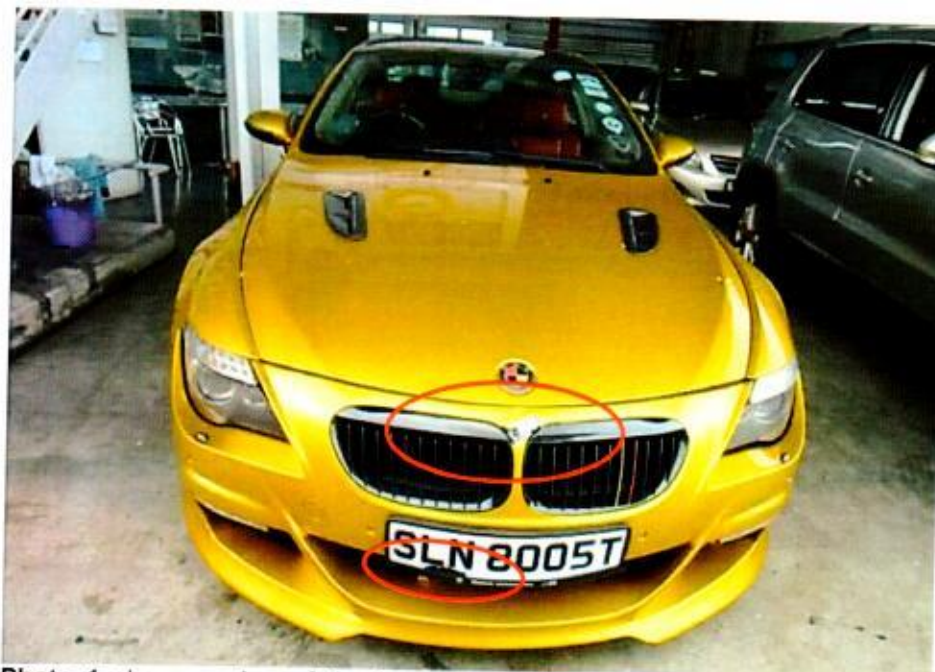
Photo 1 shows a view of the front portion of the Insured Vehicle during the accident reporting. The front bumper and front number plate of the Insured Vehicle had sustained damages as a result of the accident (circled).
