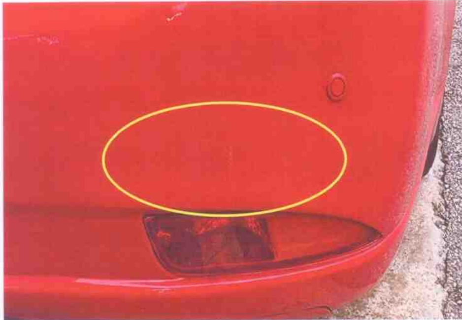
Photo 13 shows a close up view of the paint graze marks on the lower right portion of the rear bumper of the Taxi (circled).
