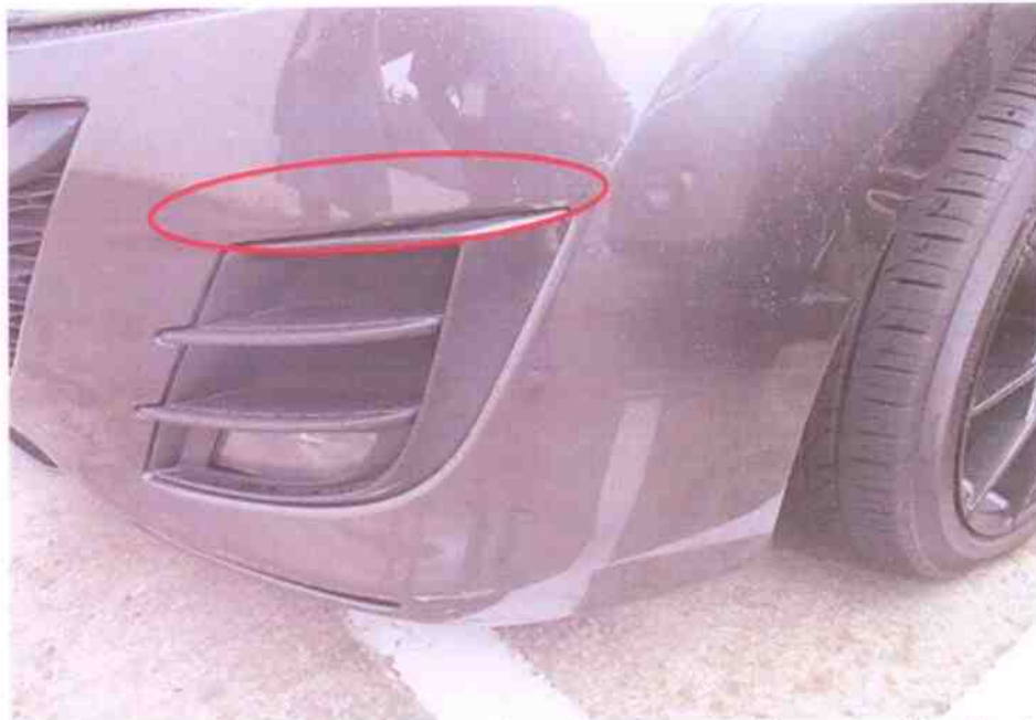
Photo 5 shows a closer view of the left portion of the front bumper of the Mazda at the time of inspection. We observed faint paint scratch marks above the front left air vent (circled).
