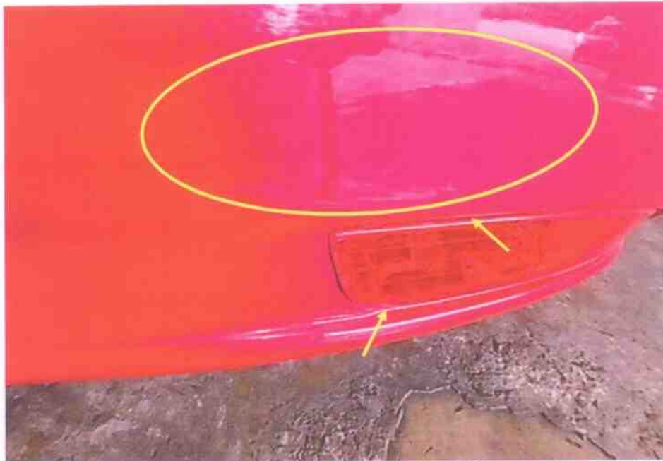
Photo 2 shows a closer view of the lower right portion of the rear bumper of the Taxi. We observed paint graze marks above (circled) and around (yellow arrows) the rear right bumper reflector of the Taxi.
