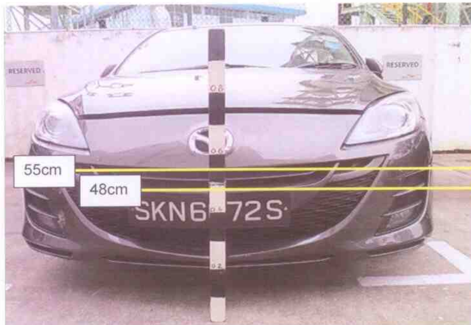
Photo 15 shows the height measurement being conducted on the front bumper of the Mazda. The faint paint scratch marks found on the Mazda are within the 48cm to 55cm range.
