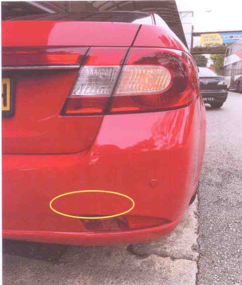
Photo 12 shows a close view of the lower right portion of the rear bumper of the Taxi taken post- accident. We observed the same paint graze marks on the lower right portion of the rear bumper of the Taxi as per the Pre- Repair Survey photographs (circled).
