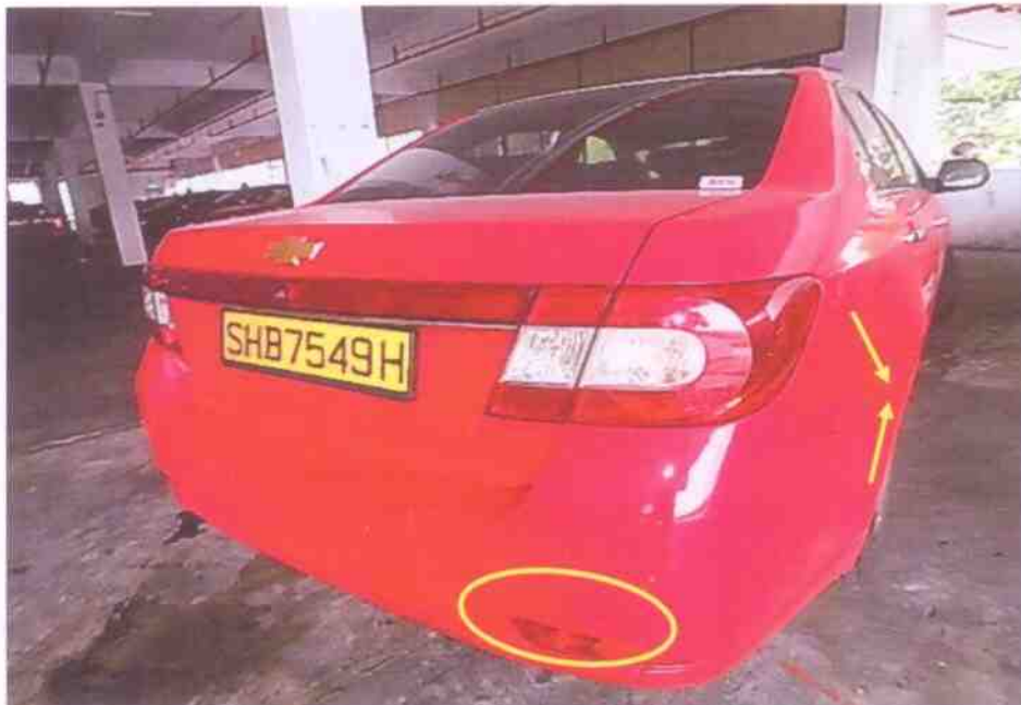
Photo 1 shows a rear view of the Taxi at the time of the Pre- Repair Survey conducted by LKK Auto Consultants Pte. Ltd. which was taken about 7 days after the accident. We observed paint graze marks above and around the rear right bumper reflector of the Taxi (circled). However we also noted that the rear bumper was not misaligned at its right corner edge (yellow arrows).
