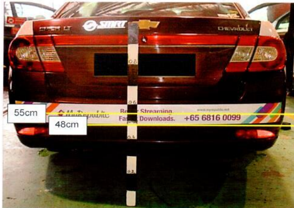
Photo 14 shows the height measurement being conducted on the rear bumper of the Taxi (using a similar make and model). The height above ground level of the lowest paint graze mark found above the rear right bumper reflector was measured to be approximately 48cm. The height above ground level of the highest paint graze mark found above the rear right bumper reflector was measured to be approximately 55cm.
