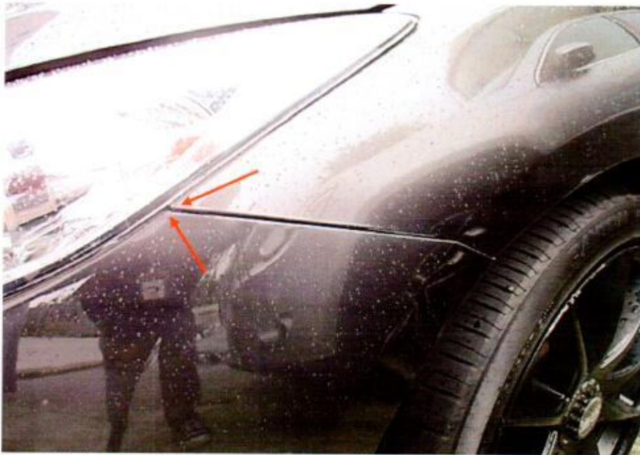
Photo 9 shows a close up view of the left corner edge of the front bumper of the Mazda. We observed that there was a slight misalignment at the left corner edge (red arrows).
