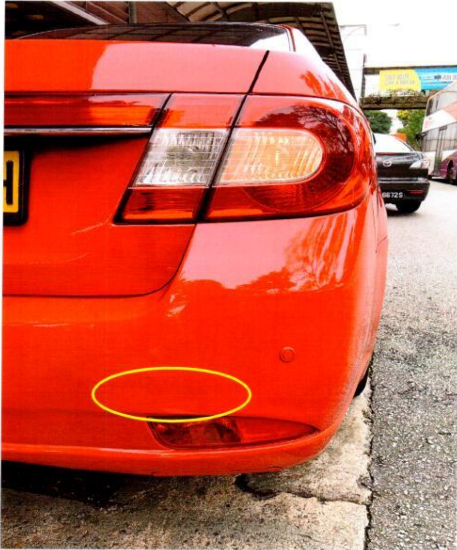
Photo 12 shows a close view of the lower right portion of the rear bumper of the Taxi taken post- accident. We observed the same paint graze marks on the lower right portion of the rear bumper of the Taxi as per the Pre- Repair Survey photographs (circled).
