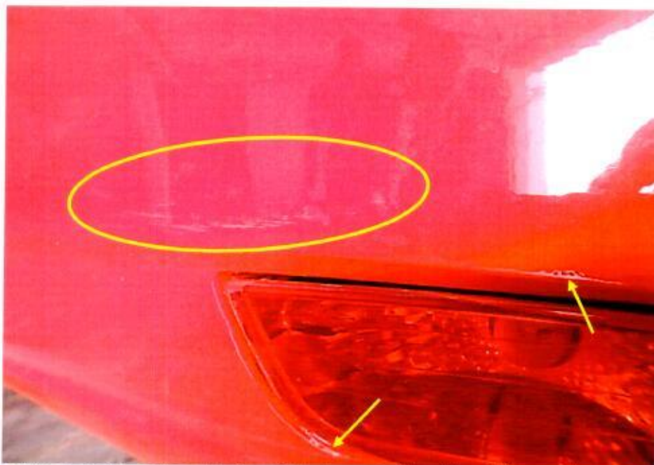
Photo 3 shows a close up view of the lower right portion of the rear bumper of the Taxi. We observed paint graze marks above (circled) and around (yellow arrows) the rear right bumper reflector of the Taxi.
