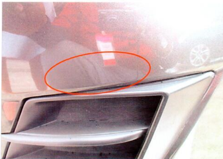
Photo 6 shows a closer view of the faint paint scratch marks above the front left air vent of the Mazda (circled).
