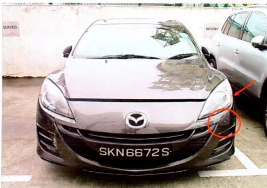
Photo 4 shows the general view of the front portion of the Mazda at the time of inspection. We noted that the Mazda had sustained a slight impact directly onto the left portion of its front bumper. Closer examination had showed faint paint scratch marks above the front left air vent (circled). We also noted that the front bumper was slightly misaligned at its left corner edge (arrowed).
