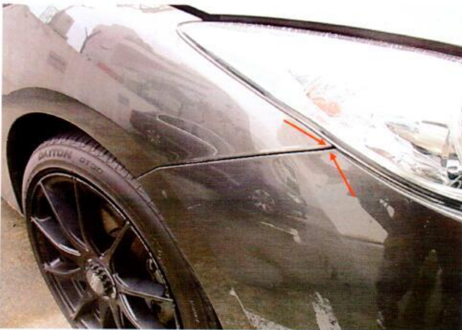
Photo 8 shows a close up view of the right corner edge of the front bumper of the Mazda. We observed that there was no misalignment at the corner edges (red arrows).
