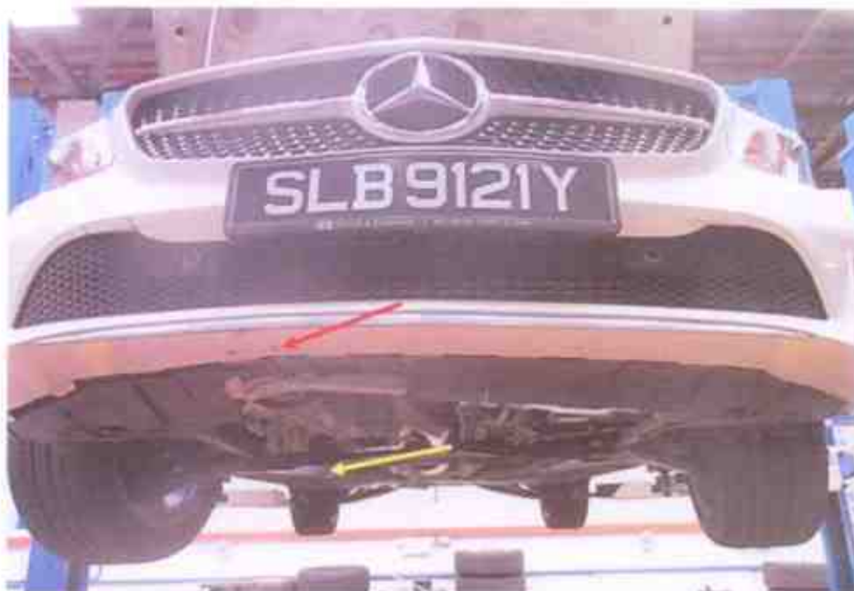
Photo 4 shows the graze marks (red arrow) that were found originating from the underside of the front bumper, onto the underside of the engine cover, stretching towards the rear (yellow arrow) of the Insured Vehicle.
