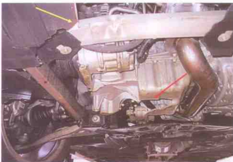
Photo 7 shows the torn front engine undercover (yellow arrow) and broken engine oil sump (red arrow) of the Insured Vehicle.
