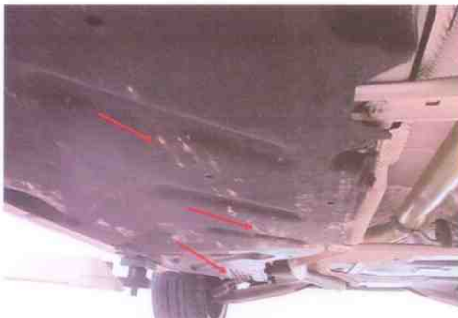
Photo 6 shows a closer view of the graze marks that had stretched towards the rear (red arrows) of the Insured Vehicle.
