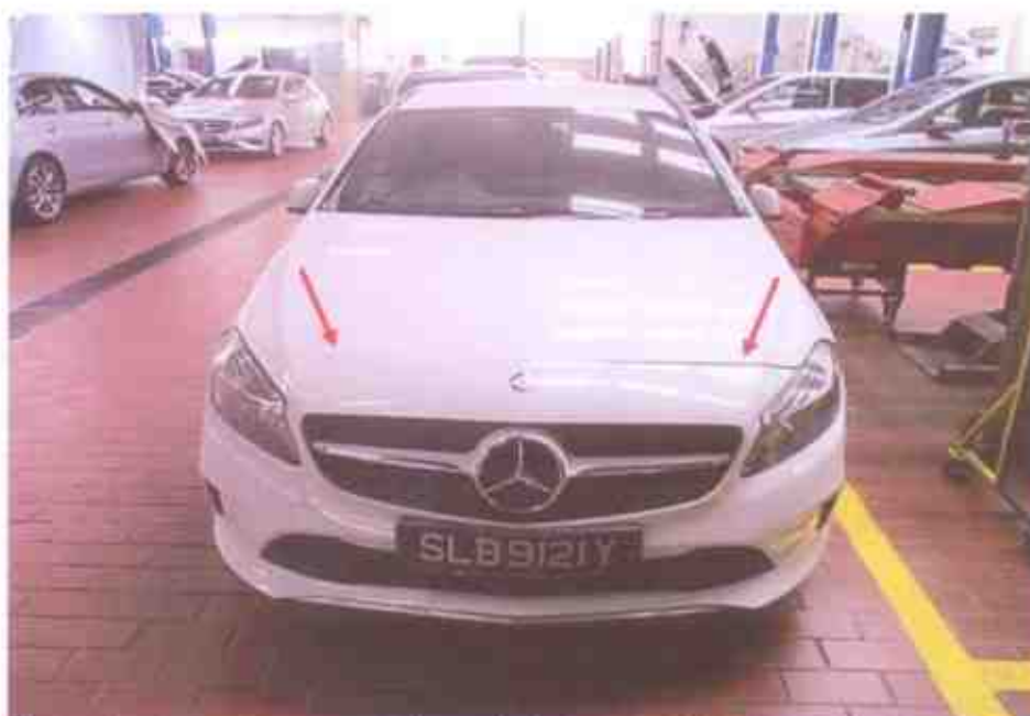
Photo 1 shows the general view of the Insured Vehicle at the time of our inspection. The Insured Vehicle was observed to be in good general condition with no visible damage to the exterior body. We did however observe that the fitment of the front bumper and front bonnet was slightly misaligned (red arrows).
