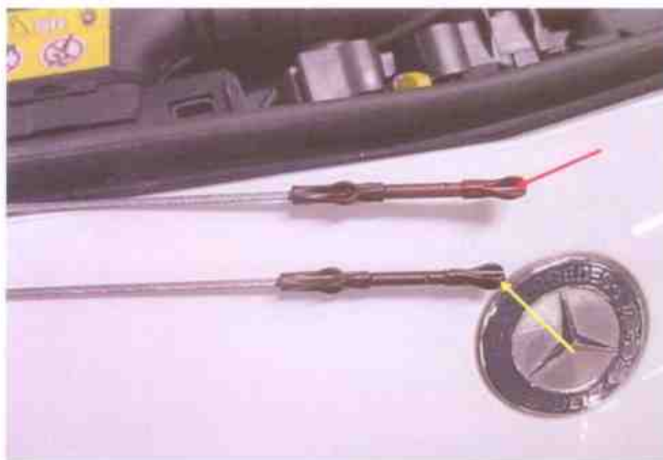
Photo 3 shows when compared with an engine oil dipstick from a similar make and model (red arrow), we observed that the engine oil dipstick of the Insured Vehicle was slightly discoloured (yellow arrow).
