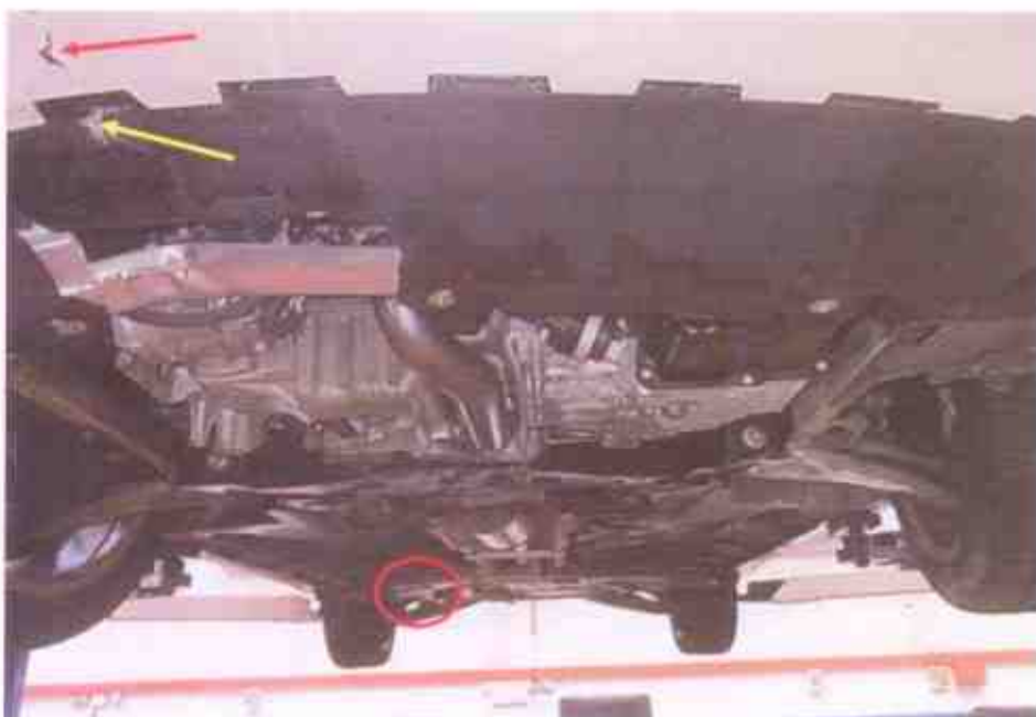
Photo 5 shows a closer view of the graze marks that were found originating from the underside of the front bumper (red arrow), onto the underside of the engine cover (yellow arrow), stretching towards the rear (circled) of the Insured Vehicle.
