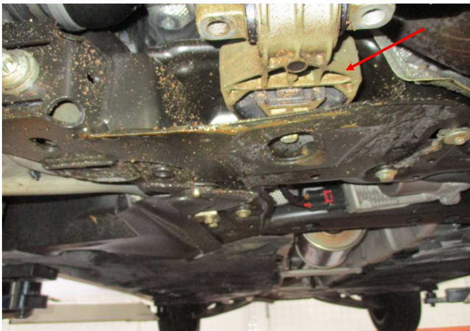
Photo 9 shows the undercarriage parts and components (arrowed) that were immediately after the punctured engine oil sump, covered with engine oil stains.
