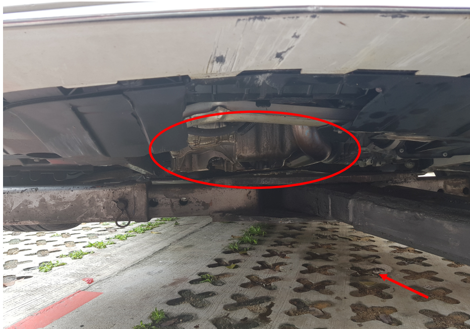
Photo 10 shows the excessive engine oil leakage was only discovered on the underside of the engine oil sump (circled) as well as on the ground (arrowed) only after the front portion of the Insured Vehicle was jacked up by the towing personnel.
