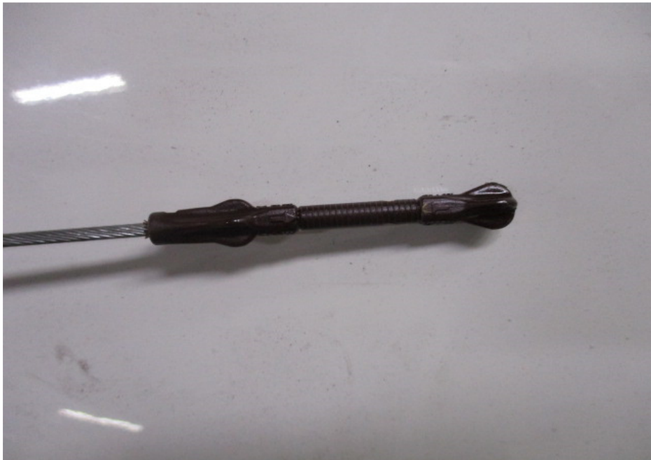
Photo 2 shows the engine oil dipstick of the Insured Vehicle, which had indicated insufficient engine oil. This was due to leakage of engine oil from a puncture/hole that was on the underside of the engine oil sump.
