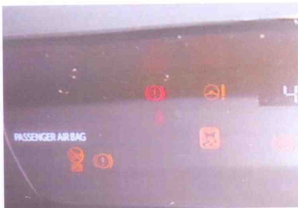
Photo 21 shows some warning lights illuminated on the instrument panel of the Motor Car after the engine was cranked. This indicates that some of the sensors failed to initialise during start-up of the engine likely due to accidents impact. However, operational test conducted on the Motor Car reveals that this does not contribute to the accident.
