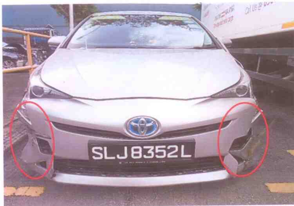
Photo 1 shows a general view of the frontal body of the Motor Car at the time of our inspection. The Motor Car had sustained relatively extensive impact damages which were confined to its frontal left & frontal right portion. The impact force was relatively significant, causing the various parts and components at the front area of the engine compartment to be damaged.
