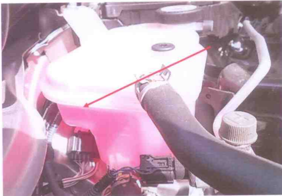
Photo 13 shows checks being carried out to the engine coolant of the Motor Car at the time of our inspection. The engine coolant was observed to be of sufficient level and without any visible contamination upon removal of the radiator cap (arrowed).
