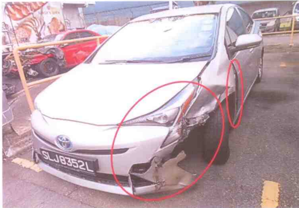
Photo 2 shows a general view of the front left body of the Motor Car at the time of our inspection. The impact force was relatively significant, causing the various parts and components at the front area of the engine compartment to be damaged.
