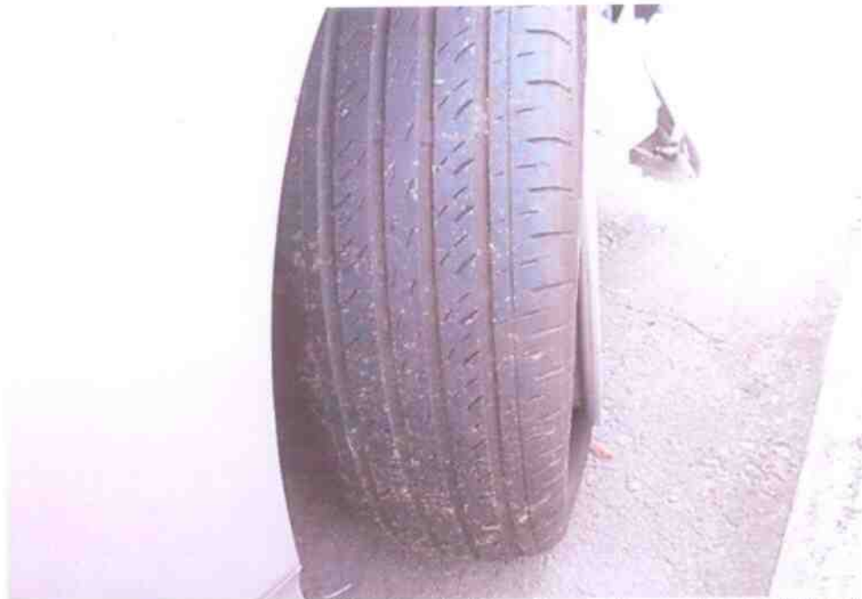
Photo 8 shows the condition of the front left tyre, it was observed to be deflated. The remaining tread depth of the front left tyre was approximately 5mm.
