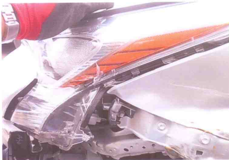
Photo 3 shows a close-up view of the front left body of the Motor Car at the time of our inspection. The impact force was relatively significant, causing the various parts and components at the front area of the engine compartment to be damaged.
