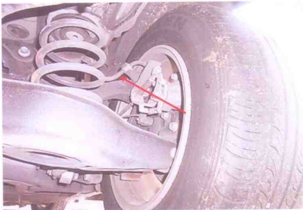
Photo 16 shows the brake hose/pipe (arrowed) at the rear right wheel of the Motor Car. We did not observe any leakage of brake fluid at the time of our inspection of the Motor Car.
