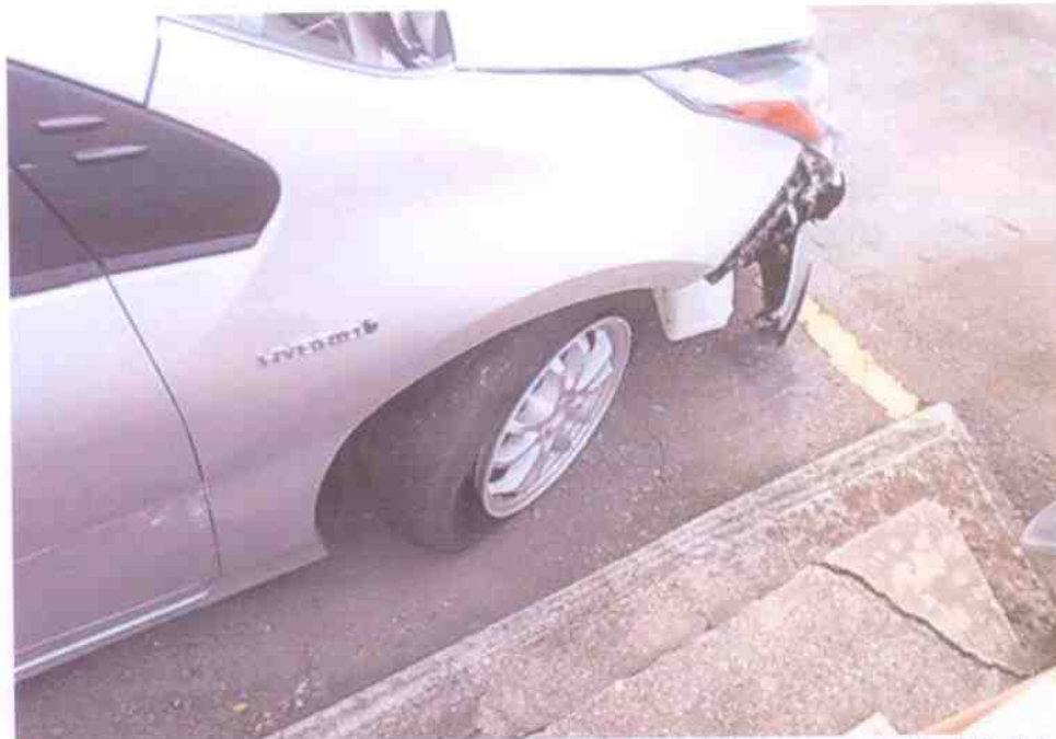
Photo 19 shows the front right wheel of the Motor Car turned to its full right. During our steering system test, we did not experience any abnormal free play and/or resistance when we turned the steering wheel towards the left and right. This would suggest that the steering system of the Motor Car was likely to be in serviceable condition at the material time of accident.
