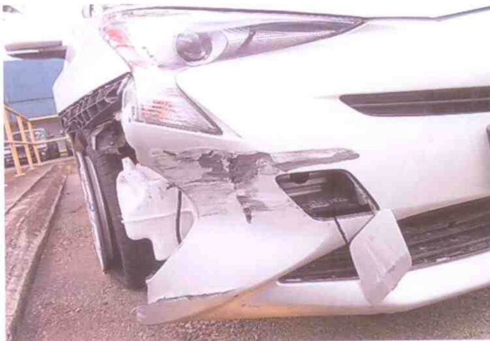
Photo 3 shows a close-up view of the front right body of the Motor Car at the time of our inspection. The impact force was relatively significant, causing the various parts and components at the front area of the engine compartment to be damaged.
