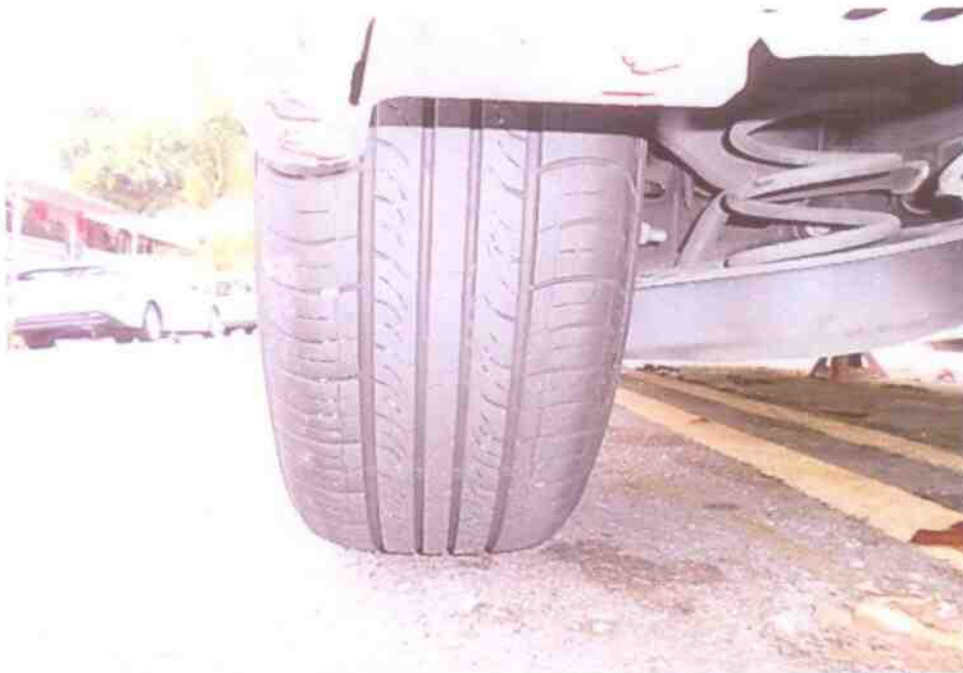
Photo 9 shows the condition of the rear left tyre of the Motor Car, which was observed to be in serviceable condition with remaining tread depth of approximately 5mm. The tyre, which was wrapped around alloy wheel rim, was also observed to be sufficiently inflated for vehicular operation.
