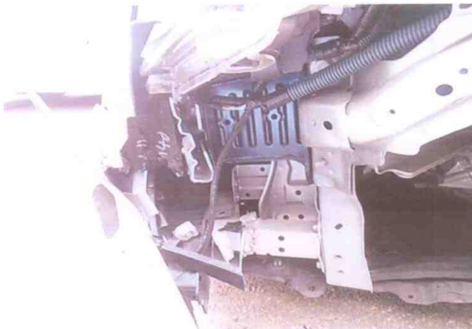
Photo 3 shows a close-up view of the front left body of the Motor Car at the time of our inspection. The impact force was relatively significant, causing the various parts and components at the front left area of the engine compartment to be damaged.
