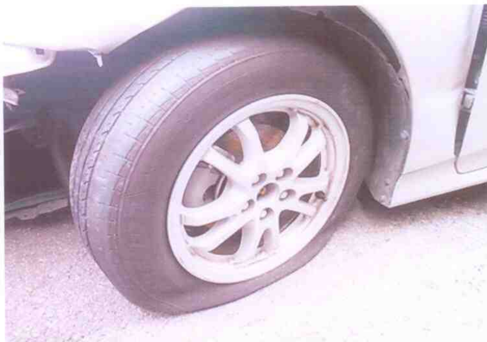
Photo 6 shows the condition of the front left tyre, it was observed to be deflated likely due to the accident's collision impact.
