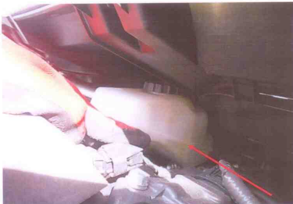
Photo 12 shows the brake fluid reservoir of the Motor Car at the time of our inspection. The brake fluid was observed to be of sufficient level and without any visible contamination (arrowed).
