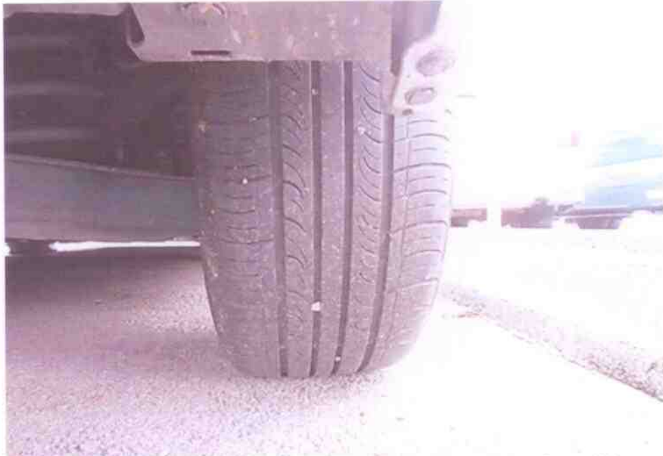
Photo 10 shows the condition of the rear right tyre of the Motor Car, which was observed to be in serviceable condition with remaining tread depth of approximately 6mm. There was also no tear, cut or burst mark(s) on the outer and the inner sidewalls as well as across the tread of the 4 tyres.
