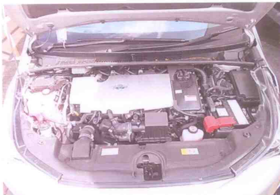
Photo 11 shows a general view of the Motor Car's engine compartment. The various parts and components inside the engine compartment were unaffected by the accident. There was also no sign(s) or indication(s) of fluid leakage and/or fluid stain within the engine compartment.
