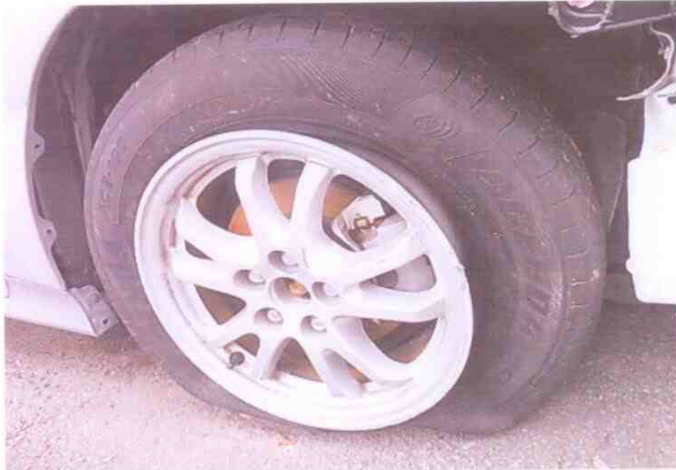
Photo 6 shows the condition of the front right tyre, it was observed to be deflated likely due to the accident's collision impact.
