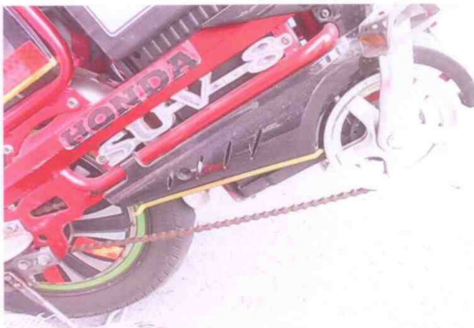
Photo 10 shows the general view of the gear train (arrowed) of the Electric Bicycle, which was observed to be intact with no misalignment.
