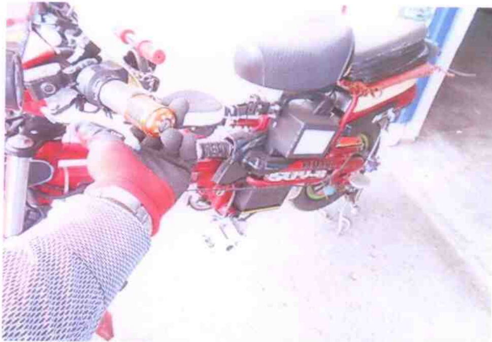
Photo 16 shows a static brake test was conducted only on the Bicycle's front brake. The test was conducted by lifting the front tyre in the air & applies a little spinning action to it. The hand brake lever was then gripped in order to stop the spinning front tyre. The result was unsatisfactory. It didn't stop after gripping the hand brake to the fullest.
