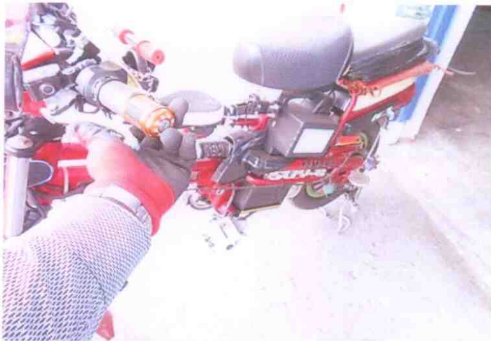
Photo 15 shows a static brake test was conducted only on the Bicycle's rear brake. The test was conducted by lifting the rear tyre above ground & applies a little spinning action to it. The hand brake lever was then gripped in order to stop the spinning front tyre. The result was satisfactory. It stopped after gripping the left hand brake to the fullest. It shows that the rear brake clamps was responding to the gripping action. This had appeared to indicate that the rear brake was in a serviceable condition.
