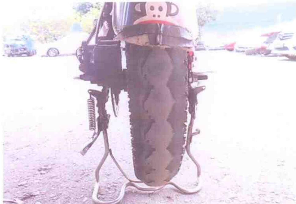
Photo 8 shows the rear tyre of the Electric Bicycle at the time of our inspection. The tread pattern of the 2 tyres was clearly visible. We did not observe any tear, burst mark(s) and/or punctured hole(s) on the sidewalls.
