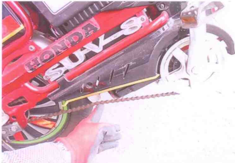
Photo 11 shows a close-up view of the rear chain of the Bicycle at the time of our inspection. Free play tension test was also conducted & found adequately acceptable. It was also observed to be in operational condition.
