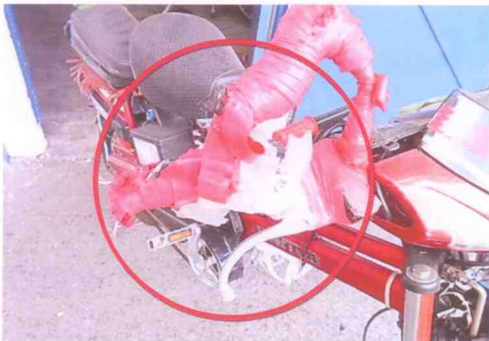
Photo 3 shows the right portion of the Electric Bicycle at time of inspection. Damage on the right hand handle, brake lever & right hand foot pedal was observed likely due to the accident.
