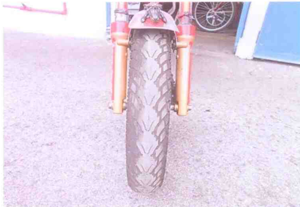
Photo 9 shows the front tyre of the Electric Bicycle at the time of our inspection. The tread pattern of the 2 tyres was clearly visible. We did not observe any tear, burst mark(s) and/or punctured hole(s) on the sidewalls.
