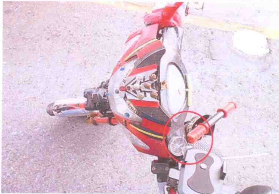
Photo 14 shows the handle bar of the Electric Bicycle while trying to turn to the fullest left. It was hindered by an additional child seat handle bar that was installed in the middle section of the Electric Bicycle's body. Hence, disrupting the normal operating sequence for the Electric Bicycle's steering system.
