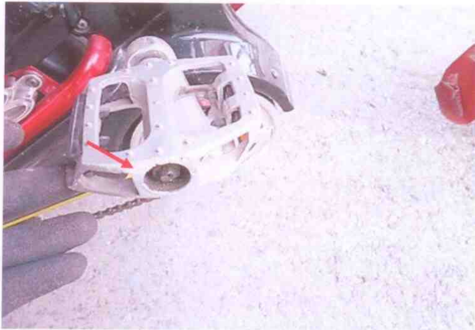
Photo 4 shows the right portion of the Electric Bicycle at time of inspection. Damage on the right hand foot pedal was observed likely due to the accident.
