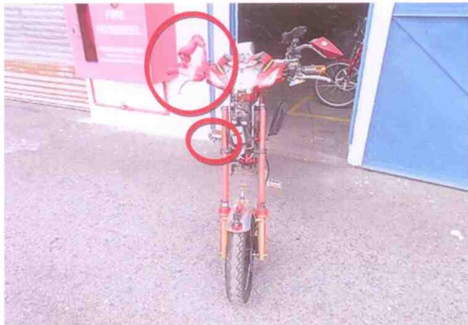
Photo 2 shows the frontal portion of the Electric Bicycle at time of inspection. Damage on the right hand handle & right hand foot pedal was observed likely due to the accident.
