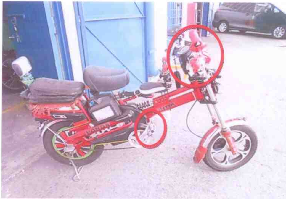
Photo 2 shows the right portion of the Electric Bicycle at time of inspection. Damage on the right hand handle & right hand foot pedal was observed likely due to the accident.
