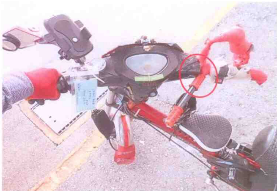
Photo 13 shows the handle bar of the Electric Bicycle while trying to turn to the fullest right. It was hindered by an additional child seat handle bar that was installed in the middle section of the Electric Bicycle's body. Hence, disrupting the normal operating sequence for the Electric Bicycle's steering system.
