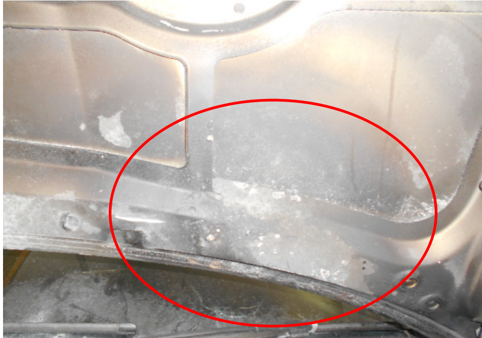
Photo 6 shows the whitish burn marks that were found on the underside of the front bonnet, directly under the area where the same whitish burn marks were found on the top side of the front bonnet. The rust (circled) that had developed around this area was a result of prolong exposure to high heat intensity, which had caused the steel/metal material of the front bonnet to be exposed to natural environmental condition.
