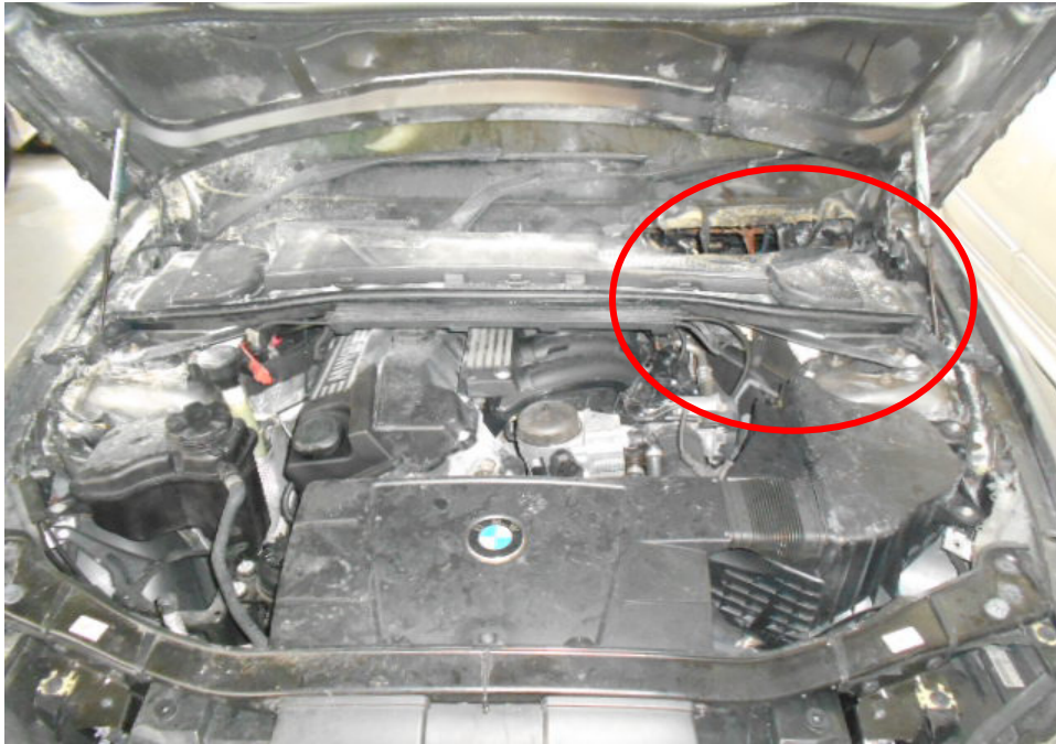
Photo 3 shows the engine compartment of the Insured Vehicle at the time of our inspection. The engine compartment of the Insured Vehicle was observed to be partially burnt. Some parts inside the engine compartment, at the rear left area (circled), were found to be burnt and/or melted as a result of the fire.
