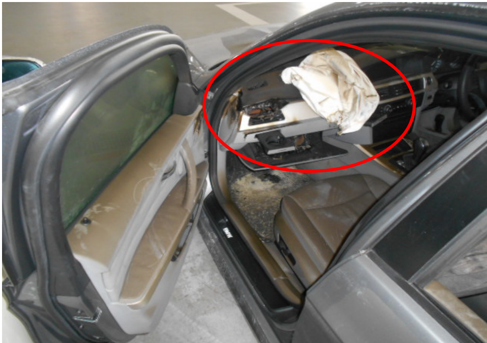
Photo 4 shows the interior compartment of the Insured Vehicle, which was observed to be partially burnt and/or melted. The front dashboard & front windscreen were amongst the parts that were found to have been burnt and/or melted as a result of the fire. The front left air bag was also found to be activated due to the incident.
