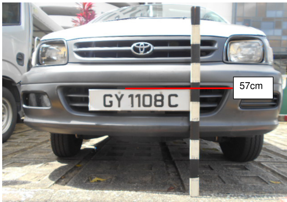
Photo 16 shows the height measurement that was conducted on the frontal portion of the Insured Vehicle. The top end of the front number plate was found to be 57cm above ground level.
