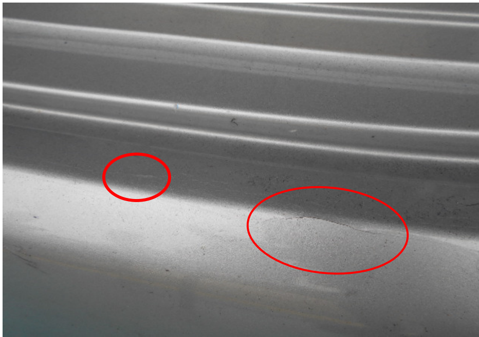
Photo 7 shows the slight paint cracks (circled) that was observed on the top surface area of the Third Party Vehicle's rear bumper. Such paint cracks are usually caused when a force/load is applied to the rear bumper, causing the rear bumper to be compressed inwards. Due to the elastic nature of the rear bumper, the paint at the top surface area of the rear bumper would tend to crack when the rear bumper returns back to shape after being compressed inwards.
