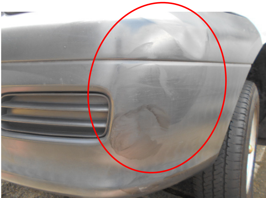
Photo 10 shows the grazed marks (circled) that were found on the left corner area of the Insured Vehicle's front bumper. These grazed marks were amongst the multiple damages that were found on the front bumper of the Insured Vehicle.
