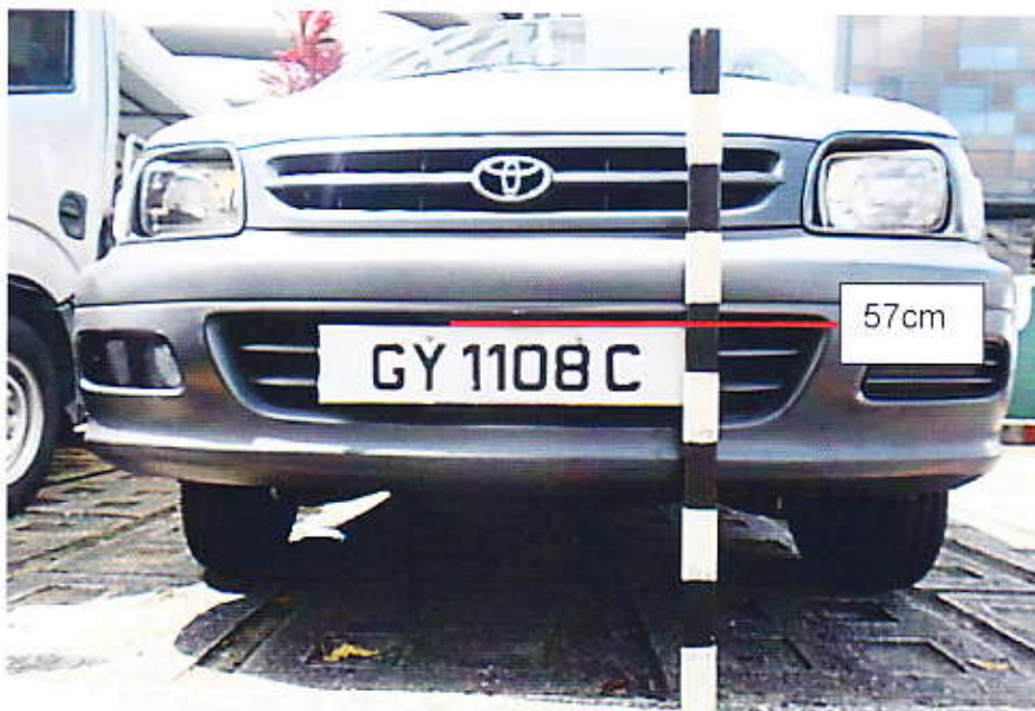
Photo 16 shows the height measurement that was conducted on the frontal portion of the Insured Vehicle. The top end of the front number plate was found to be 57cm above ground level.
