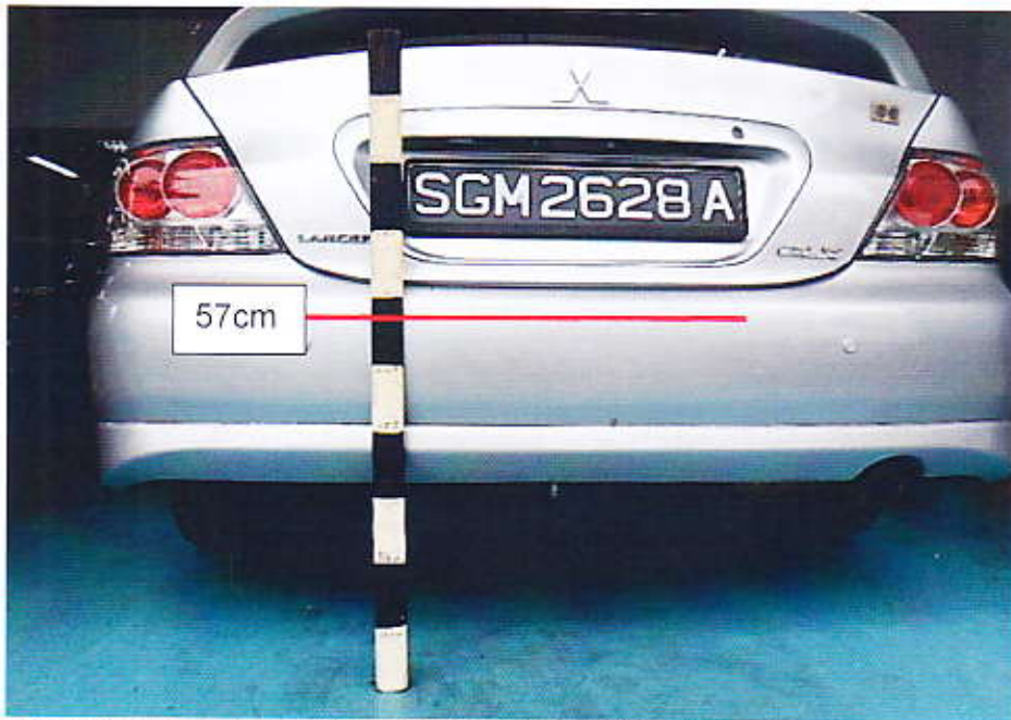
Photo 15 shows the height measurement that was conducted on the rear portion of the Third Party Vehicle. The height above ground level of the minor scratches on the centre area of the rear bumper was approximately 57cm.
