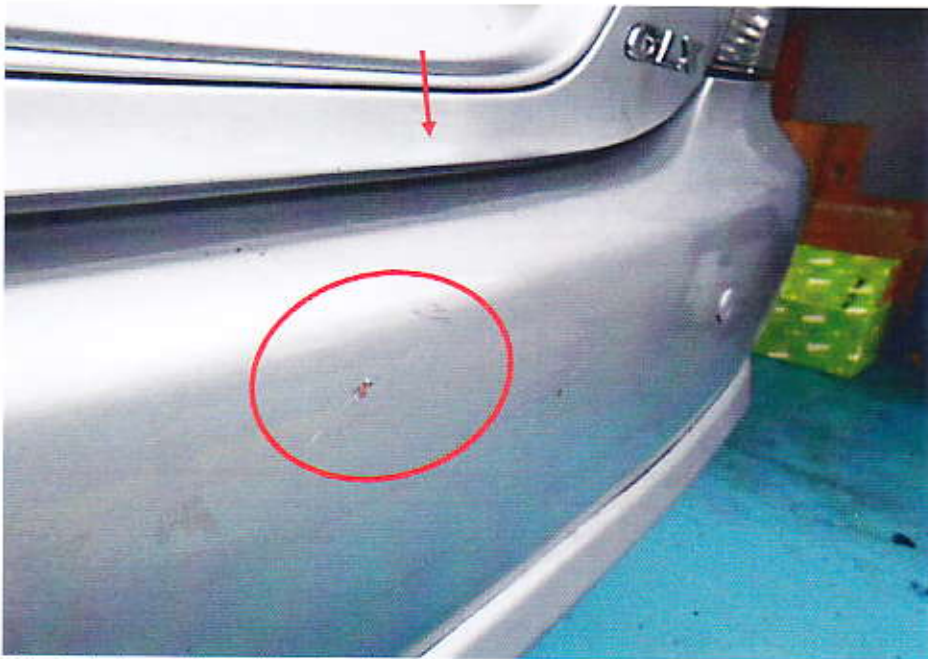
Photo 5 shows the relatively minor scratch marks (circled) that were observed on the rear bumper, and slight dent (arrowed) that was observed on the lower edge of the rear bootlid.
