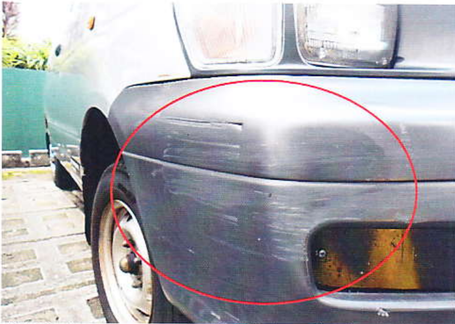
Photo 11 shows the grazed marks (circled) that were found on the right corner area of the Insured Vehicle's front bumper. These grazed marks were amongst the multiple damages that were found on the front bumper of the Insured Vehicle.
