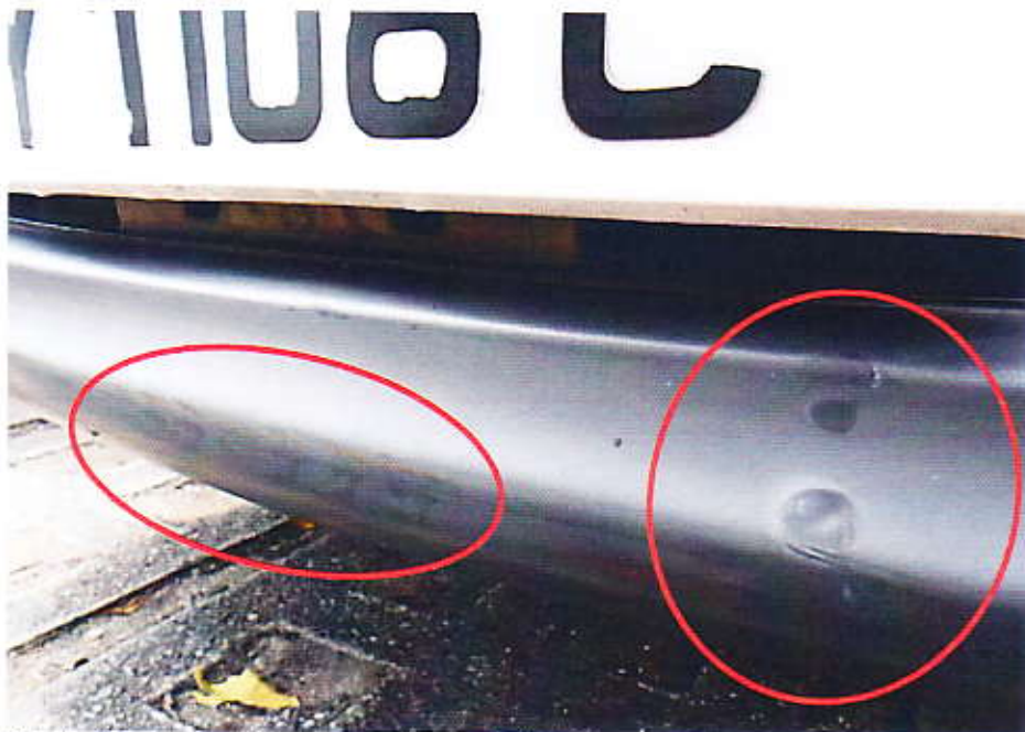
Photo 13 shows the damage (circled) that was found on the lower part of the Insured Vehicle's front bumper, at the centre area of the front bumper. These damages were amongst the multiple damages that were found on the front bumper of the Insured Vehicle.
