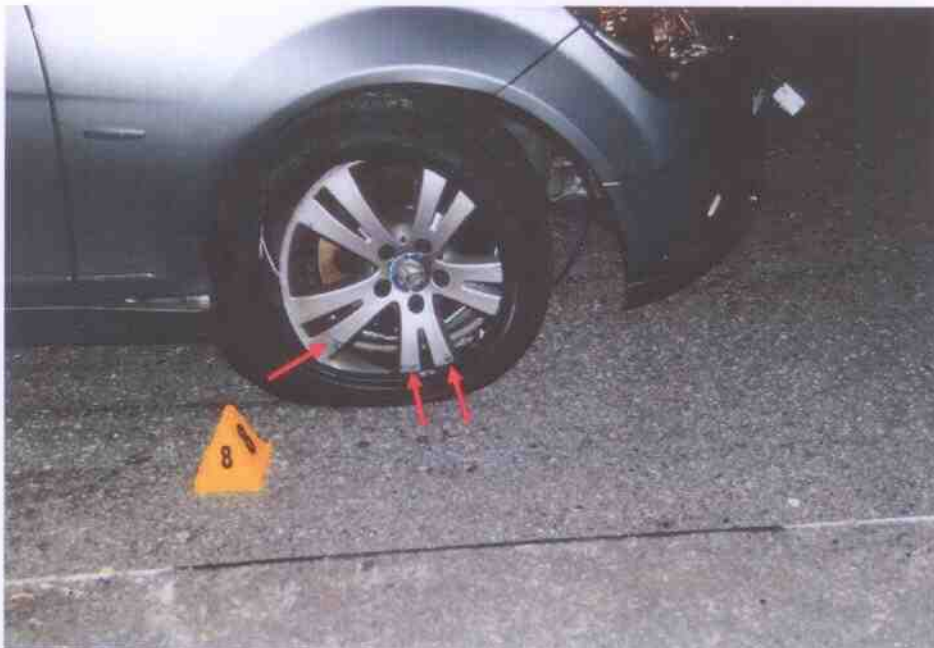
Photo 3 shows the Motor Car at the accident scene. The front right wheel rim was broken while the front right tyre was deflated and loosely wrapped around the front right wheel rim. The exterior surfaces of the wheel rim did not appear to have sustained any significant damage except for some blackish grazed marks (arrowed) on its outer spokes.
