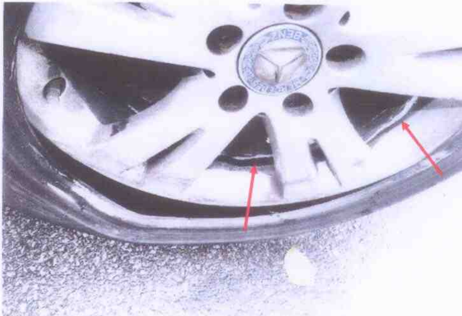
Photo 4 shows a closer view of the damaged front right wheel rim of the Motor Car. Upon closer examination of the photograph, it was observed that the front right wheel rim was broken on the inner side width of the wheel rim (arrowed). This indicates that the impact causing the wheel rim to be broken was from the underside of the Motor Car and not from the exterior side of the Motor Car.
