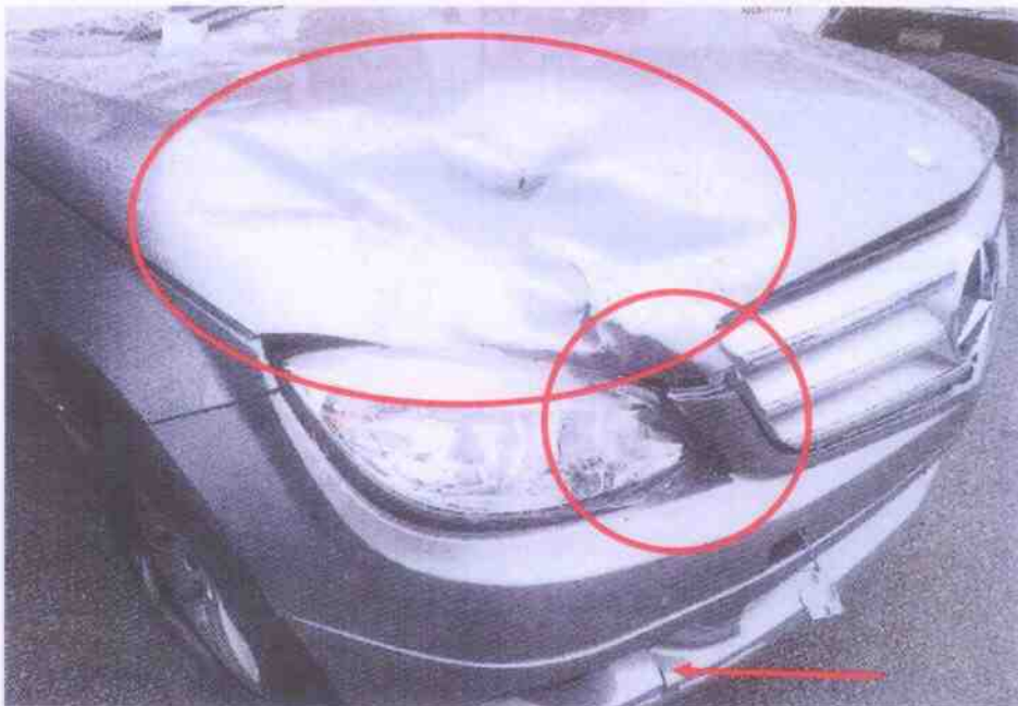
Photo 2 shows the front body of the Motor Car. The damage to the front bumper (arrowed), front right headlamp and front bonnet (circled) were all caused by the Motor Car's collision with the Deceased.
