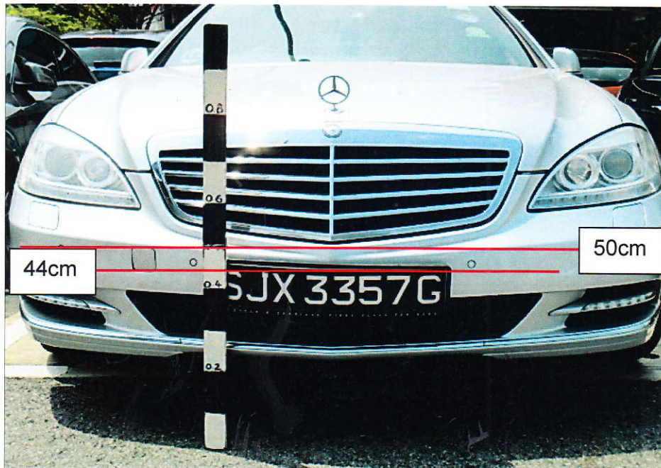
Photo 9 shows the height measurement being conducted on the front portion of the Mercedes. The height above ground level of the bottom portion of the Mercedes's front right tow cover which was observed to be pushed inwards was measured to be approximately 44cm. The height above ground level of the top corners of the Mercedes's front number plate frame was also measured to be approximately 44cm. The height above ground level of the top portion of the Mercedes's front right tow cover was measured to be approximately 50cm.
