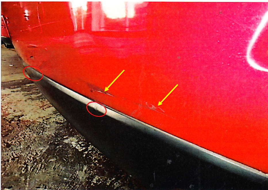
Photo 4 shows a close up view of the paint graze marks (yellow arrows) on the centre portion of the Taxi's rear bumper as well as vertical indentations (red circles) on the lower rear bumper of the Taxi.
