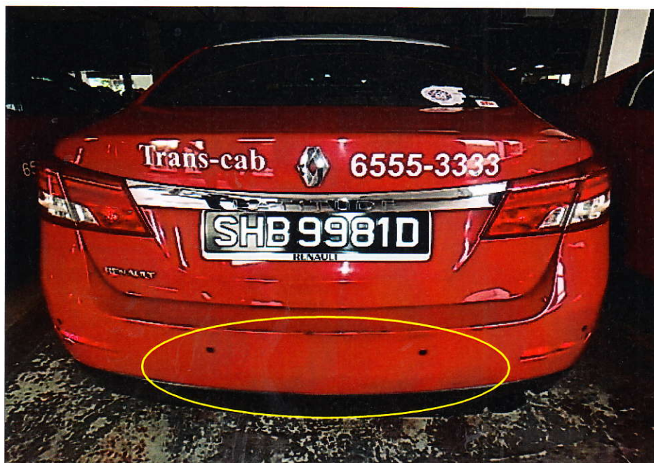
Photo 1 shows the general view of the rear of the Taxi at the time of the Pre-Repair Survey conducted by LKK Auto Consultants Pte. Ltd. taken 2 days after the accident. The damage to the Taxi was observed to be confined to its rear centre portion (circled).
