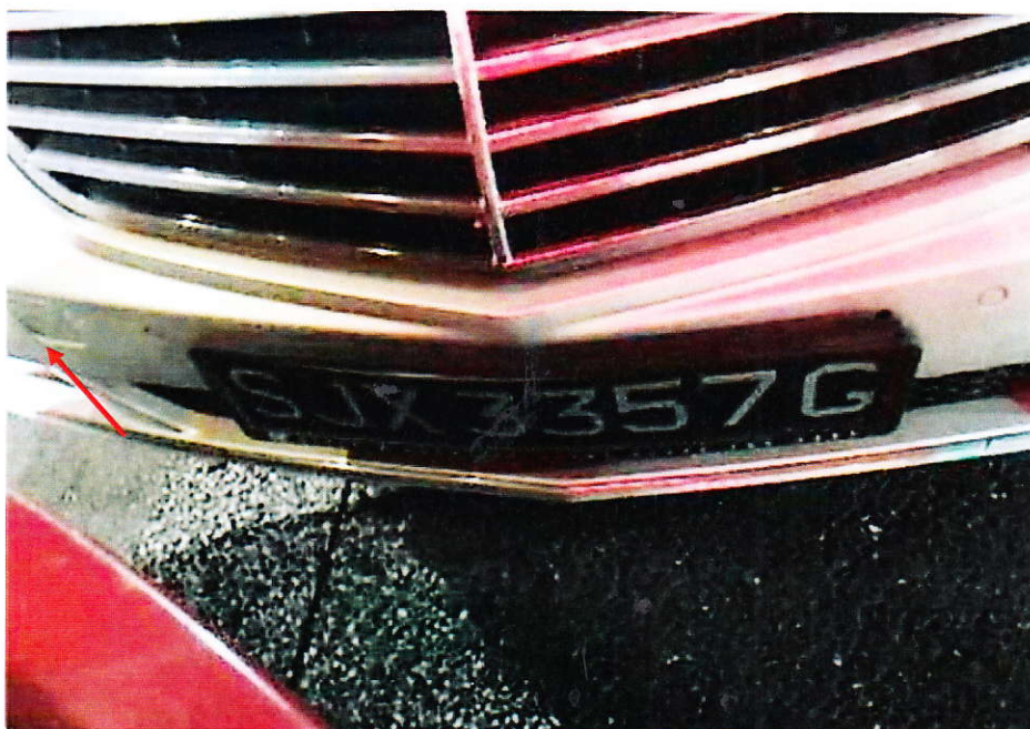
Photo 7 shows the position of the Mercedes after the accident. Upon closer examination we observed that the front right tow cover of the Mercedes was pushed inwards (arrowed).
