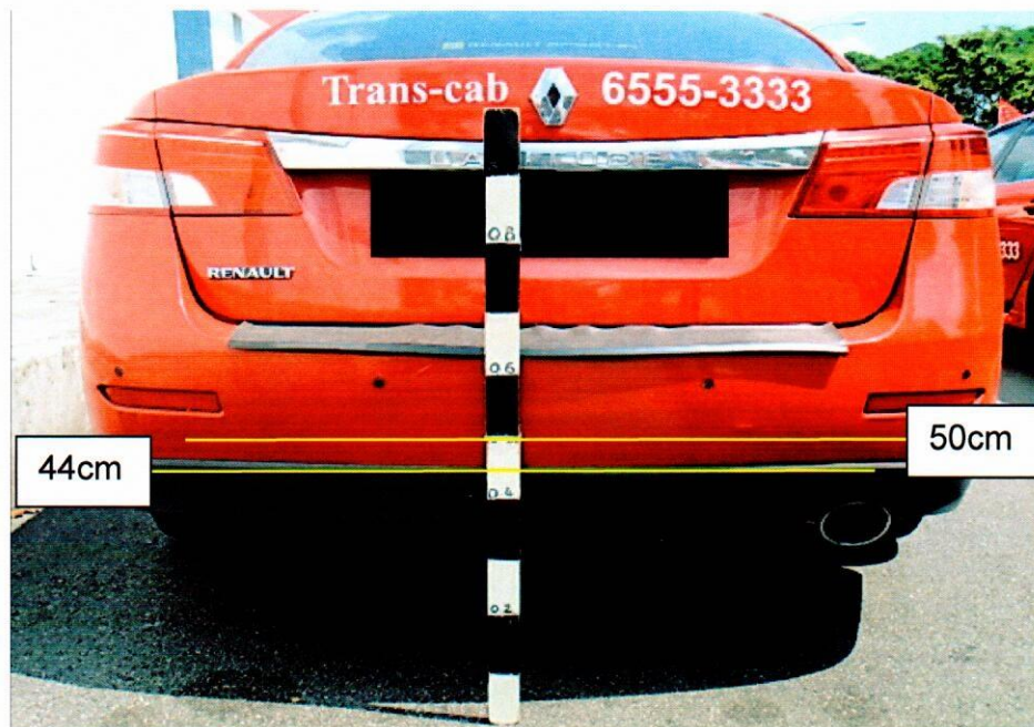
Photo 8 shows the height measurement being conducted on the rear portion of the Taxi (using a similar make and model). The height above ground level of the Taxi's lower rear bumper where the vertical indentations were found was measured to be approximately 44cm. The height above ground level of the Taxi's rear bumper where the dent and paint graze marks were found was measured to be approximately 50cm.
