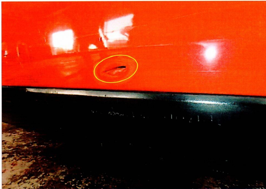
Photo 3 shows a close up view of the dent (yellow circle) on the centre portion of the Taxi's rear bumper.
