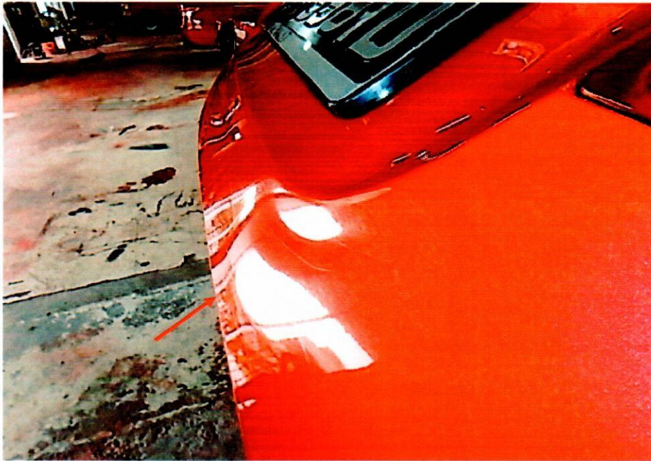
Photo 5 shows a close up view of the slight dent on the lower centre portion of the Taxi's boot lid (arrowed).
