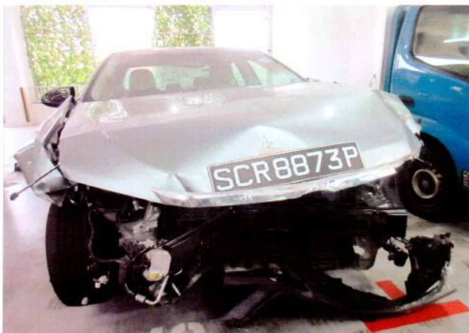
Photo 14 shows the general front view of the Insured Vehicle during the physical inspection at KKH. The Insured Vehicle had sustained extensive damages to its entire front portion, particularly to its front windscreen, front bonnet, front bumper, front bumper reinforcement panel and side panels.
