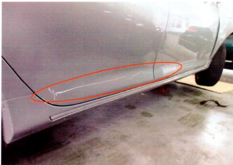
Photo 20 shows a closer view of the graze marks observed on the lower right portion of the Insured Vehicle (circled), corresponding to Mr Chong mounting the kerb.
