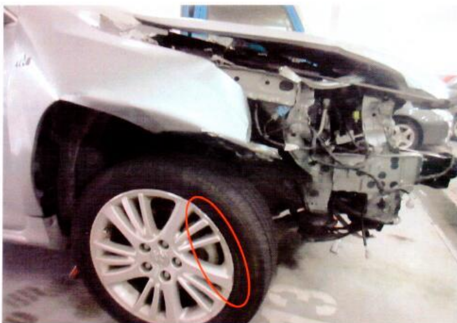
Photo 18 shows some relatively minor marks of grazing nature observed around the edges of the front right wheel rim (circled) as a result of Mr Chong mounting the kerb.
