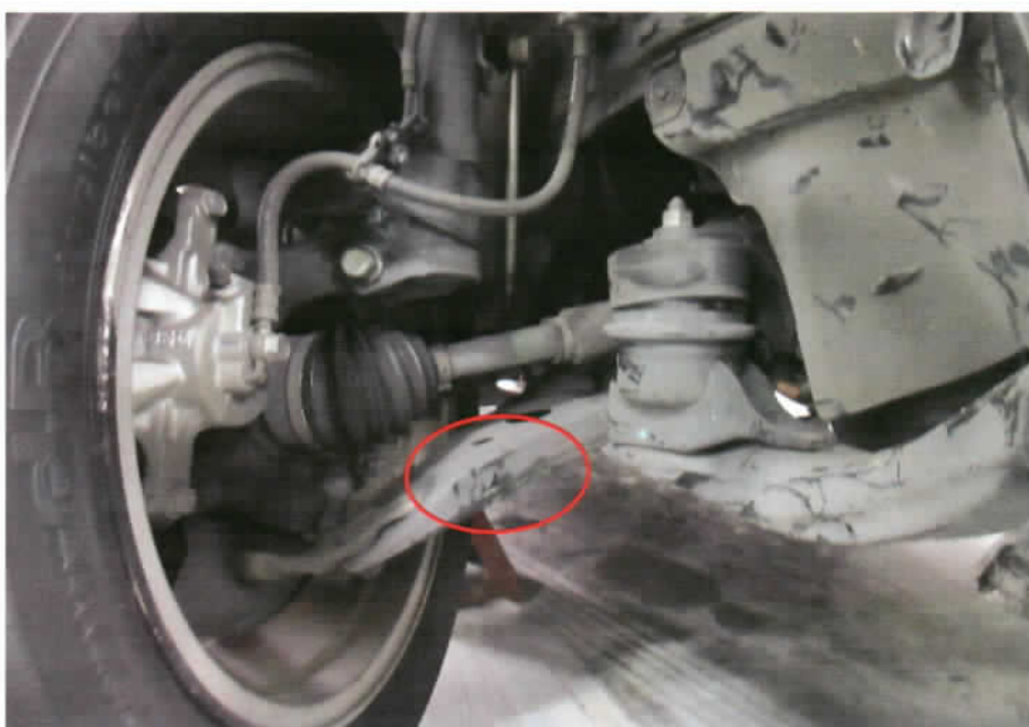
Photo 16 shows the green paint transfer marks found on the right tie rod of the Insured Vehicle (circled), corresponding to the Insured Vehicle running over the greenish metal railings.
