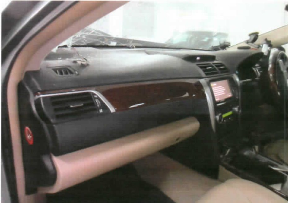
Photo 21 shows the interior compartment of the Insured Vehicle. There were no remains of both airbags which corroborates with Mr Chong's statement that none of the airbags were deployed upon the Insured Vehicle's collision with the tree.
