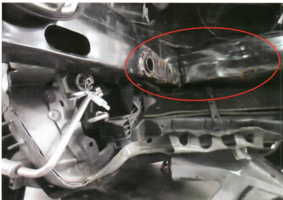
Photo 15 shows a closer view of the broken pieces of tree bark and/or soil particles that were found stuck to the front bumper reinforcement panel (circled) of the Insured Vehicle.
