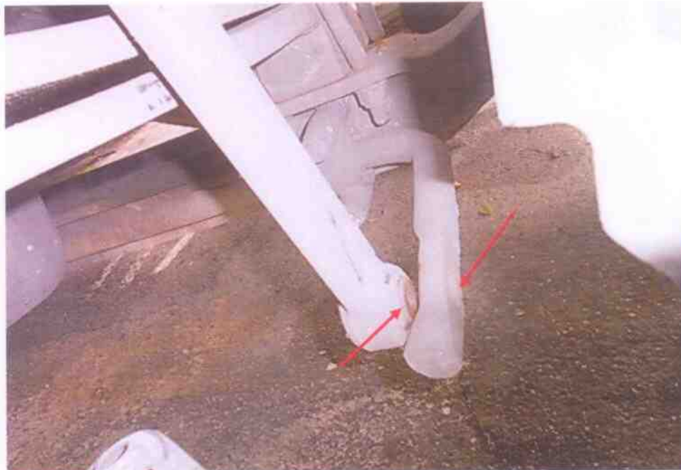
Photo 16 shows the steering rod at the front left wheel of the Tow Truck. It was observed to be dislodged from the original installation likely due to the accident's collision impact.
