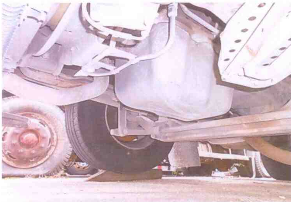
Photo 14 shows a general view of the underside of the engine compartment area. The engine assembly was observed to be intact and unaffected by the collision. There was also no sign(s) or indication(s) of fresh fluid leak and/or fluid stain found.
