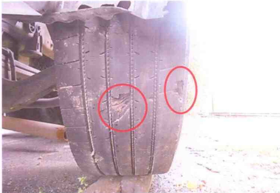
Photo 7 shows the condition of the front left tyre of the Tow Truck, which was observed to be chipped off at time of our inspection. However, it was still in serviceable condition with remaining tread depth of approximately 10mm.
