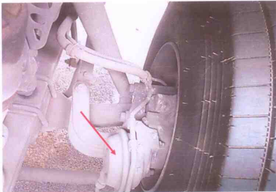
Photo 22 shows the brake air cylinder (arrowed) at the front right wheel of the Tow Truck. Such air cylinder, which is amongst the various components for the full air-assisted braking system, can be found attached to all the front wheels and all the wheels of the Tow Truck. Upon our checks, we had found all the brake air cylinders to be undamaged and securely fitted to all the wheels of the Tow Truck.
