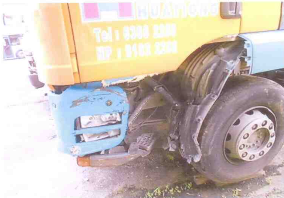
Photo 5 shows a semi close-up view of the damaged area on the front left hand side of the Tow Truck.
