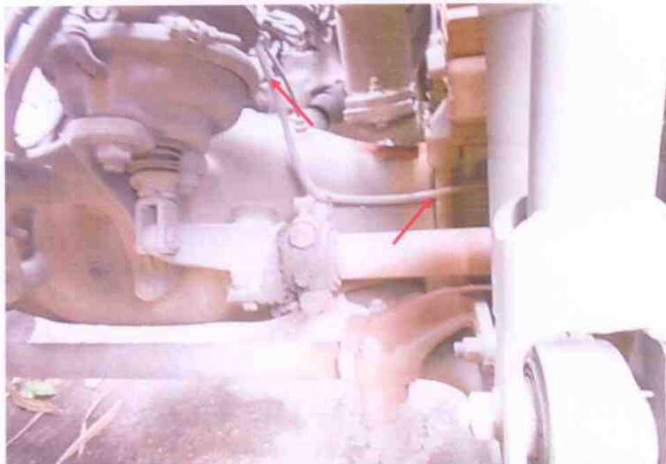
Photo 21 shows the brake hoses (arrowed) leading to the rear right wheel of the Tow Truck. At the time of our inspection, the various mechanical components of the air-assisted hydraulic braking system of the Tow Truck were all found to be in good general condition and securely fitted.
