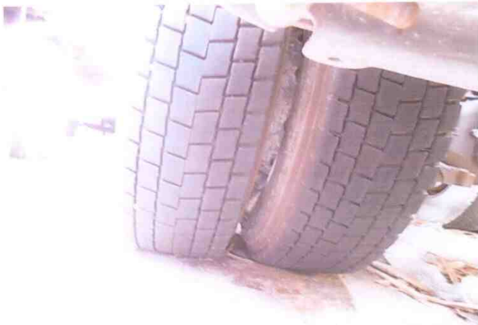
Photo 12 shows the condition of the rear right tyres (centre axle) of the Garbage Truck, which were observed to be in serviceable condition with remaining, tread depth of approximately 5mm. The tyres, which were wrapped around standard alloy wheel rims, were also observed to be sufficiently inflated for vehicular operation.
