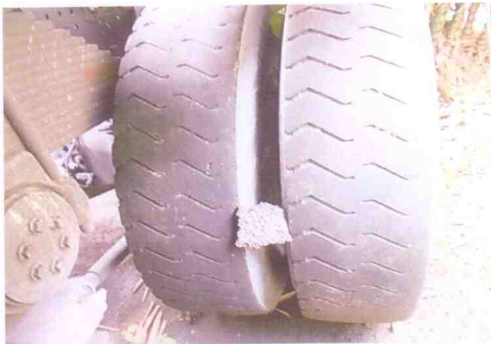
Photo 10 shows the condition of the rear left tyres of the Tow Truck, which were observed to be in serviceable condition with remaining tread depth of approximately 10mm. The tyres were also observed to be sufficiently inflated for vehicular operation.
