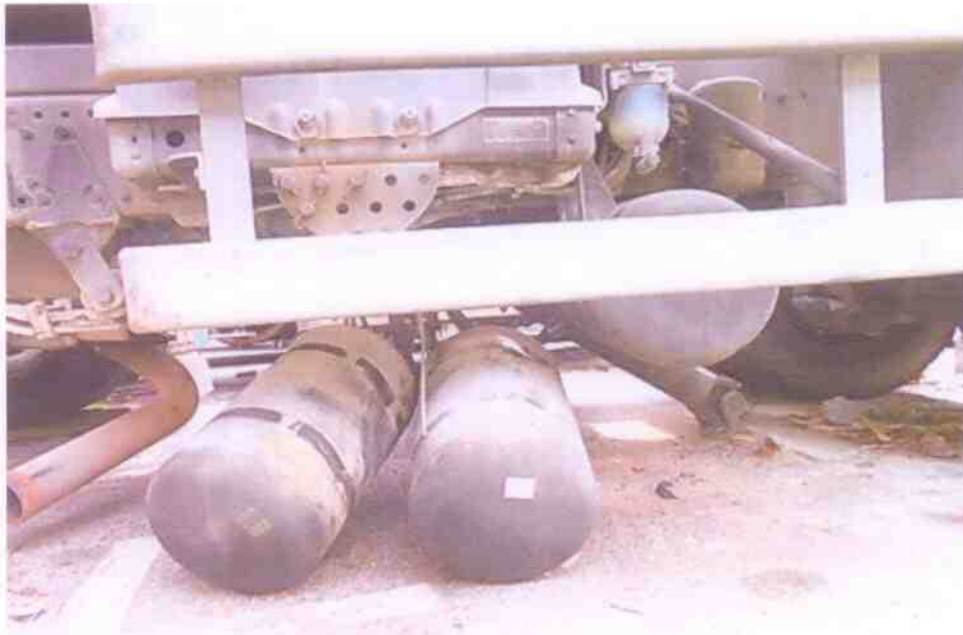
Photo 18 shows the air tanks, valves, pipes and hoses, which was found to be damaged as a result of the accident's impact.
