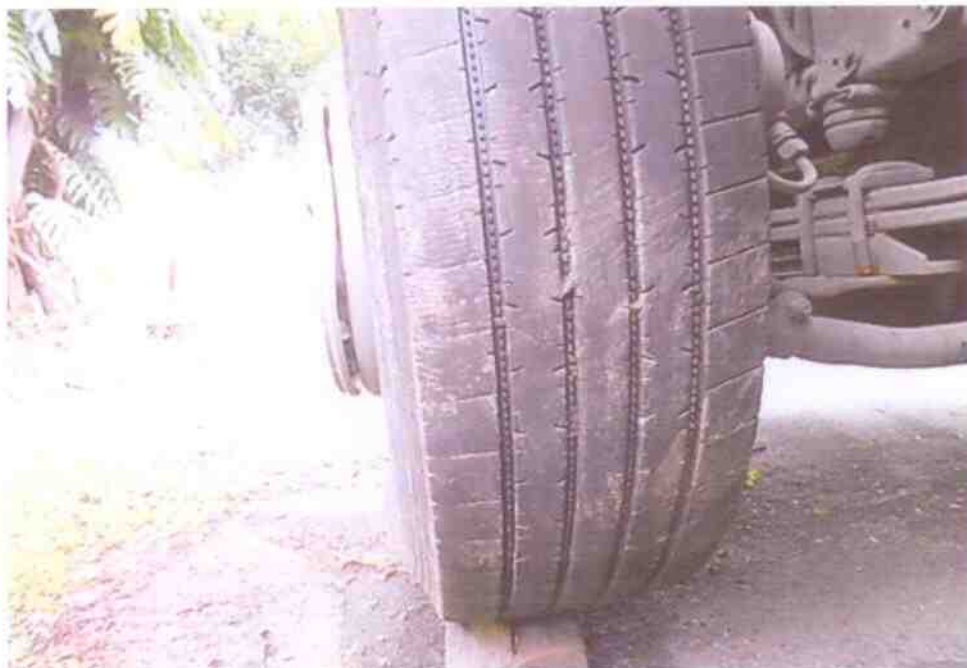
Photo 8 shows the condition of the front right tyre of the Tow Truck, which was observed to be in serviceable condition with remaining tread depth of approximately 8mm.
