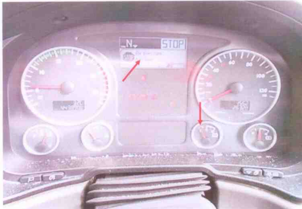
Photo 20 shows the air pressure meter on the dashboard, it indicates that there a low pressure on the air pressure while in idling mode.
