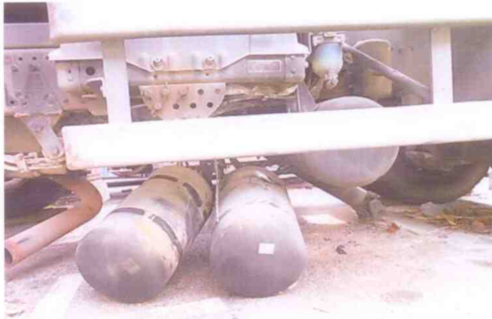
Photo 6 shows a semi close-up view of the damaged air pressure tank. It was dislodged from the original installation likely due to the accident's impact.
