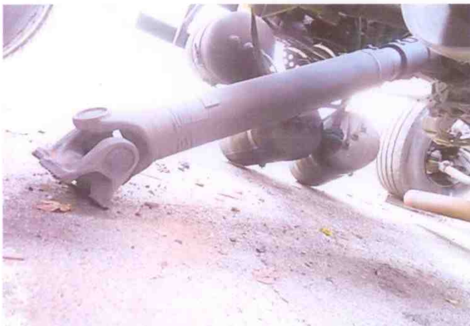
Photo 15 shows the propeller shaft of the Tow Truck at the time of our inspection. It was observed to be dislodged from the original installation likely due to the accident's collision impact.
