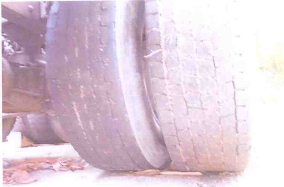
Photo 9 shows the condition of the rear left tyres (centre axle) of the Tow Truck, which were observed to be in serviceable condition with remaining tread depth of approximately 10mm. The tyres were also observed to be sufficiently inflated for vehicular operation.
