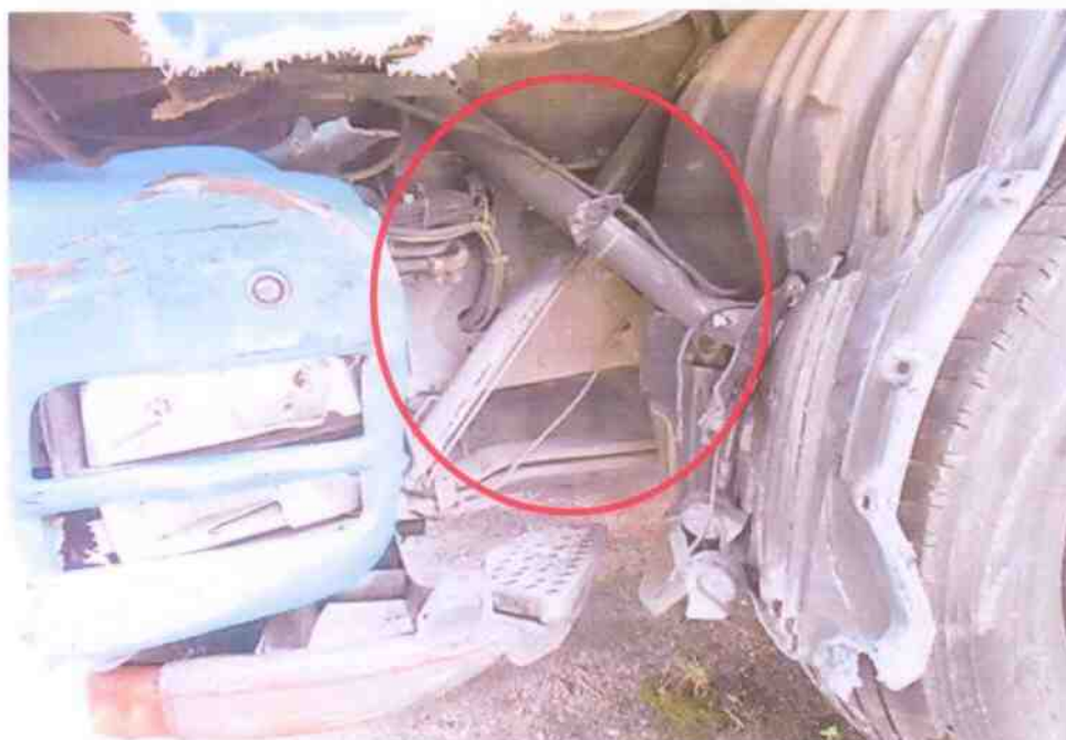
Photo 13 shows a semi close-up view of the damaged hydraulic jack that lifted up the front cabin likely due to the accident's collision impact.
