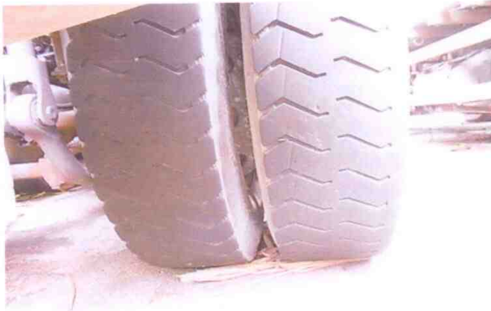
Photo 11 shows the condition of the rear right tyres of the Tow Truck, which were observed to be in serviceable condition with remaining, tread depth of approximately 8mm. The tyres were also observed to be sufficiently inflated for vehicular operation with no tear, cut or burst mark(s) on the outer and the inner sidewalls.
