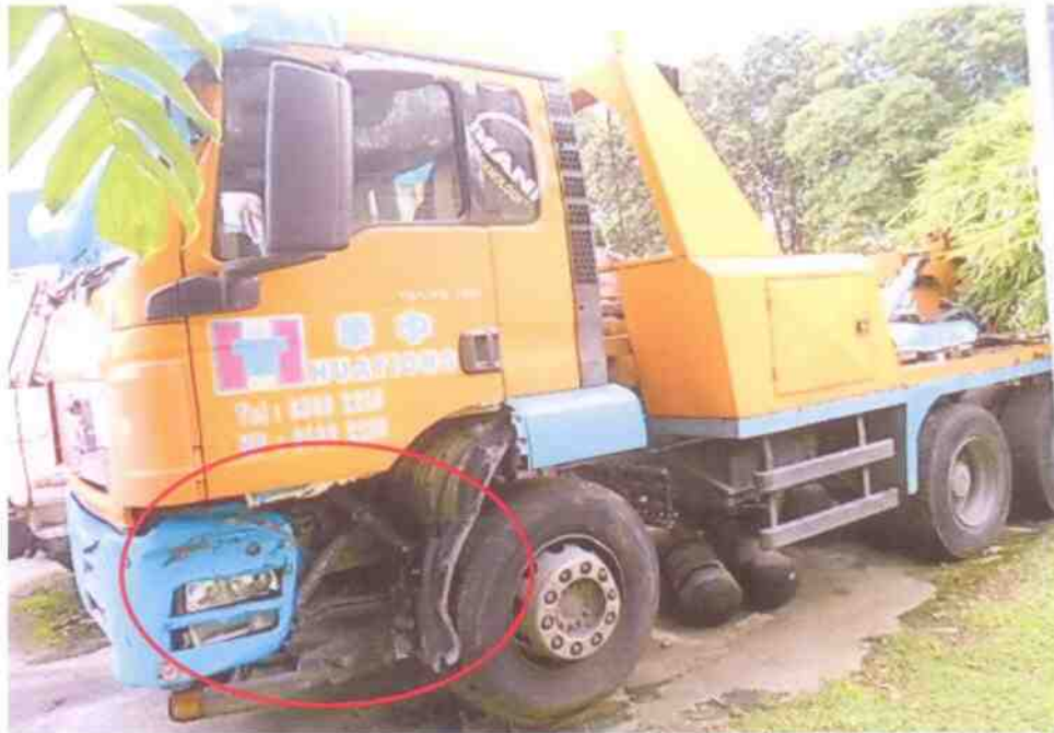
Photo 3 shows a general view of the front left body of the Tow Truck at the time of our inspection. Its front left lower bumper was observed to be buckled inwards pushing towards the rear of the Tow Truck. Its windshield was observed to be cracked. Its steering systems, breaking systems & transmission systems were amongst the affected components observed to be damaged due to the accident's collision impact.
