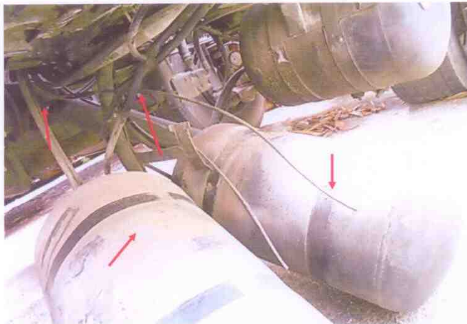
Photo 19 shows the hoses of the air pressure tanks, which are some of the components for the air-assisted braking system of the Tow Truck. These components were found to be cut & dislodged from the original installation. Hence, causing air leakage to the compressed air for the braking system.
