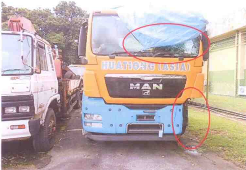
Photo 2 shows a general view of the front body of the Tow Truck at the time of our inspection. The Tow Truck was observed to have sustained damages at its left front body. Its front left lower bumper was observed to be buckled inwards pushing towards the rear of the Tow Truck. Its windshield was observed to be cracked. Its steering systems, breaking systems & transmission systems were amongst the affected components observed to be damaged due to the accident's collision impact.
