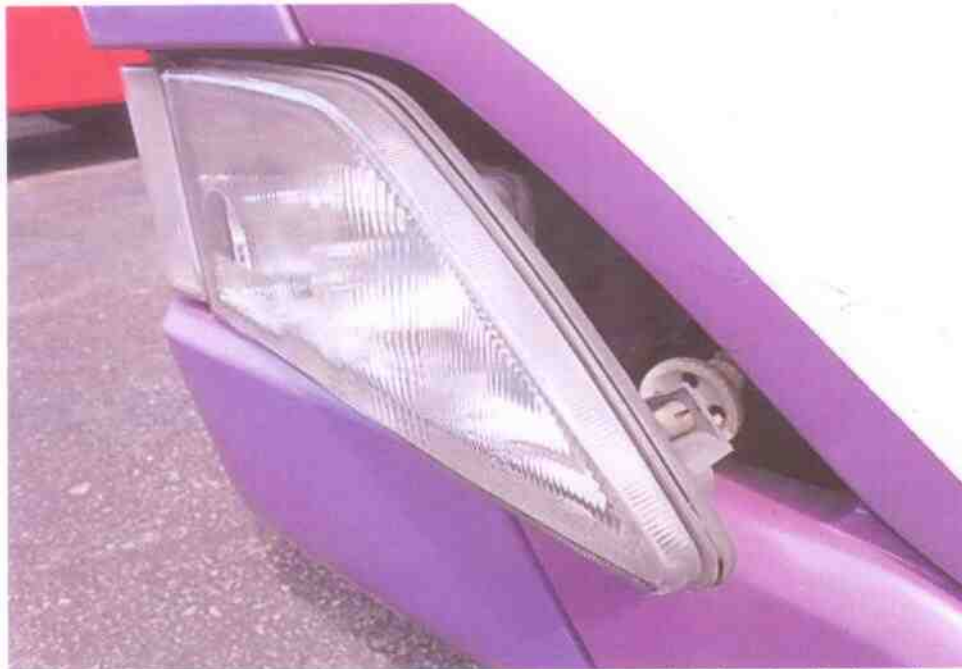
Photo 5 shows a close-up view of the Motor Bus's right hand side headlamp observed to be dislodged from its original installation likely due to the accident's impact.
