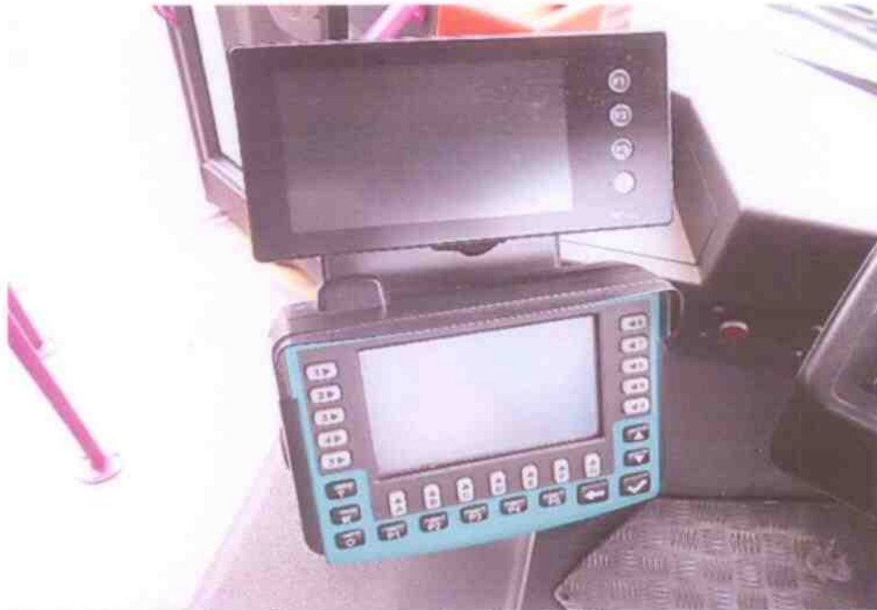
Photo 20 shows the indicators at the driver's seat. Other operational indicators were unable to be initialize due to the flat battery. Hence, no test was carried out to the Motor Bus additional devices.
