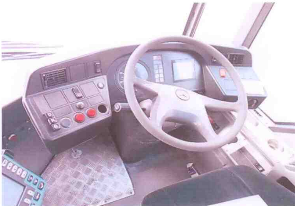
Photo 19 shows the indicators at the driver's seat. Other operational indicators were unable to be initialize due to the flat battery. Hence, no test was carried out to the Motor Bus additional devices.
