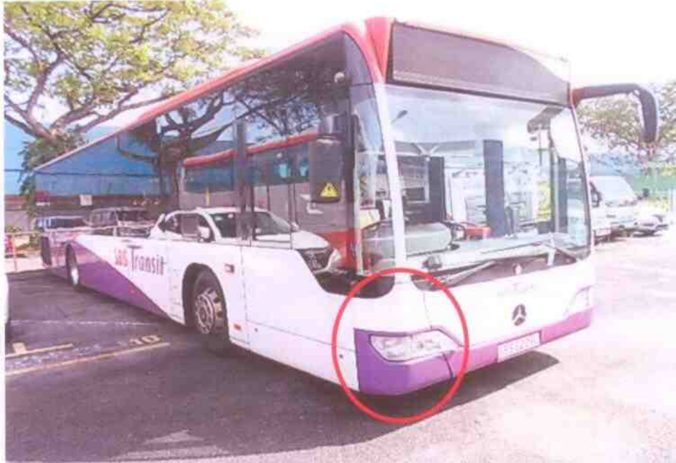
Photo 2 shows a general view of the front right body of the Motor Bus at the time of our inspection. The Motor Bus was observed to have sustained relatively minor damage at its front right body. Its front right lower bumper was observed to be cracked & misaligned; its front right headlamp was observed to be dislodged from the original installation.
