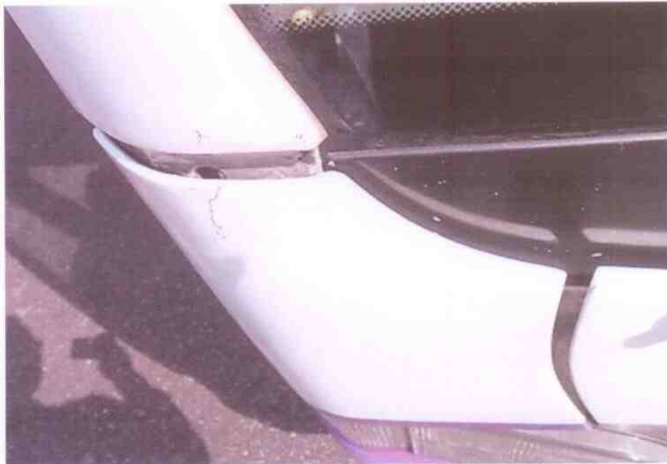
Photo 7 shows a close-up view of the Motor Bus's right hand side fender next to wiper garnish was observed to be misaligned likely due to the accident's impact.
