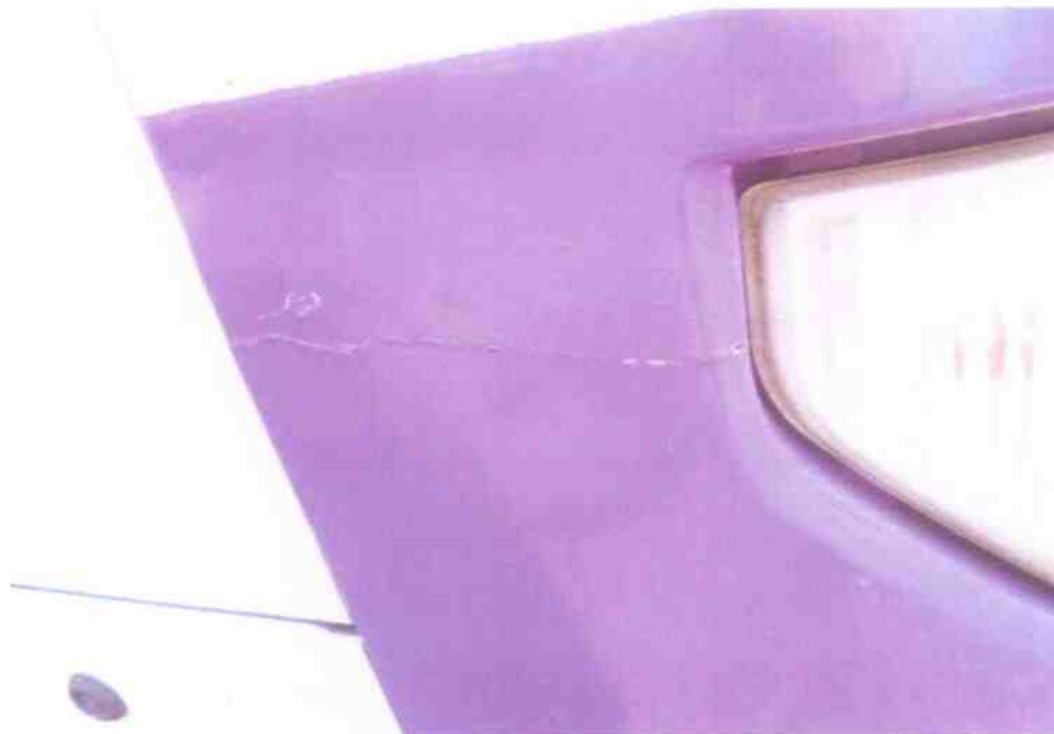
Photo 6 shows a close-up view of the Motor Bus's right hand lower bumper observed to be cracked likely due to the accident's impact.
