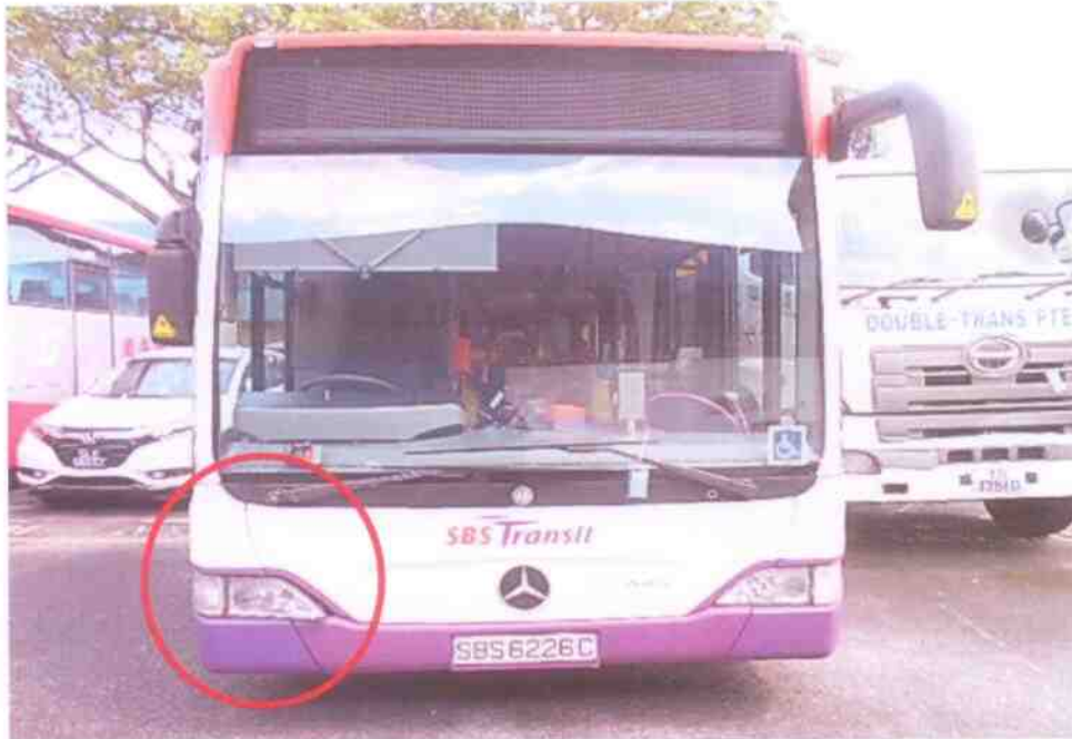
Photo 1 shows a general view of the front body of the Motor Bus at the time of our inspection. The Motor Bus was observed to have sustained relatively minor damage at its front right body. Its front right lower bumper was observed to be cracked & misaligned; its front right headlamp was observed to be dislodged from the original installation.
