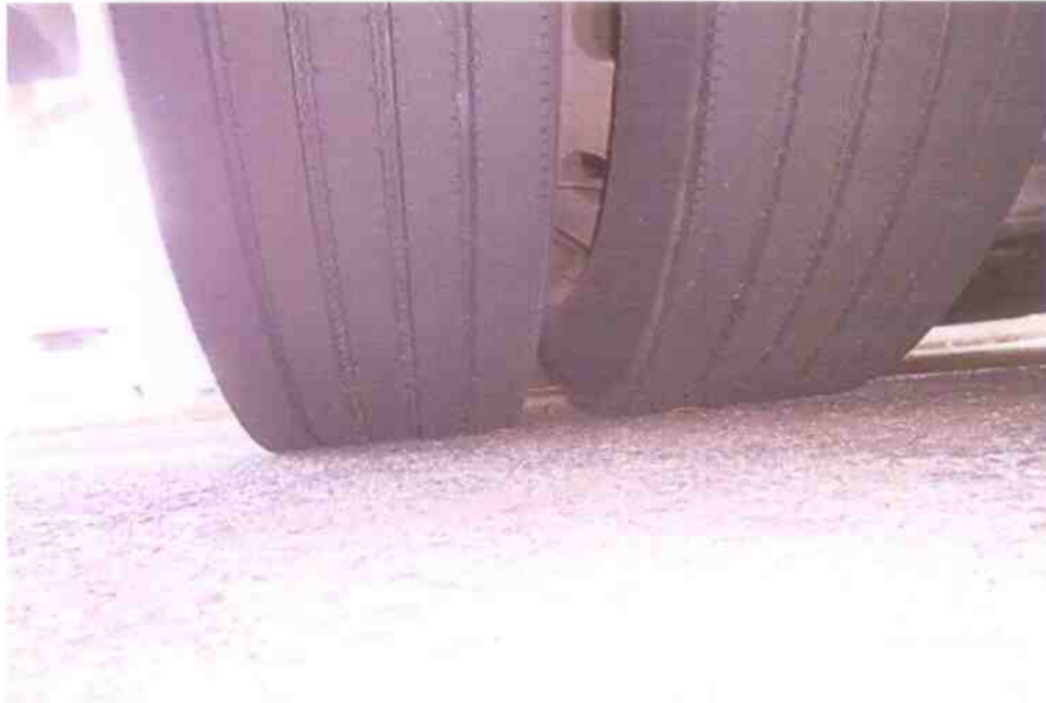
Photo 10 shows the condition of the rear right tyres of the Motor Bus, which were observed to be in serviceable condition with remaining tread depth of approximately 3mm. The tyres, which were wrapped around standard alloy wheels rims, were also observed to be sufficiently inflated for vehicular operation.
