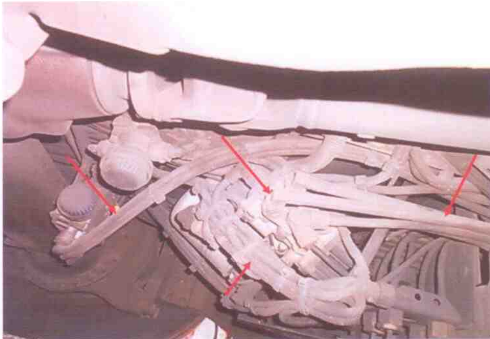
Photo 18 shows a general view of the air tank, valves, pipes and hoses, which are some of the components for the air-assisted braking system of the Motor Bus. This was at the underside of the Motor Bus's front right body. We were however not able to carry out any operational test(s) to the braking system of the Motor Bus as its engine was unable to be started.
