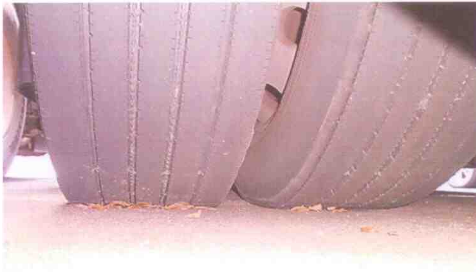
Photo 10 shows the condition of the rear right tyres of the Motor Bus, which were observed to be in serviceable condition with remaining tread depth of approximately 3mm. The tyres, which were wrapped around standard alloy wheels rims, were also observed to be sufficiently inflated for vehicular operation.
