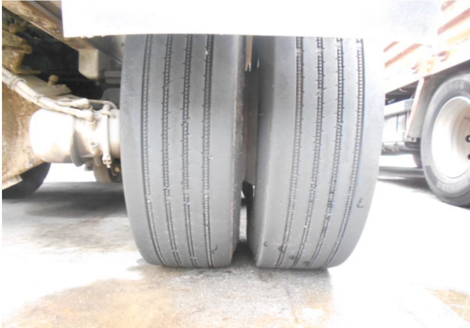
Photo 12 shows the condition of the rear right tyres of the Tipper Truck, which were observed to be in serviceable condition with remaining, tread depth of approximately 6mm. The tyres were also observed to be sufficiently inflated for vehicular operation with no tear, cut or burst mark(s) on the outer and the inner sidewalls.
