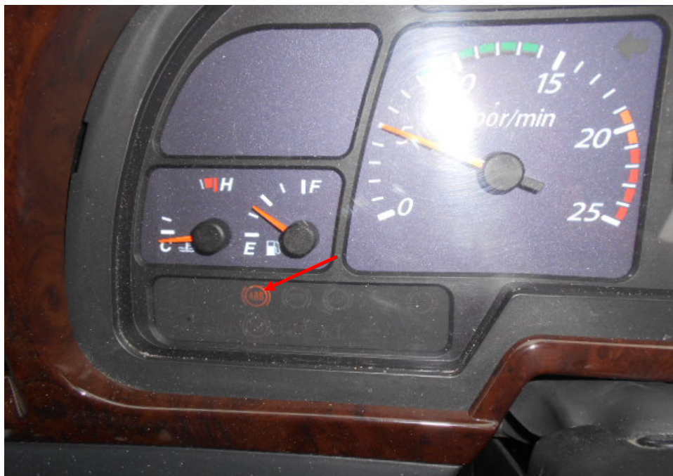
Photo 28 shows the warning indicator for Anti-Brake Lock System (ABS) was observed to be lighted up during cranking & after engine was in idling speed.
