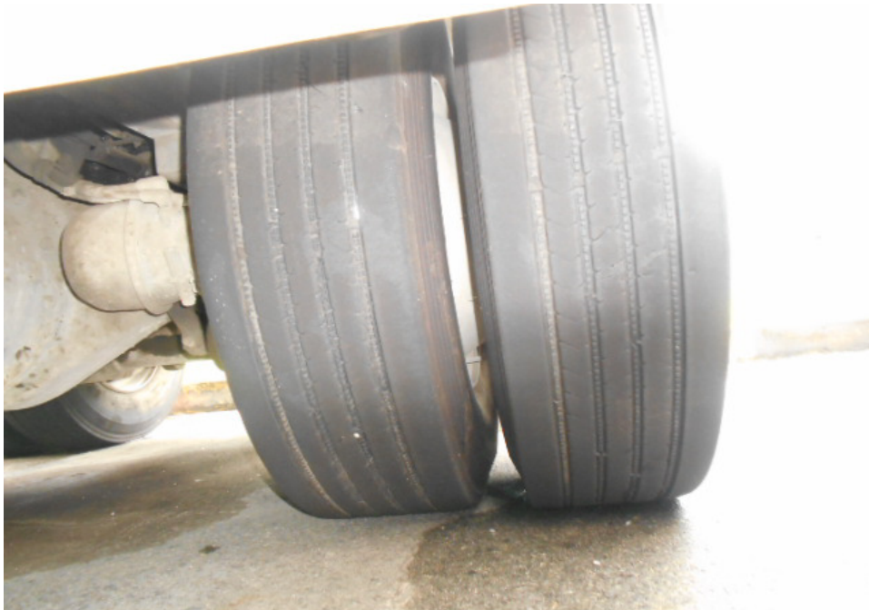
Photo 13 shows the condition of the rear right tyres (centre axle) of the Tipper Truck, which were observed to be in serviceable condition with remaining, tread depth of approximately 3mm. The tyres, which were wrapped around standard alloy wheel rims, were also observed to be sufficiently inflated for vehicular operation.
