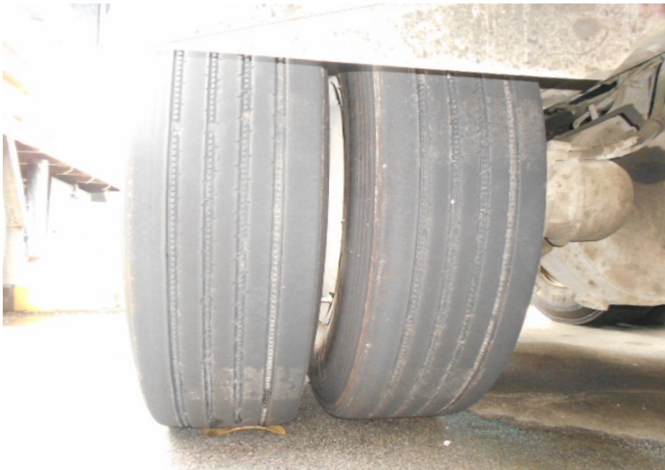
Photo 11 shows the condition of the rear left tyres (centre axle) of the Tipper Truck, which were observed to be in serviceable condition with remaining tread depth of approximately 6mm. The tyres were also observed to be sufficiently inflated for vehicular operation.
