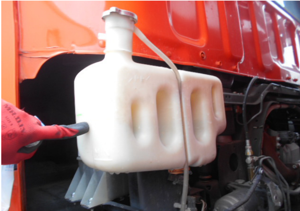
Photo 17 shows the engine coolant reservoir of the Tipper Truck at the time of our inspection. The engine coolant was observed to be of sufficient level and without any visible contamination for operational purposes.
