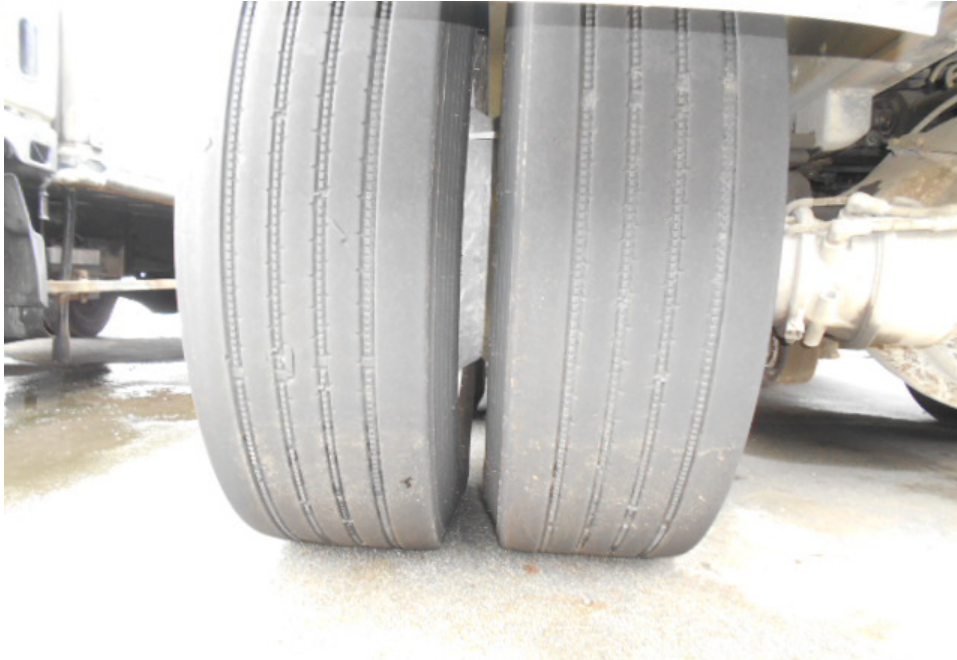
Photo 10 shows the condition of the rear left tyres of the Tipper Truck, which were observed to be in serviceable condition with remaining tread depth of approximately 6mm. The tyres were also observed to be sufficiently inflated for vehicular operation.
