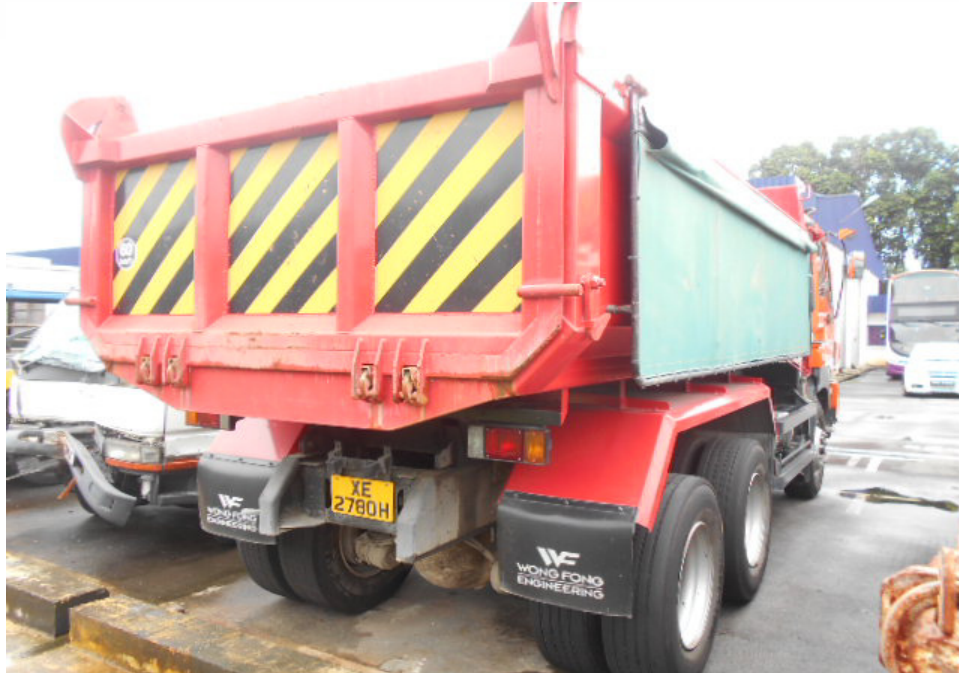
Photo 7 shows a general view of the rear right body of the Tipper Truck at the time of our inspection. The Tipper Truck was observed to have no signs of fresh damages on its body portion, this is likely due to the consistency of the accident's case fact that the Tipper Truck ran over the other involved party (bicycle).
