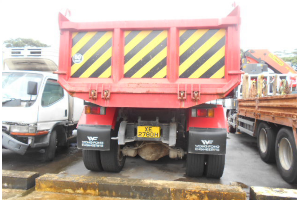
Photo 5 shows a general view of the rear body of the Tipper Truck at the time of our inspection. The Tipper Truck was observed to have no signs of fresh damages on its body portion, this is likely due to the consistency of the accident's case fact that the Tipper Truck ran over the other involved party (bicycle).
