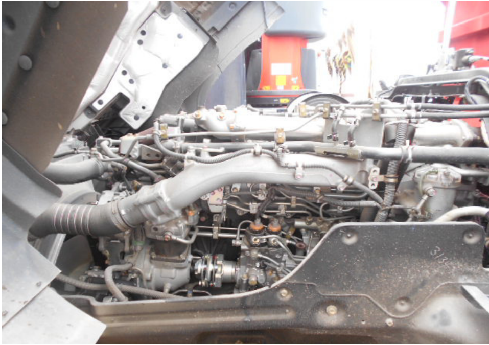
Photo 15 shows a general view of the engine area from under the front cabin of the Tipper Truck. The engine assembly and transmission assembly of the Tipper Truck were both observed to be intact and unaffected by the collision. There was also no sign(s) or indication(s) of fluid leak and/or fluid stain found.
