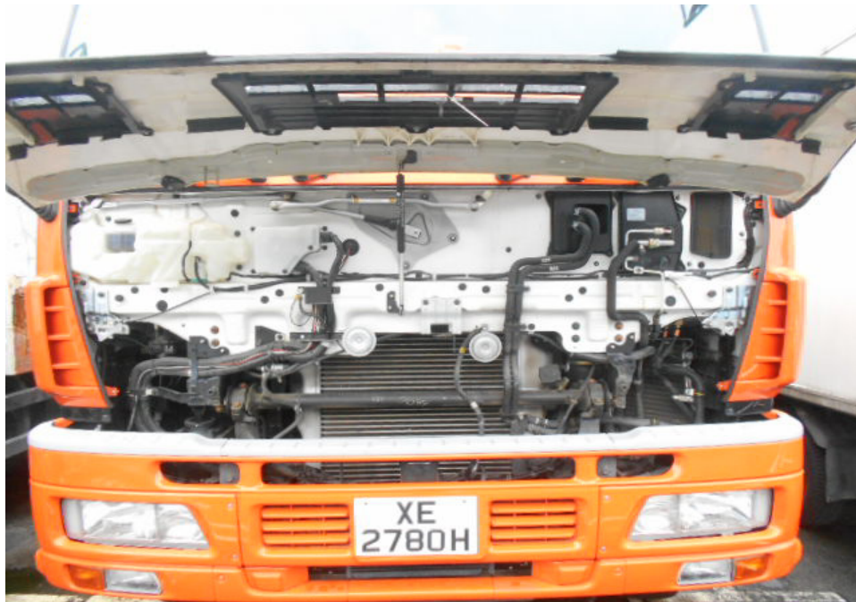
Photo 14 shows a general view of the engine compartment area from the front bonnet of the Tipper Truck. It was observed to be intact and unaffected by the collision. There was also no sign(s) or indication(s) of fluid leak and/or fluid stain found.
