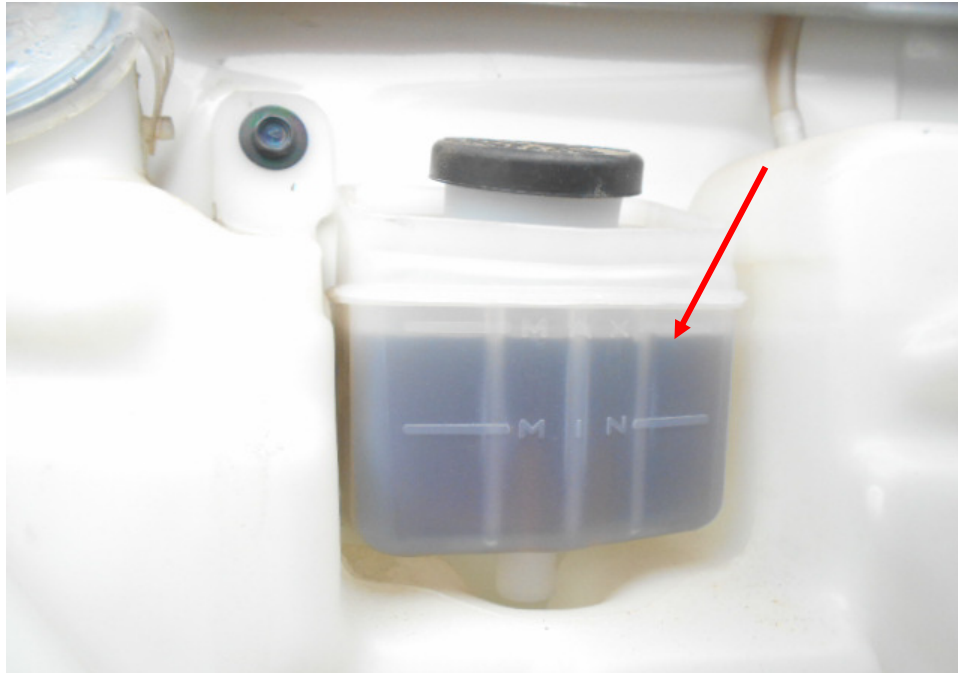
Photo 24 shows the brake fluid at the front bonnet of the Tipper Truck. The brake fluid was found to be of sufficient level for operating purposes. Visually, there was also no contamination found to these fluids.
