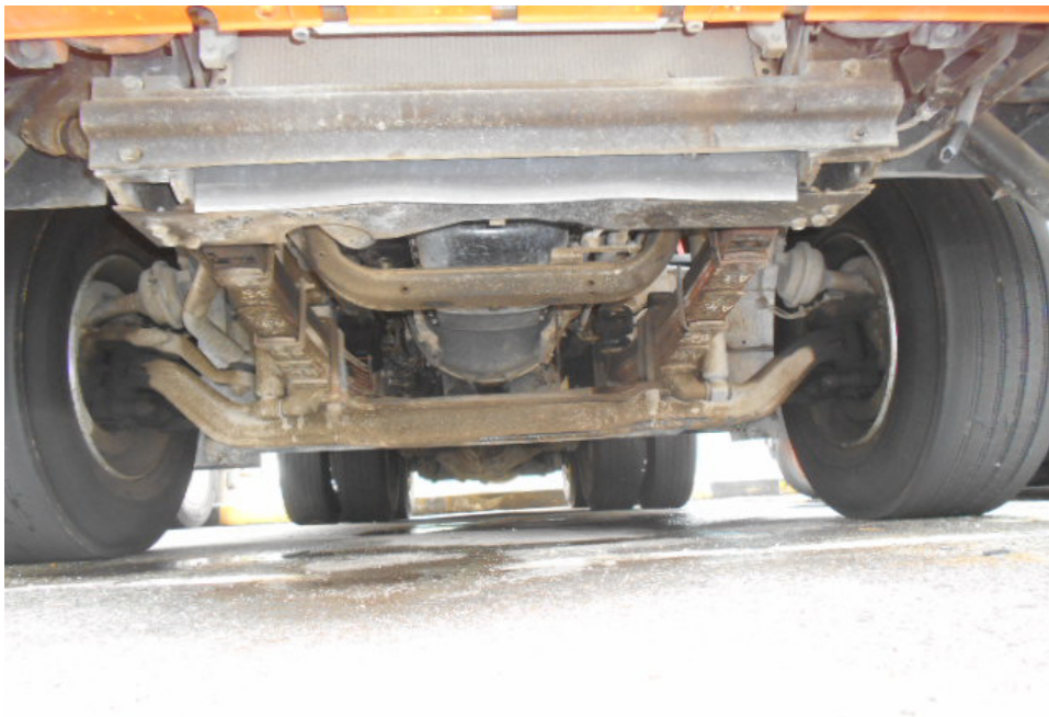
Photo 16 shows a general view of the engine area from the underside of the Tipper Truck. The engine assembly and transmission assembly of the Tipper Truck were both observed to be intact and unaffected by the collision. There was also no sign(s) or indication(s) of fluid leak and/or fluid stain found.
