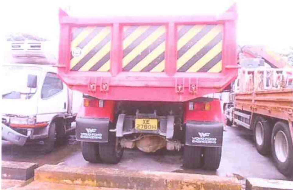
Photo 5 shows a general view of the rear body of the Tipper Truck at the time of our inspection. The Tipper Truck was observed to have no signs of fresh damages on its body portion, this is likely due to the consistency of the accident's case fact that the Tipper Truck ran over the other involved party (bicycle).
