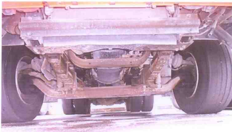
Photo 15 shows a general view of the engine area from under the front cabin of the Tipper Truck. The engine assembly and transmission assembly of the Tipper Truck were both observed to be intact and unaffected by the collision. There was also no sign(s) or indication(s) of fluid leak and/or fluid stain found.
