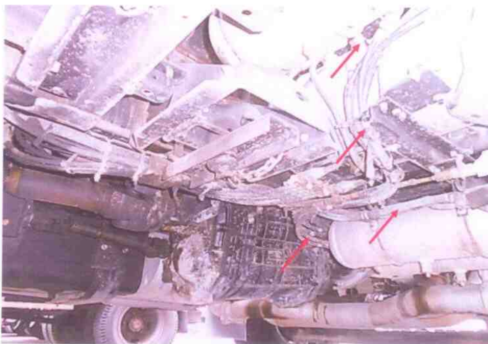
Photo 21 shows the valves, brake hoses and pipes, which are some of the components for the air-assisted braking system of the Tipper Truck. These components were mainly located around the right centre body of the Tipper Truck, and were unaffected by the accident. Our visual examination of these parts revealed all to be in good general condition and securely fitted.
