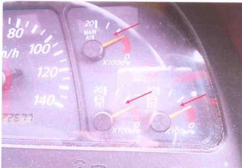
Photo 27 shows the compressed air meters for braking system. This shows that there's no dropped of pressure. Hence, revealed that no air leakage at the time of our inspection.
