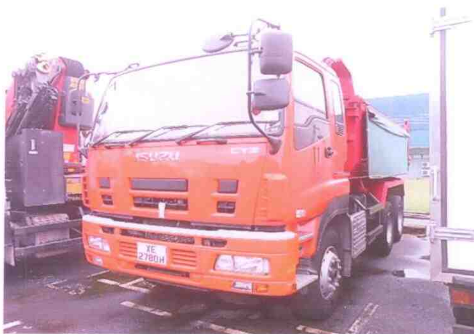
Photo 4 shows a general view of the front left body of the Tipper Truck at the time of our inspection. The Tipper Truck was observed to have no signs of fresh damages on its body portion, this is likely due to the consistency of the accident's case fact that the Tipper Truck ran over the other involved party (bicycle).
