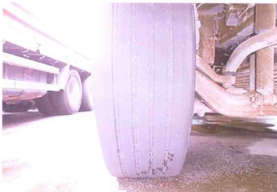
Photo 9 shows the condition of the front right tyre of the Tipper Truck, which was observed to be in serviceable condition with remaining tread depth of approximately 6mm.
