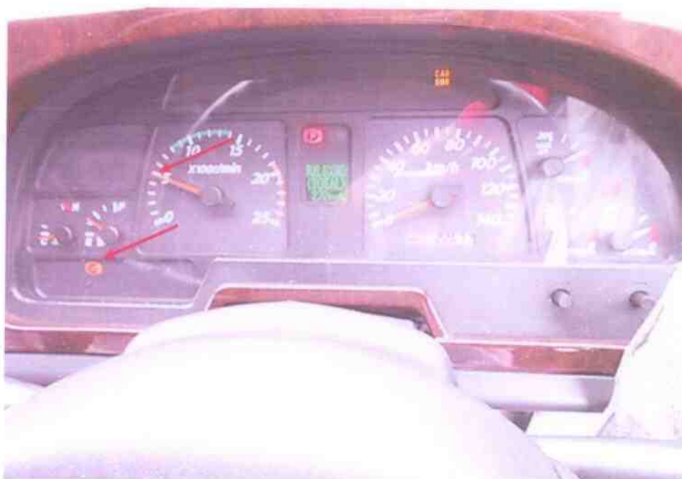
Photo 26 shows the warning indicator for Anti-Brake Lock System (ABS) was observed to be lighted up during cranking & after engine was in idling speed.
