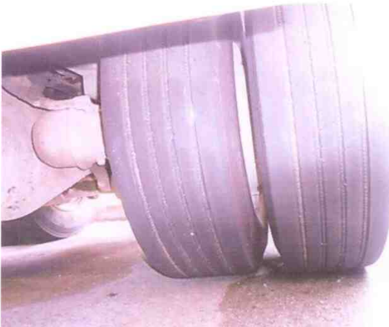
Photo 13 shows the condition of the rear right tyres (centre axle) of the Tipper Truck, which were observed to be in serviceable condition with remaining, tread depth of approximately 3mm. The tyres, which were wrapped around standard alloy wheel rims, were also observed to be sufficiently inflated for vehicular operation.
