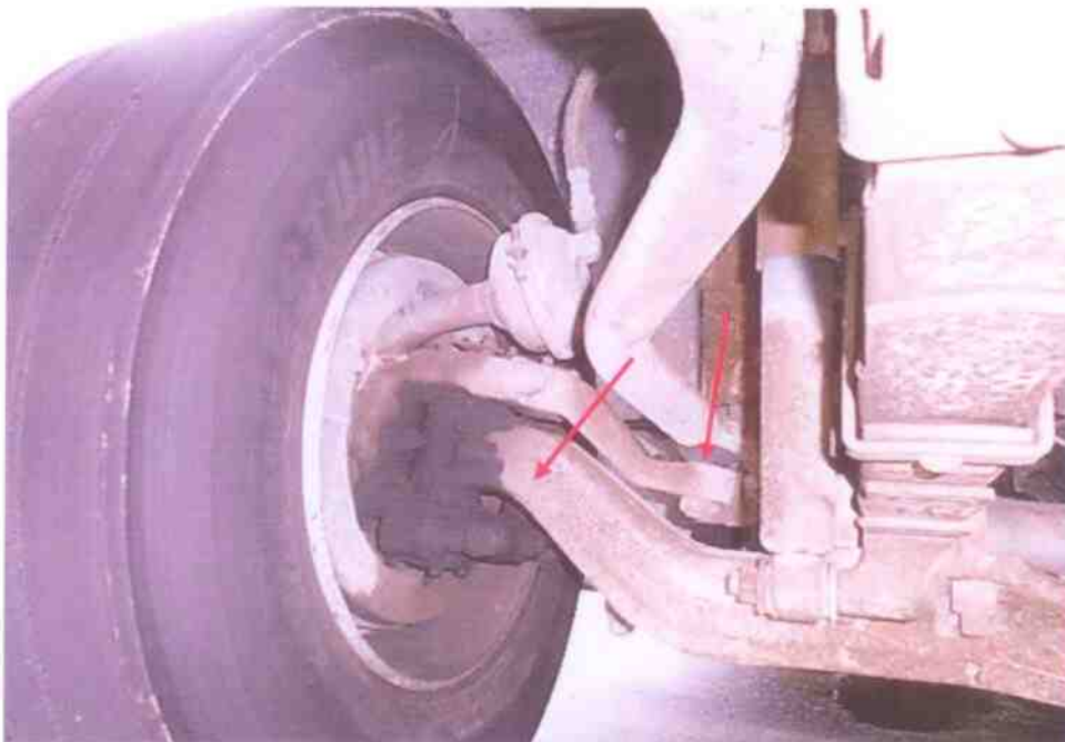
Photo 19 shows the undercarriage components at the front right wheel of the Tipper Truck. The various undercarriage components of the Tipper Truck were all observed to be intact and without any visible damage. This had included the steering rack and steering linkages (arrowed) of the Tipper Truck.
