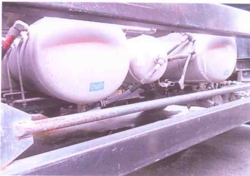
Photo 20 shows the air tanks, valves, pipes and hoses, which are some of the components for the air-assisted braking system of the Tipper Truck. These components were mainly located around the right centre body of the Tipper Truck, and were unaffected by the accident.
