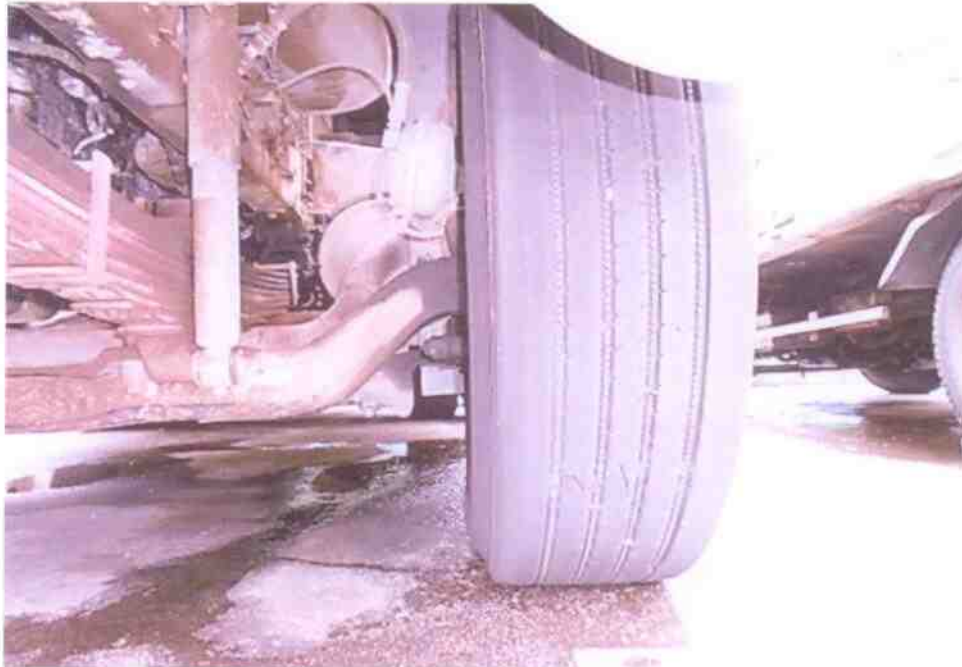
Photo 8 shows the condition of the front left tyre of the Tipper Truck, which was observed to be in serviceable condition with remaining tread depth of approximately 3mm.
