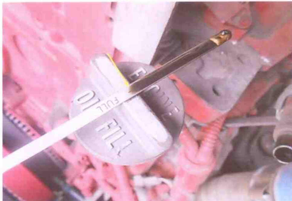
Photo 16 shows the engine fluid of the Motor Bus. It was observed to be of sufficient level (Yellow) without any contamination at time of our inspection.
