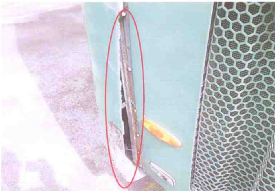
Photo 10 shows a close-up view of the Motor Bus's rear body at the time of our inspection. Its rear right lower bumper was observed to be misaligned & cracked likely due to the accident's collision impact.
