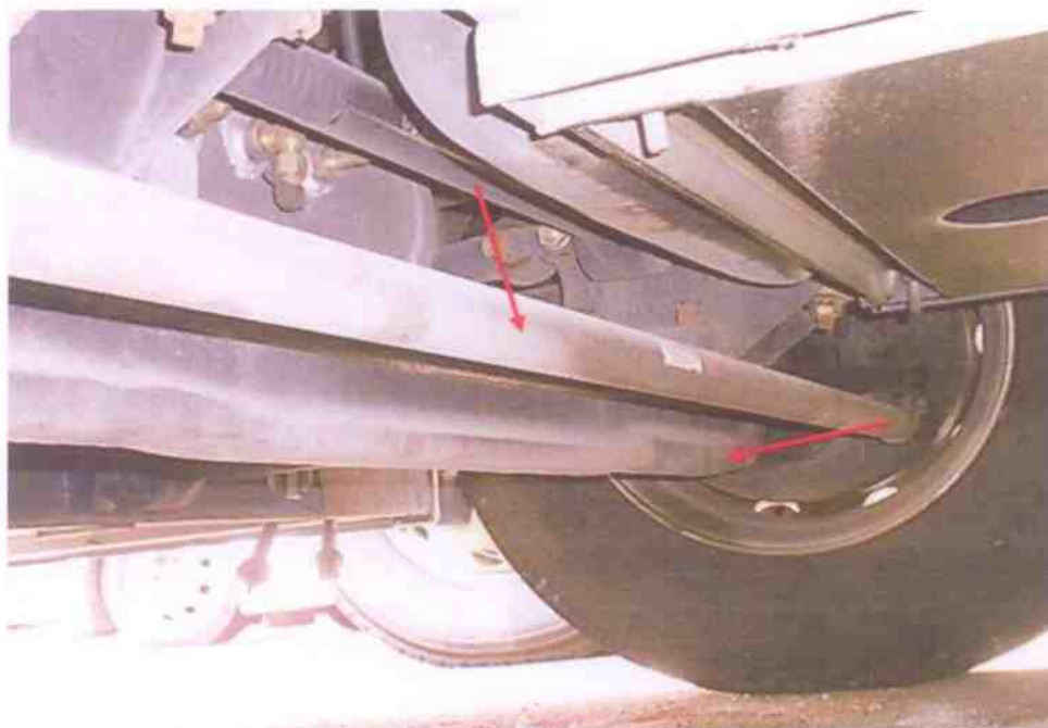
Photo 20 shows the undercarriage components at the front right wheel of the Motor Bus. The various undercarriage components of the Motor Bus were all observed to be intact and without any visible damage. This had included the steering rack and steering ball joints (arrowed) of the Motor Bus.
