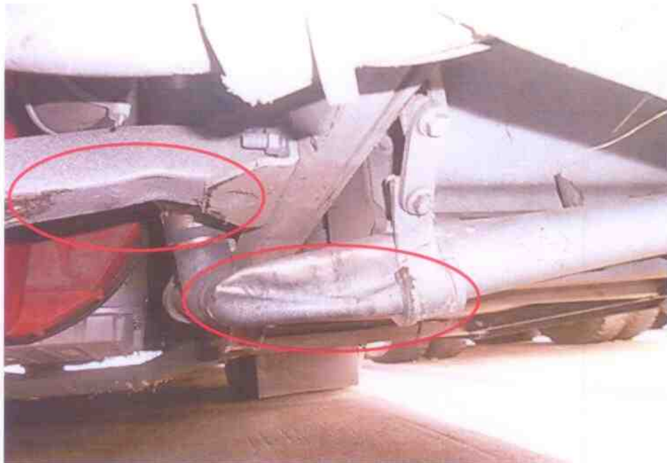
Photo 9 shows a close-up view of the Motor Bus's rear body at the time of our inspection. Its rear right reinforcement bar & steel pipe was observed to be scratched & dented likely due to the accident's collision impact.
