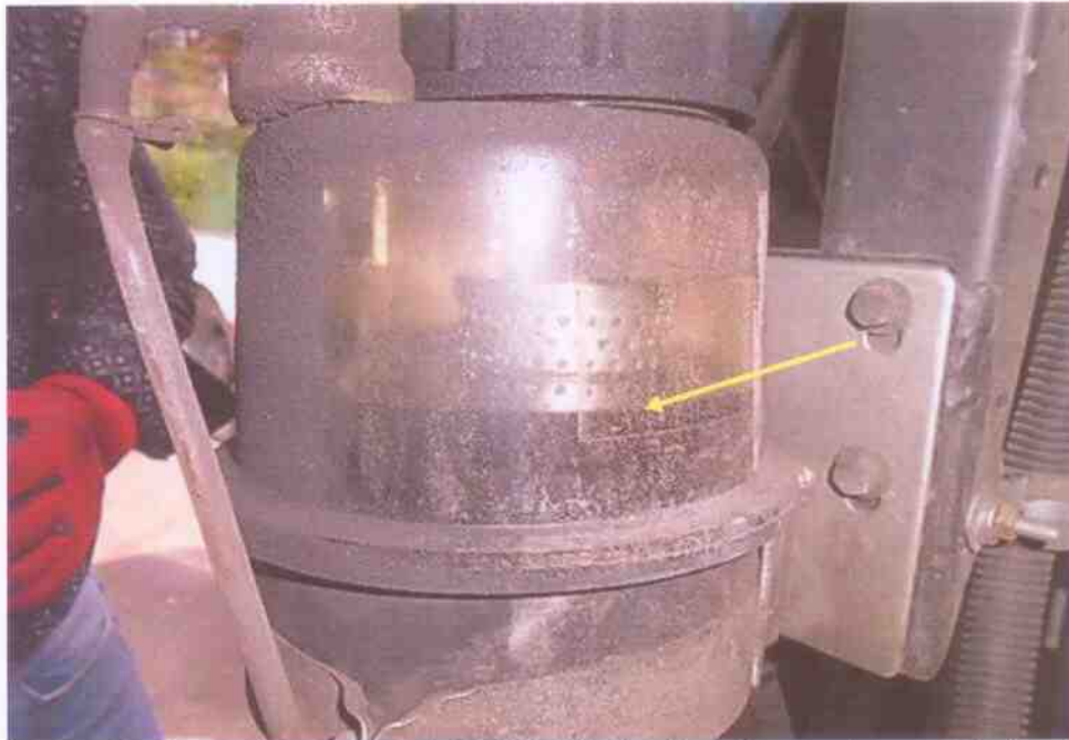
Photo 17 shows the steering fluid of the Motor Bus. It was observed to be of sufficient level (Yellow) without any contamination at time of our inspection.
