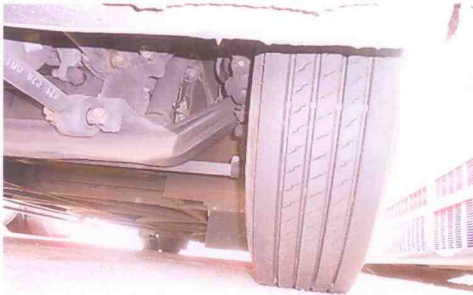
Photo 12 shows the condition of the front left tyre of the Motor Bus, which was observed to be in serviceable condition with remaining tread depth of approximately 6mm. The tyre was also observed to be sufficiently inflated for vehicular operation.
