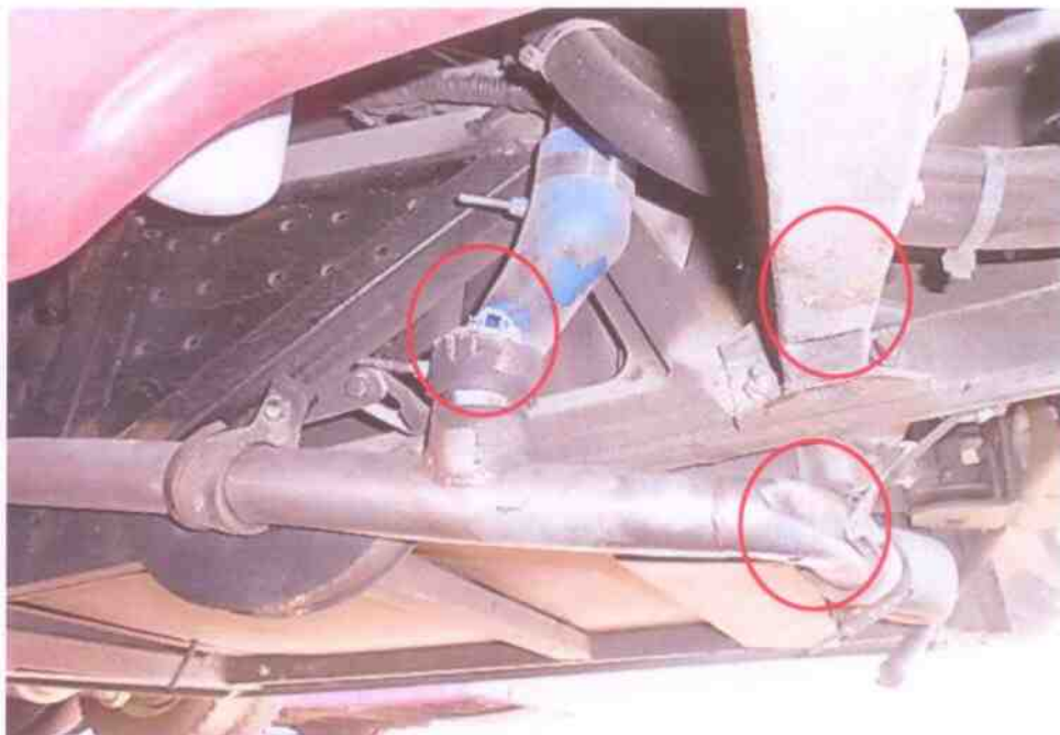
Photo 8 shows a close-up view of the Motor Bus's rear body at the time of our inspection. Its rear right reinforcement bar, hose & steel pipe was observed to be scratched, cut & dented likely due to the accident's collision impact.
