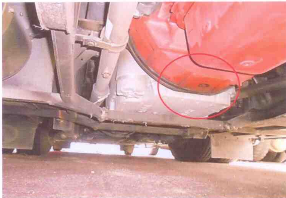
Photo 18 shows the engine underside of the Motor Bus. Our subsequent checks on the underside of the Motor Bus reveals some fluid stain sighted under the engine compartment. Further investigation found that the fluid stain was a pre-existed prior the accident & not a fresh fluid. This was due to some dirt observed on the fluid stain. Conclusively, it is not likely to be related to the accident. Visually, the various undercarriage components of the Motor Bus were observed to be intact and without any visible damage except for the damages caused by the accident.
