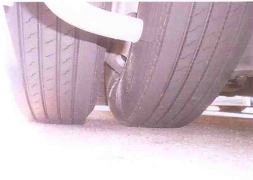
Photo 12 shows the condition of the front left tyre of the Motor Bus, which was observed to be in serviceable condition with remaining tread depth of approximately 6mm. The tyre was also observed to be sufficiently inflated for vehicular operation.
