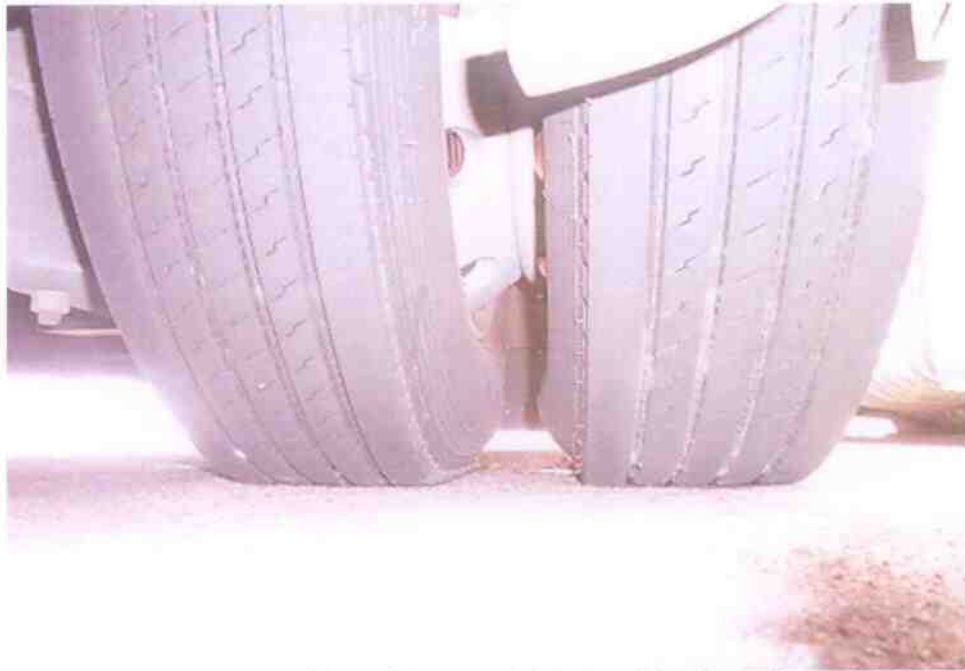
Photo 14 shows the condition of the rear left tyres of the Motor Bus, which were observed to be in serviceable condition with remaining tread depth of approximately 6mm. The tyres, which were wrapped around standard alloy wheel rims, were also observed to be sufficiently inflated for vehicular operation.
