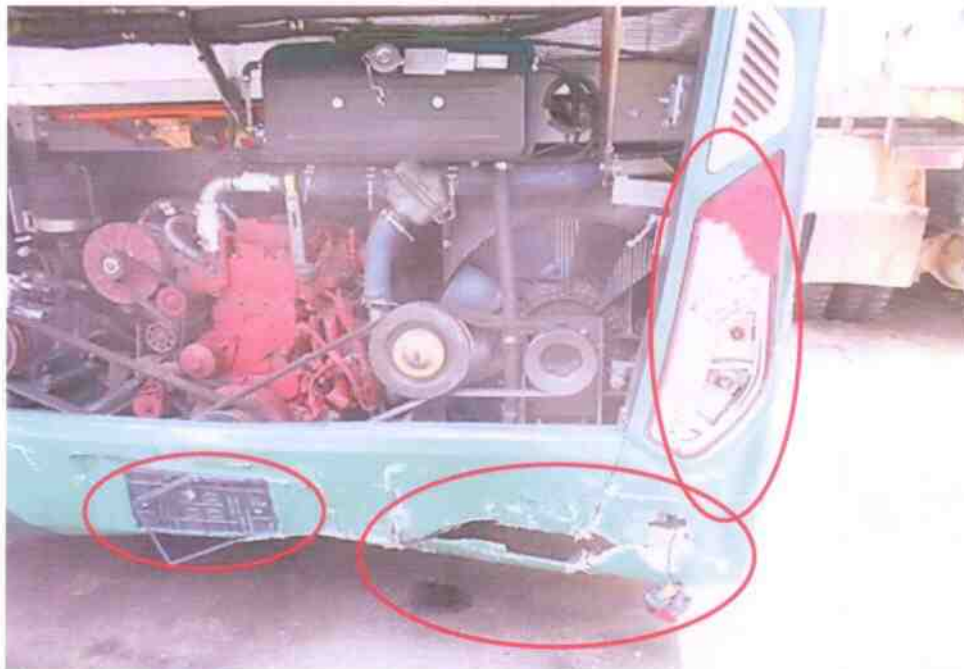
Photo 5 shows a semi close-up view of the Motor Bus's rear body at the time of our inspection. The Motor Bus was observed to have sustained relatively minor impact damage at its rear body portion due to the accident's impact.
