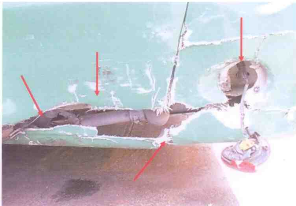
Photo 6 shows a close-up view of the Motor Bus's rear body at the time of our inspection. The Motor Bus rear lower bumper was observed to be cracked & the spot light was dislodged from its bracket.
