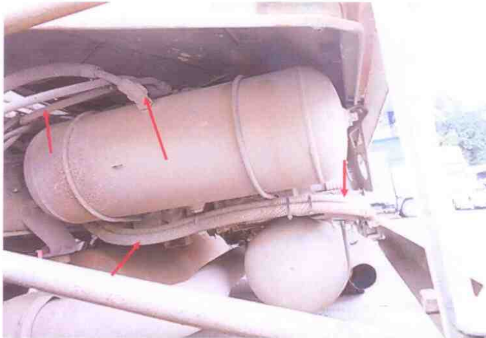
Photo 22 shows the valves, brake hoses and pipes, which are some of the components for the air-assisted braking system of the Garbage Truck. These components were mainly located around the right centre body of the Garbage Truck, and were unaffected by the accident. Our visual examination of these parts revealed all to be in good general condition and securely fitted.
