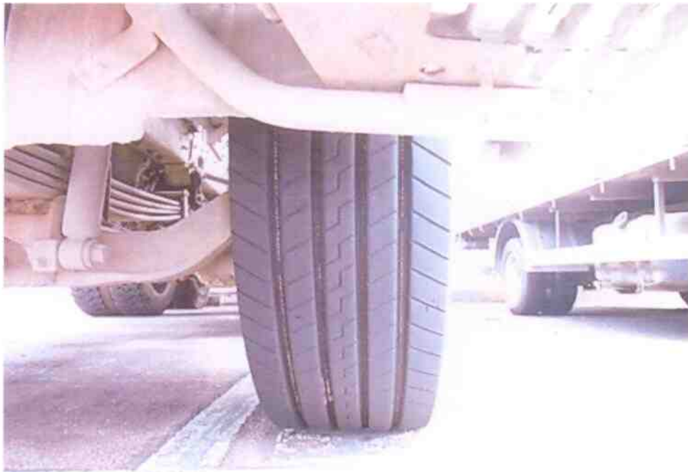
Photo 7 shows the condition of the front left tyre of the Garbage Truck, which was observed to be in serviceable condition with remaining tread depth of approximately 8mm.
