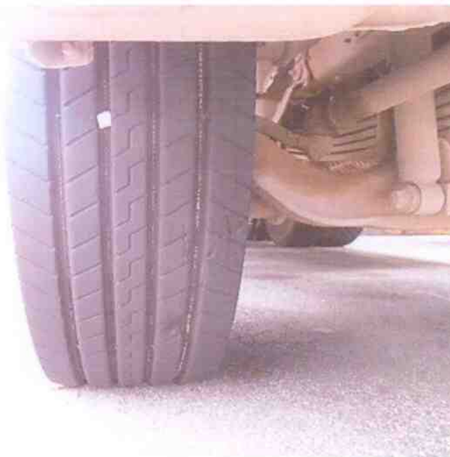
Photo 8 shows the condition of the front right tyre of the Garbage Truck, which was observed to be in serviceable condition with remaining tread depth of approximately 10mm.
