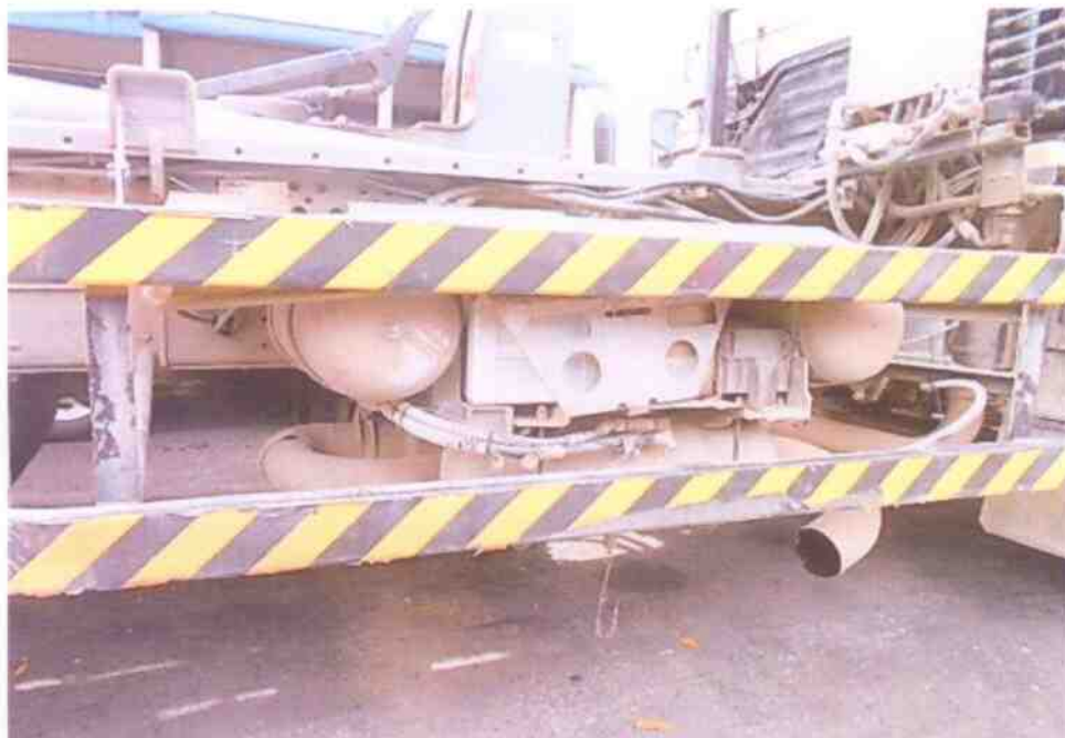
Photo 21 shows the air tanks, valves, pipes and hoses, which are some of the components for the air-assisted braking system of the Garbage Truck.
