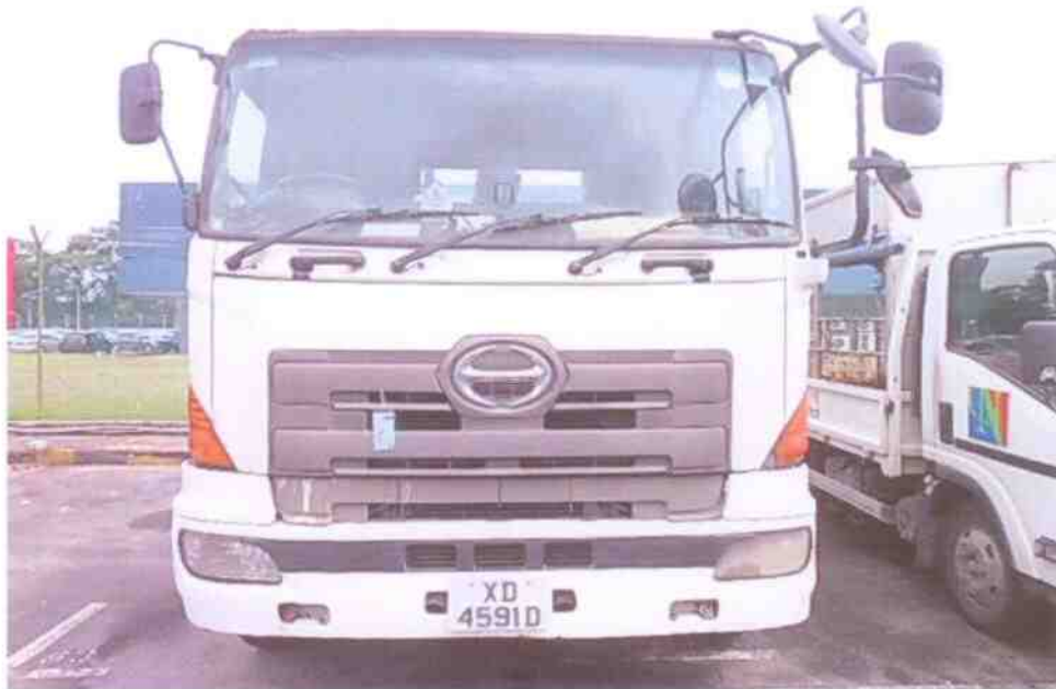
Photo 1 shows a general view of the front body of the Garbage Truck at the time of our inspection. The Garbage Truck was observed to have no signs of fresh damages on its body portion.
