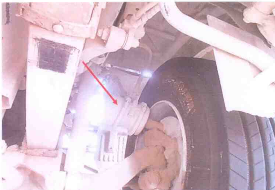
Photo 24 shows the brake air cylinder (arrowed) at the front left rear wheel of the Garbage Truck. Such air cylinder, which is amongst the various components for the air-assisted hydraulic braking system, can be found attached to all the front wheels and all the wheels of the Garbage Truck. Upon our checks, we had found all the brake air cylinders to be undamaged and securely fitted to all the wheels of the Garbage Truck.
