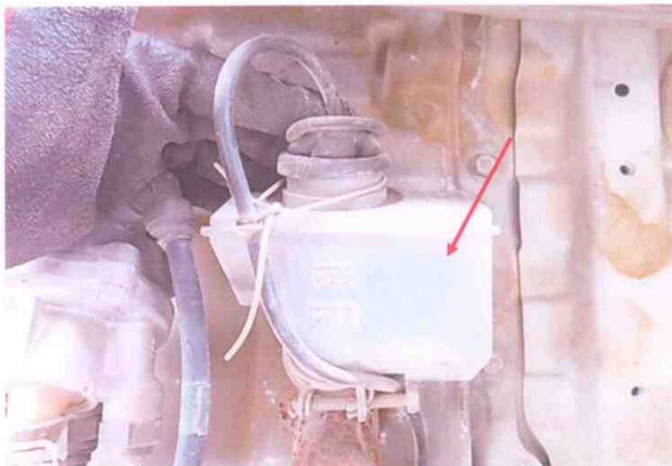
Photo 25 shows the brake fluid at the front bonnet of the Garbage Truck. The brake fluid was found to be of sufficient level for operating purposes. Visually, there was also no contamination found to these fluids.
