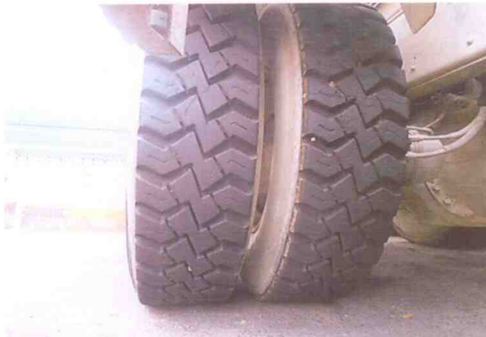
Photo 12 shows the condition of the rear right tyres (centre axle) of the Garbage Truck, which were observed to be in serviceable condition with remaining, tread depth of approximately 14mm. The tyres, which were wrapped around standard alloy wheel rims, were also observed to be sufficiently inflated for vehicular operation.
