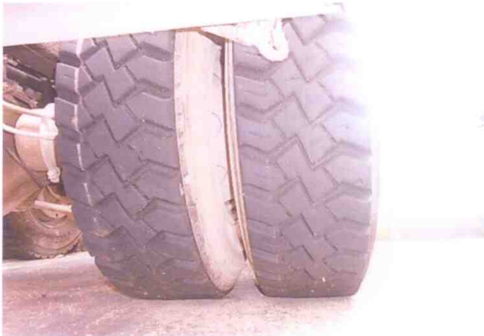
Photo 9 shows the condition of the rear left tyres (centre axle) of the Garbage Truck, which were observed to be in serviceable condition with remaining tread depth of approximately 8mm. The tyres were also observed to be sufficiently inflated for vehicular operation.
