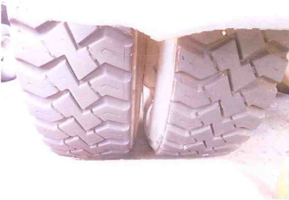
Photo 10 shows the condition of the rear left tyres of the Garbage Truck, which were observed to be in serviceable condition with remaining tread depth of approximately 13mm. The tyres were also observed to be sufficiently inflated for vehicular operation.
