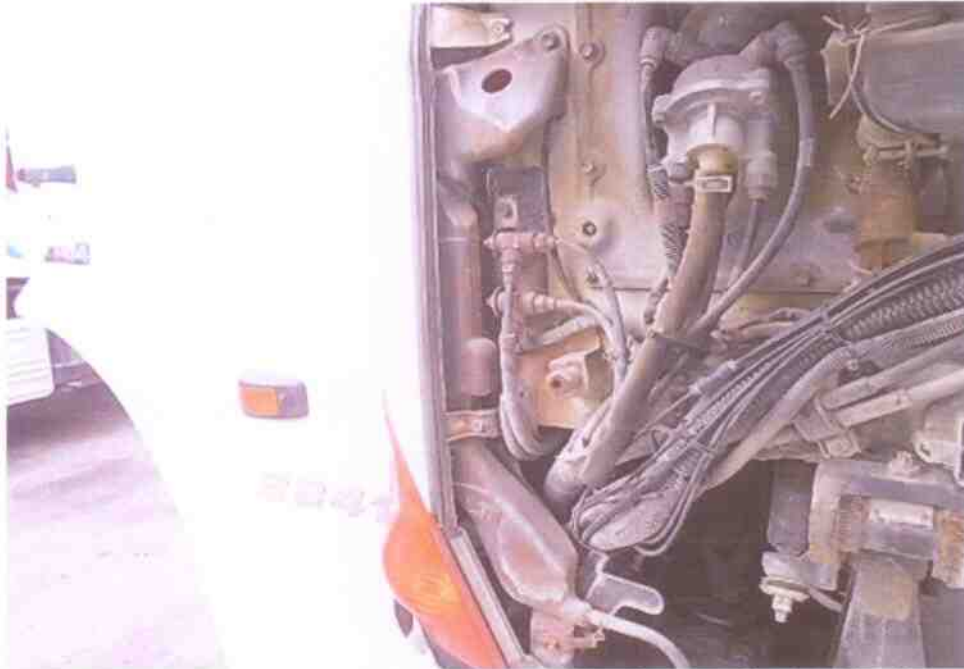
Photo 16 shows the engine coolant reservoir of the Garbage Truck at the time of our inspection. The engine coolant was observed to be of sufficient level and without any visible contamination for operational purposes.
