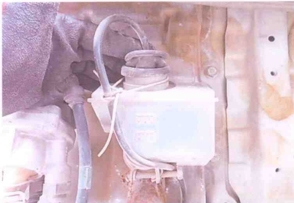
Photo 17 shows the brake fluid reservoir of the Garbage Truck at the time of our inspection. It was observed to be of sufficient level and without any visible contamination for operational purposes.
