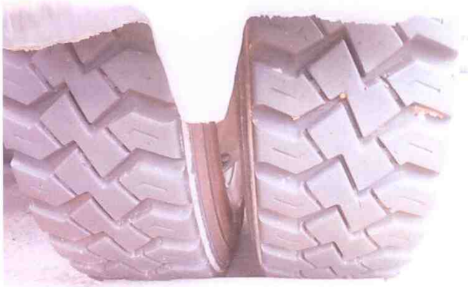
Photo 11 shows the condition of the rear right tyres of the Garbage Truck, which were observed to be in serviceable condition with remaining, tread depth of approximately 13mm. The tyres were also observed to be sufficiently inflated for vehicular operation with no tear, cut or burst mark(s) on the outer and the inner sidewalls.
