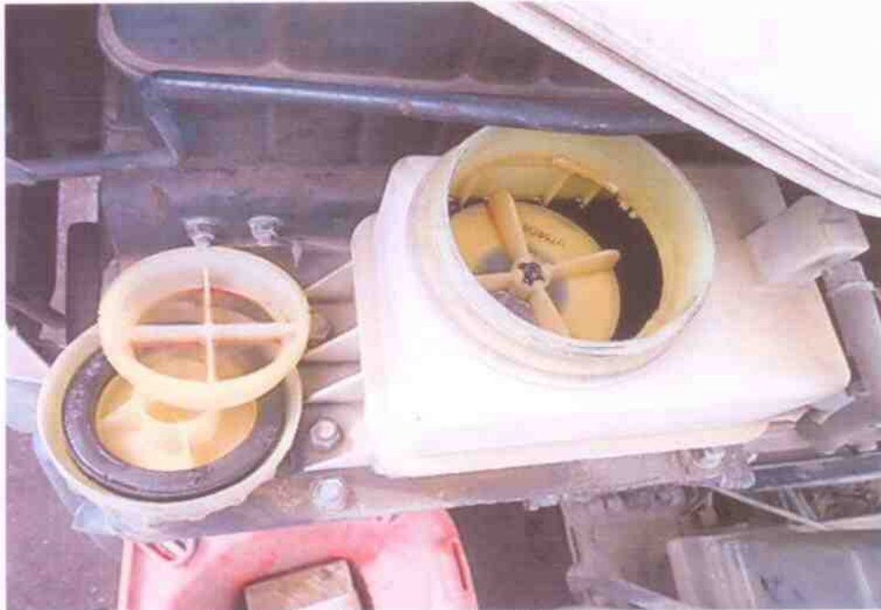
Photo 18 shows the steering fluid reservoir of the Garbage Truck at the time of our inspection. It was observed to be of sufficient level and without any visible contamination for operational purposes.
