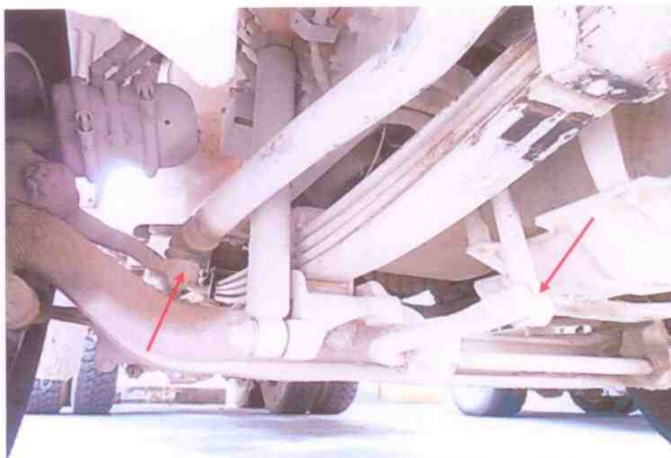
Photo 19 shows the undercarriage components at the front right wheel of the Garbage Truck. The various undercarriage components of the Garbage Truck were all observed to be intact and without any visible damage. This had included the steering rack and steering linkages (arrowed) of the Garbage Truck.
