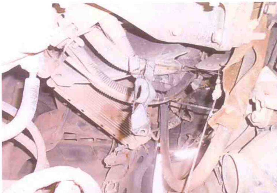
Photo 14 shows a general view of the engine area from the underside of the Tipper Truck. The engine assembly and transmission assembly were both observed to be intact and unaffected by the collision. There was also no sign(s) or indication(s) of fresh fluid leak and/or fluid stain found.
