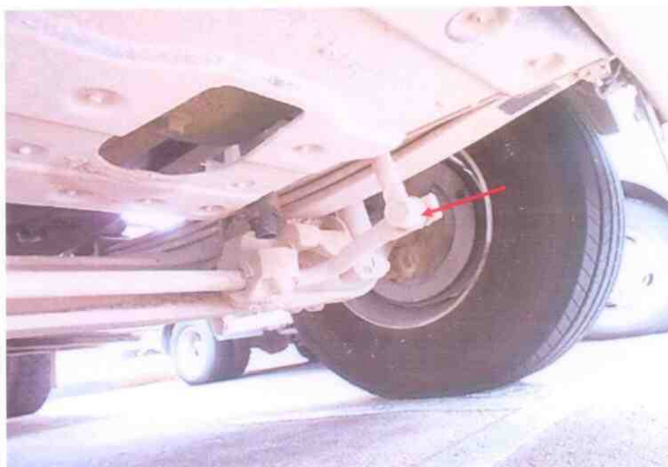
Photo 20 shows the undercarriage components at the front left wheel of the Garbage Truck. The various undercarriage components of the Garbage Truck were all observed to be intact and without any visible damage. This had included the steering rack (arrowed) of the Garbage Truck, which was observed to be securely attached to the front left wheel.
