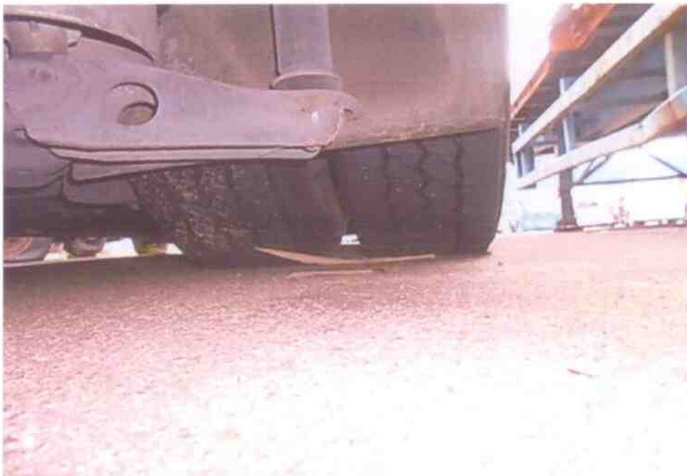
Photo 7 shows the condition of the rear right tyres of the Motor Bus, which were observed to be in serviceable condition with remaining tread depth of approximately 11mm. The tyres, which were wrapped around standard alloy wheels rims, were also observed to be sufficiently inflated for vehicular operation.
