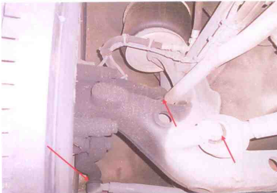
Photo 12 shows some of the mechanical components (arrowed) of the Motor Bus's steering system. Our visual checks on the various mechanical components of the steering system revealed all to be intact and in good condition. The steering system of the Motor Bus is hence likely to be in serviceable condition at the time of accident.
