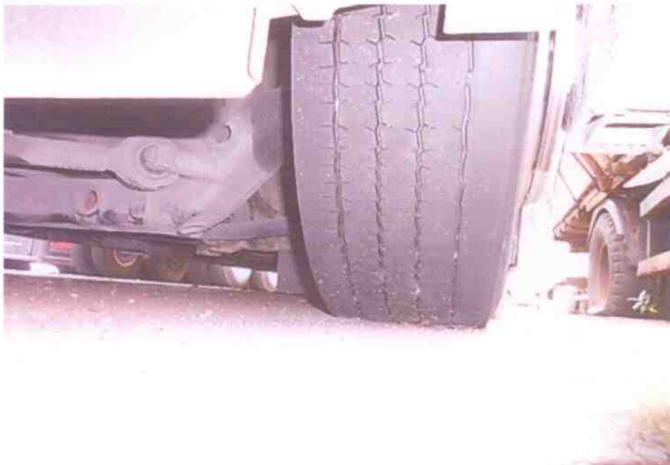
Photo 6 shows the condition of the front left tyre of the Motor Bus, which was observed to be in serviceable condition with remaining tread depth of approximately 9mm. The tyre was also observed to be sufficiently inflated for vehicular operation.
