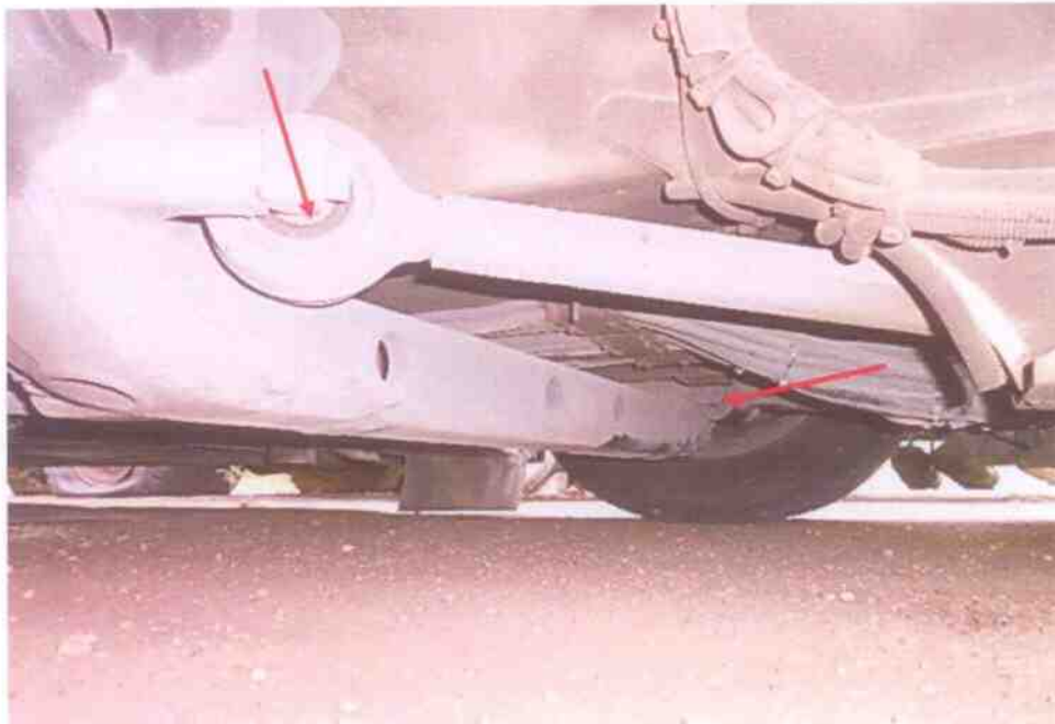
Photo 13 shows the undercarriage components at the front right wheel of the Motor Bus. The various undercarriage components of the Motor Bus were all observed to be intact and without any visible damage. This had included the steering rack and steering ball joints (arrowed) of the Motor Bus.
