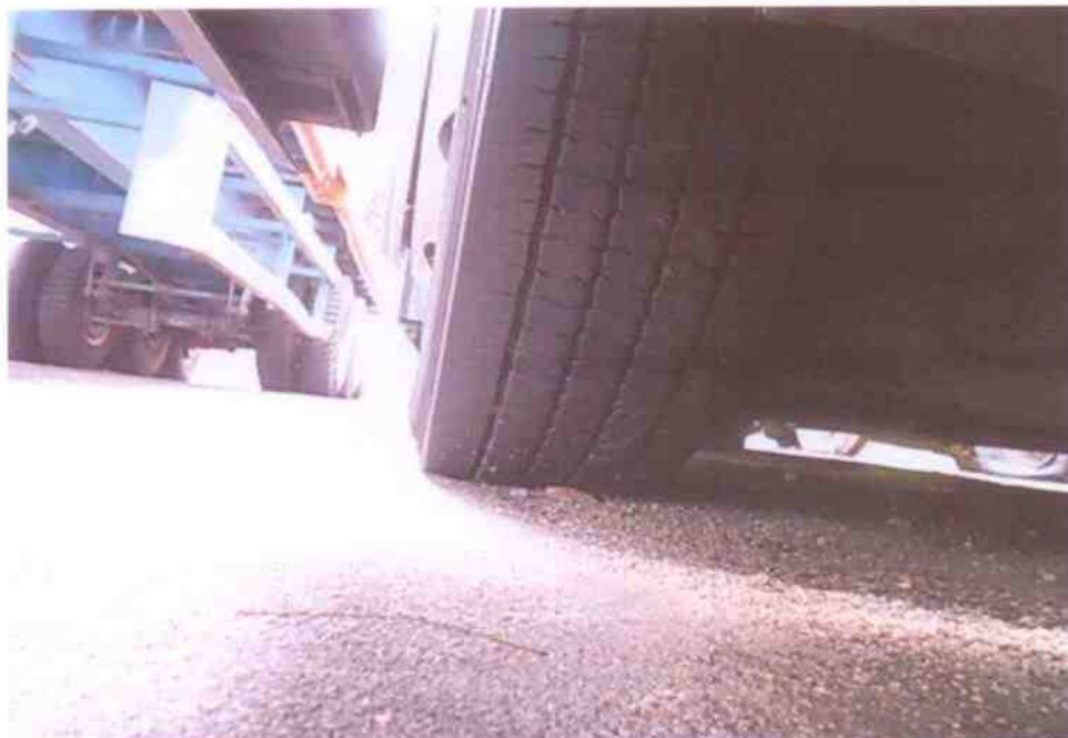
Photo 5 shows the condition of the front right tyre of the Motor Bus, which was with remaining tread depth of approximately 12mm. The tyre was also observed to be sufficiently inflated for vehicular operation.
