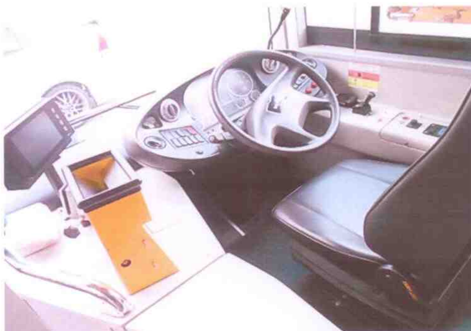
Photo 15 shows the indicators at the driver's seat. Other operational indicators were unable to be initialize due to the flat battery. Hence, no test was carried out to the Motor Bus operational indicators.
