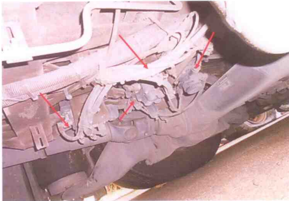
Photo 14 shows a general view of the air tank, valves, pipes and hoses, which are some of the components for the air-assisted braking system of the Motor Bus. This was at the underside of the Motor Bus. We were however not able to carry out any operational test(s) to the braking system of the Motor Bus as its engine was unable to be started.
