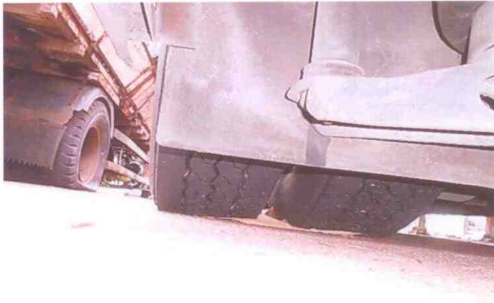
Photo 8 shows the condition of the rear left tyres of the Motor Bus, which were observed to be in serviceable condition with remaining tread depth of approximately 11mm. The tyres, which were wrapped around standard alloy wheel rims, were also observed to be sufficiently inflated for vehicular operation.
