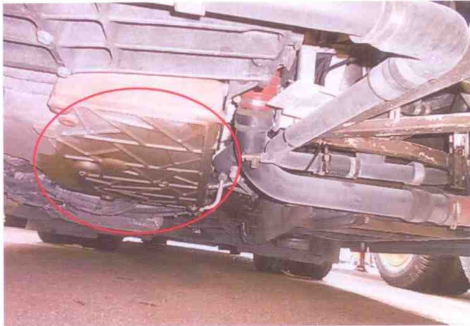
Photo 11 shows the engine underside of the Motor Bus. Our subsequent checks on the underside of the Motor Bus reveals some fluid stain sighted under the engine compartment. Further investigation found that the fluid stain was a pre-existed prior the accident & not a fresh fluid. This was due to some dirt observed on the fluid stain. Conclusive, it is not likely to be related to the accident. Visually, the various undercarriage components of the Motor Bus were all observed to be intact and without any visible damage.
