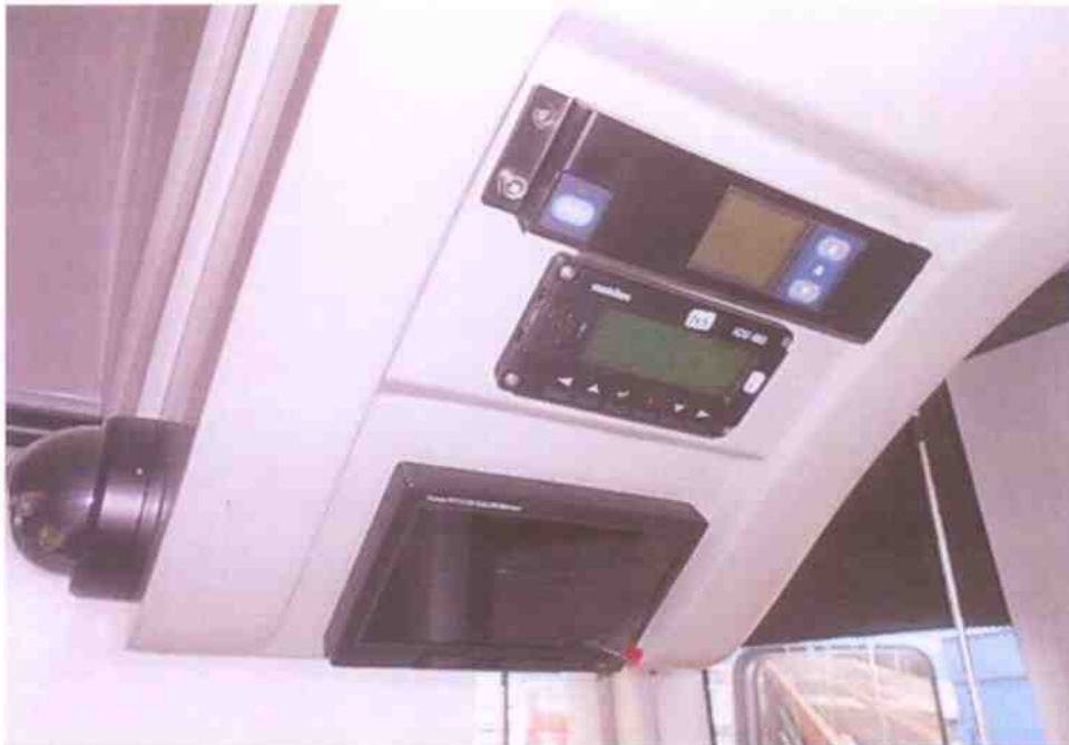
Photo 16 shows the indicators at the driver's seat. Other operational indicators were unable to be initialize due to the flat battery. Hence, no test was carried out to the Motor Bus operational indicators.
