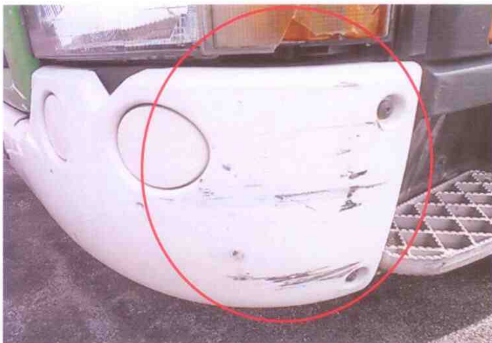
Photo 6 shows a close up view of the minor scratches on the left front lower bumper of the Prime Mover.
