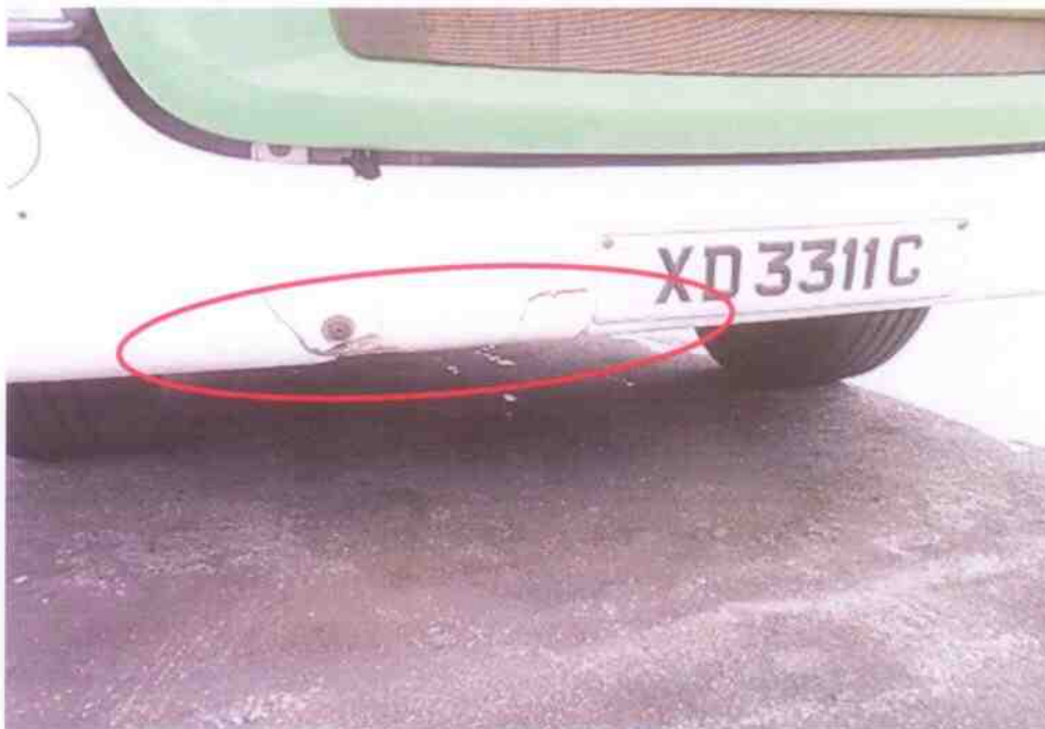
Photo 8 shows a semi-close up view of the minor scratches on the front lower bumper of the Prime Mover.
