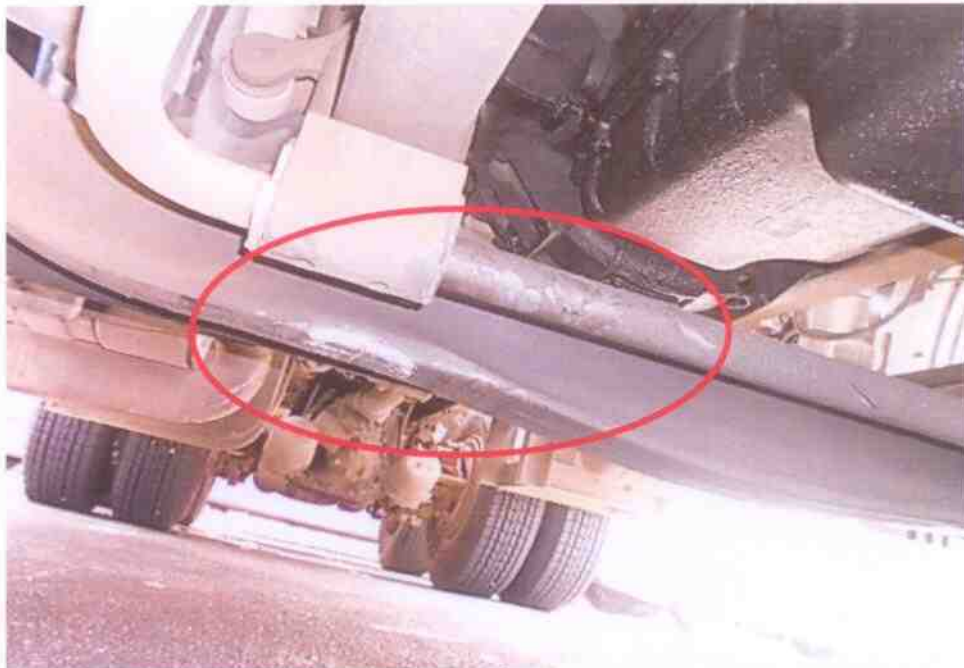
Photo 19 shows from the underside, a deep scratch had occurred as a result of the accident. However, it does not affect the alignment of the steering rack.
