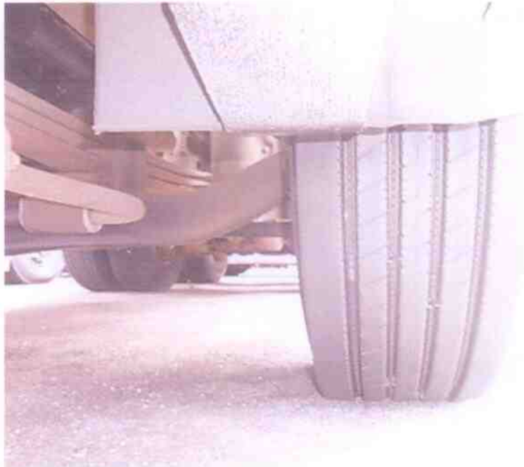
Photo 9 shows the condition of the front left tyre of the Prime Mover, which was observed to be in serviceable condition with remaining tread depth of approximately 11mm.
