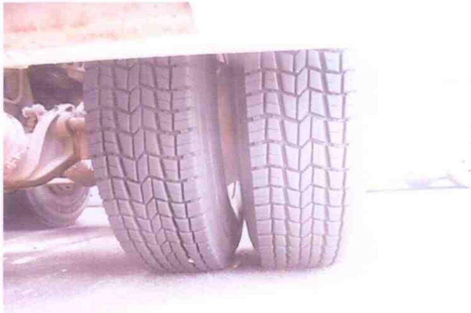
Photo 13 shows the condition of the rear left tyres (Centre Axle) of the Prime Mover, which were observed to be in serviceable condition with remaining, tread depth of approximately 11mm. The tyres were also observed to be sufficiently inflated for vehicular operation.
