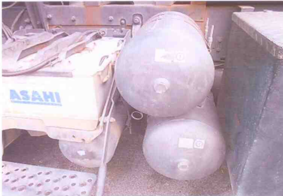
Photo 22 shows a general view of the air tanks, valves, pipes and hoses, which are some of the components for the full air-assisted braking system of the Prime Mover. These components were unaffected by the accident. It had all appeared to be in good general condition and securely fitted upon my visual examination of these parts.
