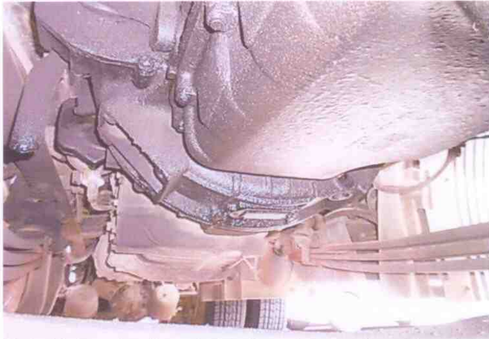
Photo 18 shows from the underside, the engine assembly and transmission assembly of the Prime Mover were both observed to be covered with fresh fluid, suggesting that fluid leakage had occurred as a result of the accident.
