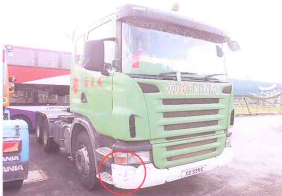
Photo 3 shows a general view of the front right body of the Prime Mover at the time of our inspection. The Prime Mover was observed to have sustained relatively minor damage at its left front lower bumper (circled).
