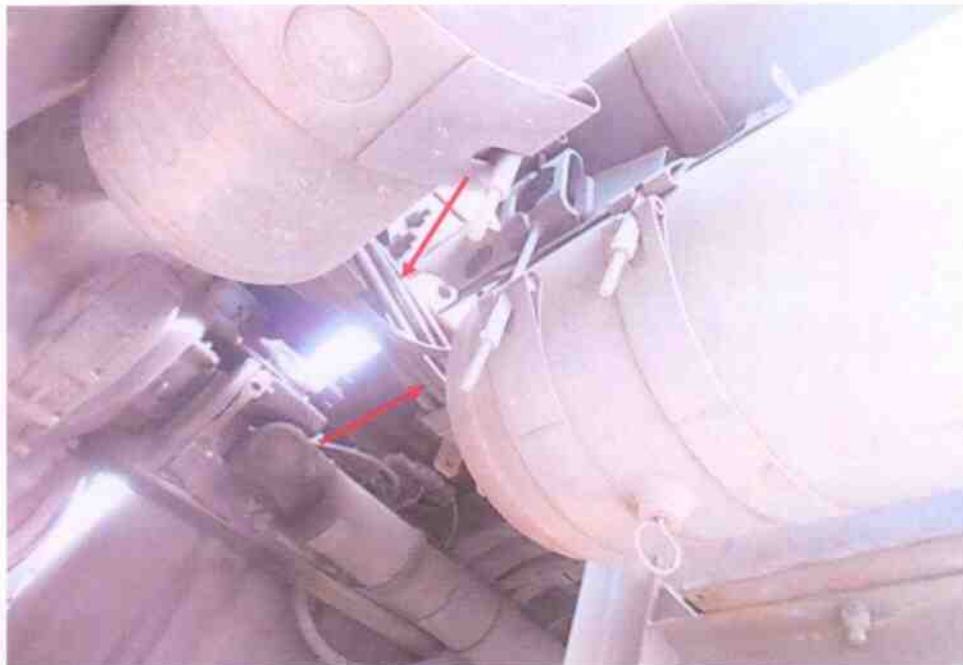
Photo 23 shows a general view of the air tanks, valves, pipes and hoses, which are some of the components for the full air-assisted braking system of the Prime Mover. These components were unaffected by the accident. It had all appeared to be in good general condition and securely fitted upon my visual examination of these parts.
