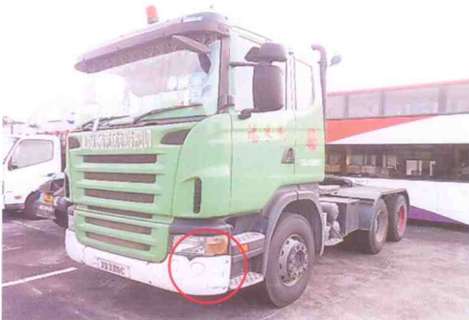
Photo 2 shows a general view of the front left body of the Prime Mover at the time of our inspection. The Prime Mover was observed to have sustained relatively minor damage at its left front lower bumper (circled) & cracked left headlamp.
