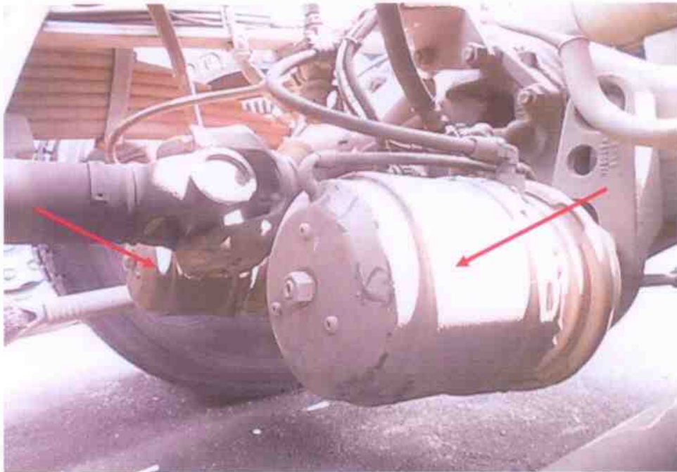
Photo 24 shows the brake air cylinder (arrowed) at the rear left & right wheel of the Prime Mover. Such air cylinder, which is amongst the various components for the full air-assisted braking system, can be found attached to all the front wheels and all the rear wheels. Upon checking, we had found all the brake air cylinders to be undamaged and securely fitted to all the wheels of the Prime Mover.
