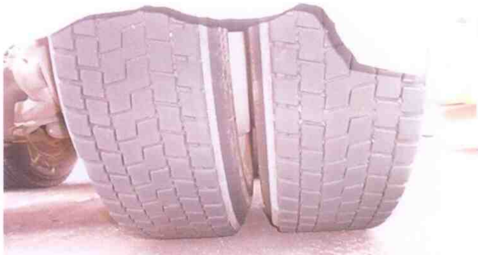
Photo 11 shows the condition of the rear left tyres of the Prime Mover, which were observed to be in serviceable condition with remaining tread depth of approximately 3mm. The tyres were also observed to be sufficiently inflated for vehicular operation.
