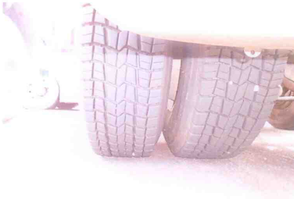
Photo 14 shows the condition of the rear right tyres (Centre Axle) of the Prime Mover, which were observed to be in serviceable condition with remaining, tread depth of approximately 10mm. The tyres were also observed to be sufficiently inflated for vehicular operation.
