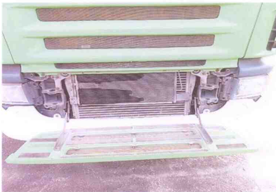
Photo 15 shows the front panel of the Prime Mover open for checks on some of the components of the cooling system.
