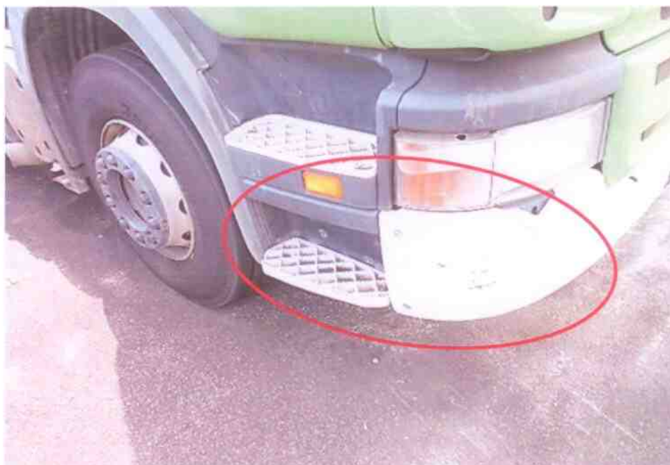
Photo 5 shows a semi-close up view of the front right body of the Prime Mover at the time of our inspection. The Prime Mover was observed to have sustained relatively minor damage at its front right lower bumper (circled).
