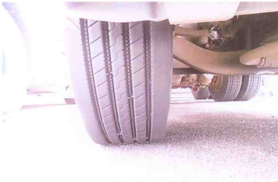
Photo 10 shows the condition of the front right tyre of the Prime Mover, which was observed to be in serviceable condition with remaining tread depth of approximately 10mm.
