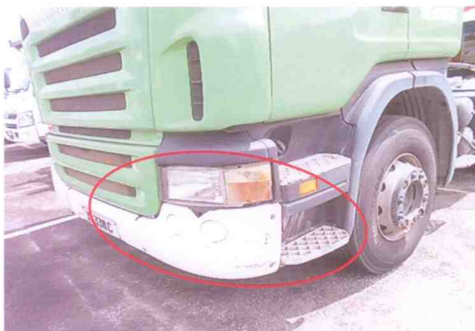
Photo 4 shows a semi-close up view of the minor scratches on the left front lower bumper of the Prime Mover.
