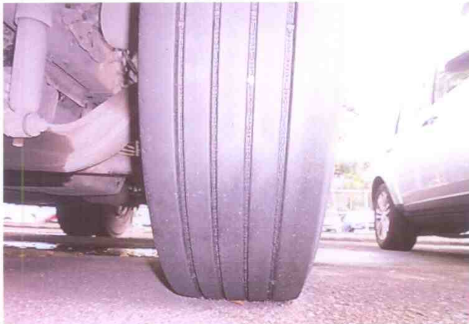
Photo 4 shows the condition of the front left tyre of the Prime Mover, which was observed to be in serviceable condition with remaining tread depth of approximately 8mm.
