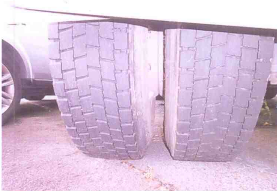
Photo 6 shows the condition of the rear left tyres of the Prime Mover, which were observed to be in serviceable condition with remaining tread depth of approximately 4mm. The tyres were also observed to be sufficiently inflated for vehicular operation.
