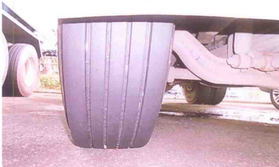
Photo 5 shows the condition of the front right tyre of the Prime Mover, which was observed to be in serviceable condition with remaining tread depth of approximately 8mm.
