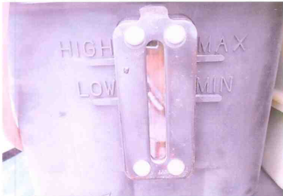
Photo 9 shows the engine coolant reservoir of the Prime Mover at the time of our inspection. The engine coolant was observed to be of sufficient level and without any visible contamination for operational purposes.
