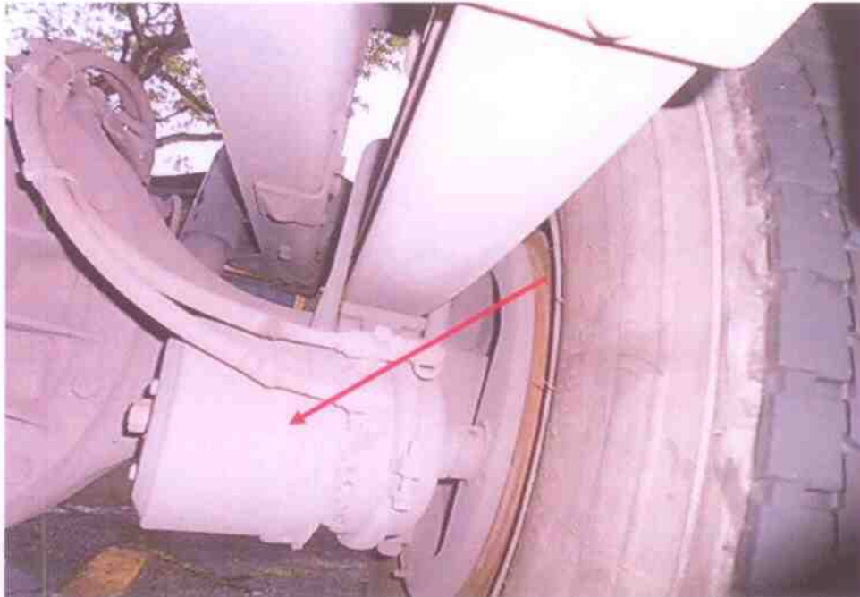
Photo 15 shows the brake air cylinder (arrowed) at the rear left wheel of the Prime Mover. Such air cylinder, which is amongst the various components for the full air-assisted braking system, can be found attached to all the front wheels and all the rear wheels. Upon checking, we had found all the brake air cylinders to be undamaged and securely fitted to all the wheels of the Prime Mover.
