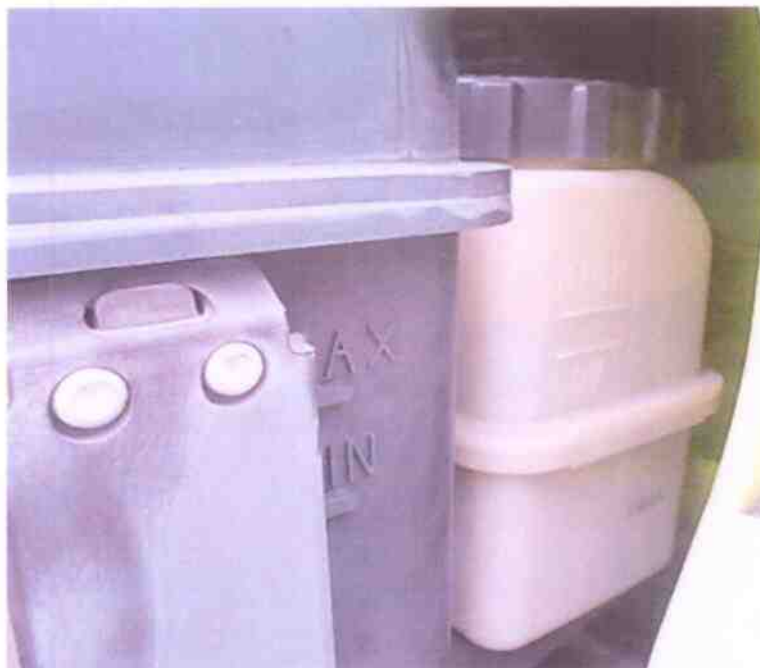
Photo 10 shows checks being carried out to the power steering fluid of the Prime Mover. The power steering fluid was observed to be of sufficient level and without any visible contamination for operational purposes.
