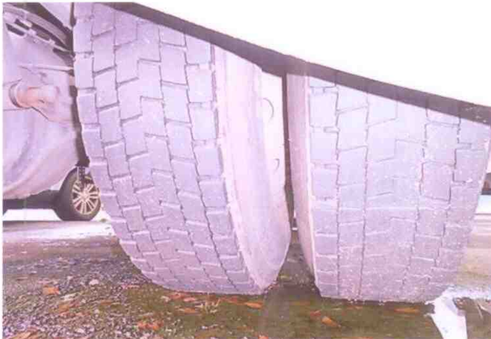
Photo 7 shows the condition of the rear right tyres of the Prime Mover, which were observed to be in serviceable condition with remaining tread depth of approximately 4mm. The tyres were also observed to be sufficiently inflated for vehicular operation.
