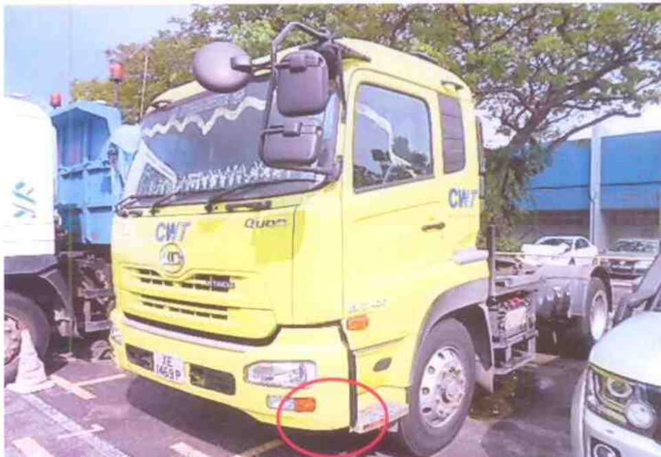
Photo 2 shows a general view of the front left body of the Prime Mover at the time of our inspection. The Prime Mover was observed to have sustained relatively minor damage at its left front lower bumper (circled).
