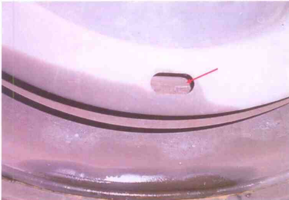
Photo 17 shows the brake shoes (brake pads) at the front left wheel of the Prime Mover. The brake shoes (brake pads) of the Prime Mover were all found to be in serviceable condition with sufficient frictional material for operational purposes.
