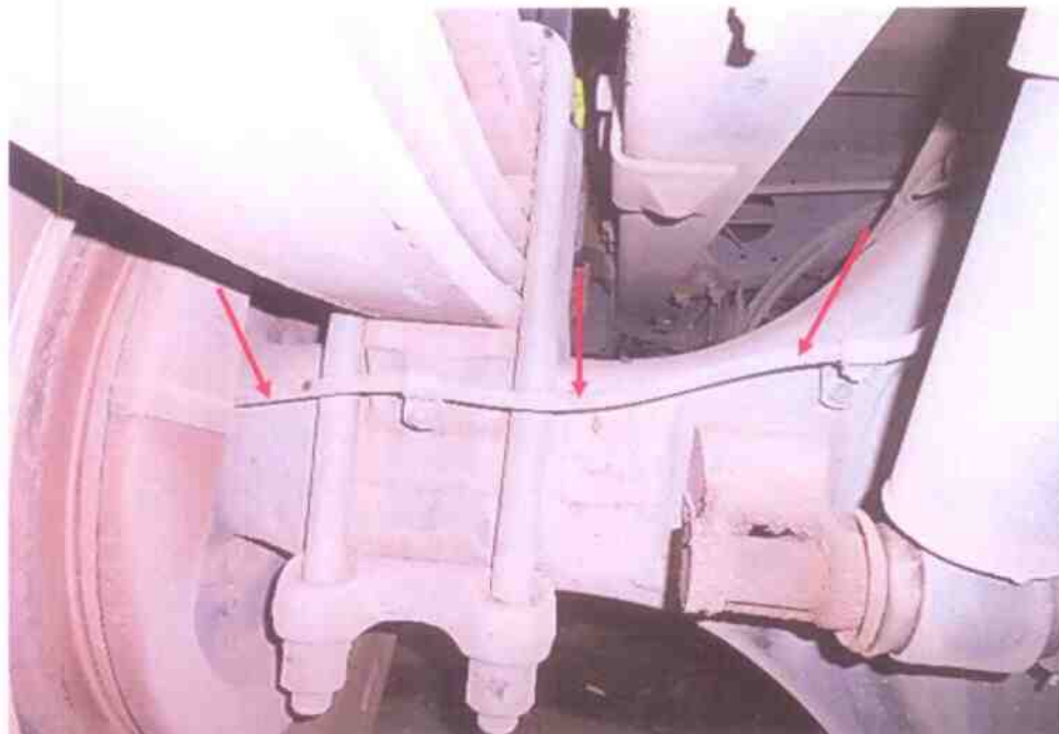
Photo 14 shows the undercarriage components at the rear left wheel of the Prime Mover, in particular the brake hose (arrowed). Visual inspection of the mechanical components of the Prime Mover's braking system appear to suggest that its braking system was in serviceable condition at the material time of accident.
