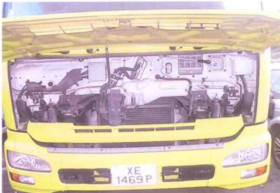
Photo 8 shows the front panel of the Prime Mover lifted for checks on some of the components of the cooling system & engine system.
