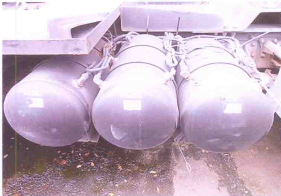
Photo 13 shows a general view of the air tanks, valves, pipes and hoses, which are some of the components for the full air-assisted braking system of the Prime Mover. These components were unaffected by the accident. It had all appeared to be in good general condition and securely fitted upon my visual examination of these parts.
