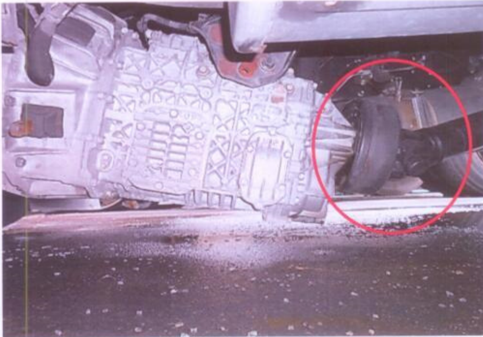
Photo 16 shows the transmission assembly (circled) of the Motor Lorry was observed to be bent due to the accident's collision.
