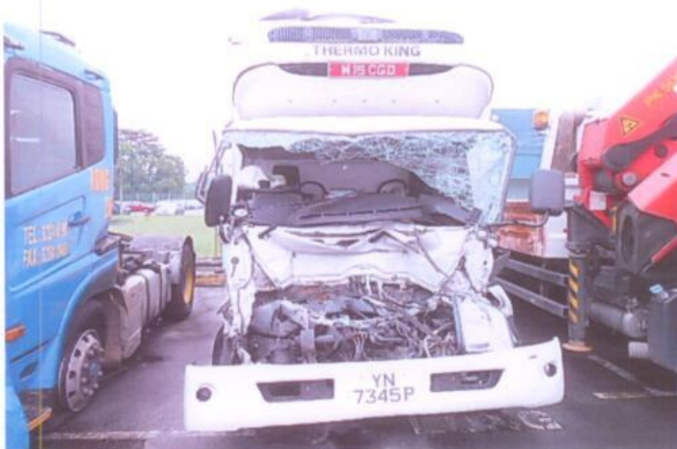
Photo 1 shows a general view of the frontal portion of the Motor Lorry at the time of my inspection. The Motor Lorry was observed to have sustained extensive impact damage at its frontal portion. The impact force was relatively significant, causing its entire front cabin to be buckled and crumpled.
