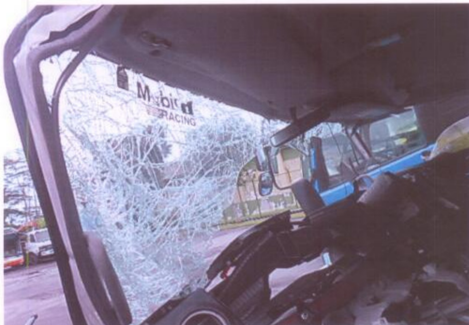
Photo 8 shows the interior of the front cabin. The windshield was observed to be cracked due to the accident.
