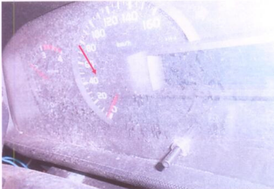
Photo 24 shows the speedo meter that was observed to be not in working condition due to the damages sustained in the ignition system. However, evidence showed that it is in serviceable condition prior the accident. The driver's airbag was activated at the time of the impact.
