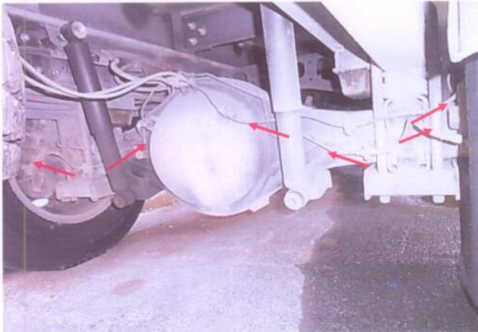
Photo 23 shows the brake pipes and hoses, which were visibly unaffected by the accident. I was however not able to carry out any operational tests to the braking system of the Motor Lorry due to the extent of damage to its front cabin, which had affected several mechanical components of the braking system like the brake booster and brake pedal amongst others.
