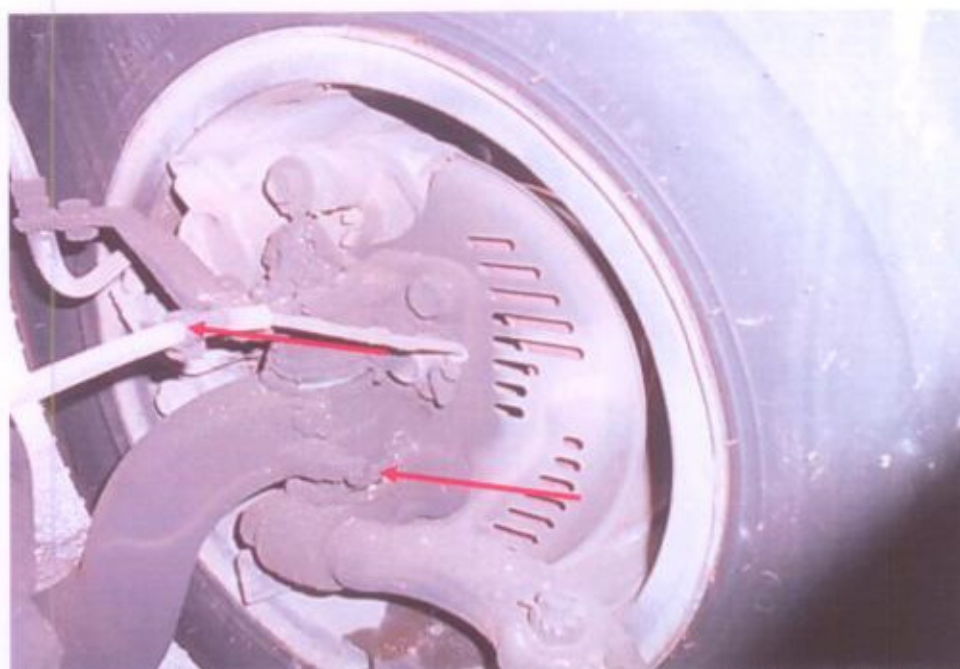
Photo 20 shows the unaffected mechanical components on the front right wheel of the steering system. The steering shaft and steering rack of the Motor Lorry were observed to be intact and securely attached to the front left wheel. No fluid leakage on the brake fluid hoses.
