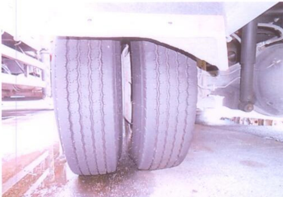
Photo 12 shows the condition of the rear left tyres of the Motor Lorry, which was observed to be in serviceable condition with remaining tread depth of approximately 8mm. There was no tear, cut or burst mark(s) on the outer and the inner sidewalls as well as across the tread of these 2 tyres, which were also observed to be sufficiently inflated for vehicular operation.
