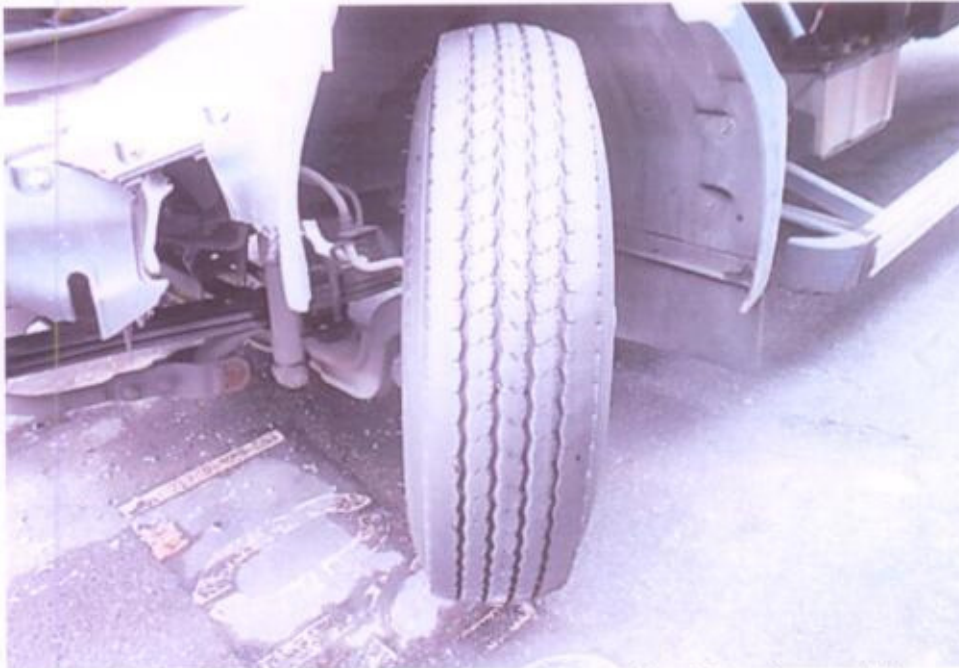
Photo 13 shows the condition of the front left tyre of the Motor Lorry, which was observed to be in serviceable condition with remaining tread depth of approximately 8mm. There was also no tear, cut or burst mark(s) on the outer and the inner sidewalls as well as across the tread of this tyre.
