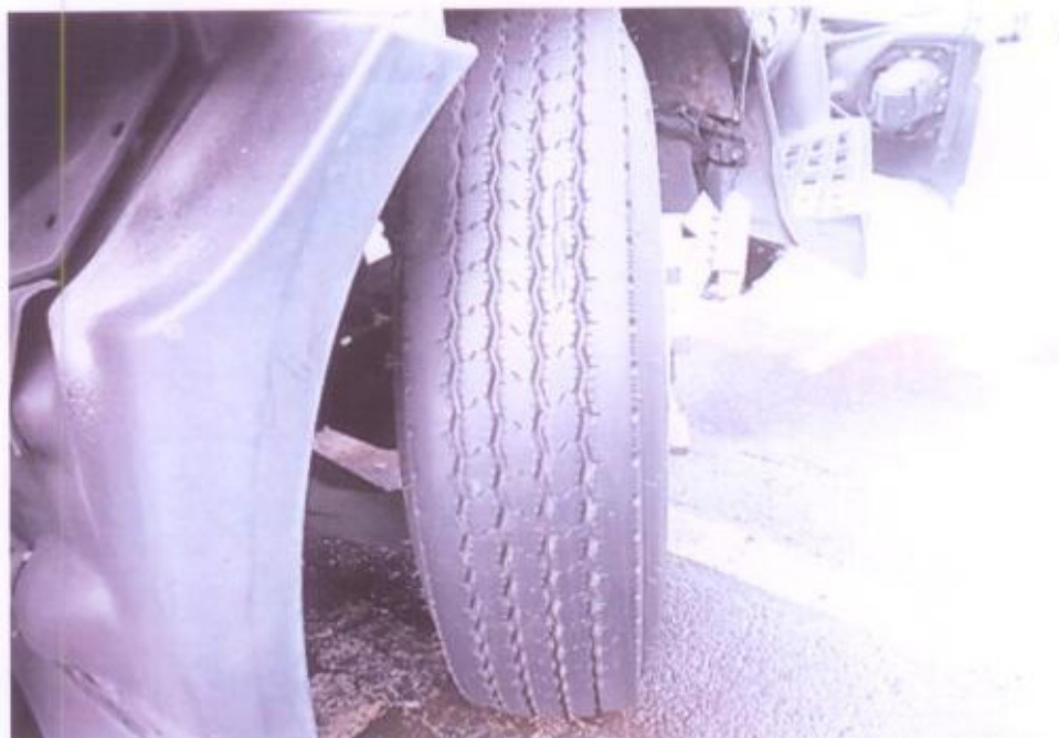
Photo 14 shows the condition of the front right tyre of the Motor Lorry. The front right tyre was observed to be in serviceable condition with remaining tread depth of approximately 7mm. There was also no tear, cut or burst mark(s) on the outer and the inner sidewalls as well as across the tread of this tyre. The tyre, which was wrapped around alloy wheel rim, was also observed to be sufficiently inflated for vehicular operation.
