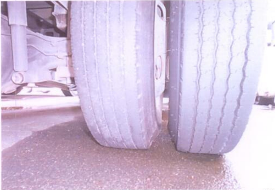
Photo 11 shows the condition of the rear right tyres of the Motor Lorry, which was observed to be in serviceable condition with remaining tread depth of approximately 5mm.
