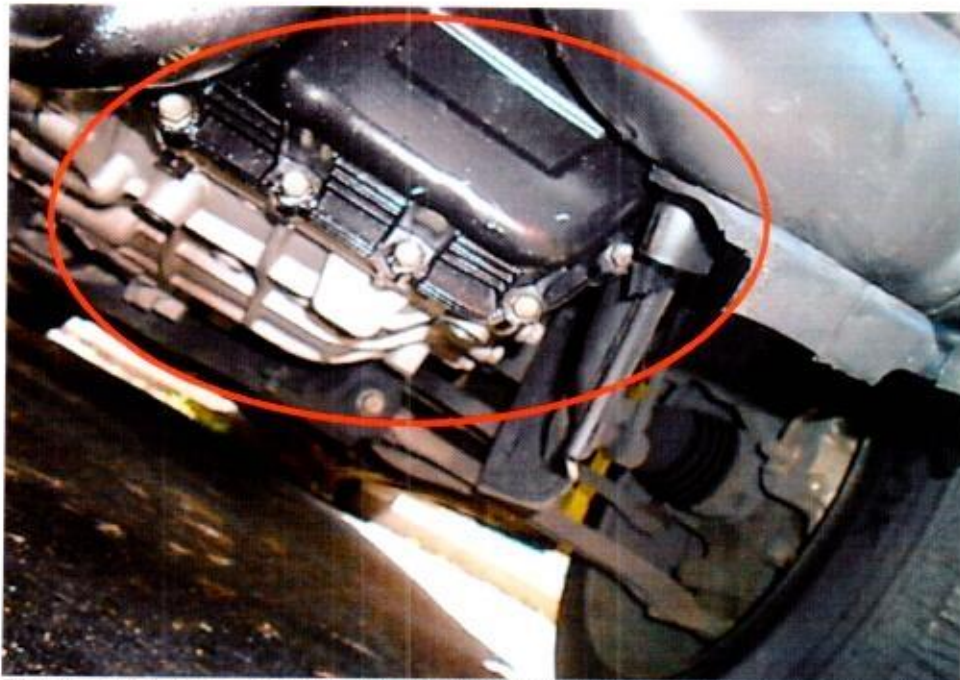
Photo 23 shows the frontal portion of the undercarriage components of the Motor Taxi. We observe signs of fluid leakage at the time of our inspection of the Motor Taxi.
