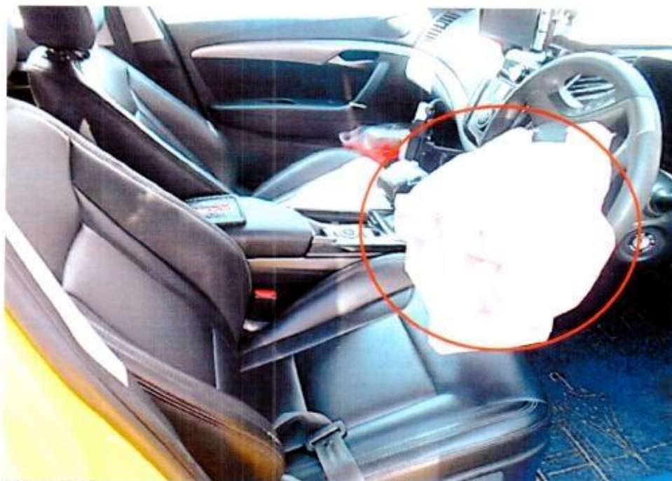
Photo 8 shows a closer view of the interior portion of the Motor Taxi. The impact force was significant, causing the driver's seat air bag activated.
