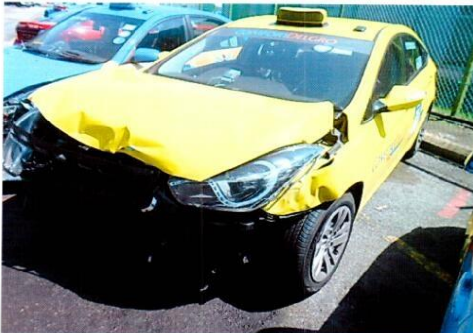
Photo 3 shows a general view of the front left portion of the Motor Taxi at the time of our inspection. The Motor Taxi was observed to have sustained extensive impact damage at its frontal portion.
