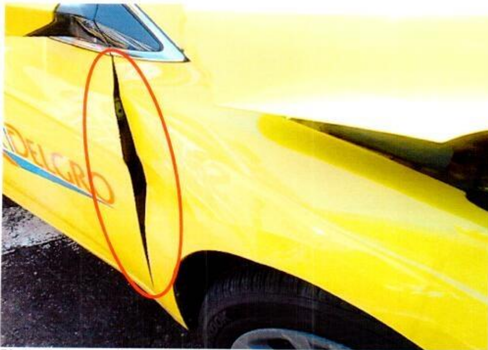
Photo 7 shows a closer view of the damage at the right frontal portion of the Motor Taxi. The impact force was significant, causing the right hand door to be partially stuck, unable to be open smoothly.
