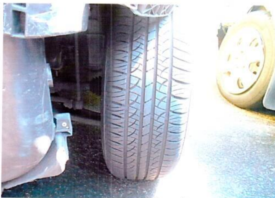
Photo 12 shows the condition of the front left tyre of the Motor Taxi, which was observed to be in serviceable condition with remaining tread depth of approximately 7mm. There was no tear, cut or burst mark(s) on the outer and the inner sidewalls as well as across the tread of this tyre, which was also sufficiently inflated for vehicular operation.
