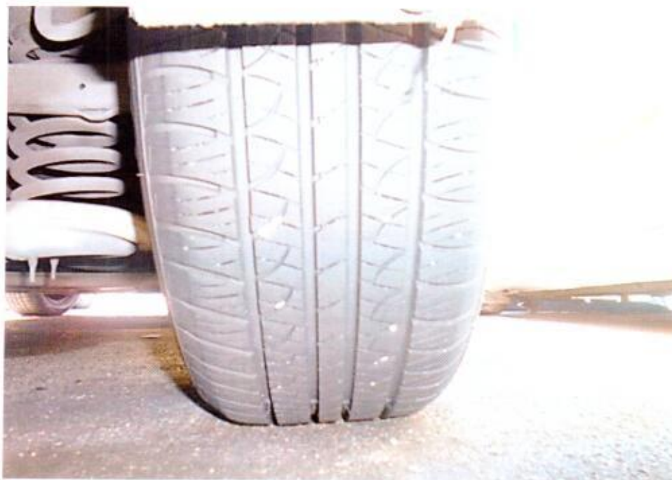
Photo 13 shows the condition of the rear right tyre of the Motor Taxi, which was observed to be in serviceable condition with remaining tread depth of approximately 6mm. There was also no tear, cut or burst mark(s) on the outer and the inner sidewalls as well as across the tread of this tyre.
