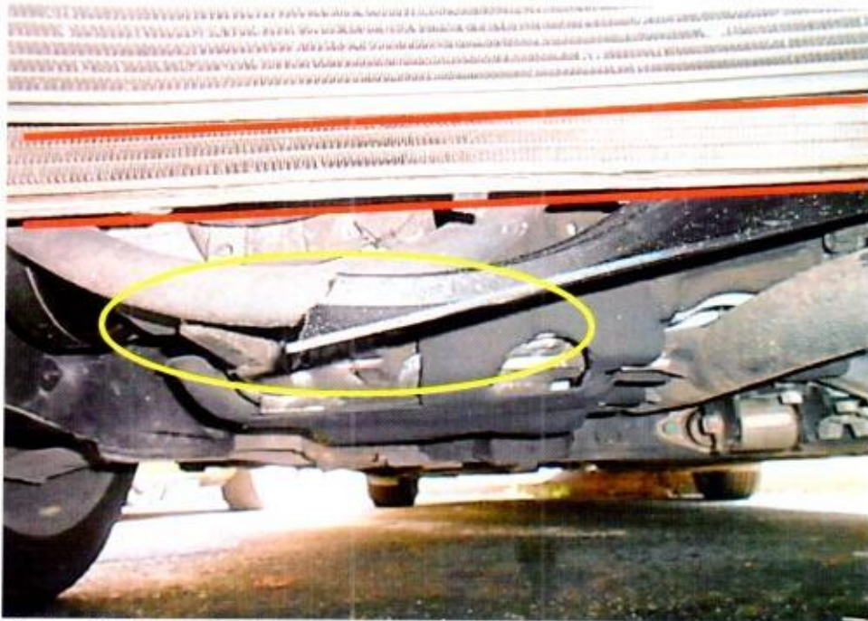
Photo 15 shows the close up view of the radiator of the Motor Taxi. Dented radiator (Red arrowed) & broken parts (Circled) was observed at time of our inspection.
