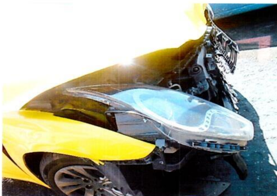
Photo 5 shows a closer view of the damage at the frontal right portion of the Motor Taxi. The impact force was significant, causing the various parts and components inside the engine compartment to be pushed inwards, towards the rear of the Motor Taxi.
