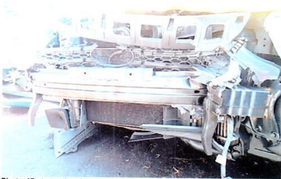
Photo 17 shows the close up view of the re-inforcement bar, air intake system, ignition system, transmission system & cooling system that was observed to be damaged likely due to the accident impact.
