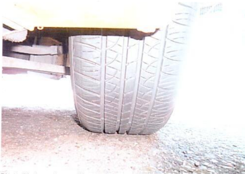
Photo 11 shows the condition of the front right tyre of the Motor Taxi, which was observed to be in serviceable condition with remaining tread depth of approximately 7mm. There was no tear, cut or burst mark(s) on the outer and the inner sidewalls as well as across the tread of this tyre.
