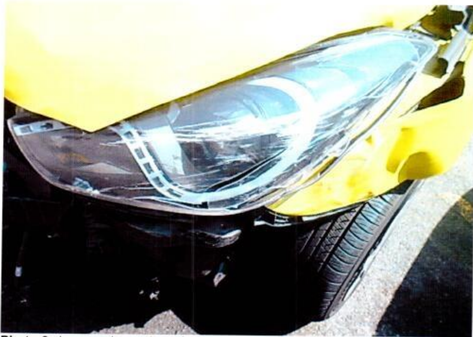
Photo 6 shows a closer view of the damage at the frontal left portion of the Motor Taxi. The impact force was significant, causing the various parts and components inside the engine compartment to be pushed inwards, towards the rear of the Motor Taxi.
