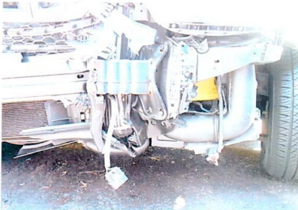
Photo 16 shows the close up view of the re-inforcement bar, air intake system, ignition system, transmission system & cooling system that was observed to be damaged likely due to the accident impact.
