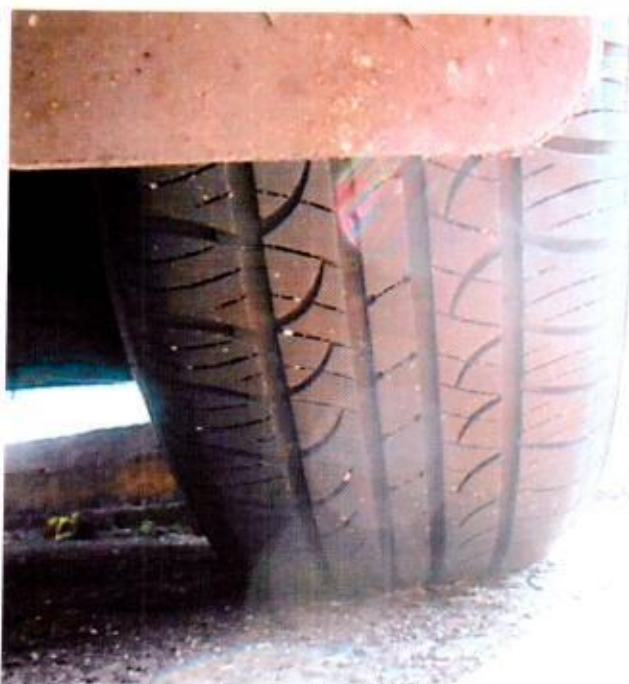
Photo 14 shows the condition of the rear left tyre of the Motor Taxi, which was observed to be in serviceable condition with remaining tread depth of approximately 6mm. There was also no tear, cut or burst mark(s) on the outer and the inner sidewalls as well as across the tread of this tyre.
