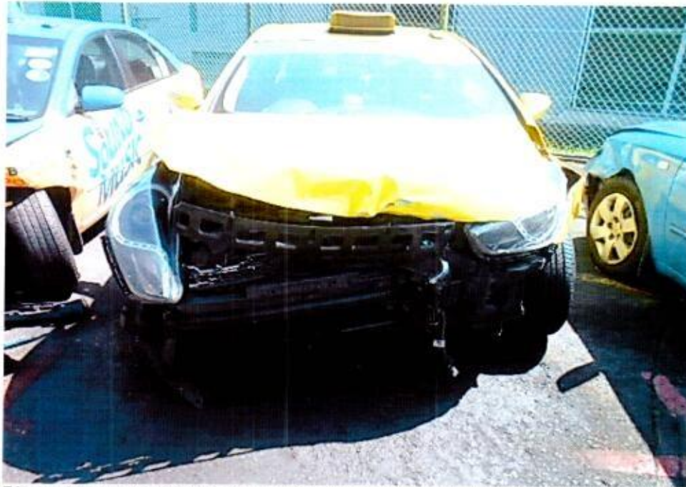
Photo 1 shows a general view of the frontal portion of the Motor Taxi at the time of our inspection. The Motor Taxi was observed to have sustained extensive impact damage at its frontal portion. The impact force was significant, causing the various parts and components inside the engine compartment to be buckled inwards.
