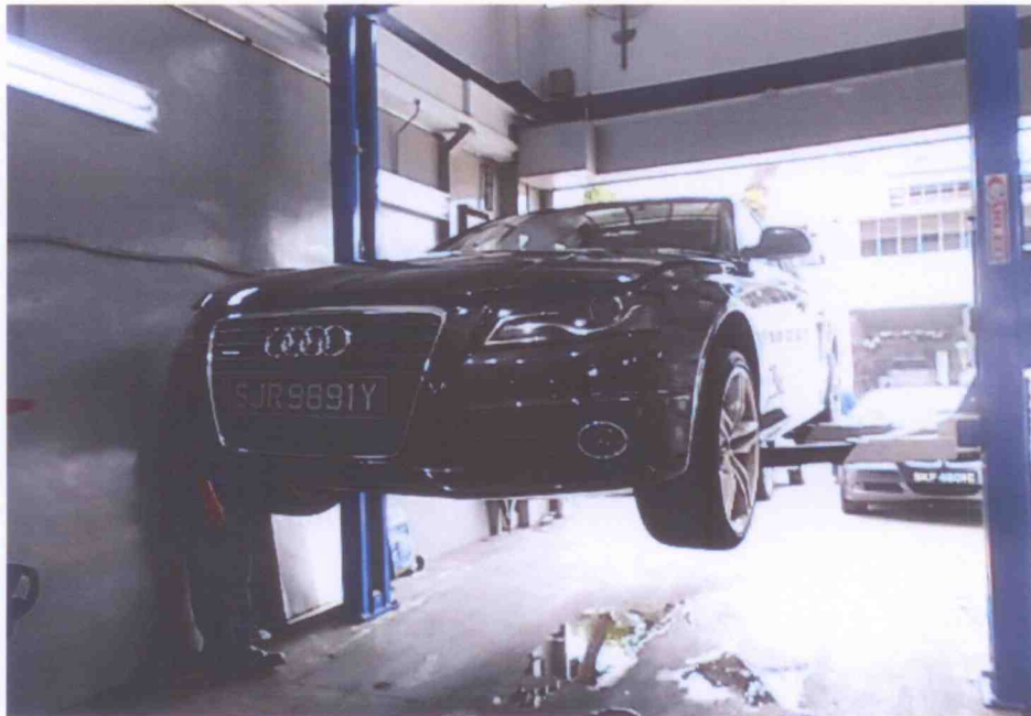
Photo 5 shows the Insured Vehicle being hoisted up for checks on its underside, in particular to its transmission assembly and transmission fluid.
