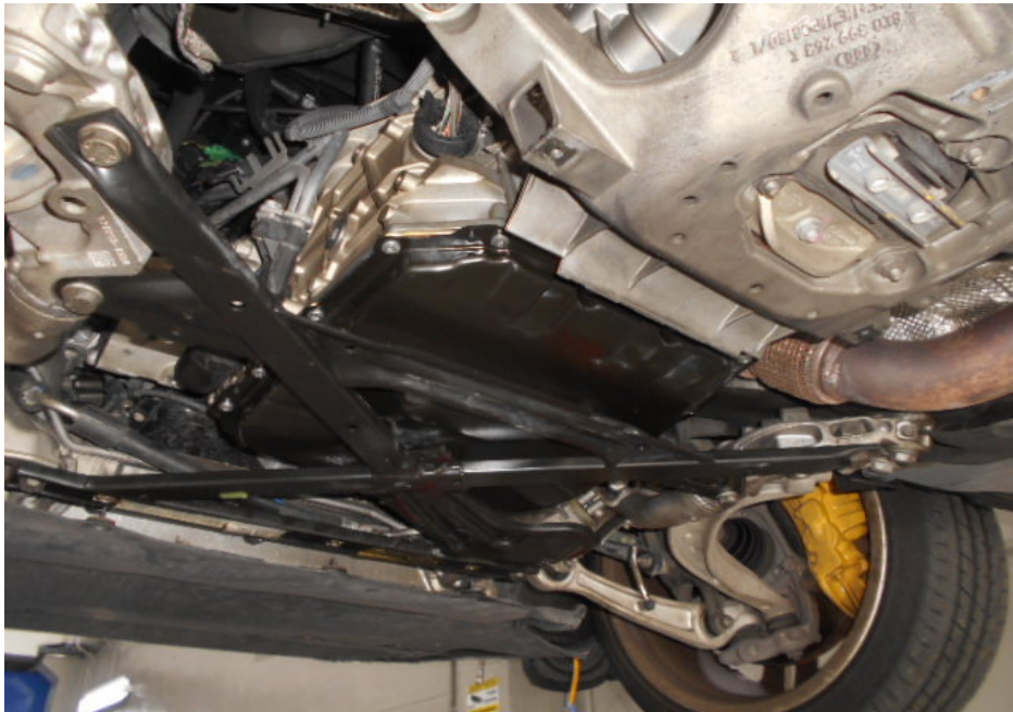
Photo 7 shows a general view of the underside of the Insured Vehicle where the transmission housing was located. There was no sign(s) of fluid stain(s) and/or fluid leakage observed on the underside of the Insured Vehicle.
