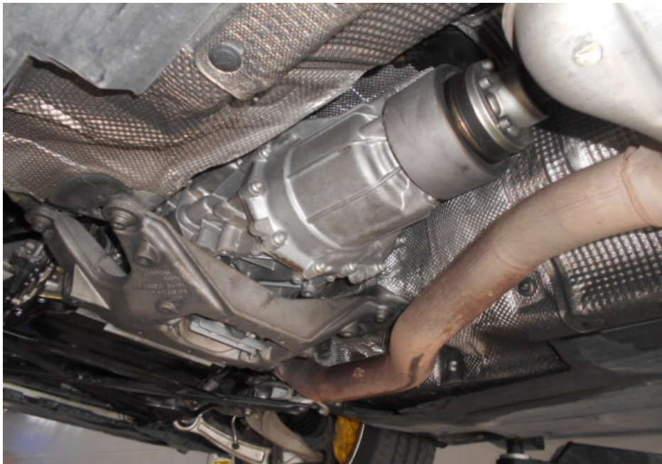
Photo 8 shows a general view of the underside of the Insured Vehicle, at the area where the transmission housing was located. There was no sign(s) of fluid stain(s) and/or fluid leakage observed on the underside of the Insured Vehicle. There was also no visible damage observed on the transmission housing. The electronic sensors were all securely fitted into the connector ports.
