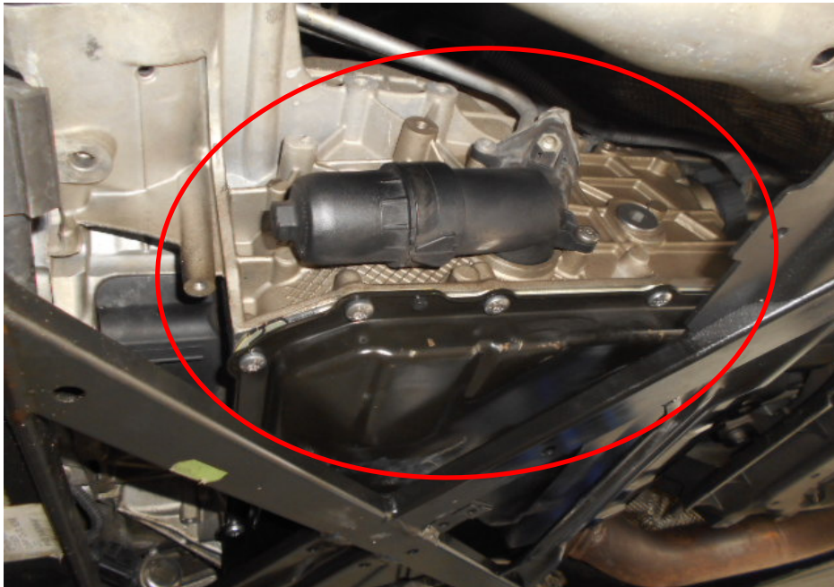
Photo 10 shows a general view of the Insured Vehicle's transmission valve body (mechatronic) (circled).
