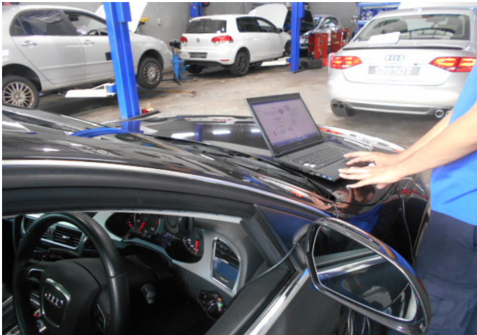
Photo 3 shows the diagnostic test being carried out on the Insured Vehicle to check for any electronic fault(s). Data from the various electronic control modules of the Insured Vehicle were being retrieved.
