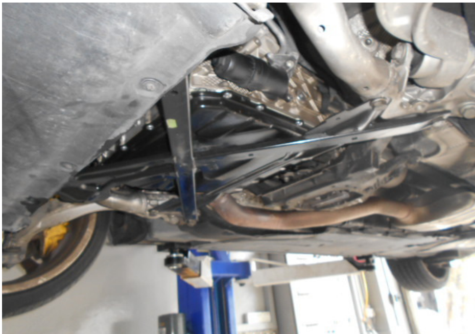
Photo 6 shows a general view of the underside of the Insured Vehicle where the transmission housing was located. There was no sign(s) of fluid stain(s) and/or fluid leakage observed on the underside of the Insured Vehicle.
