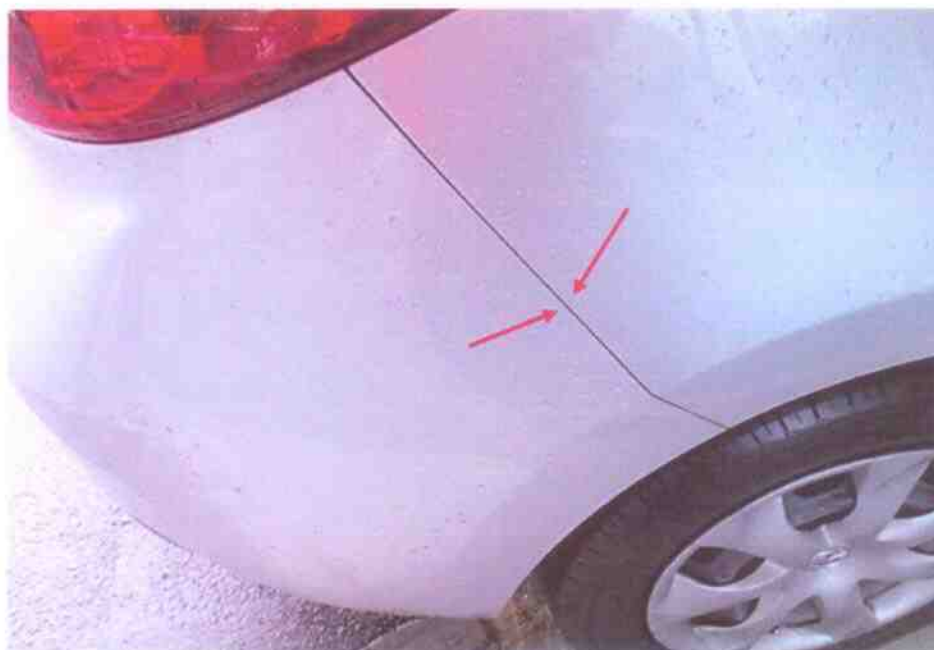
Photo 8 shows a close up view of the right corner edge of the rear bumper of the Mazda. We observed that there was no misalignment at the corner edges (red arrows).
