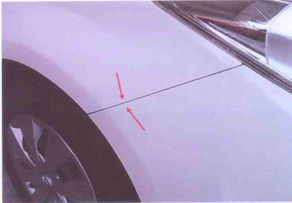
Photo 13 shows a close up view of the right corner edge of the front bumper of the Toyota. We observed that there was no misalignment at the corner edges (red arrows).
