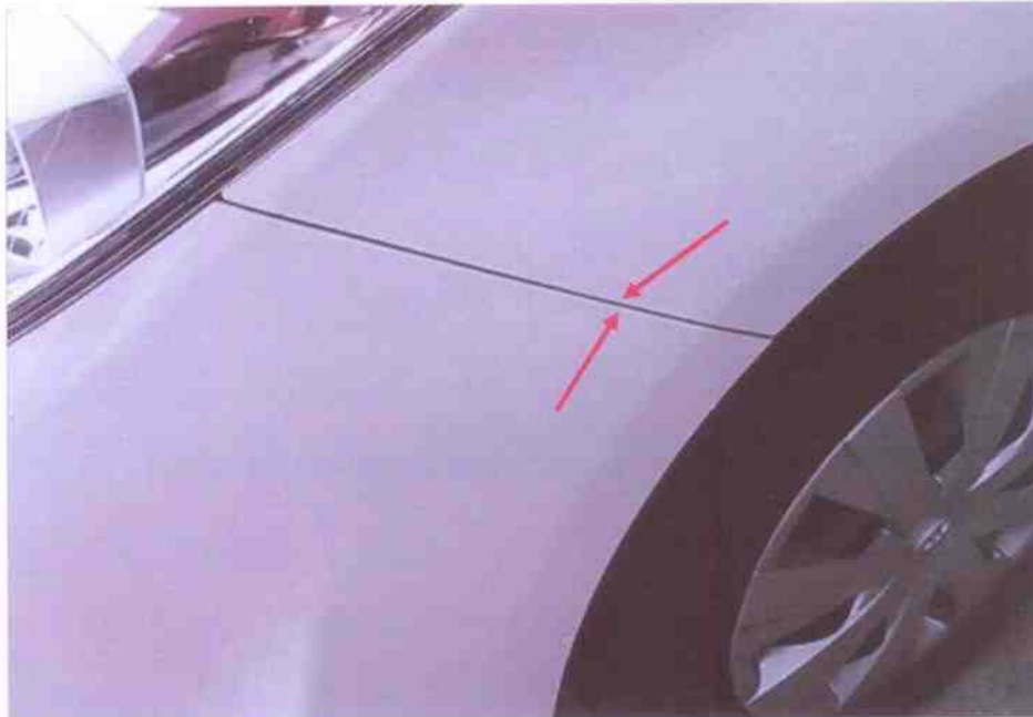
Photo 14 shows a close up view of the left corner edge of the front bumper of the Toyota. We observed that there was no misalignment at the corner edges (red arrows).
