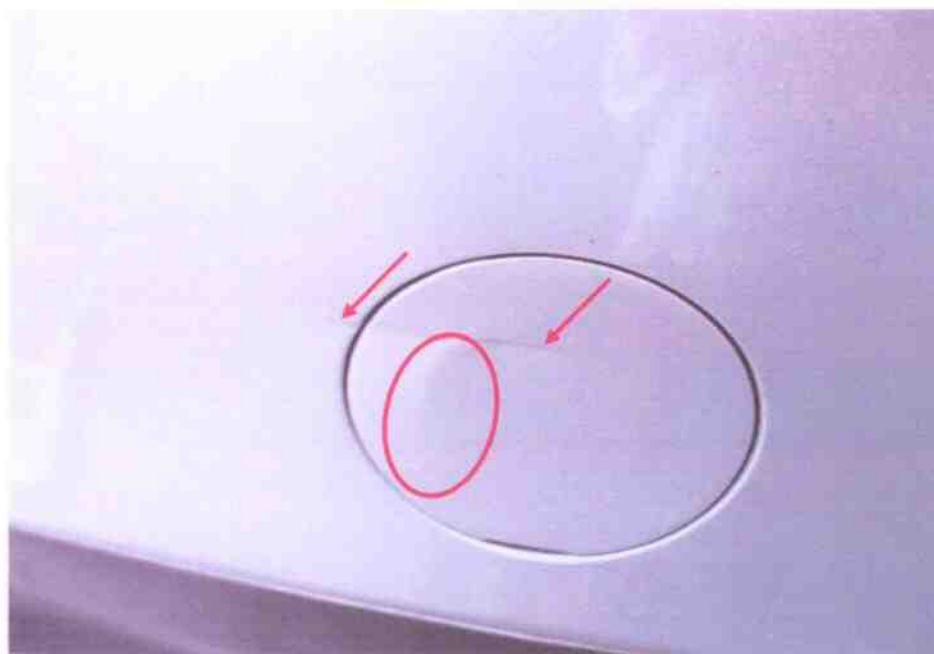
Photo 7 shows a close up view of the faint broken black marks which had stretched horizontally downwards towards the lower left portion of the Mazda's rear bumper (red arrows). Below the black marks there was a right-facing crescent- shaped slight indentation (circled). The right-facing crescent- shaped slight indentation was noted to be slightly towards the left from the lower centre portion of the Mazda's rear bumper.
