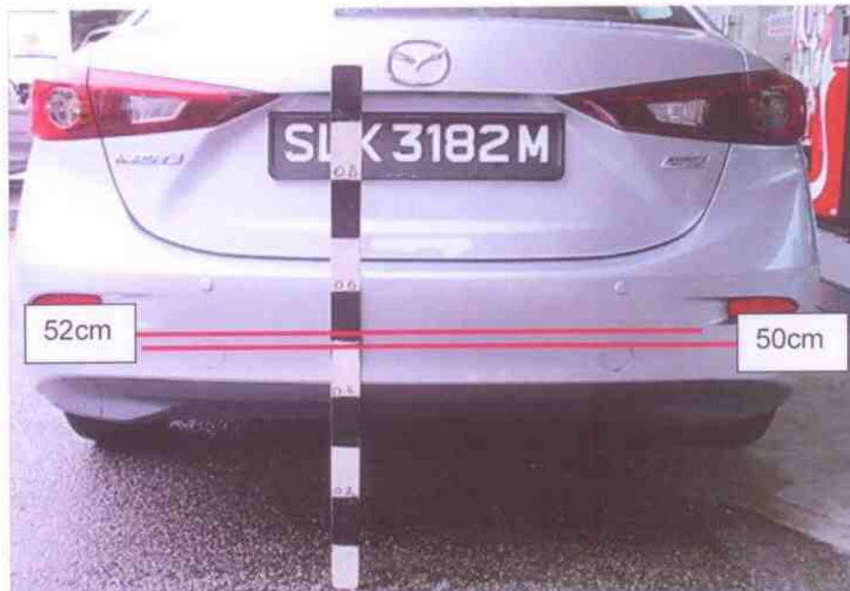
Photo 15 shows the height measurement being conducted on the rear portion of the Mazda. The height above ground level of the top end and lower end of the damages that were found on the lower portion of the rear bumper of the Mazda were measured to be approximately between 50cm and 52cm above ground level respectively.
