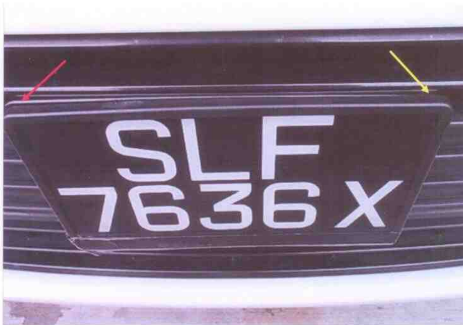
Photo 11 shows a top view of the Toyota's front number plate. The frame was observed to be distorted and bent with the top left corner of the frame appearing to be pressed inwards (yellow arrow) as compared to the right top corner (red arrow). However there was no obvious crack or break on the front number plate frame.
