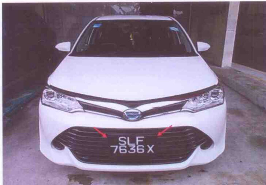
Photo 10 shows the general view of the front portion of the Toyota at the time of our physical inspection. The only body part shape on the front of the Toyota that could possibly correspond to the damages found on the lower portion of the rear bumper of the Mazda was the top portion as well as top corners of its rectangular- shaped front number plate frame. (red arrows).
