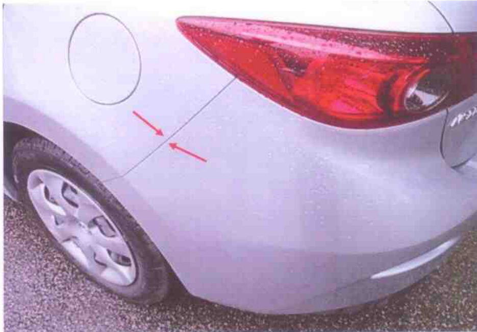
Photo 9 shows a close up view of the left corner edge of the rear bumper of the Mazda. We observed that there was no misalignment at the corner edges (red arrows).
