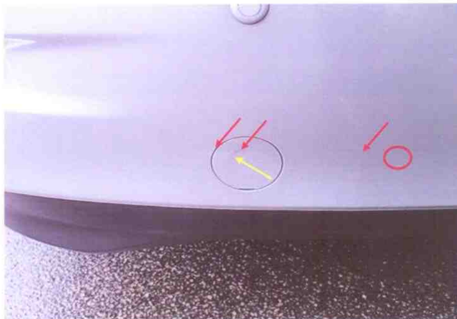
Photo 4 shows upon closer examination, we observed a left-facing curved black mark on the lower centre portion of its rear bumper (circled) followed by faint broken black marks which had stretched horizontally downwards towards the lower left portion of its rear bumper (red arrows). Below the black marks there was a right-facing crescent- shaped slight indentation (yellow arrow). The right-facing crescent- shaped slight indentation was noted to be slightly towards the left from the lower centre portion of the Mazda's rear bumper.
