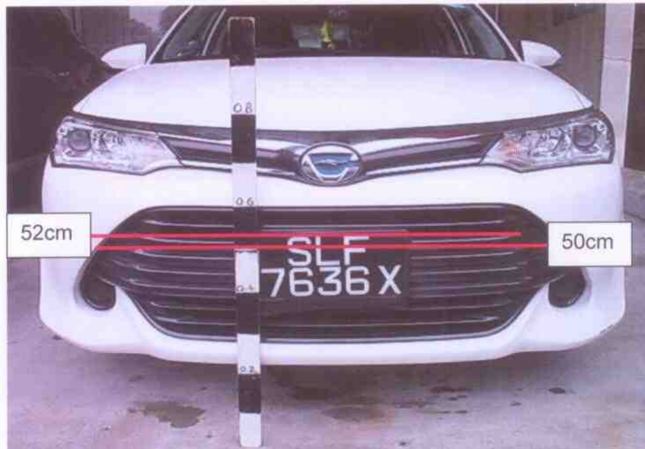
Photo 16 shows the height measurement being conducted on the front portion of the Toyota. The top portion of the Toyota's front number plate frame is within the 50cm to 52cm range.
