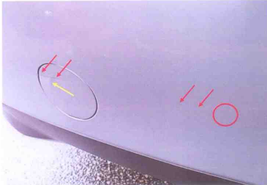
Photo 5 shows a closer view of the left-facing curved black mark on the lower centre portion of the Mazda's rear bumper (circled) followed by faint broken black marks which had stretched horizontally downwards towards the lower left portion of its rear bumper (red arrows). Below the black marks there was a right-facing crescent-shaped slight indentation (yellow arrow). The right-facing crescent-shaped slight indentation was noted to be slightly towards the left from the lower centre portion of the Mazda's rear bumper.
