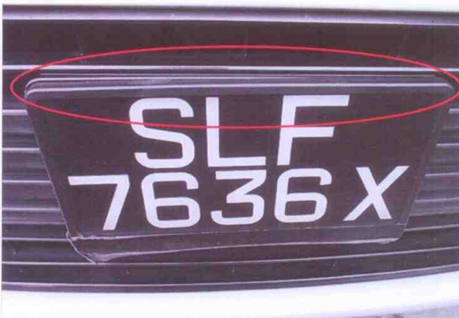
Photo 12 shows a closer view of the front number plate of the Toyota. The front number plate frame was also observed to be at a slight downward angle (circled).
