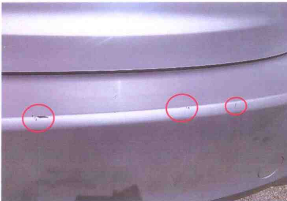
Photo 2 shows a closer view of the rear portion of the Mazda at the time of reporting, which was 4 days after the accident. Paint chip marks were found on the top centre portion of the rear bumper (circled).
