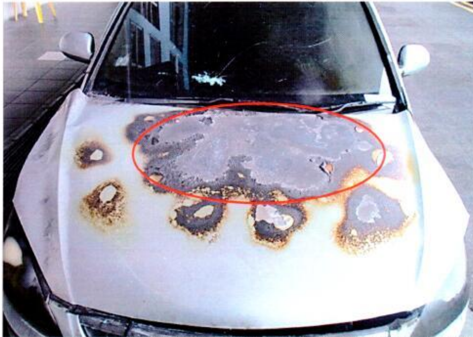
Photo 8 shows the burn pattern and whitish burn marks (circled) that were found on the centre portion of the front bonnet of the Insured Vehicle. Such whitish burn marks are a result of exposure to prolonged heat intensity, which may indicate where the fire had started. Rust would also begin to develop on these areas soon after the fire.
