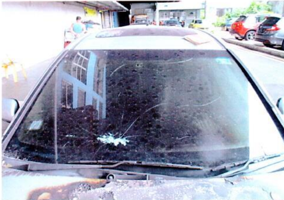
Photo 4 shows the general view of the front windscreen of the Insured Vehicle at the time of our inspection. The fire damage to the Insured Vehicle was confined to its front portion. Its front windscreen, front windscreen wipers, front wiper panel garnish and front windscreen water nozzles were amongst the body parts that were found to have been affected as a result of the fire.
