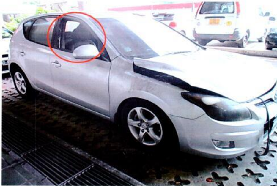
Photo 2 shows the general view of the right side of the Insured Vehicle at the time of our inspection. The fire damage to the Insured Vehicle was confined to its front portion. Its front bonnet, right side panel and right headlight were amongst the body parts that were found to have been affected as a result of the fire. The driver window glass was observed to be smashed (circled).
