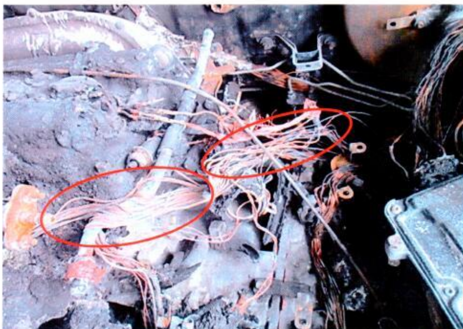
Photo 12 shows a closer view of the greenish residue found on some of the wirings (circled) at the centre portion of the engine compartment. The presence of such greenish residue suggests occurrence of an electrical short circuit.
