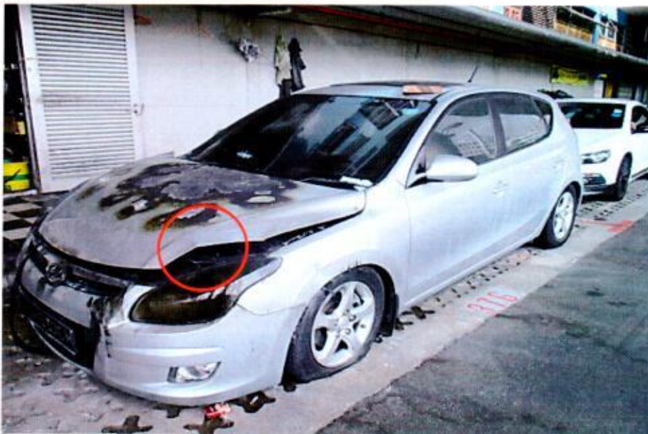
Photo 3 shows the general view of the left side of the Insured Vehicle at the time of our inspection. The fire damage to the Insured Vehicle was confined to its front portion. Its front bonnet, left side panel, left headlight, front left tyre and front left wheel rim were amongst the body parts that were found to have been affected as a result of the fire. The left side of the front bonnet of the Insured Vehicle was slightly buckled (circled), likely due to rescue damage.
