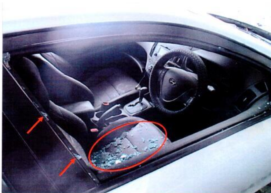
Photo 6 shows the interior compartment of the Insured Vehicle, which was observed to be partially burnt and/or melted. The dashboard and front windscreen were amongst the parts that were found to have been partially burnt and/or melted as a result of the fire. The driver window glass was observed to be smashed. Upon closer inspection, we found glass shards on the edges of the driver window (red arrows) as well as on the driver seat (circled).
