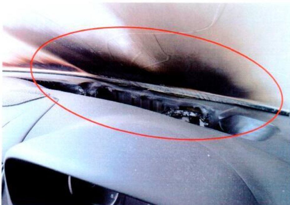
Photo 7 shows a closer view of the damaged front windscreen and dashboard (circled) of the Insured Vehicle (as viewed from the interior compartment).
