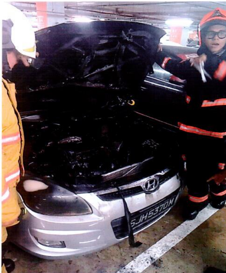
Photo 22 shows the front portion of the Insured Vehicle after the fire was extinguished. The extensive damages observed had corresponded to the events that were related to us by Mr Chia, which is the fire had started from the engine compartment and that the front bonnet was pried open by the SCDF to gain access to the engine bay.
