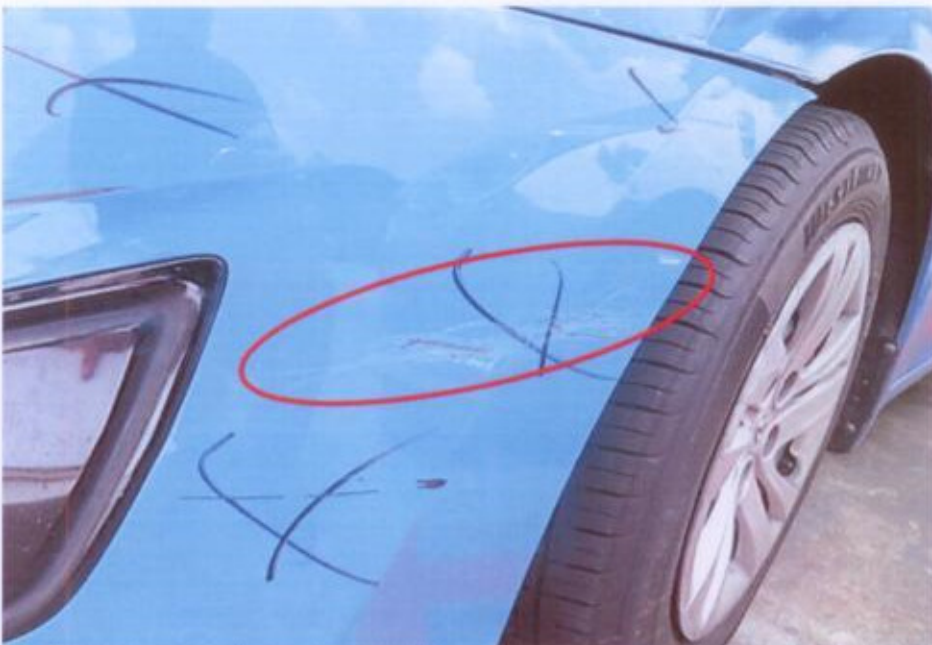
Photo 4 shows a close up view of the paint graze marks found around the left corner of the front bumper of the Taxi (circled).
