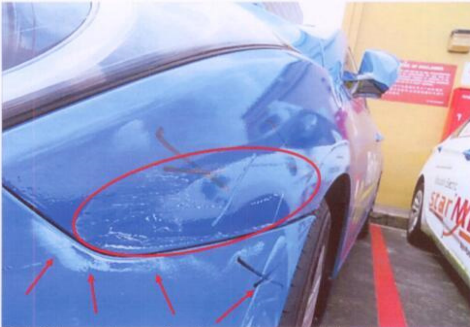
Photo 3 shows a close up view of the paint graze marks found on the top portion of the left side panel as well as around the left corner of the front bumper of the Taxi (red arrows).
