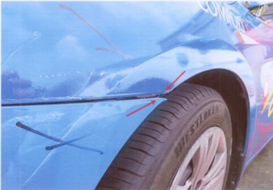
Photo 5 shows a close up view of the left side of the front bumper of the Taxi. We noted that the front bumper was slightly misaligned at its left corner edge (red arrows).
