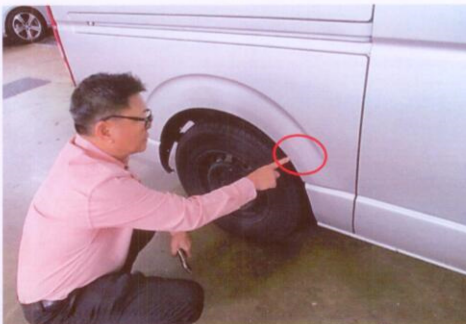
Photo 8 shows a closer examination of the rear right portion of the Van together with Principal Consultant, Mr K K Lau. We found paint graze marks and several paint scratch marks on the front portion of the rear right wheel fender (as pointed by Mr K K Lau) (circled).
