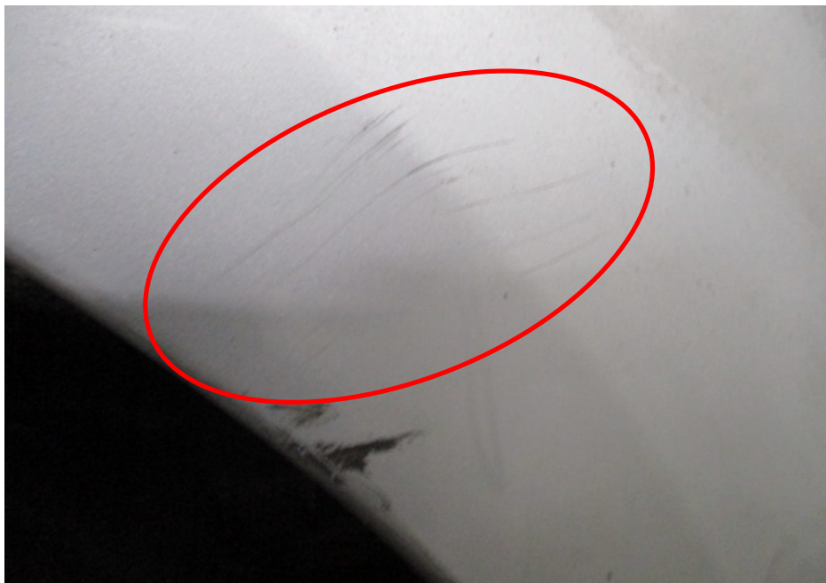
Photo 11 shows a close up view of the several paint scratch marks found on the front portion of the rear right wheel fender (circled).
