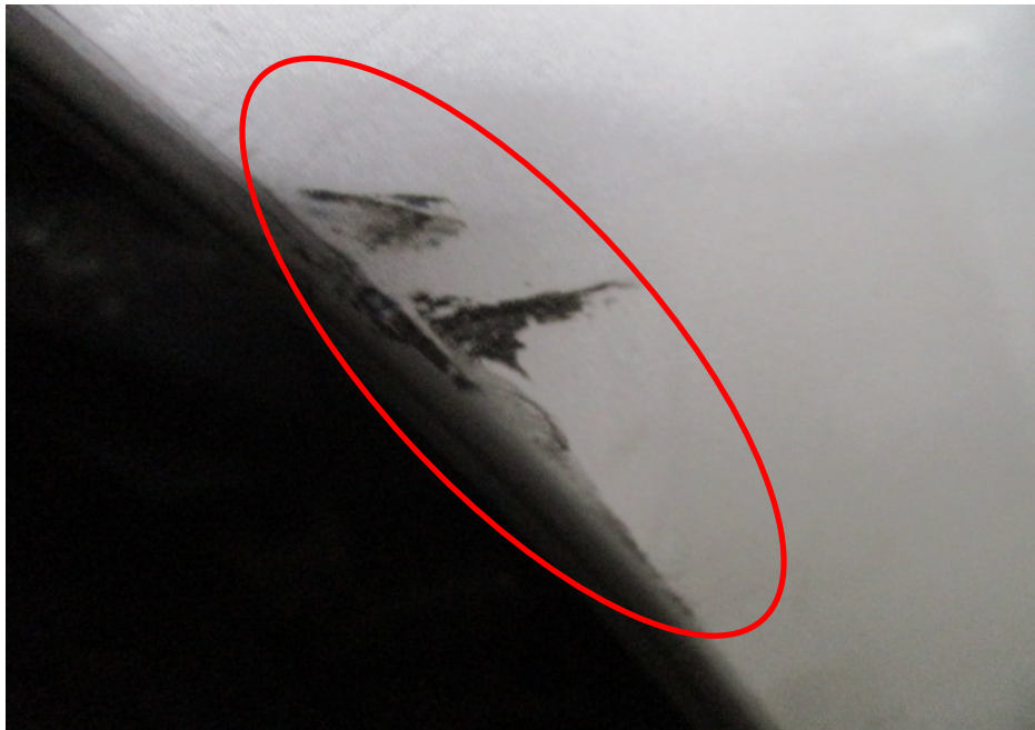
Photo 10 shows a close up view of the paint graze marks found on the front portion of the rear right wheel fender (circled).
