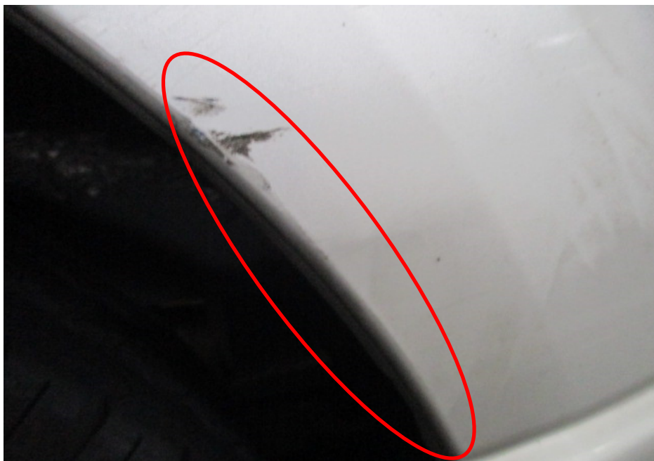
Photo 9 shows a closer view of the paint graze marks found on the front portion of the rear right wheel fender (circled).
