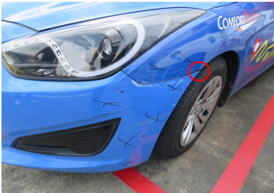
Photo 2 shows a closer view of the left front portion of the Taxi. We observed paint graze marks on the top portion of the left side panel as well as around the left corner of the front bumper (as marked by the X's). We also noted that the front bumper was slightly misaligned at its left corner edge (circled).
