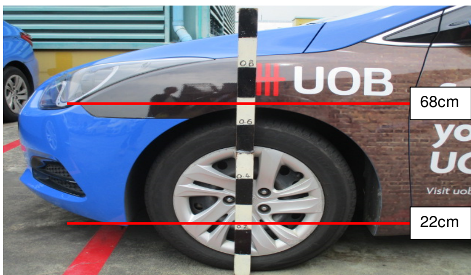
Photo 12 shows the height measurement being conducted on the left front portion of the Taxi (using a similar make and model). The height above ground level of the paint graze marks was between the ranges of 22cm to 68cm.
