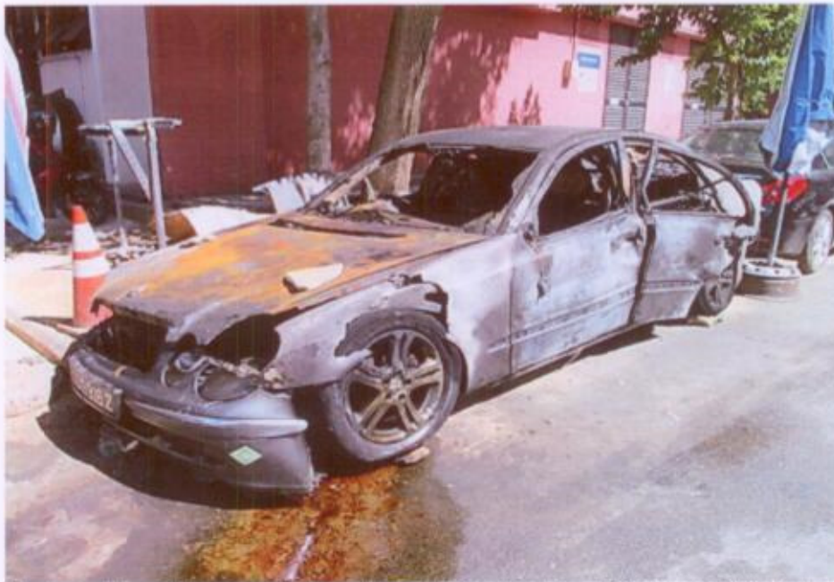
Photo 3 shows the general view of the left front portion of the Insured Vehicle at the time of our inspection. The exterior body of the Insured Vehicle had sustained visible fire damage. This included its front windscreen, front bonnet, headlights, front bumper, front bumper reinforcement panel, left side panel, front left rim and front left tyre.
