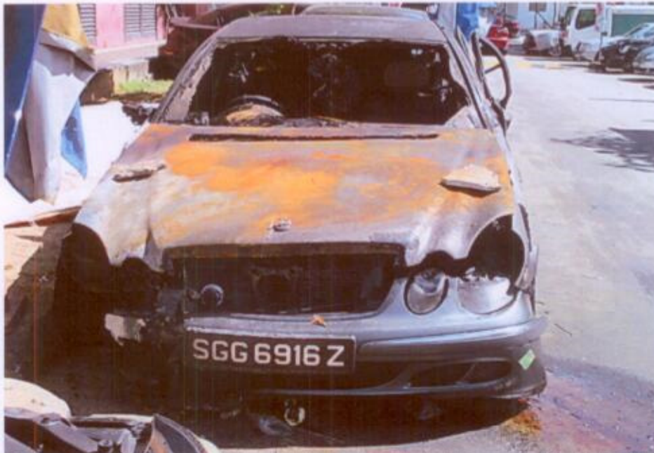
Photo 1 shows the general view of the front portion of the Insured Vehicle at the time of our inspection. The exterior body of the Insured Vehicle had sustained visible fire damage. This included its front windscreen, front bonnet, headlights, front bumper, front bumper reinforcement panel, side panels, front rims and front tyres.
