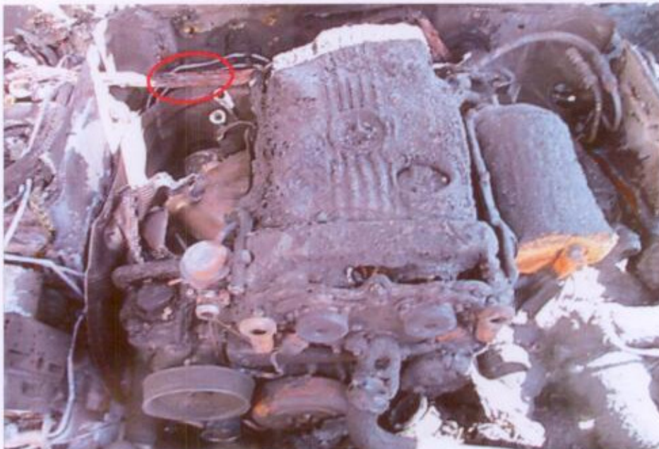
Photo 7 shows the wirings around the rear centre portion of the engine compartment which is near to the vicinity where the fire to the Insured Vehicle had likely started. We observed greenish residue on some of the wirings (circled). The presence of greenish residue indicates internal heating of copper wires, a sign of an electrical short circuit occurring.
