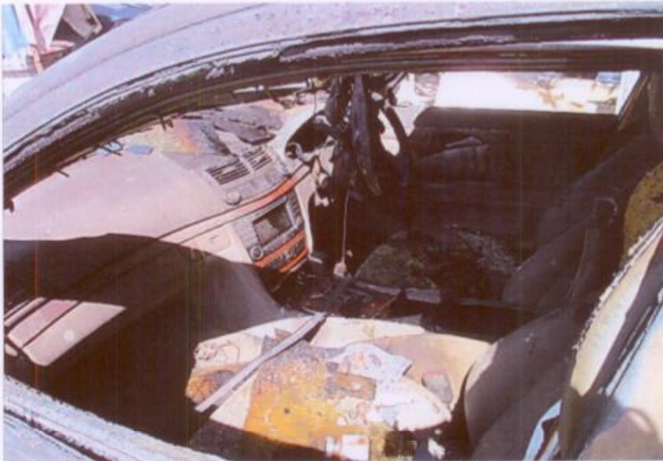
Photo 5 shows the interior compartment of the Insured Vehicle at the time of our inspection. The interior compartment of the Insured Vehicle was observed to be significantly affected by the fire which included the dashboard, steering wheel, front seats and roof upholstery amongst others.
