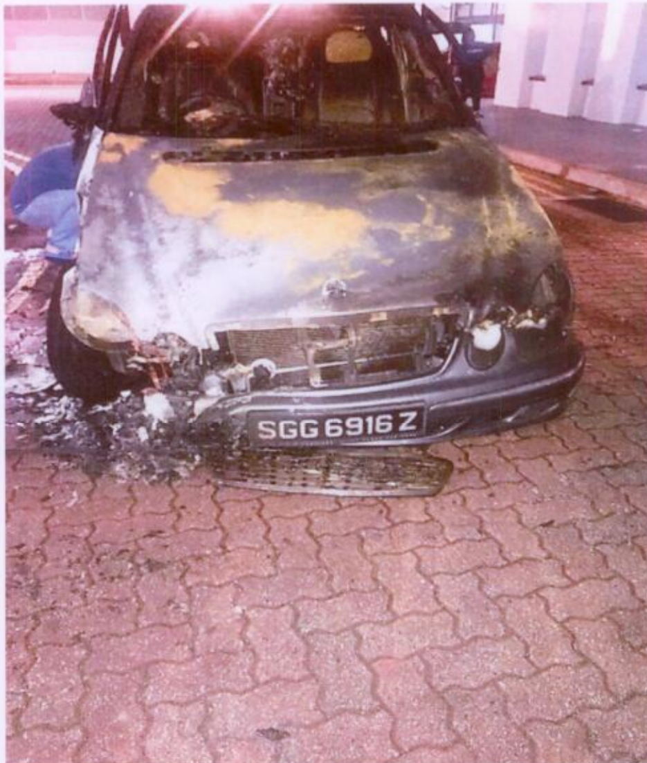
Photo 21 shows a front view of the Insured Vehicle as it was being prepped to be towed away. In general, the extensive damages sustained to the front portion had corresponded to the events that were related to us by Mr Hum, which is the fire started from the front bonnet.
