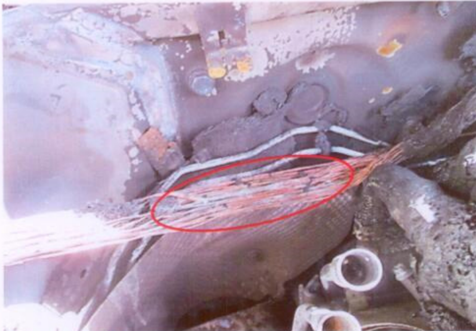
Photo 8 shows a closer view of the greenish residue found on the wirings (circled) at the rear centre portion of the engine compartment. The presence of such greenish residue suggests occurrence of an electrical short circuit.
