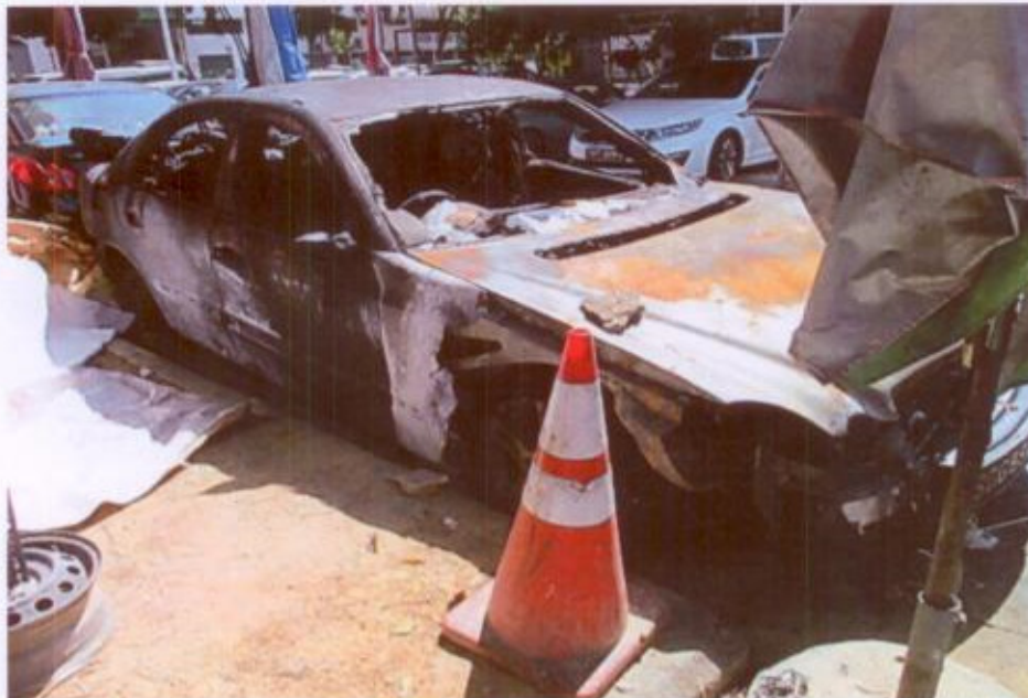
Photo 2 shows the general view of the right front portion of the Insured Vehicle at the time of our inspection. The exterior body of the Insured Vehicle had sustained visible fire damage. This included its front windscreen, front bonnet, headlights, front bumper, front bumper reinforcement panel, right side panel, front right rim and front right tyre.
