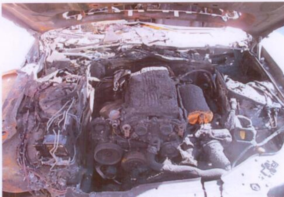
Photo 6 shows a general view of the engine compartment of the Insured Vehicle at the time of our inspection. Most of the components inside the engine compartment were severely burnt and/or melted as a result of the fire.
