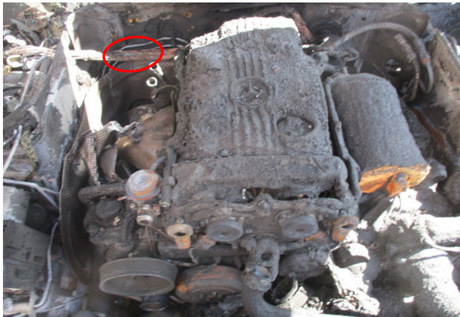
Photo 7 shows the wirings around the rear centre portion of the engine compartment which is near to the vicinity where the fire to the Insured Vehicle had likely started. We observed greenish residue on some of the wirings (circled). The presence of greenish residue indicates internal heating of copper wires, a sign of an electrical short circuit occurring.
