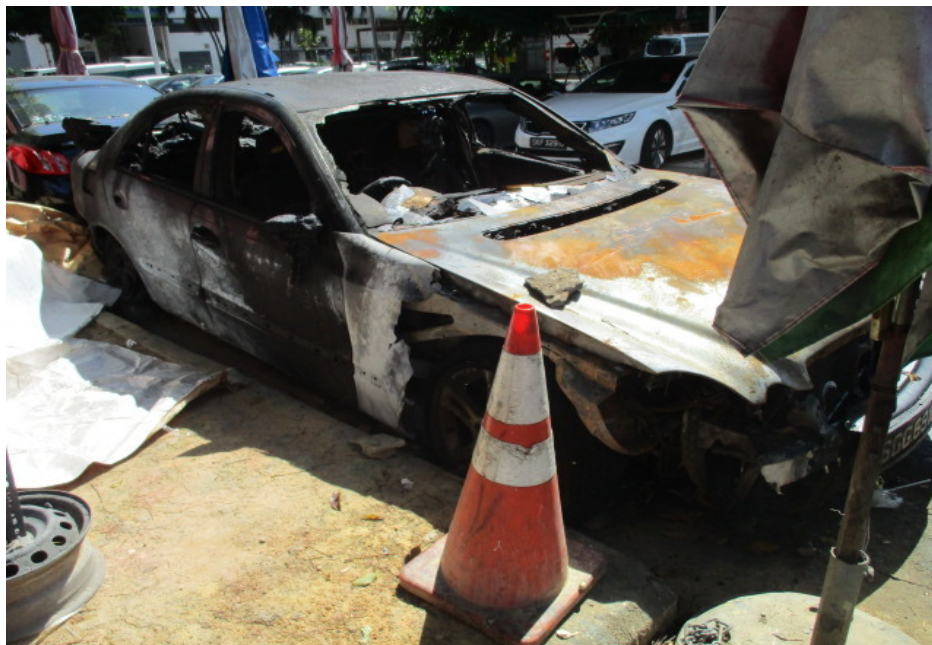
Photo 2 shows the general view of the right front portion of the Insured Vehicle at the time of our inspection. The exterior body of the Insured Vehicle had sustained visible fire damage. This included its front windscreen, front bonnet, headlights, front bumper, front bumper reinforcement panel, right side panel, front right rim and front right tyre.
