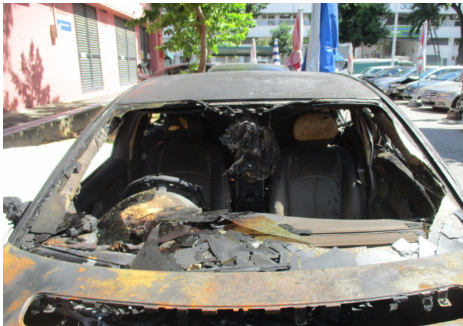
Photo 4 shows a closer view of the front windscreen of the Insured Vehicle at the time of our inspection. The front windscreen had sustained serious fire damage.
