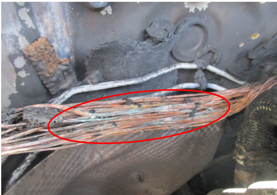
Photo 9 shows a close up view of the greenish residue found on the wirings (circled) at the rear centre portion of the engine compartment. The presence of such greenish residue suggests occurrence of an electrical short circuit.
