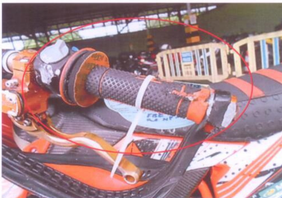
Photo 5 shows a closer view of the left handle of the Motorcycle at the time of our inspection. The Motorcycle was observed to have sustained with relatively minor damages due to the accident collision. (Circled)
