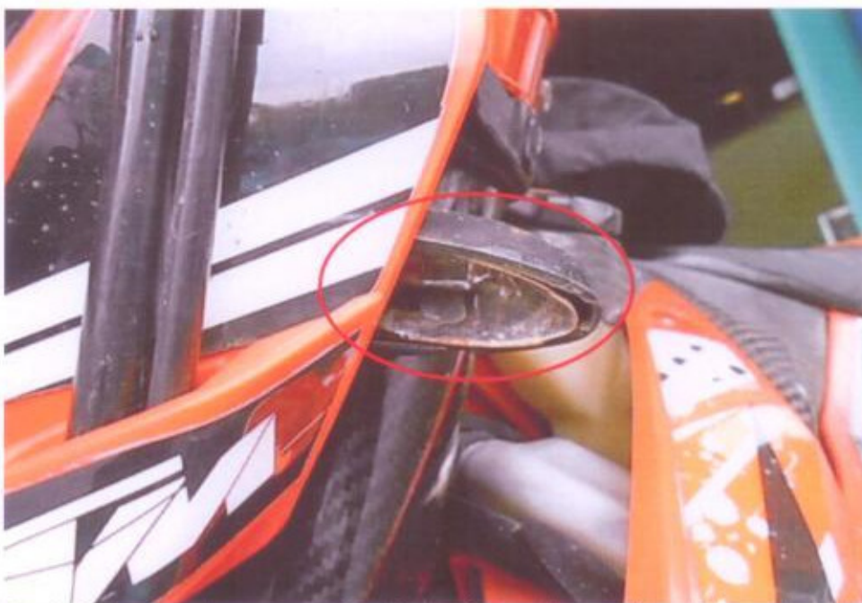
Photo 6 shows a closer view of the front left signal lamp of the Motorcycle at the time of our inspection. It was observed to be damage likely due to the accident. (Circled)
