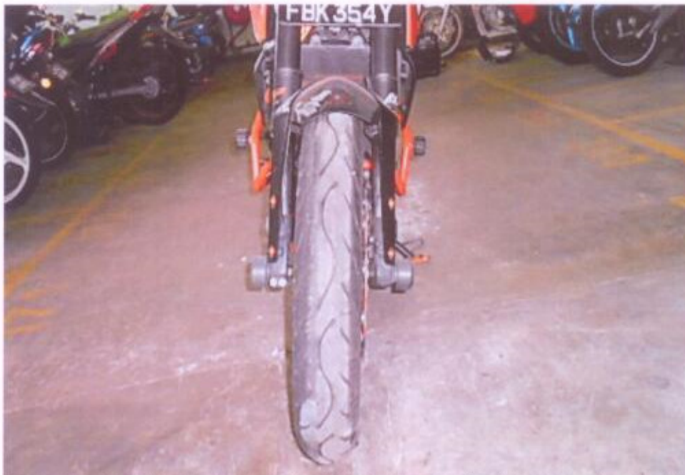
Photo 12 shows the front tyre of the Motorcycle. The front tyre was observed to be in serviceable condition with remaining tread depth of approximately 2mm. The tyre was also observed to be sufficiently inflated for vehicular operation.
