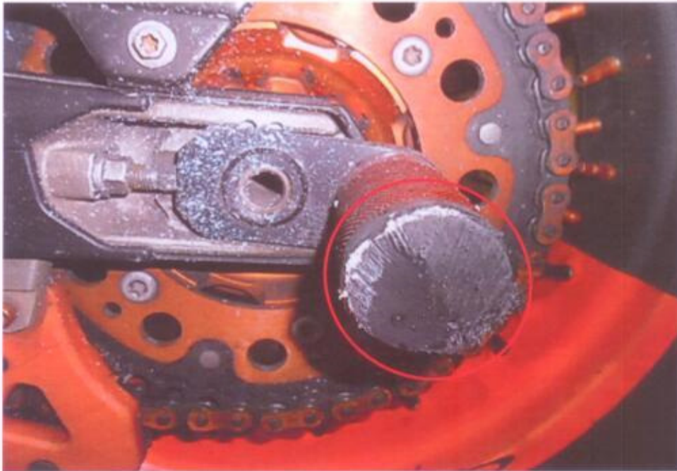
Photo 9 shows a closer view of the left rear wheel protector of the Motorcycle at the time of our inspection. It was observed to be damage due to the accident impact. (Circled)
