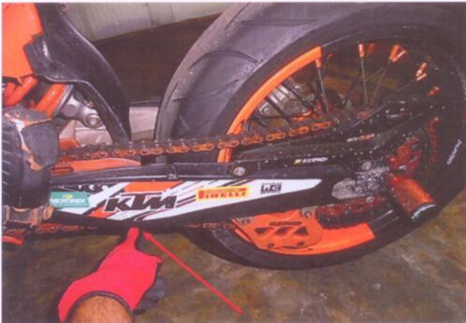
Photo 17 shows the general view of the gear train (arrowed) of the Motorcycle, which was observed to be intact with no misalignment. It was also adequately lubricated for operating purposes. Free play tension was also observed & found adequately acceptable.
