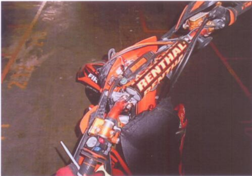
Photo 18 shows the steering system was observed to be in a serviceable condition. It was able to be steered to the full left & right at time of our inspection.
