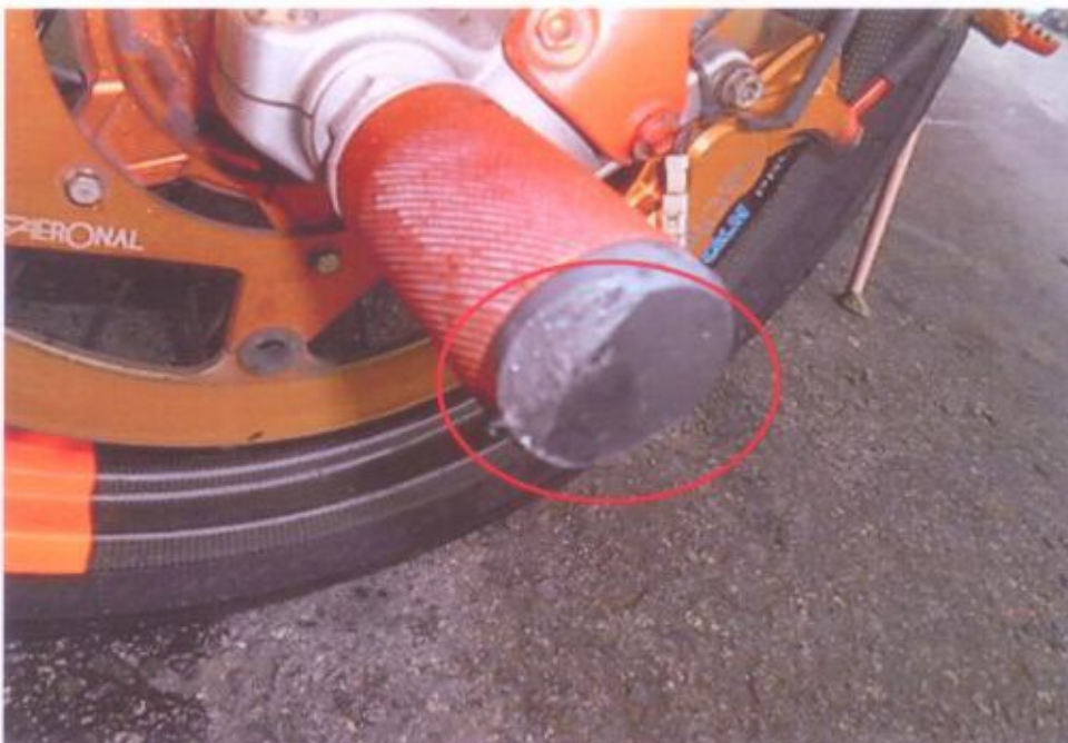
Photo 8 shows a closer view of the left front wheel protector of the Motorcycle at the time of our inspection. It was observed to be damage due to the accident impact. (Circled)
