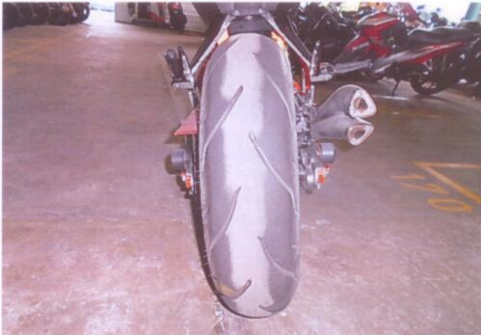
Photo 11 shows the rear tyre of the Motorcycle. The rear tyre was observed to be in serviceable condition with remaining tread depth of approximately 3mm. The tyre was also observed to be sufficiently inflated for vehicular operation.
