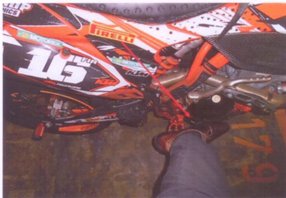
Photo 21 shows testing of the braking of the rear brake in progress. There was some resistance felt (spongy like feel) upon stepping on the brake pedal.
