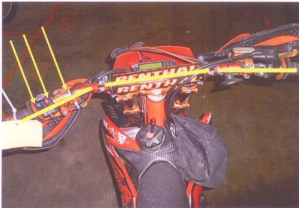
Photo 7 shows a close-up view of the front handle of the Motorcycle at the time of our inspection. It was observed to have sustained slight misalignment due to the accident collision. (Arrowed)
