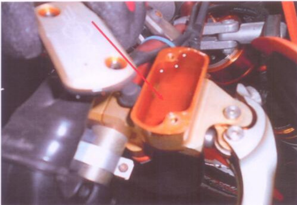
Photo 19 shows our checks on the brake fluid reservoir had also indicated that the brake fluid was of sufficient level for operational purposes, and without contamination.
