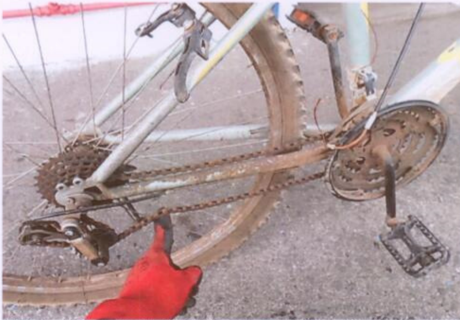
Photo 12 shows a close-up view of the rear chain of the Bicycle at the time of our inspection. It was observed to be out of tension at time of our inspection.
