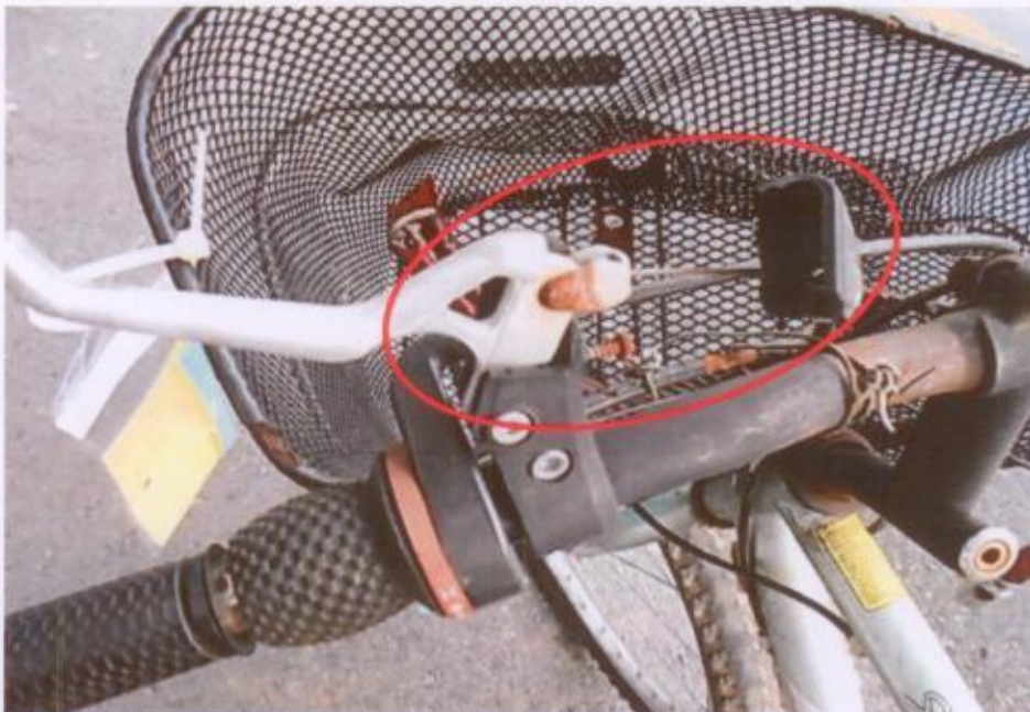
Photo 6 shows a close-up view of the rear brake lever of the Bicycle at the time of our inspection. It was observed to be damage at the rear brake lever of the Bicycle likely due to the accident.
