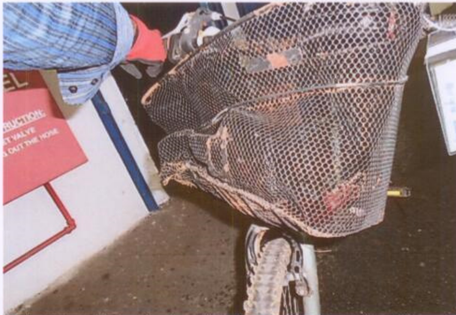
Photo 3 shows the front basket of the Bicycle at time of inspection. Damage on the front basket was observed likely due to the accident.
