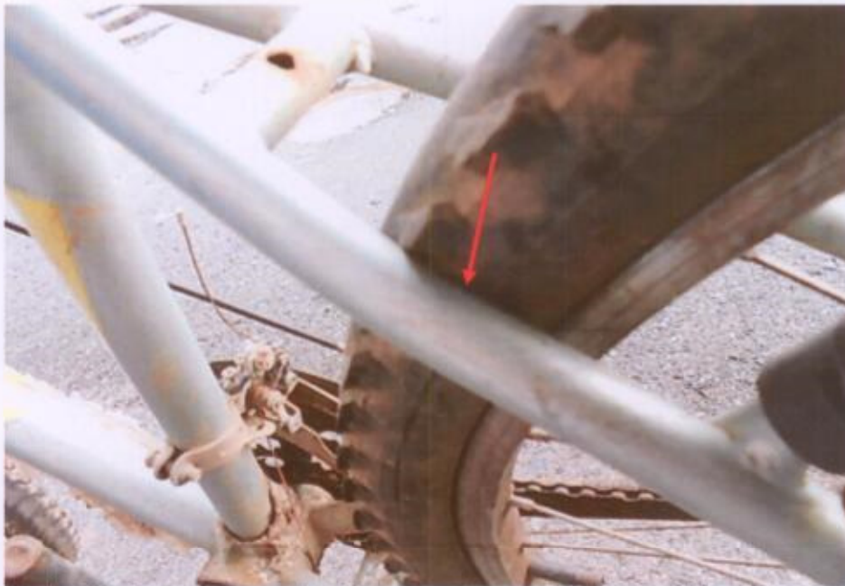
Photo 14 shows the rear fork that was observed to have sustained damages likely due to the accidents impact.
