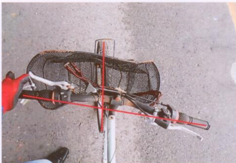
Photo 4 shows the frontal portion of the Bicycle (top view) at time of inspection. Misalignment of the handle bar & front tyre was observed.
