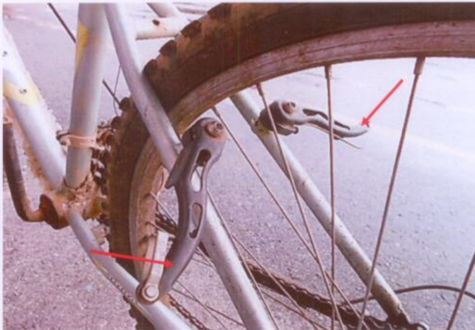
Photo 18 shows the rear brake clamp that was seen dislodged from the original assembly.
