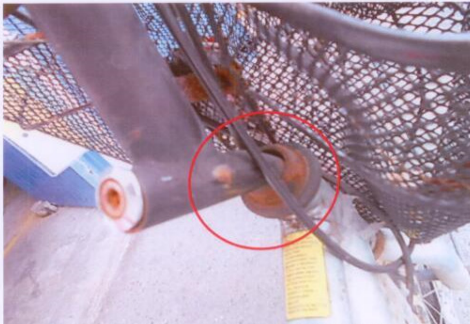
Photo 13 shows the front fork that was observed to have sustained damages likely due to the accidents impact.
