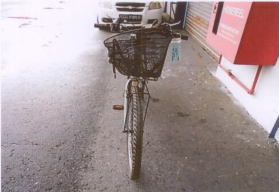
Photo 10 shows the front tyre of the bicycle. The tread pattern of the front tyre was observed only visible on the sides of the tyre, the middle section of the tyre was observed to be bald.
