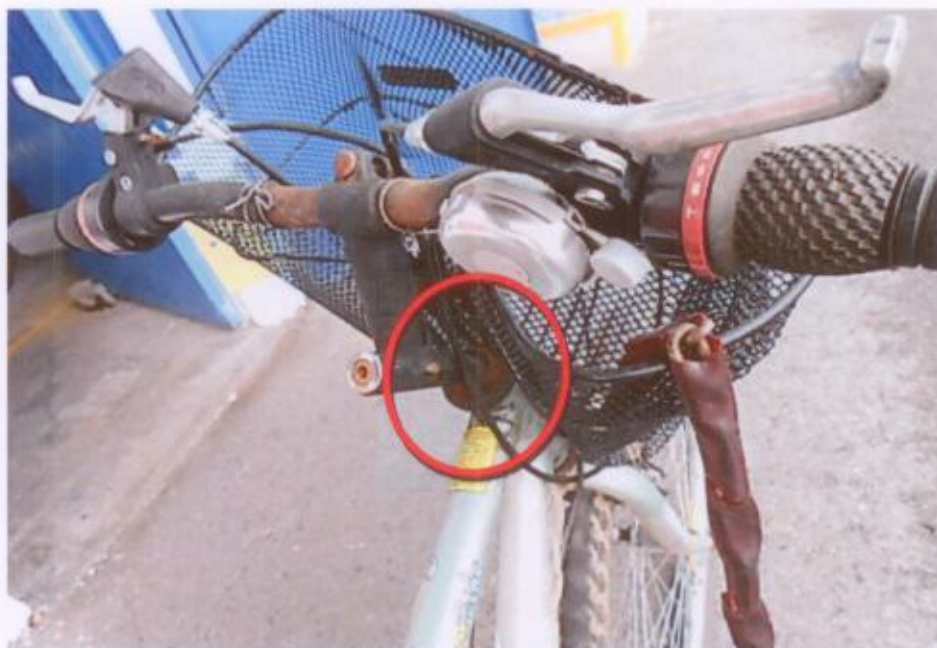
Photo 2 shows the frontal portion of the Bicycle at time of inspection. Damage on the handle & fork connecting bar was observed likely due to the accident.
