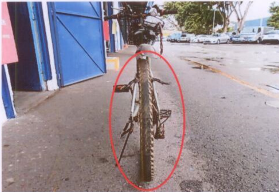
Photo 8 shows the rear tyre of the Bicycle at the time of our inspection. The tread pattern of the rear tyre was observed only visible on the sides of the tyre, the middle section of the tyre was observed to be bald.
