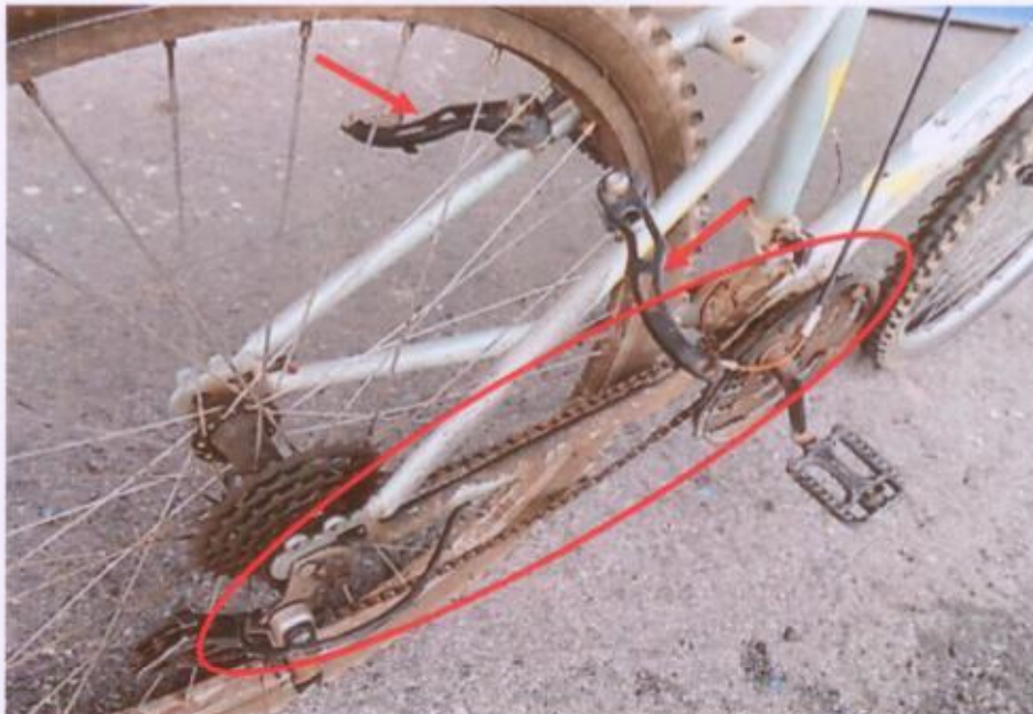
Photo 5 shows a close-up view of the chain gear of the Bicycle at the time of our inspection. It was observed to be out of tension at time of our inspection (circled). The rear brake clamp was also found to be dislodging from the original assembly.
