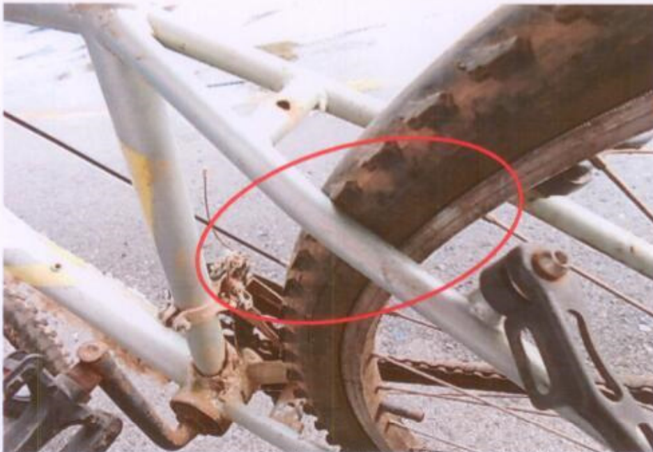
Photo 7 shows a close-up view of the rear tyre of the Bicycle at the time of our inspection. It was observed to be pushed against the rear fork of the Bicycle likely due to the accident.
