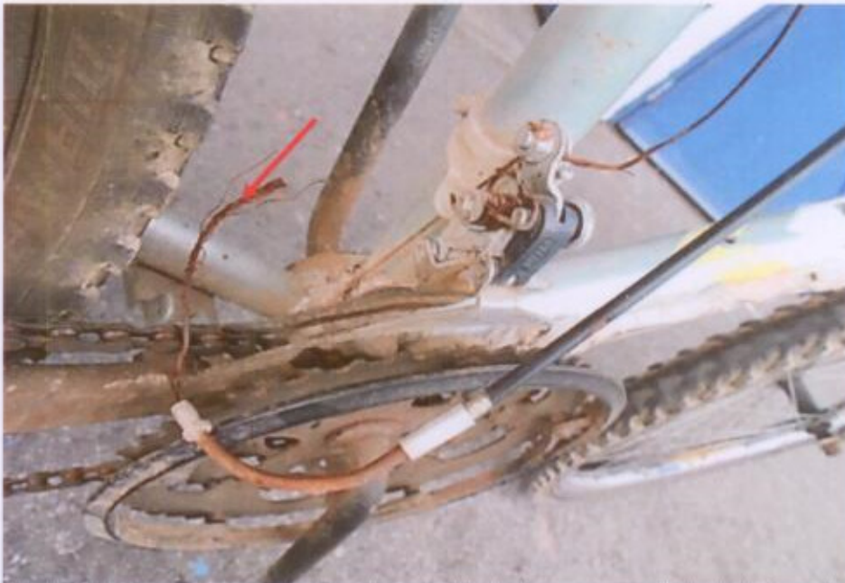
Photo 17 shows the rear brake clamp cable that was seen dislodged from the original assembly.
