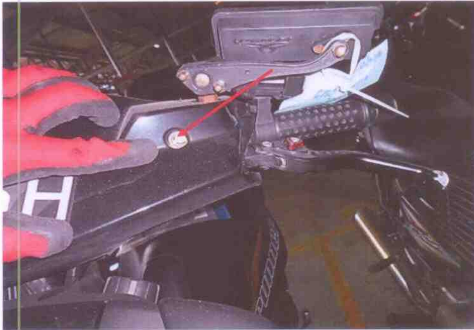
Photo 20 shows the left hand brake fluid reservoir on the Motorcycle that indicates that it was sufficient at time of inspection.
