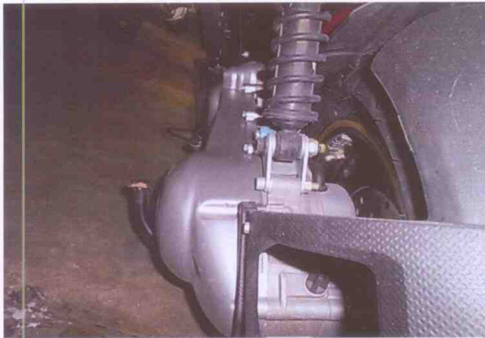
Photo 15 shows the drive train of the motorcycle was found to be intact without any misalignment.
