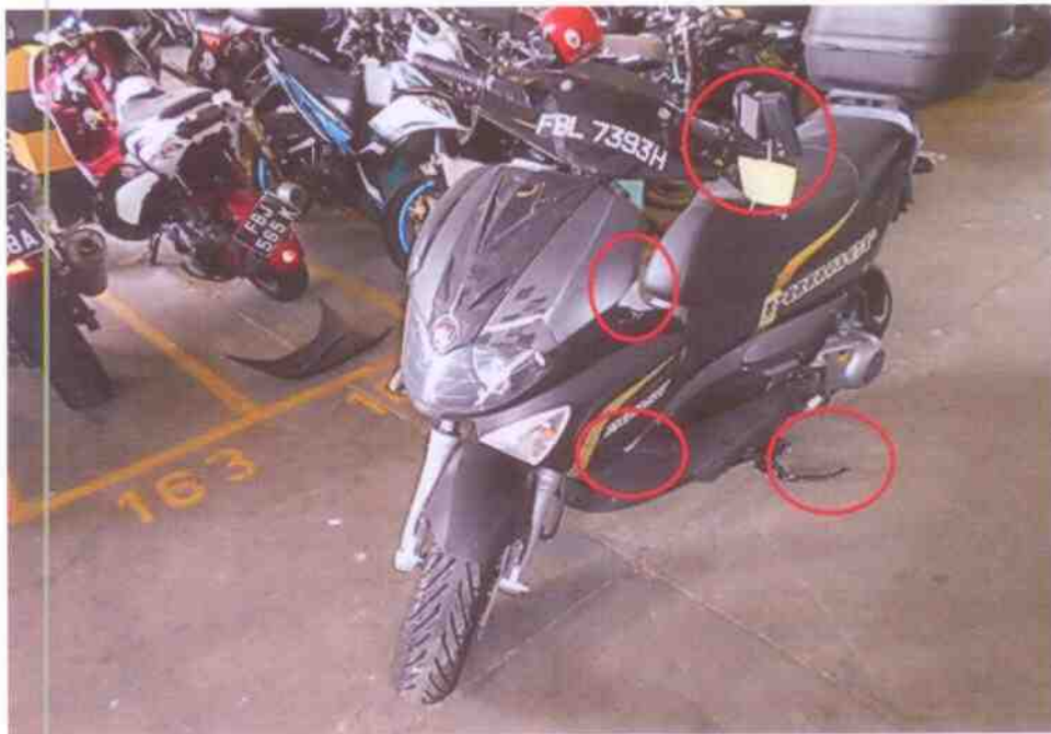
Photo 3 shows a general view of the front left body of the Motorcycle at the time of our inspection. The Motorcycle was observed to have sustained minor damages at the frontal portion & along its left side. (Circled)
