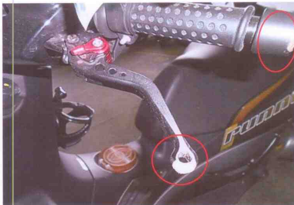
Photo 4 shows a closer view of the frontal portion of the Motorcycle at the time of our inspection. The Motorcycle was observed to be sustained relatively minor impact due to the accident collision. (Circled)
