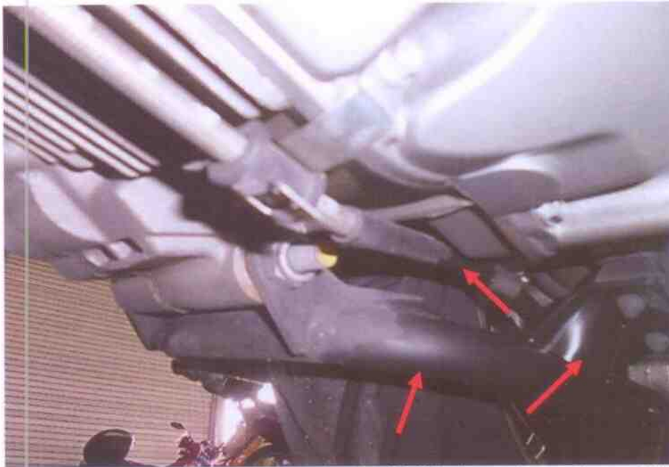
Photo 13 shows was sign(s) or indication(s) of fluid leakage observed around the engine undercarriage area of the Motorcycle.
