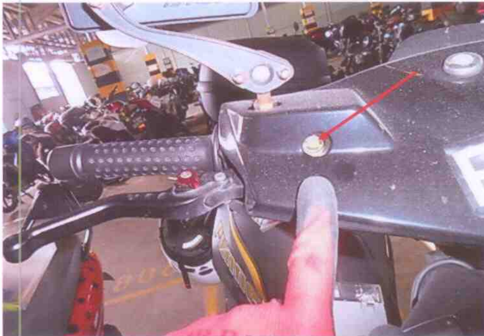
Photo 19 shows the right hand brake fluid reservoir on the Motorcycle that indicates that it was sufficient at time of inspection.
