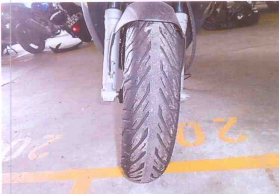
Photo 11 shows the front tyre of the Motorcycle. The pattern of the tread was clearly visible. There was no tear, burst mark(s) and/or punctured hole(s) on the sidewalls as well as across the tread of the front tyre.
