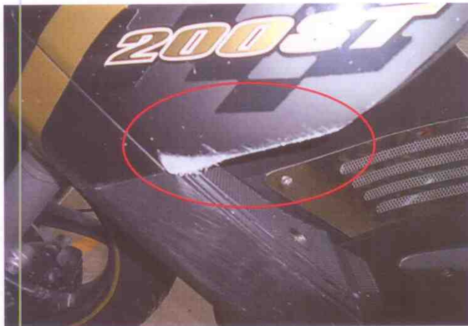
Photo 6 shows a closer view of the left portion fairing of the Motorcycle at the time of our inspection. It was observed to have sustained deep grazing mark due to the accident collision. (Circled)
