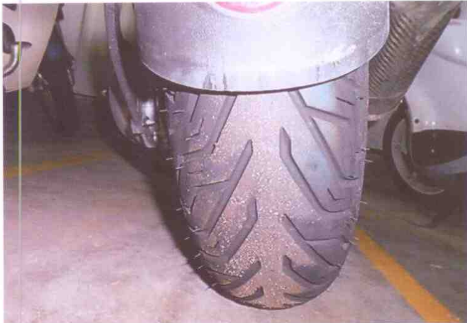
Photo 10 shows the rear tyre of the Motorcycle. The rear tyre was observed to be in serviceable condition with remaining tread depth of approximately 4mm. The tyre was also observed to be sufficiently inflated for vehicular operation.
