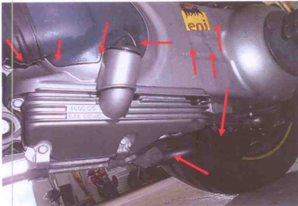
Photo 12 shows was sign(s) or indication(s) of fresh fluid leakage observed around the engine area of the Motorcycle.
