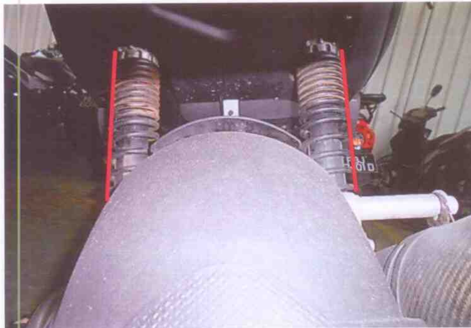
Photo 14 shows the rear shock absorber of the motorcycle was found to be intact without any misalignment.
