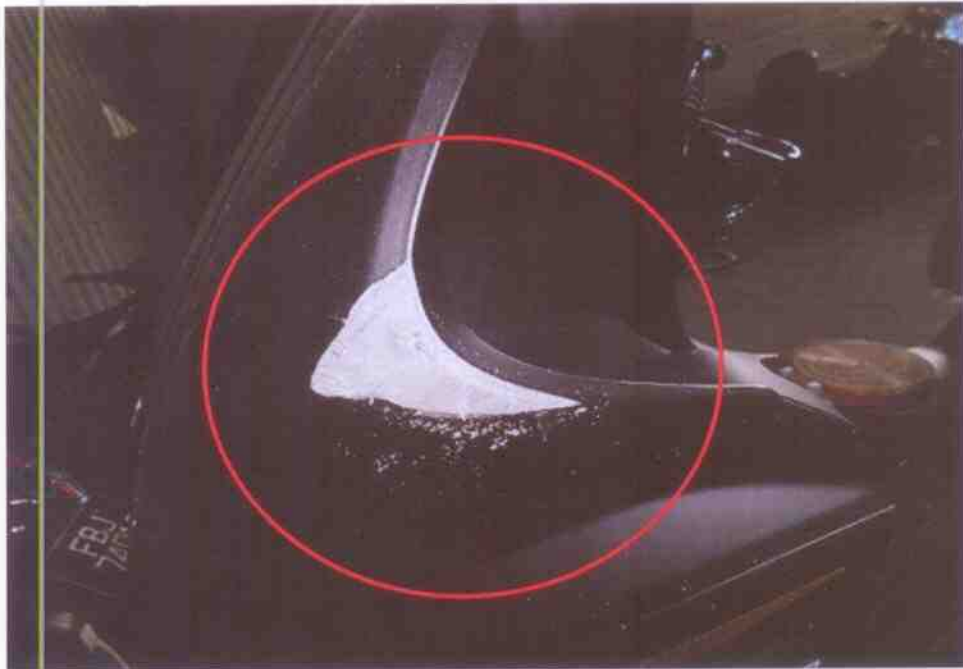
Photo 5 shows a closer view of the left portion fairing of the Motorcycle at the time of our inspection. It was observed to have sustained deep grazing mark due to the accident collision. (Circled)
