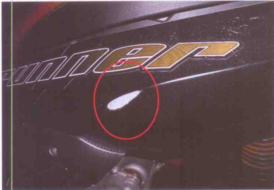
Photo 7 shows a closer view of the left portion fairing of the Motorcycle at the time of our inspection. It was observed to have sustained deep grazing mark due to the accident collision. (Circled)
