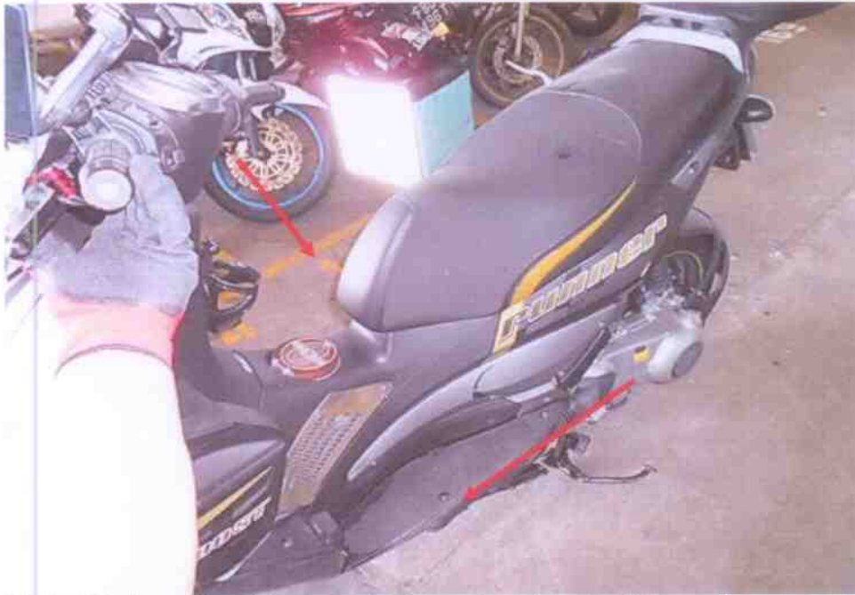
Photo 18 shows the static brake tests conducted on the Motorcycle rear brake had appeared to indicate that the brake system of the Motorcycle was in serviceable condition. There was some resistance felt (spongy like feel) upon pressing the brake lever at the right side of the handle bar.
