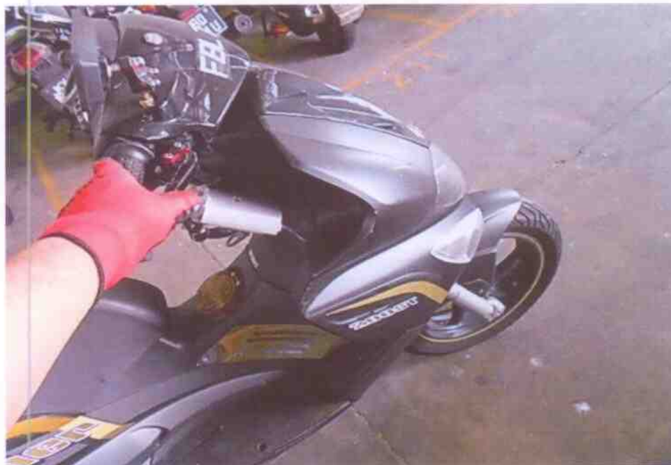
Photo 17 shows the static brake tests conducted on the Motorcycle front brake had appeared to indicate that the brake system of the Motorcycle was in serviceable condition. There was some resistance felt (spongy like feel) upon pressing the brake lever at the right side of the handle bar.
